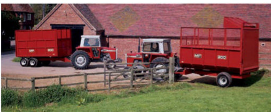
MF's 200 range followed the Weeks-built 20 to 26 models and comprised numerous models from 3 to 10 tonnes. The smallest of the dropside trailers able to be fitted with silage sides was the 4-tonne model, with a capacity of 296.7cu ft, while the largest was the 8.5-tonne mode – able to hold 621cu ft. The monocoque models ranged from 6.5-10 tonnes and could hold 620.4-815.7cu ft of grass. The 5-tonne dropside model, in basic silage configuration, cost £1,567 in July 1979. Photo: AGCO.
