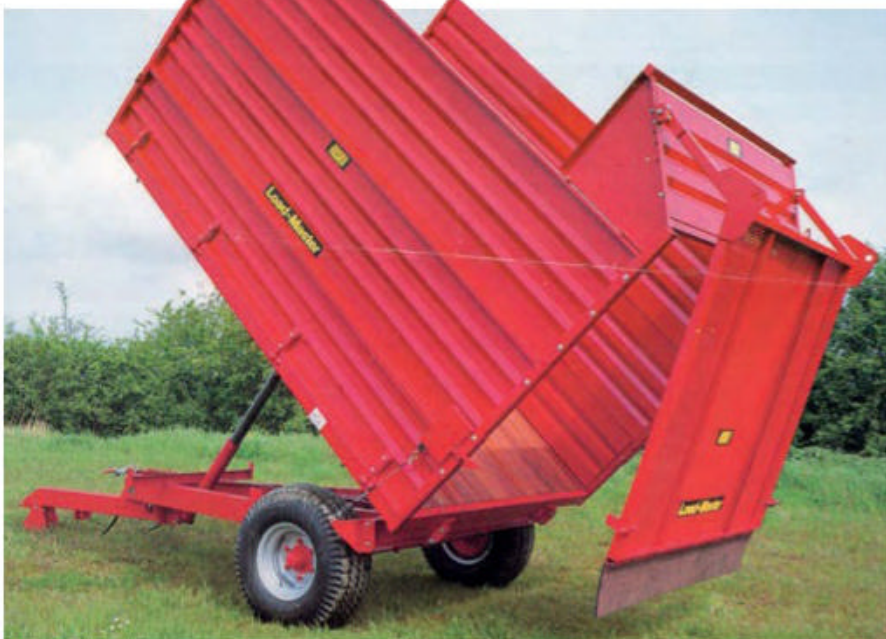
Foster (Farm Equipment) Ltd.'s 4- and 5-tonne models featured 1ft 6in sides as standard, with 1ft 6in grain extensions available. The 5-tonne 'ST' model shown also features the additional 2ft 8in silage sides. The capacity in this configuration was 381cu ft. Note: ST denotes steel sides, timber floor – where the timber was tongue and grooved Keruing, treated with linseed oil.
