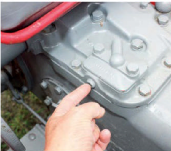
Oil for external hydraulic use can be tapped from this point, or external selector valves fitted to the transfer cap shown here.
