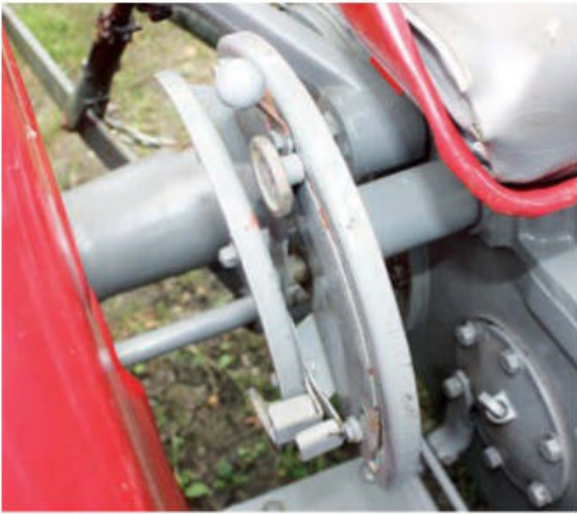
This view shows the control quadrant, with the operational lever and draft lever close to hand for easy operation.
