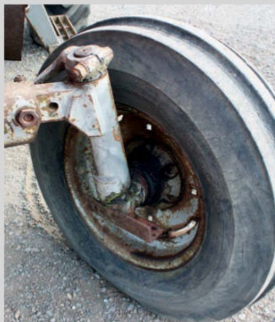
Check for the usual wear and tear on kingpins, as well as wheel bearings and the axle pivot.
