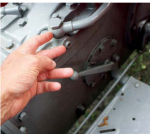
The trailer tipper pipe and a further tapping point are located on the left-hand side of the hydraulic top cover.
