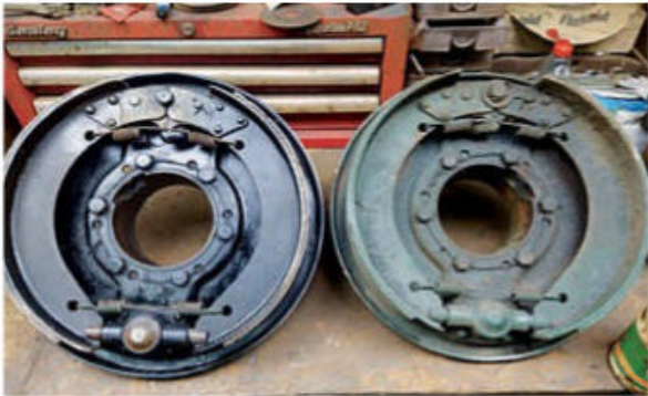
The brake mechanisms before (right) and after they were overhauled.
