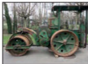
Gooseneck roller Le Marais – single cylinder Deutz hopper cooled
