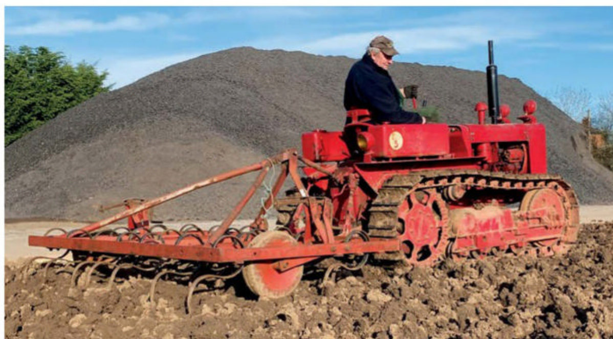
The three-point linkage allowed a variety of implements to be used in conjunction with the BTD-5. Photo: David Fenton.
