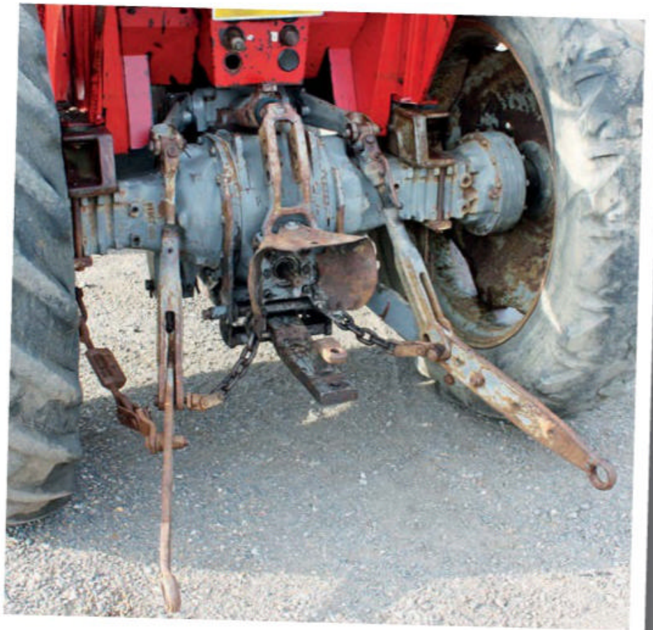
Look out for seized levelling boxes, welded drop arms and damaged ball ends – all of which this tractor has! Also note the lack of a pick-up hitch. Make enquiries before viewing a tractor if this feature is important to you.
