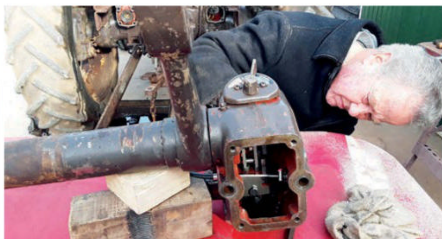
Left: You can't sort out the Selectamatic hydraulic system without stripping it down this far, Peter says. Right: Cliff Price undertaking surgery!
