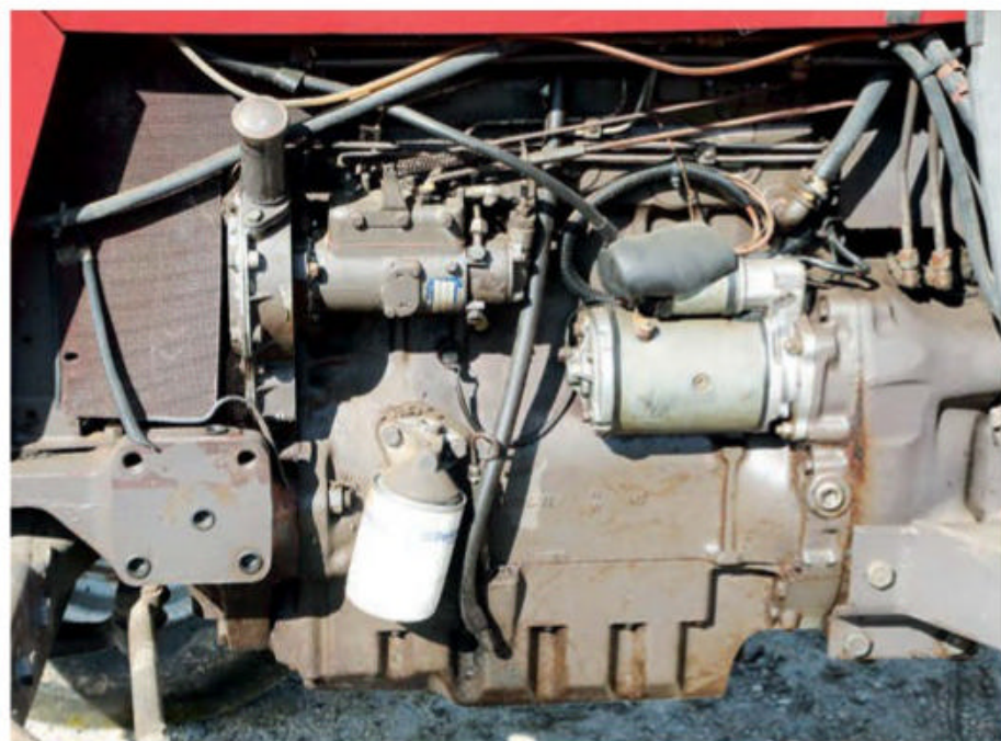
The Perkins A4.236 four-cylinder motor fits neatly under the bonnet. The starter has been replaced recently, but the engine is in fine fettle.
