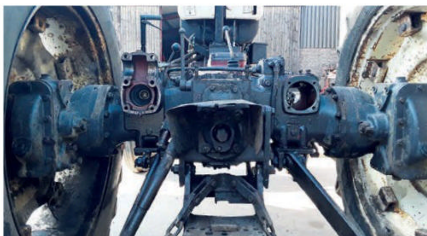
Left: You can't sort out the Selectamatic hydraulic system without stripping it down this far, Peter says. Right: Cliff Price undertaking surgery!
