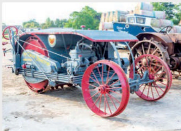
The Gray 18-36 Drum Drive with replacement Hercules four-cylinder engine, which came from a generator set, sold for £23,000.
