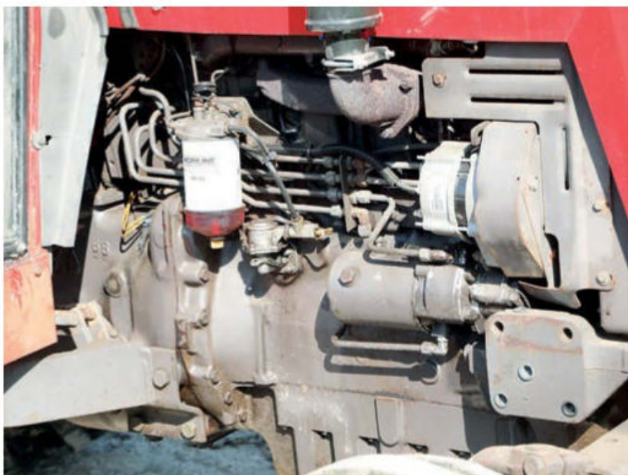
The Perkins A4.236 four-cylinder motor fits neatly under the bonnet. The starter has been replaced recently, but the engine is in fine fettle.
