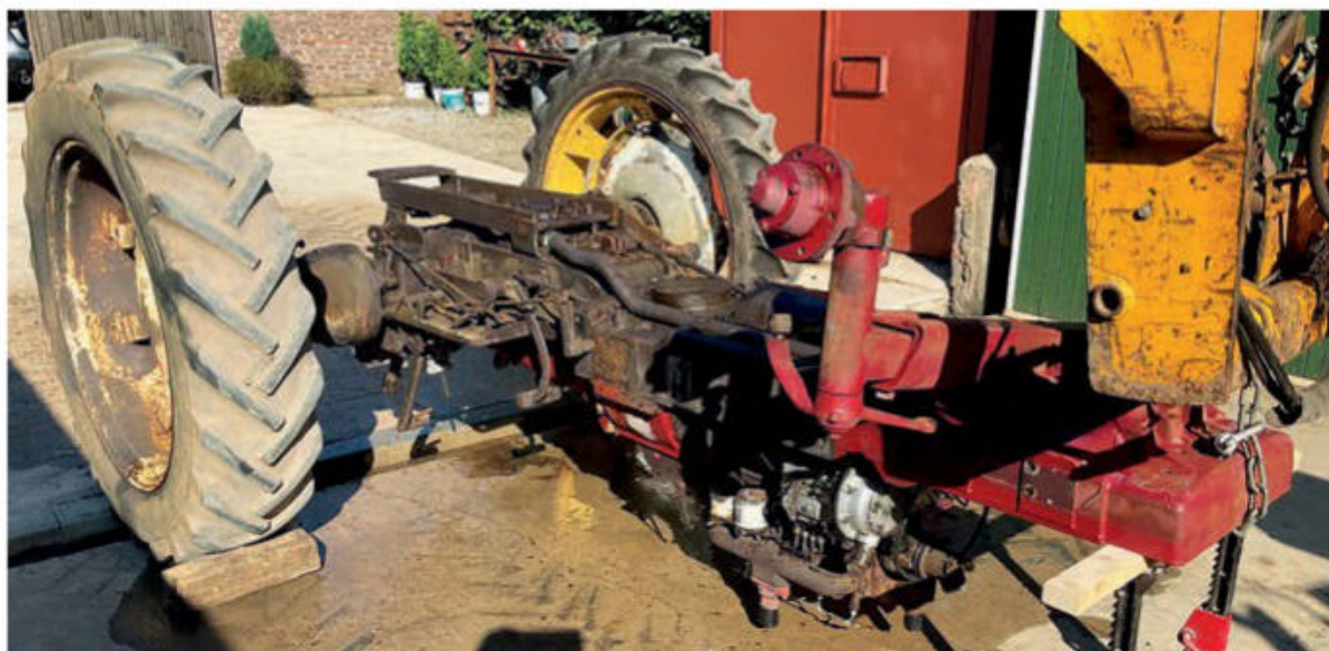
With the tractor stripped to the skid unit, a JCB Loadall was used to invert it. This enables the underside to be cleaned and painted easily.
