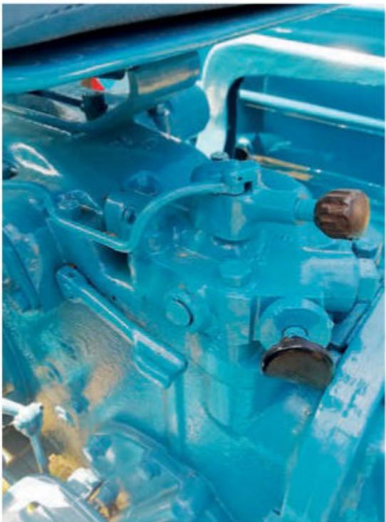
Top: Main hydraulic control quadrant, which is raised to lift the linkage and lowered to drop the linkage, and is used for both position (height control) and Qualitrol (depth control). Above: This shows the horizontal lever that selects either Qualitrol, when set vertical, or position, when set as seen in the horizontal position. The lower black knob is the auxiliary services selector knob, whilst the upper black knob is the oil flow response control, which is overridden when the quadrant lever is fully raised.
