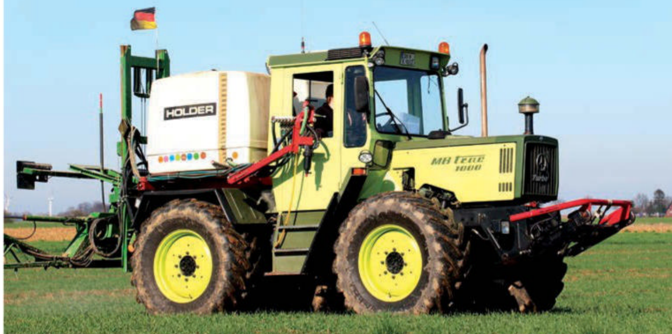
On this Holder spraying rig mounted to an MB-trac 1000, the openable door window is put to good use for operating the sprayer controls. Judging by the 'Turbo' badge on the grille, this tractor has had its power boosted by the fitting of an aftermarket turbocharger.
