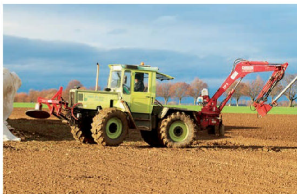
Left: With front loader attached, the equal-size wheel, four-wheel drive MB-trac 1000 is a formidable performer, being a relatively compact, yet powerful machine capable of a fast turn of speed. Right: This MB-trac 1000 is equipped with special implements used for covering sugar beet clamps to protect the crop from frost damage. The integrated front linkage was a very useful part of the MB-trac design.
