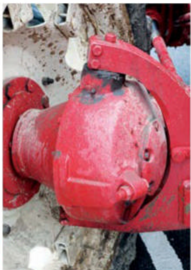
Left: The front hubs are typical County products, driven by telescopic shafts running parallel to the skid unit. Middle: The correct-style DPA injection pump was fitted to obtain the right power output. Earlier examples were fitted with a Simms inline unit. Right: IH equipped the 634 with a lower link-sensed, Vary-Touch hydraulic system and it became famed for its draft ability and pulling power.
