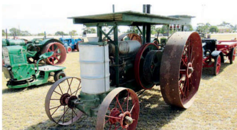
This Jelbart dates from 1916. The piston is stepped like a top hat, with a large base and a small crown. It was used on a training farm for returned soldiers at Melrose, at the close of WW1.
