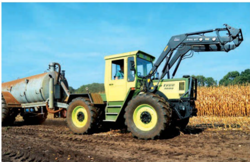
Left: With front loader attached, the equal-size wheel, four-wheel drive MB-trac 1000 is a formidable performer, being a relatively compact, yet powerful machine capable of a fast turn of speed. Right: This MB-trac 1000 is equipped with special implements used for covering sugar beet clamps to protect the crop from frost damage. The integrated front linkage was a very useful part of the MB-trac design.
