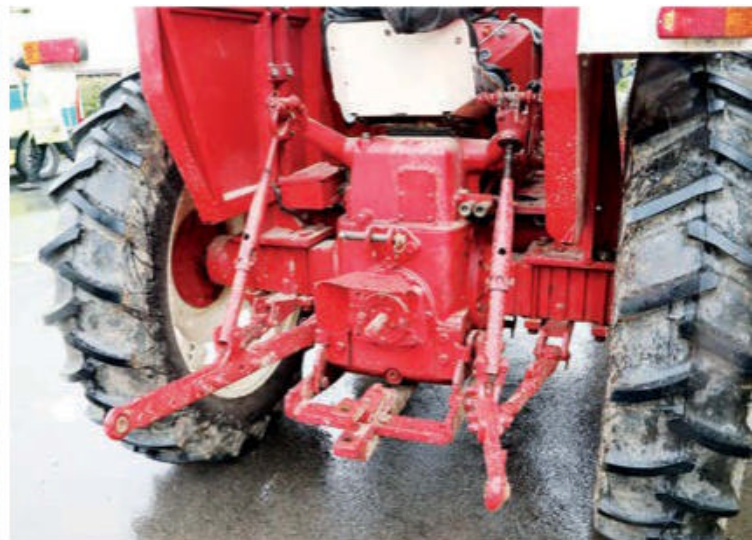
Left: The front hubs are typical County products, driven by telescopic shafts running parallel to the skid unit. Middle: The correct-style DPA injection pump was fitted to obtain the right power output. Earlier examples were fitted with a Simms inline unit. Right: IH equipped the 634 with a lower link-sensed, Vary-Touch hydraulic system and it became famed for its draft ability and pulling power.
