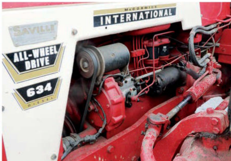
Left: The front hubs are typical County products, driven by telescopic shafts running parallel to the skid unit. Middle: The correct-style DPA injection pump was fitted to obtain the right power output. Earlier examples were fitted with a Simms inline unit. Right: IH equipped the 634 with a lower link-sensed, Vary-Touch hydraulic system and it became famed for its draft ability and pulling power.
