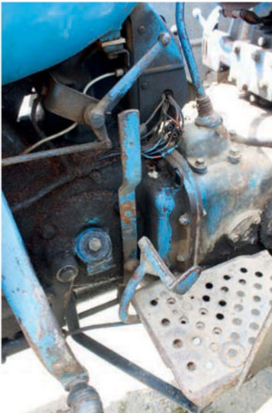
The vertical PTO lever has to be engaged to operate the hydraulic system of the tractor. To allow separate engagement of the PTO a raised PTO unit was required as an accessory.
