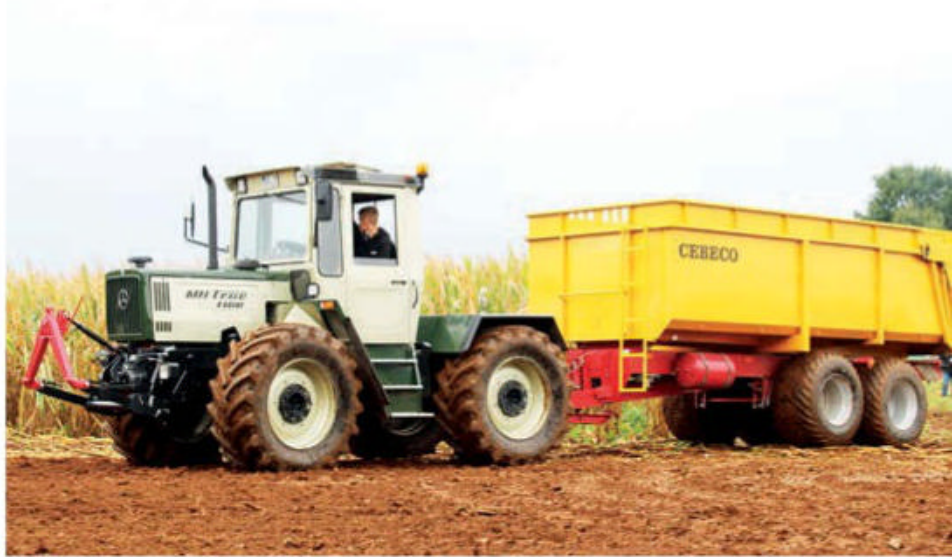
Left: The MB-trac 1100 joined the 1000 in 1987 as the second member of the middleweight series. With 110hp available from its six-cylinder Mercedes-Benz engine, the 1100 built on the success of the earlier 1000 and was ideal for top work roles, such as using front coil packers and rear-mounted combination drills. The fitting of dual wheels all round also helped the tractor tread even more softly. Right: Haulage is perhaps one of the best-known applications for the quick and comfortable MB-trac. The 1100 used the same lengthened chassis that was used for the 1000 but, thanks to more power, it was capable of even more versatility than its stablemate.
