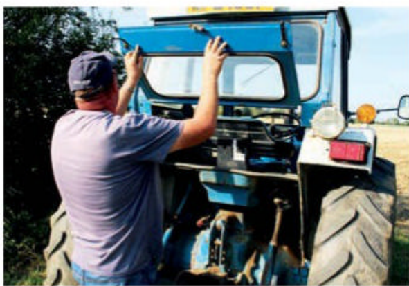
Left: Jonathan demonstrating how the bottom section of the cab window can be folded back up and latched into place. Middle: Often lost or damaged, this 5600 still has both side lights mounted on stalks in front of the cab. Right: The back end features a two-speed IPTO.
