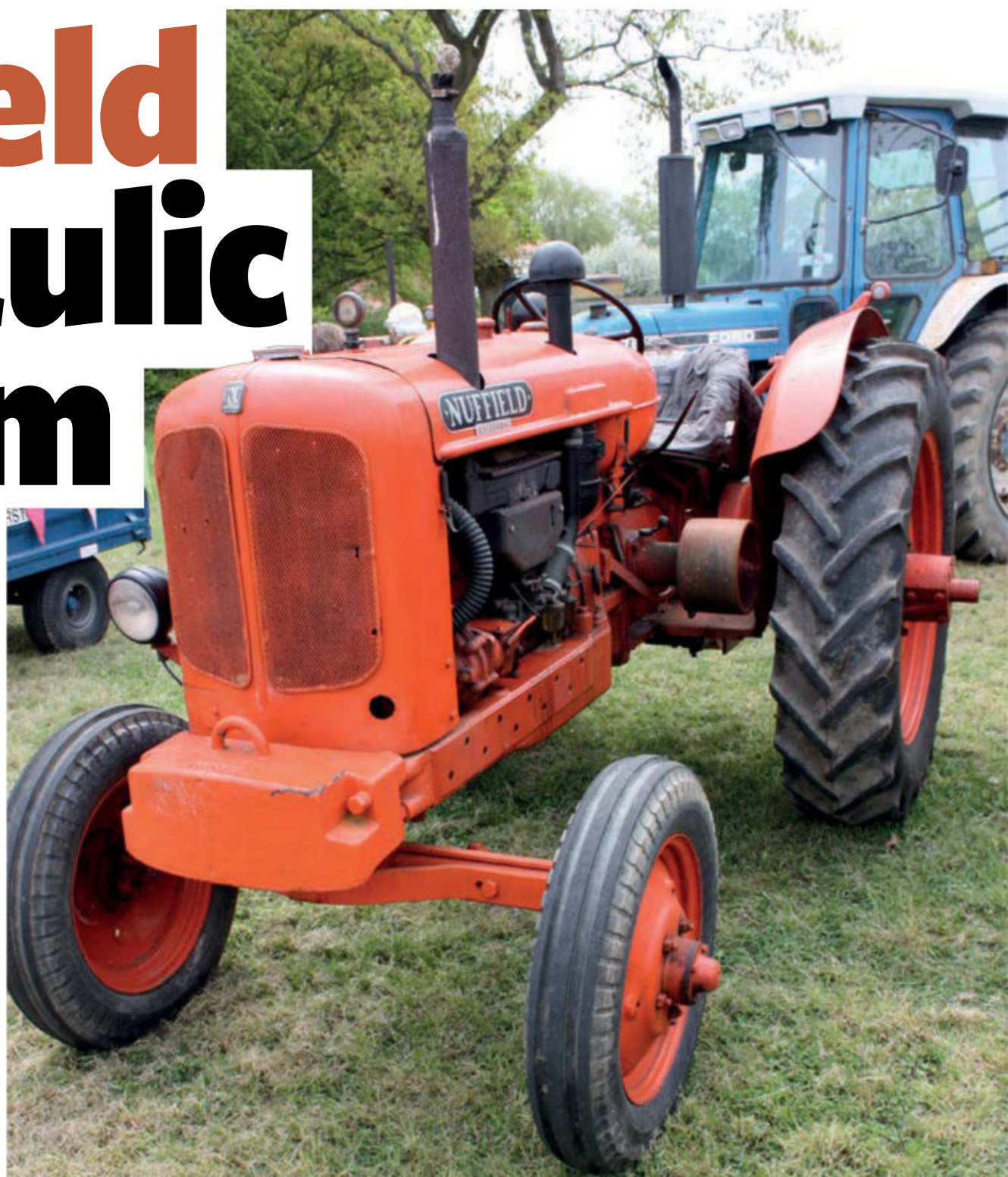
The Nuffield Universal tractor was introduced in late 1948 and featured a hydraulic lift and category two three-point linkage as an option, which remained unchanged until modified to incorporate draft control in 1961 on the 342 and 460 models.
