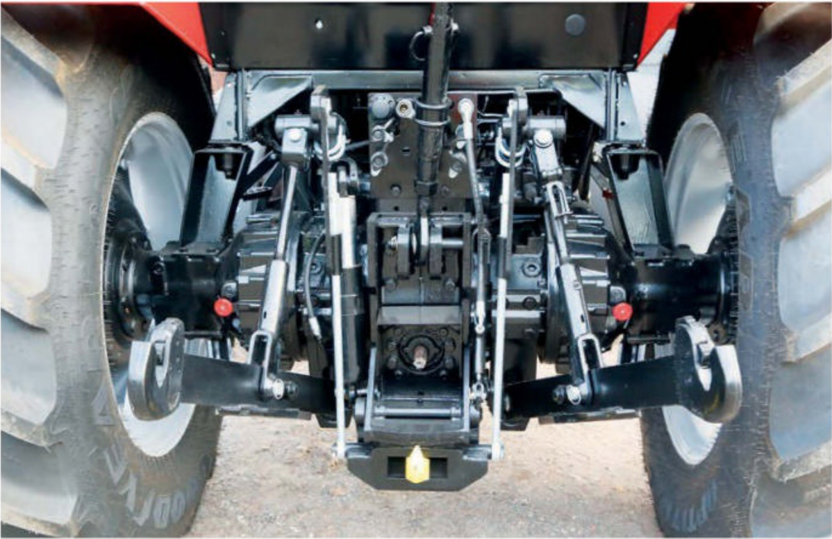
The rear end revealed that the tractor had a hard working life in Spain, but the problems have been rectified and a Dromone pick-up hitch has been fitted.
