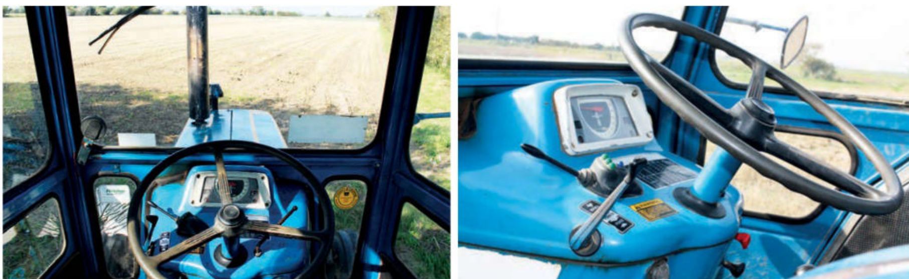
Left: The Fieco safety cab allows for good vision, with plenty of glass making it feel light and airy, and not as enclosed as many of the older weather cabs tended to do. Even on a 1976 tractor at the very end of its career, the cab was seen as a good, if rather noisy, place to spend a working day. Right: The dashboard of the 7A1 range would be familiar to any drivers of the earlier Force range. Note the Dual Power lever in the foreground providing clutch-less changes on the move between high and low in each of the eight main ratios.
