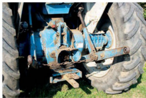
Left: Jonathan demonstrating how the bottom section of the cab window can be folded back up and latched into place. Middle: Often lost or damaged, this 5600 still has both side lights mounted on stalks in front of the cab. Right: The back end features a two-speed IPTO.
