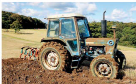
Larry Cooke, from Co. Cavan, with his 1980 County 6600-Four. This tractor has Dual Power and a creeper gearbox fitted.
