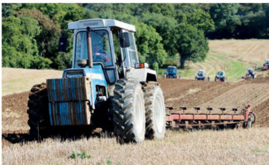
Richard McDonald driving Ken Cooke's 1974 County 1454 with a Kverneland nine-furrow spring-release plough. Ken has made sure that this tractor has plenty of nose weights fitted, to aid traction when going uphill with a large plough.
