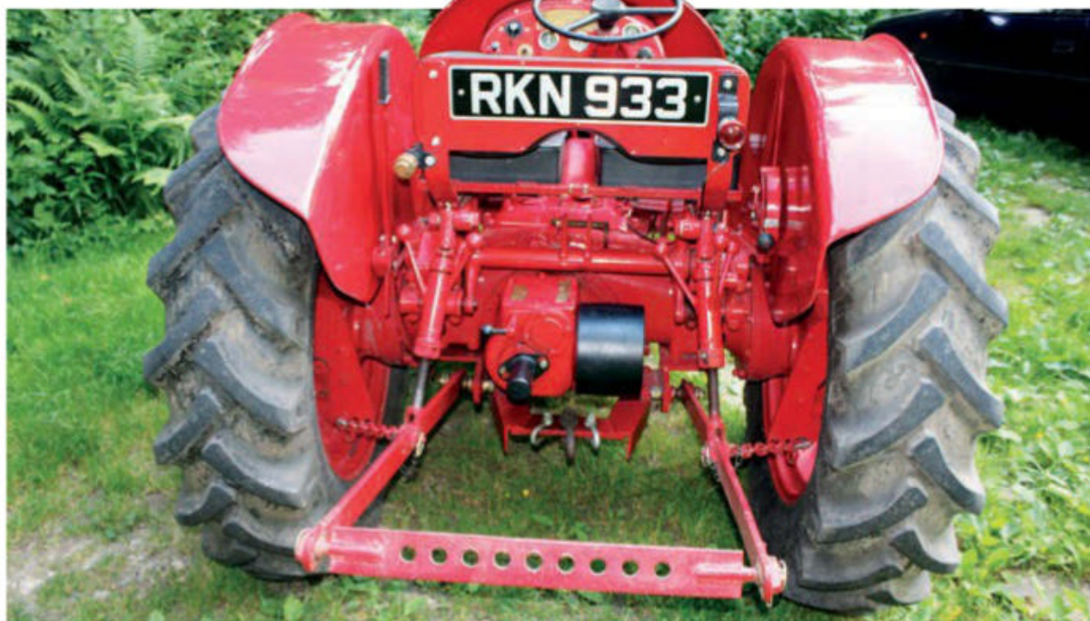
The drawbar is removed, and link arms fitted for three-point linkage operation, as seen here. This is a Super Cropmaster, which has the later MkII hydraulic system and lift lever.
