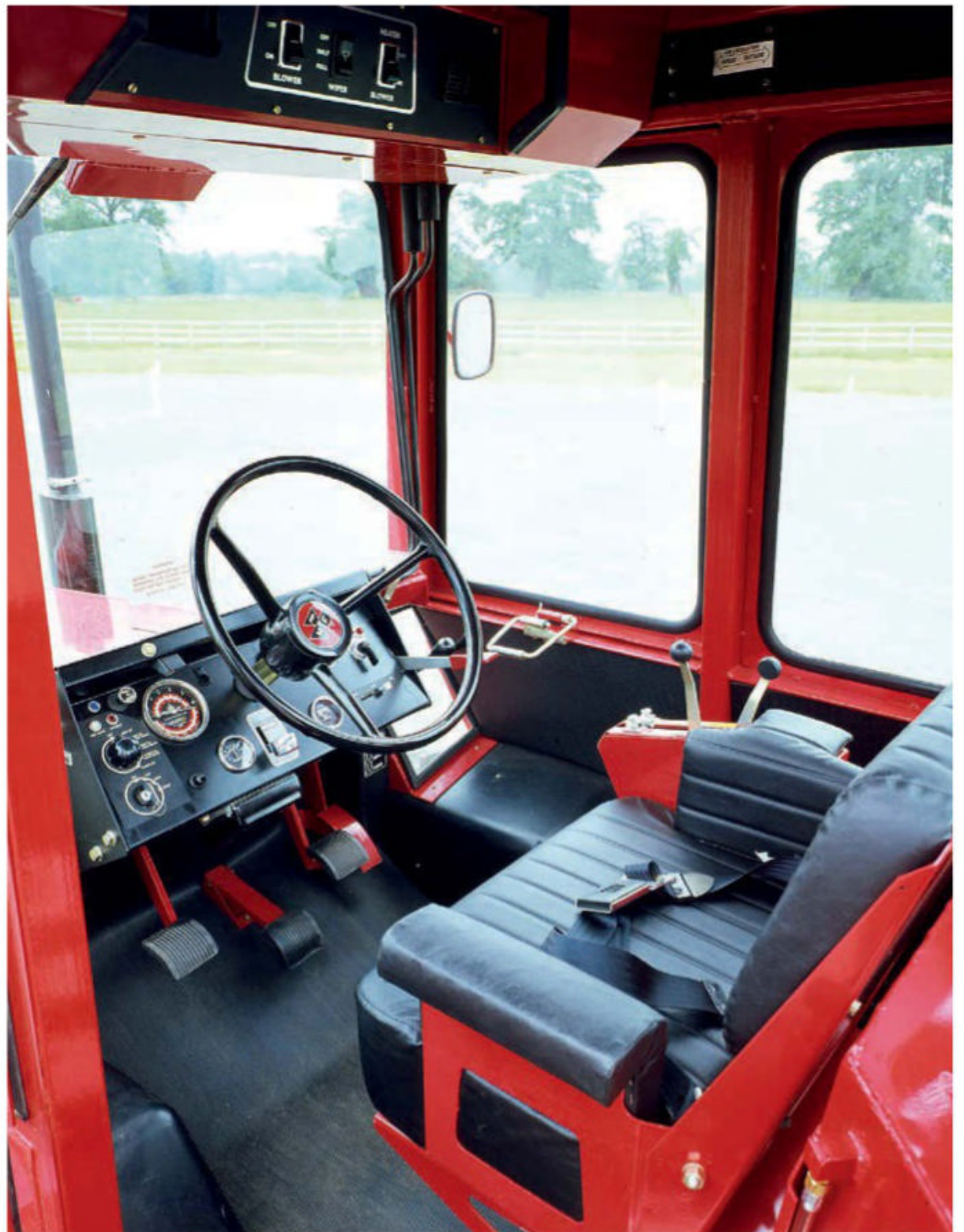
The cab for the MF 1200, built by Cab Craft, was rubber mounted, with a flat floor and pendant pedals. The hydraulic controls were positioned within the arm rest, and in a bid to retain the uncluttered feel, the blower controls were mounted above the operator's head.
