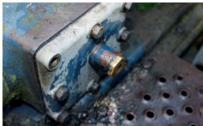
Oil for tipping trailers or front-end loaders can be supplied via this ½-inch BSP tapping point, which is controlled by the same main control lever.
