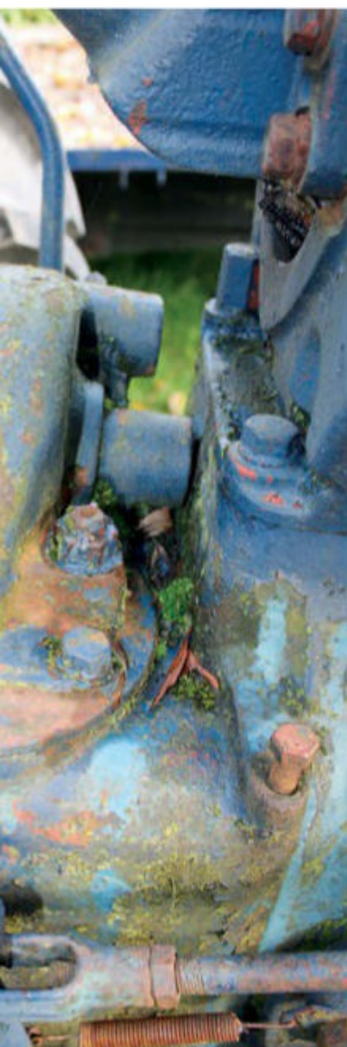
Full movement clockwise is the implement lift position. The lever is held whilst lifting. There is no intermediate height – it's either fully raised or lowered!
