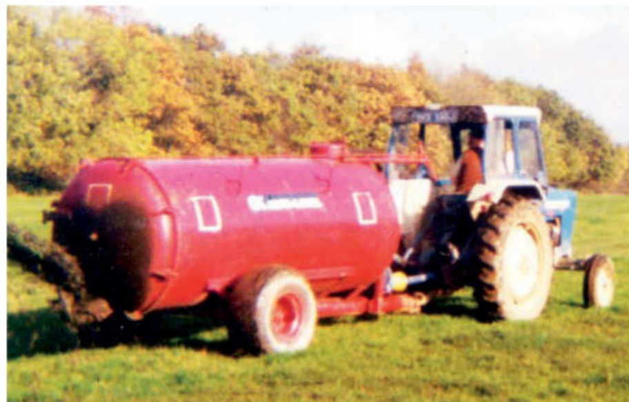
Above: While the milking herd was still in residence, there was a great deal of slurry generated from the cattle yards. The farm did not have its own vacuum tanker and instead hired one in to clear out an underground slurry tank every month during the winter, and slightly less often during the rest of the year. Here the trusty 4000 is using an Alfa-Laval tanker to do the job.
