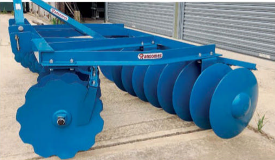
Paul’s disc harrow is fitted with 20in (50cm) discs – cutaway (scalloped) at the front and plain at the rear.
