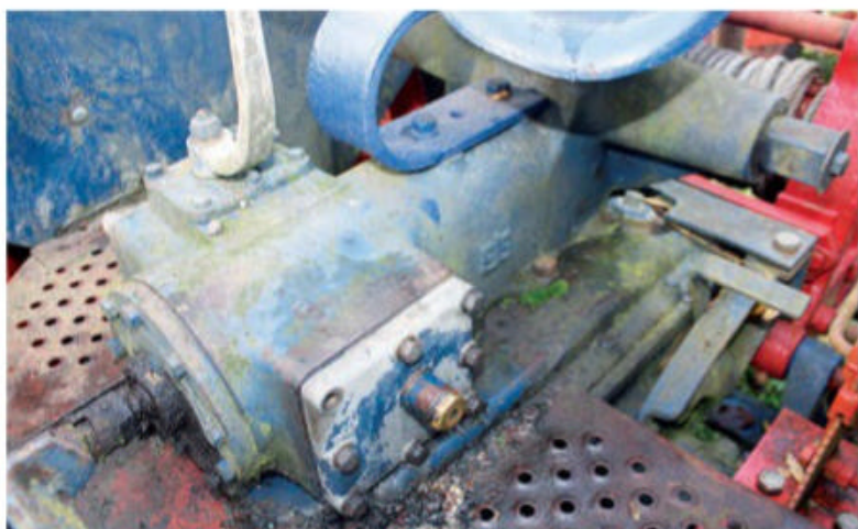
The Smith lift was designed as a self-contained unit, which bolted onto the rear axle top cover and allowed the use of a category two three-point linkage.
