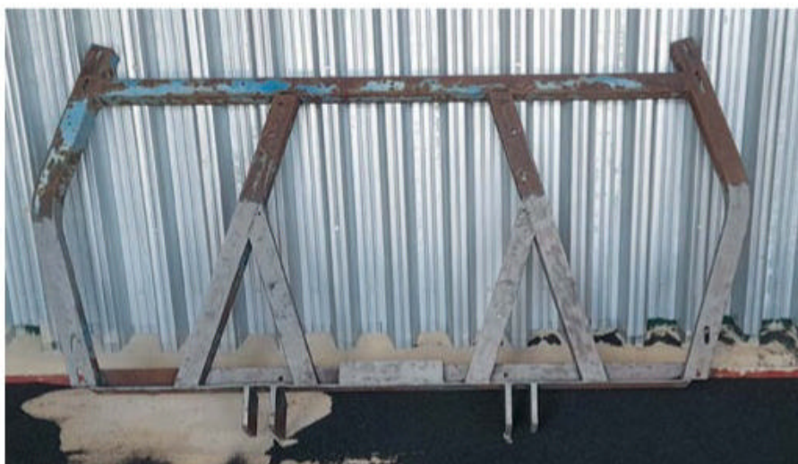
Shot blasting made short work of the rust.
