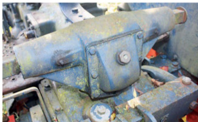
Oil is filled via this plug in the rear cover. Note the three-point linkage has been removed to accommodate a winch.
