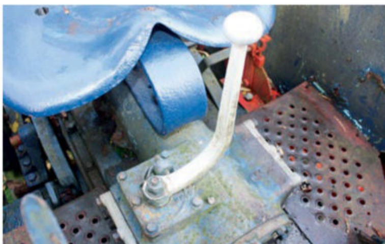
An aluminium or fabricated steel lever is the main control for raising and lowering implements or operating external hydraulic services as required.
