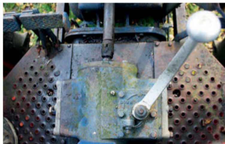
Full movement clockwise is the implement lift position. The lever is held whilst lifting. There is no intermediate height – it's either fully raised or lowered!
