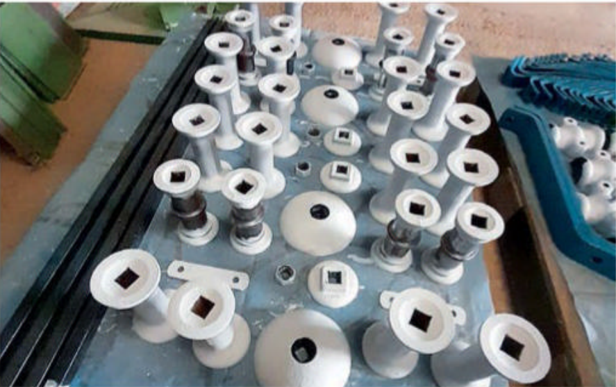
Everything was primed before the top coats of paint went on.
