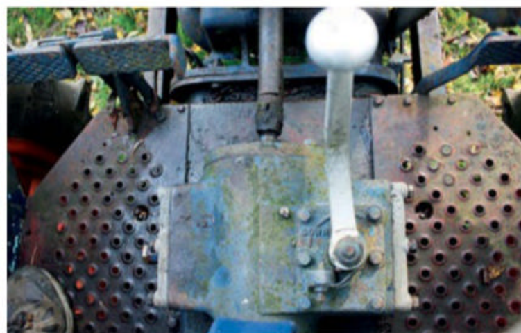
Once fully raised the lever moves back to the 'up' position until it is required to lower an implement.
