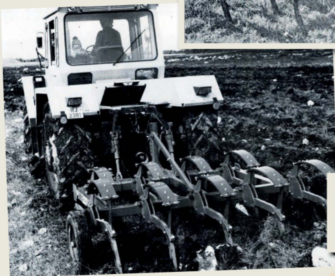
Kverneland's chisel plough was a heavy-duty implement with an automatic reset system to help counteract the panning caused by heavy machinery. It was ideally suited to sub-soiling, breaking new ground and cultivating stubble and could operate to a depth of 18in. Power requirements ranged from 75-165hp.
