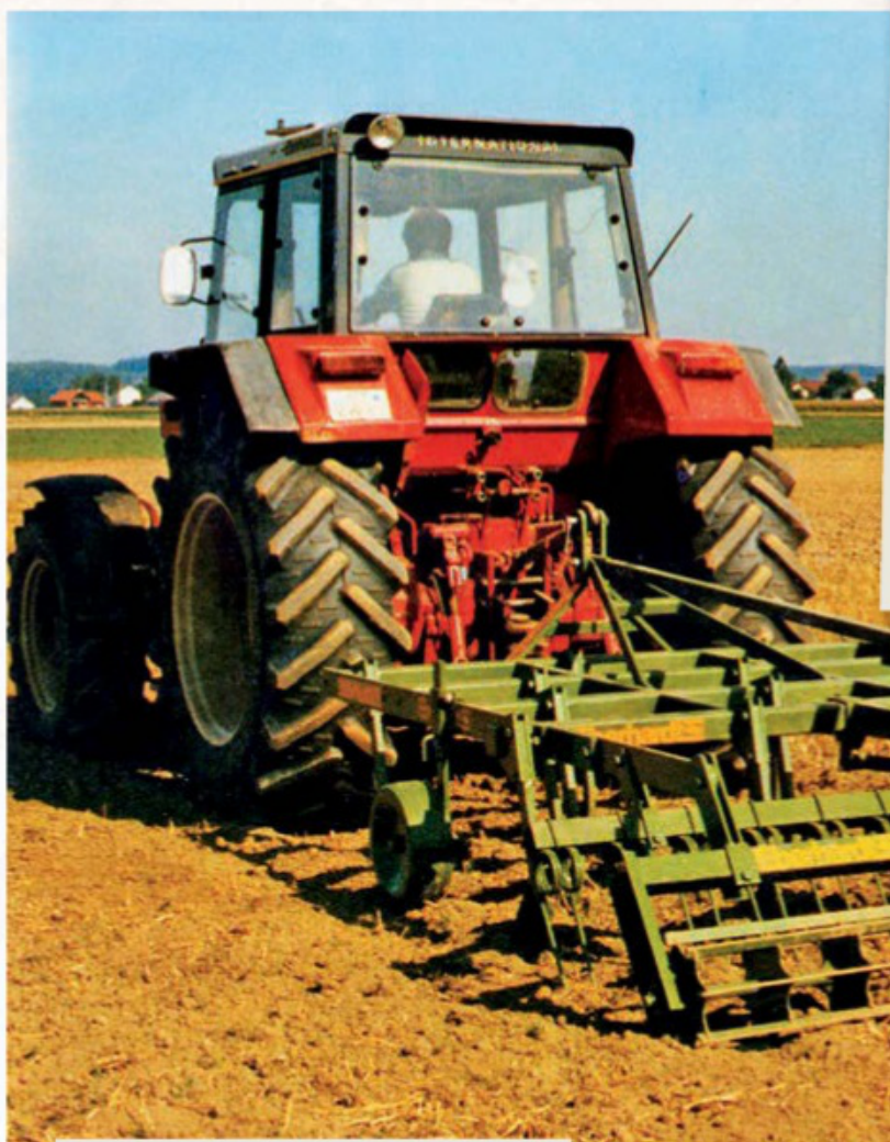
Above: Eberhardt Pflugfabrik GmbH, of the former West Germany, produced the Gazelle range of cultivators to suit tractors from 45-130hp. The example pictured features a weeder harrow and crumbler roller, but the variants could be specified with either, both, or a disc harrow follower.
