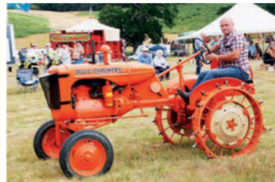
Allis-Chalmers B with starter motor and steels, as well as the front harvest screen.
