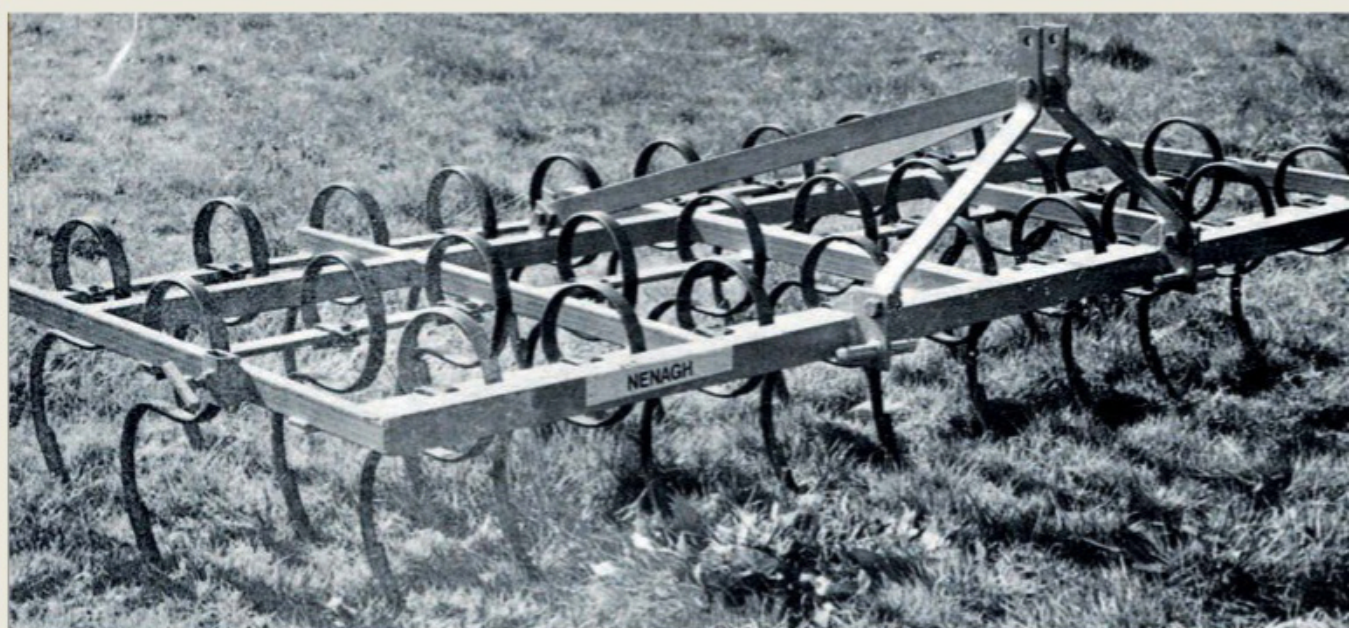
Manufactured in Nenagh, Co. Tipperary, by Abbey Machinery Ltd., the Vibrating Tine Harrow Model A (pictured above) came in working widths of 6ft to 10ft and with 16 to 30 tines, depending on the width. The Model C was similar, but the pitch of the tines could be adjusted via a winding handle.
