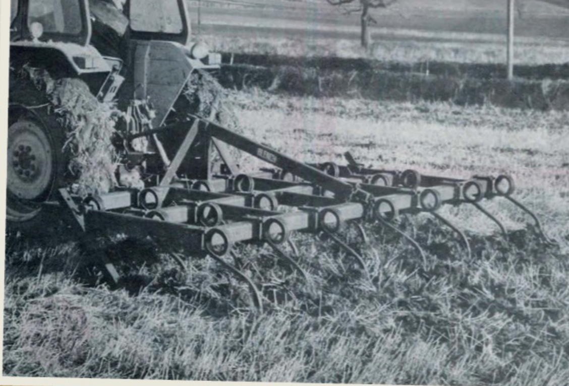
Above: Famed for his Dutch harrows, John Blench also produced other implements and attachments to suit farmers' needs. The company's range of chisel ploughs was suitable for category II tractors (8ft to 12ft working width) and category II/III tractors (14ft to 20ft working width). They could be fitted with double-coil pigtail tines (pictured) or double-leaf ripper tines.
