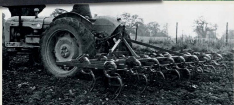
Above: Vicon's heavy-duty Vi-Till spring-tine cultivator was suitable for stubble clearance, spring, and autumn cultivations and was available in widths of 9ft 10in, 13ft 4in and 16ft 3in. Where large, folding extensions were featured, an 'A' frame and winch aided the operator.
