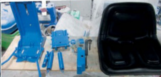
Above left: A service exchange clutch was purchased to improve matters in this area. Right: Replacement seat pans are no longer available, but a good alternative was sourced to fit the overhauled spring suspension assembly.
