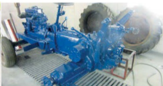
Above left: With the engine rebuilt and injection pump overhauled, the 4/98DT ran well at first start-up. Right: The skid unit receives its top coats.
