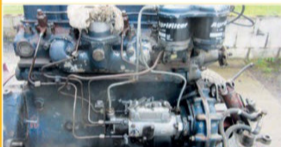
Above left: With the engine rebuilt and injection pump overhauled, the 4/98DT ran well at first start-up. Right: The skid unit receives its top coats.
