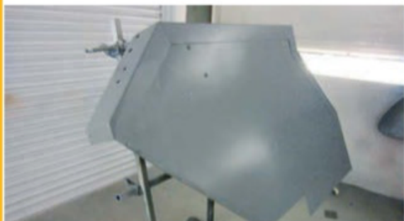
Above: Access to a spray booth enabled a good finish to be achieved, both with primer and top coat.
