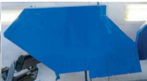
Above: Access to a spray booth enabled a good finish to be achieved, both with primer and top coat.
