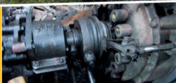
Above left: A service exchange clutch was purchased to improve matters in this area. Right: Replacement seat pans are no longer available, but a good alternative was sourced to fit the overhauled spring suspension assembly.
