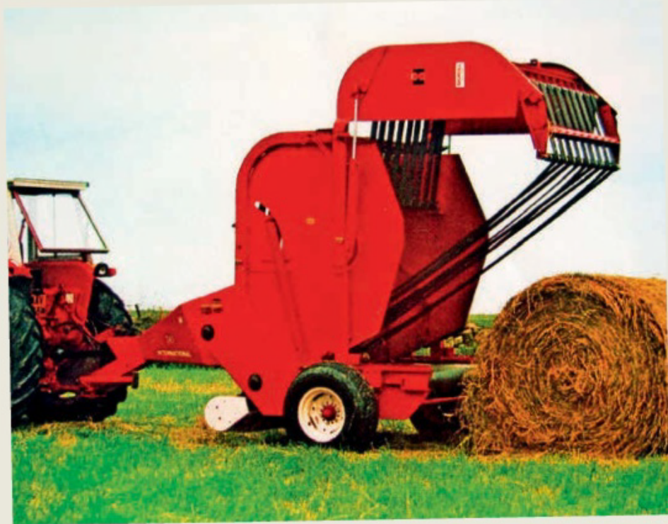
International Harvester's 241 Bigroll was a baler for the mid '70s that gave the company's loyal customers an alternative to the 430 and 440 conventional models that were popular at the time. Producing bales up to five feet (1.5m) wide and 6ft (1.8m) in diameter, weighing up to 1,500lb (680.4kg), the Bigroll needed just 45hp and a 540rpm PTO to run, meaning a 454 was more than capable of munching through the crop with the baler's 78in (1,982mm) pick-up.
