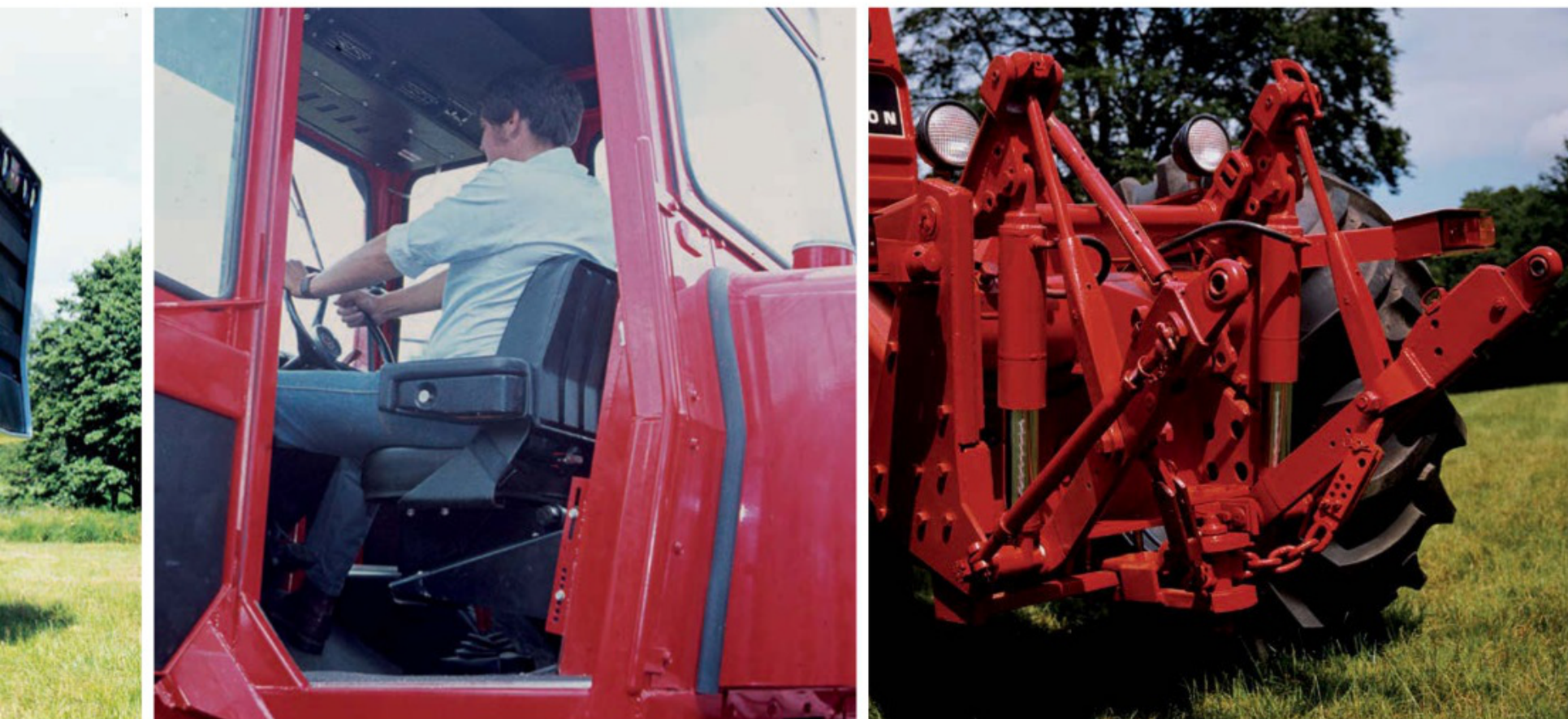
Above left: Access for daily checks and routine maintenance was permitted by these convenient steps. Above middle: The cab was spacious and comfortable. Note the rake of the floor under the pendant-type pedals. Above right: A simple lift and drop system was employed on the 1505, with none of the finesse that the Ferguson System offered on the MF 1200.
