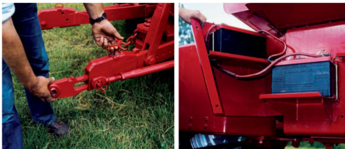
Left: Hitching was made simpler with telescoping lower links. Right: Like the 1200, two batteries were required for cranking the Caterpillar 3208 direct-injection diesel.
