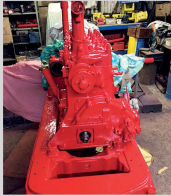
The engine in after being run and stripped down again, ready for paint to be applied.
