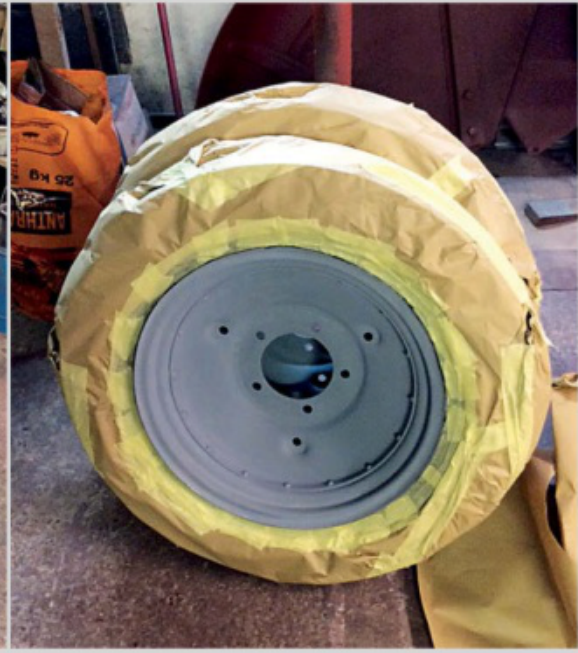
The front tyres are fitted, but not inflated, ready to be top coated.
