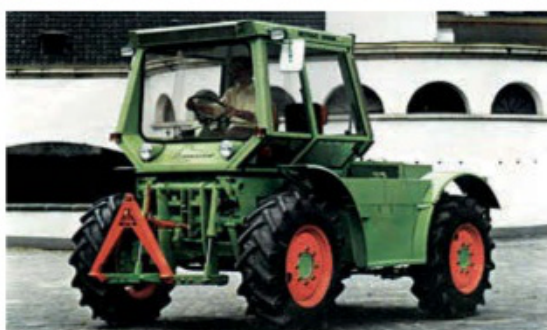
Intrac 2006 used a six-cylinder engine and hydrostatic transmission. It was not a commercial success.
