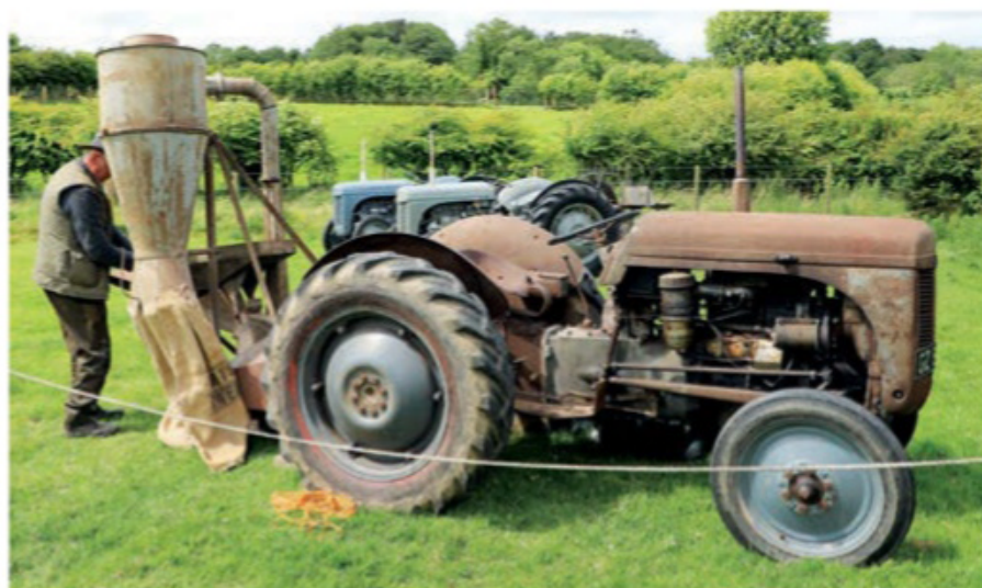
Right: Robert Bradley, from Bangor, operates an early 1950s' Ferguson cyclone mill driven by his Perkins P3-powered tractor.
