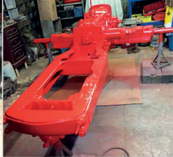
The basis of the tractor restored, waiting for the engine to be refitted.
