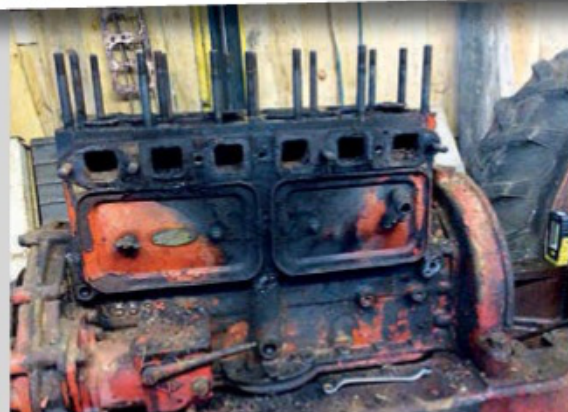
The block was in good order, considering that the tractor had overheated in the past.
