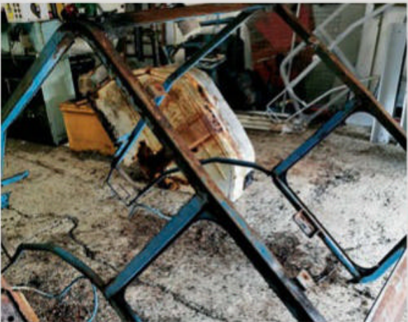
The cab frame was good, but needed sanding down and cleaning up. The mudguards were replaced by better examples.
