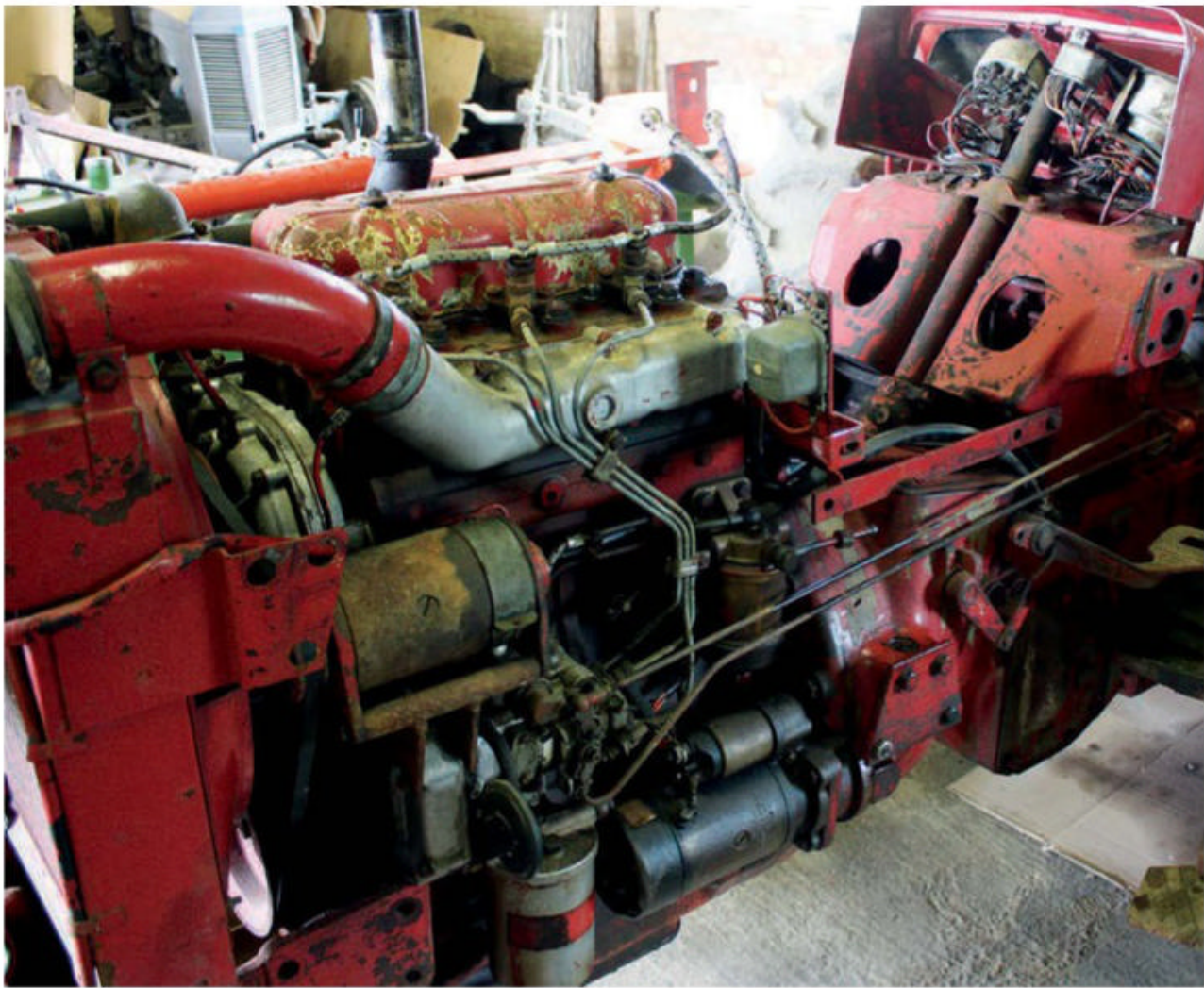
With the bonnet removed, the D-179 engine is clearly visible. Note also the cast support for the steering column and instrument panel – this speaks volumes about the 523’s build quality, and weight!
