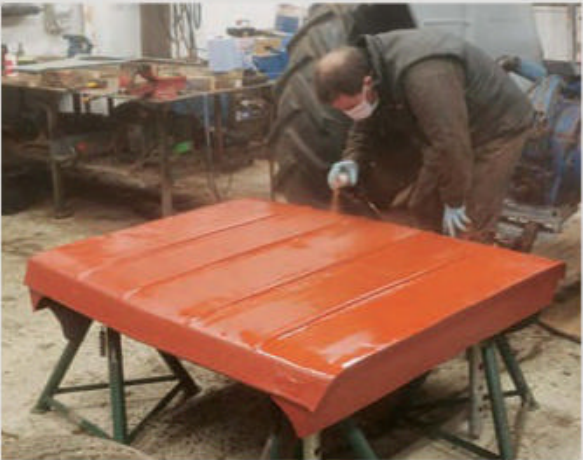
A genuine replacement cab roof was acquired and prepared for top coats of paint.
