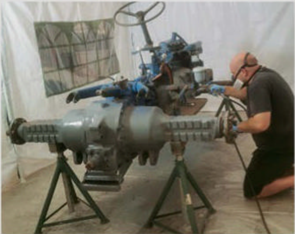
On goes the high-build primer.
