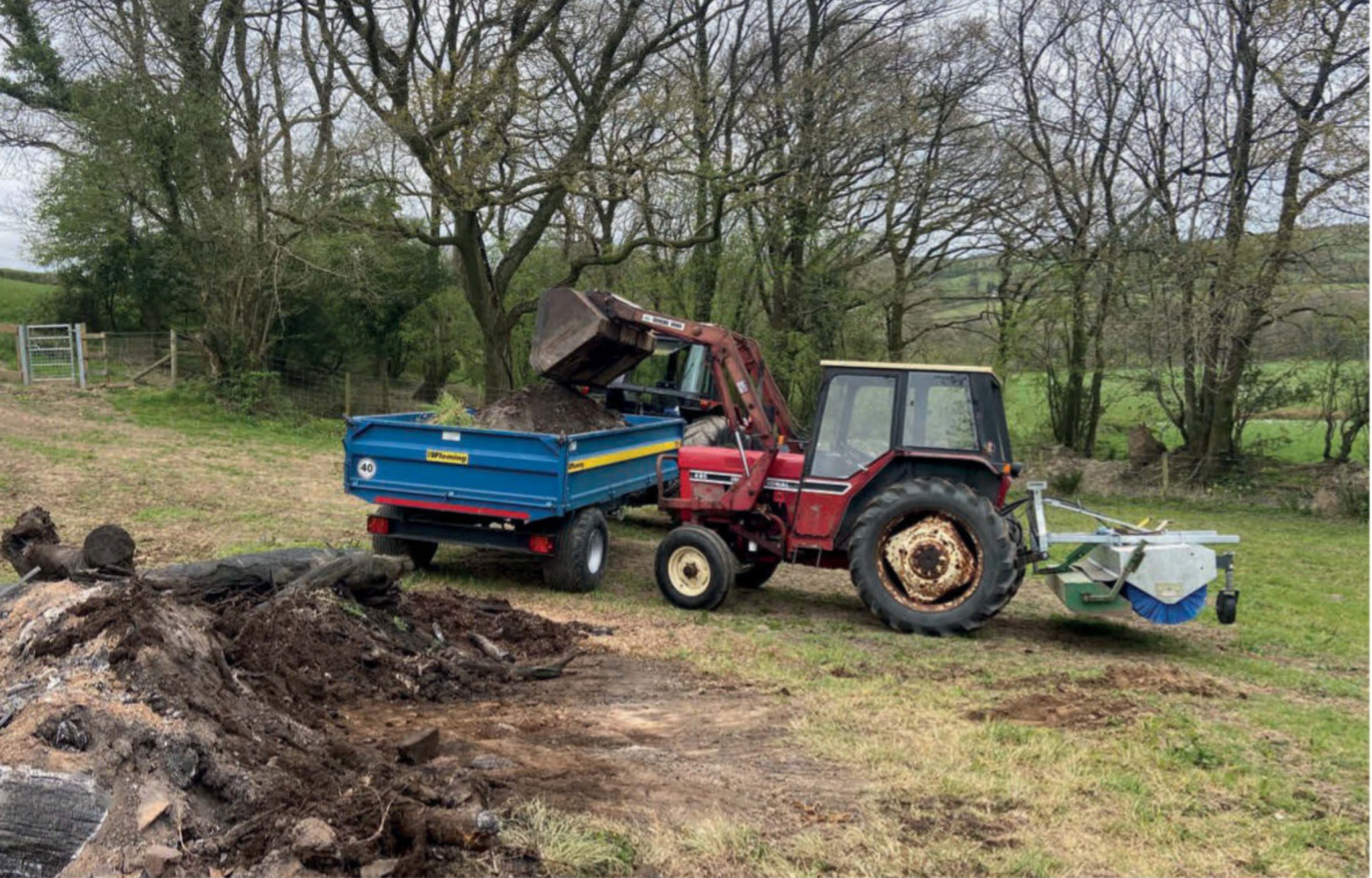
Roger Van Praet's 52hp (DIN) IH 485 was purchased at a local farm sale in September 2001. The original roof has been replaced with an 'LP' version, as the original had rusted through. The alternator was replaced last year, but other than routine servicing it's had no mechanical intervention in the last 20 years. It has completed a modest 3,200 hours. Photo: Roger Van Praet.
