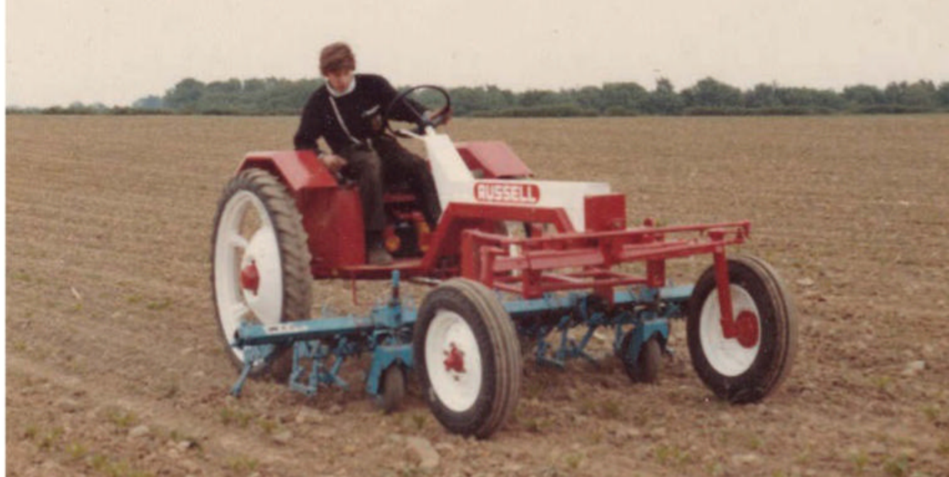
The Russell 3-D tool carrier used a two-cylinder diesel engine and hydrostatic wheel drive.
