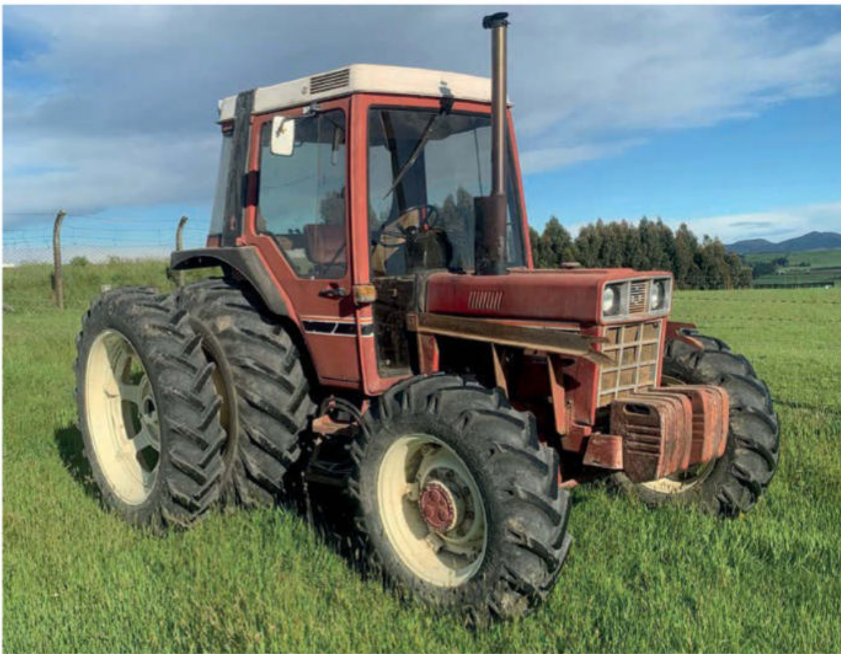
This 1984 IH 785XL is owned by the Pope family, from Southland, New Zealand. Its jobs include tedding, mowing and some loader work and it is fitted with dual rear wheels to make it more stable on the hills. Note the position of the headlights, typical of tractors for overseas markets, and the ZF side-drive front axle. Photo: Blair Pope.
