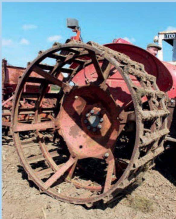
The Catchpole full-width cage wheels are fitted to the tractor in the same way as the normal wheels.
