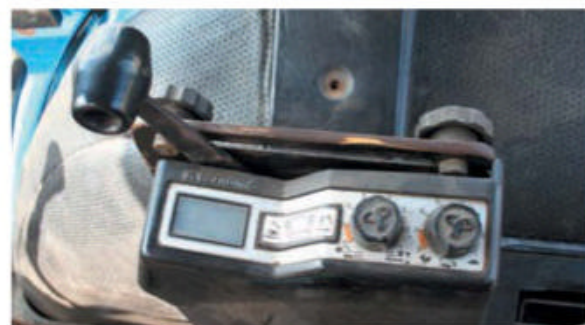
The 8210's Electronic Draft Control system replaced Load Monitor and worked well, being relatively simple to operate.
