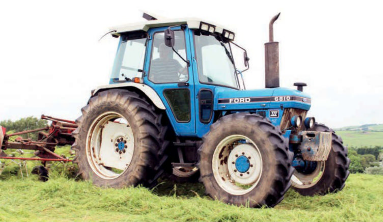
The 94hp 6810 was another new introduction as part of Generation III, designed to fill the gap between the 84hp 6410 and the 105hp 7610.
