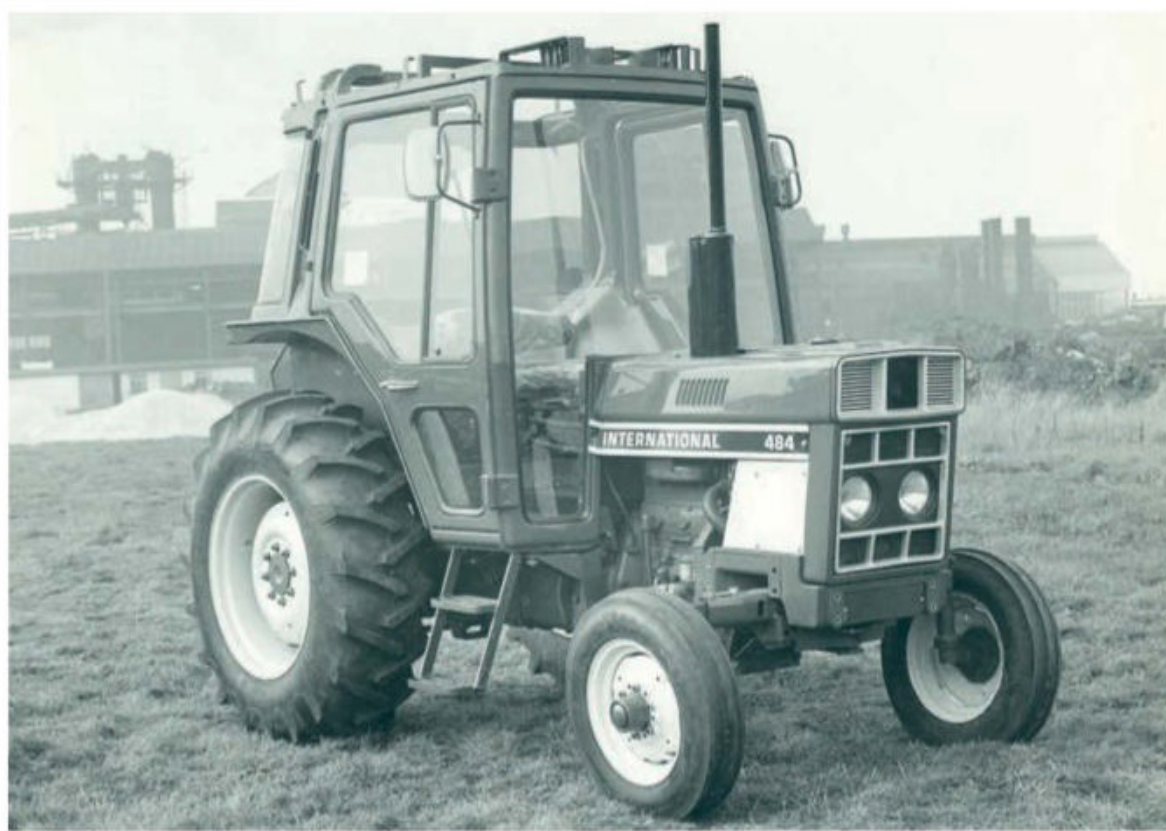
An IH 484 fitted with a pre-production XL Control Centre, photographed at Doncaster on 10 November 1978. Note the front-hinged doors and lower glazed portion. Photo: Christiaan Holwerda collection.
