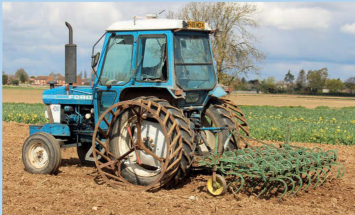
Newer tractors also used cage wheels, as demonstrated by Robbie using his Ford 6610 and Bettinson cage wheels while cultivating with a Marsk Stig implement.
