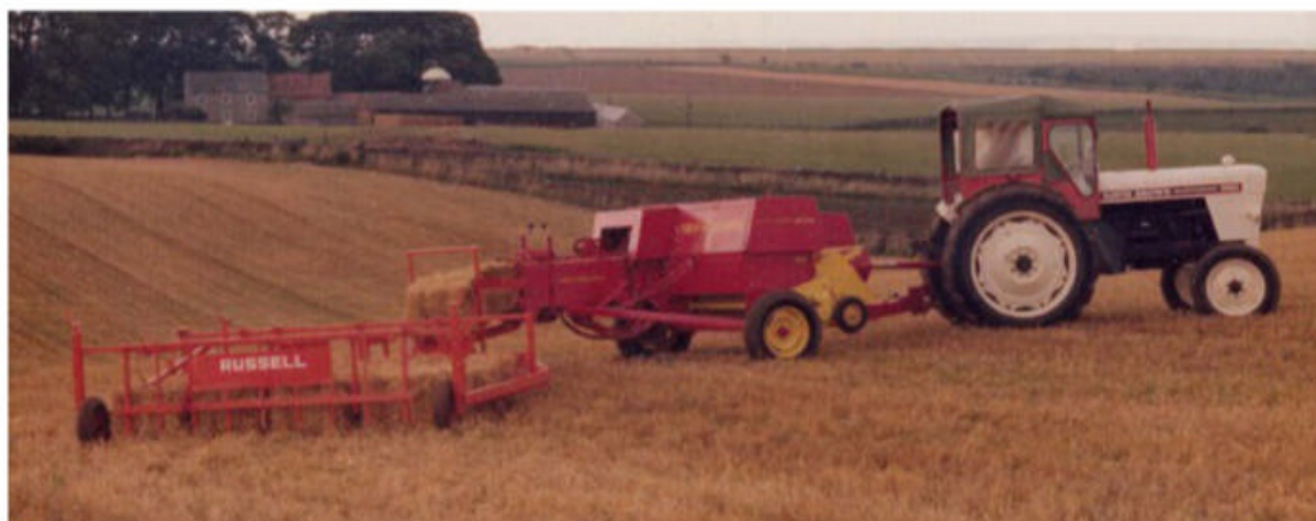
Russells developed a range of 'flat eight' bale-handling equipment, including this sledge.
