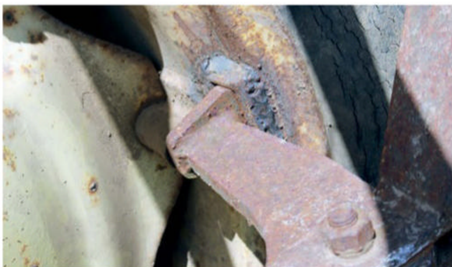
Bettinson provided the small lugs that needed to be welded to the tractor's wheel rims. The prongs on the cage wheels themselves then secured into these lugs, making a snug fit once tightened.
