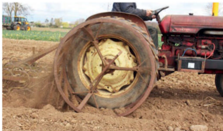
A close-up action shot of the Bettinson cage wheels on the David Brown 990, showing how they manage to accomplish a level of cultivation.
