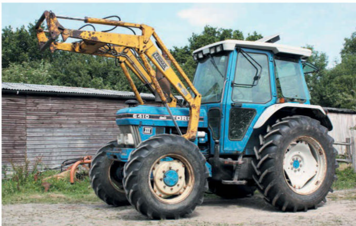
The 6410 was a new tractor introduced in 1989 with the Generation III line and replaced the 6610 in many markets, including the UK. It was powered by an 84hp four-cylinder engine.
