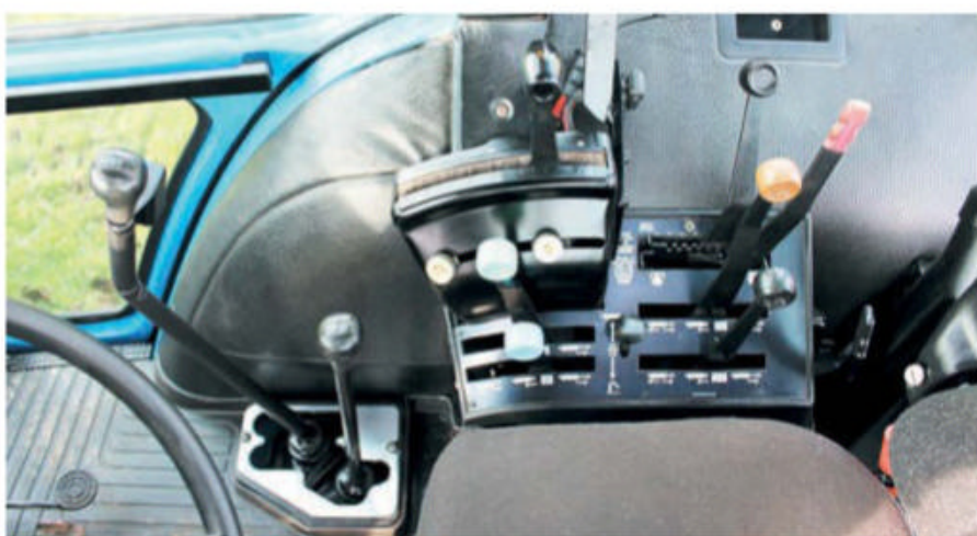
Inside the cab of a 7810 we find the neat layout of all the main controls with spool valves, rear linkage and power take-off controlled by the main console to the right-hand side of the driver's seat. The two floor-mounted gear levers control the 16-speed synchromesh Dual Power transmission.
