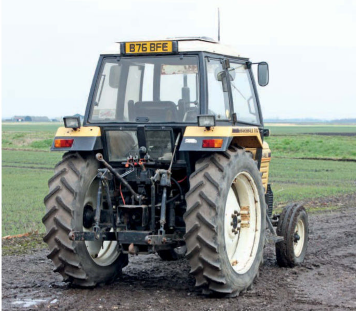
This tractor has the standard-spec rear end, with one double-acting and one-single-acting spool, 540/1,000 rpm PTO via interchangeable stub shafts, pick-up hitch and lower links with ball ends, rather than the hook type. Note the Nuffield/Leyland parentage. Photo: Scott Lambert.
