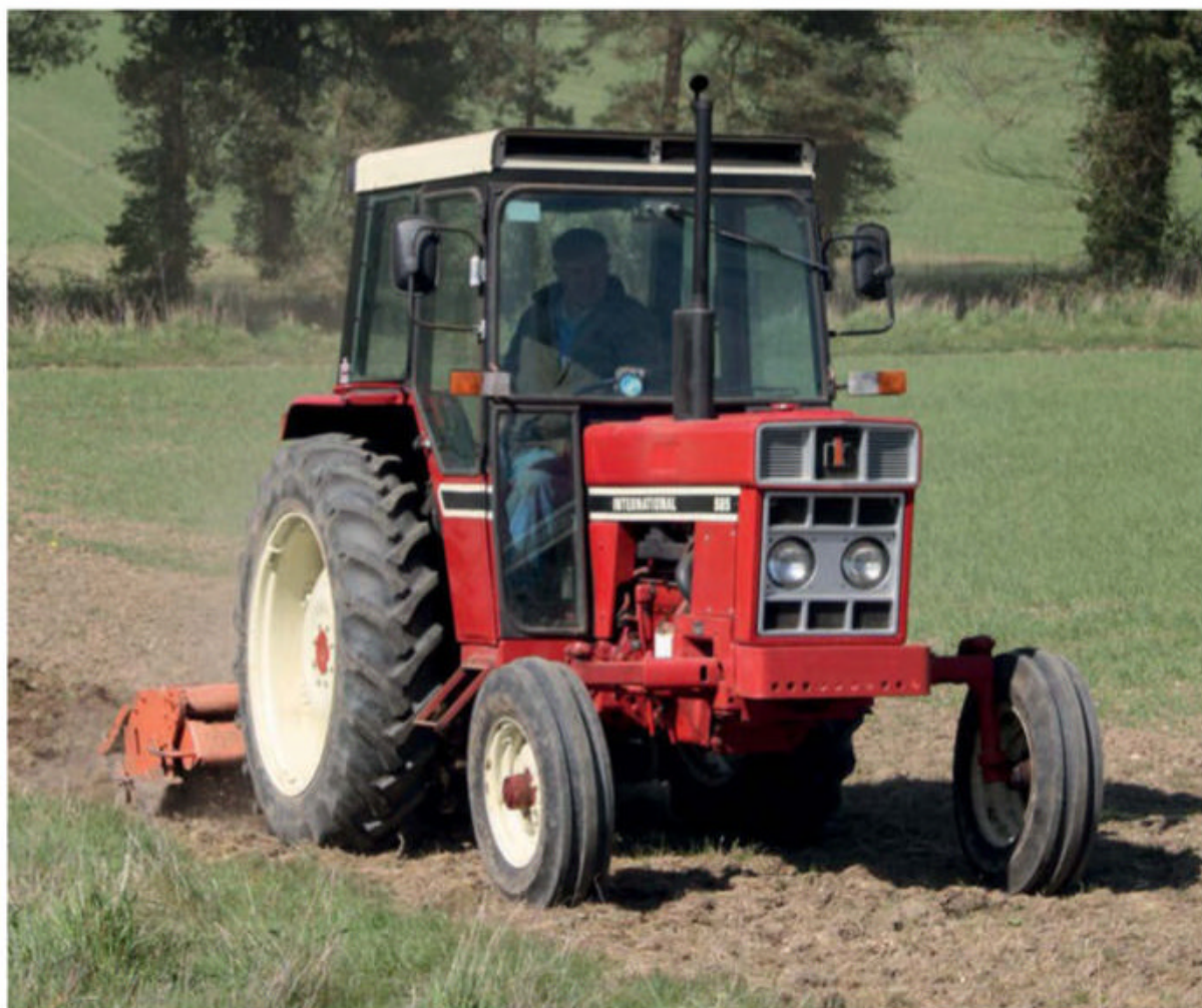
An IH 585L with a Howard Rotavator. The 58.9hp (DIN) model used the short-stroke D-206 engine and was the smallest tractor in the range to be offered with the XL Control Centre. Photo: Jonathan Whitlam.
