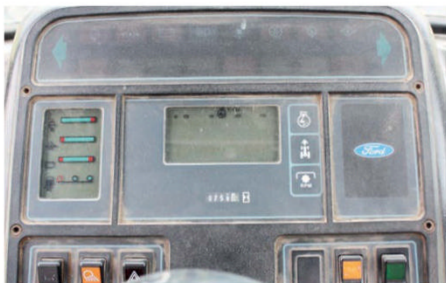
The digital dashboard, with built-in performance monitor, became a common feature on Generation III tractors after its introduction on Series TW Force II machines.
