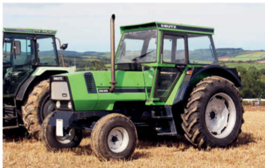
The DX85 is powered by an 85hp, five-cylinder, air-cooled Deutz engine and this one was supplied new to a farm in Coldridge, Devon.
