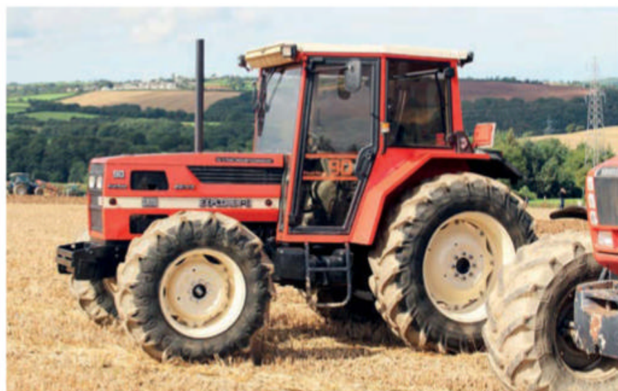
Colin Martin's fresh-looking SAME 90 Explorer II. The Explorer models proved very successful for the company and this version was powered by a 90hp, turbocharged four-cylinder engine.
