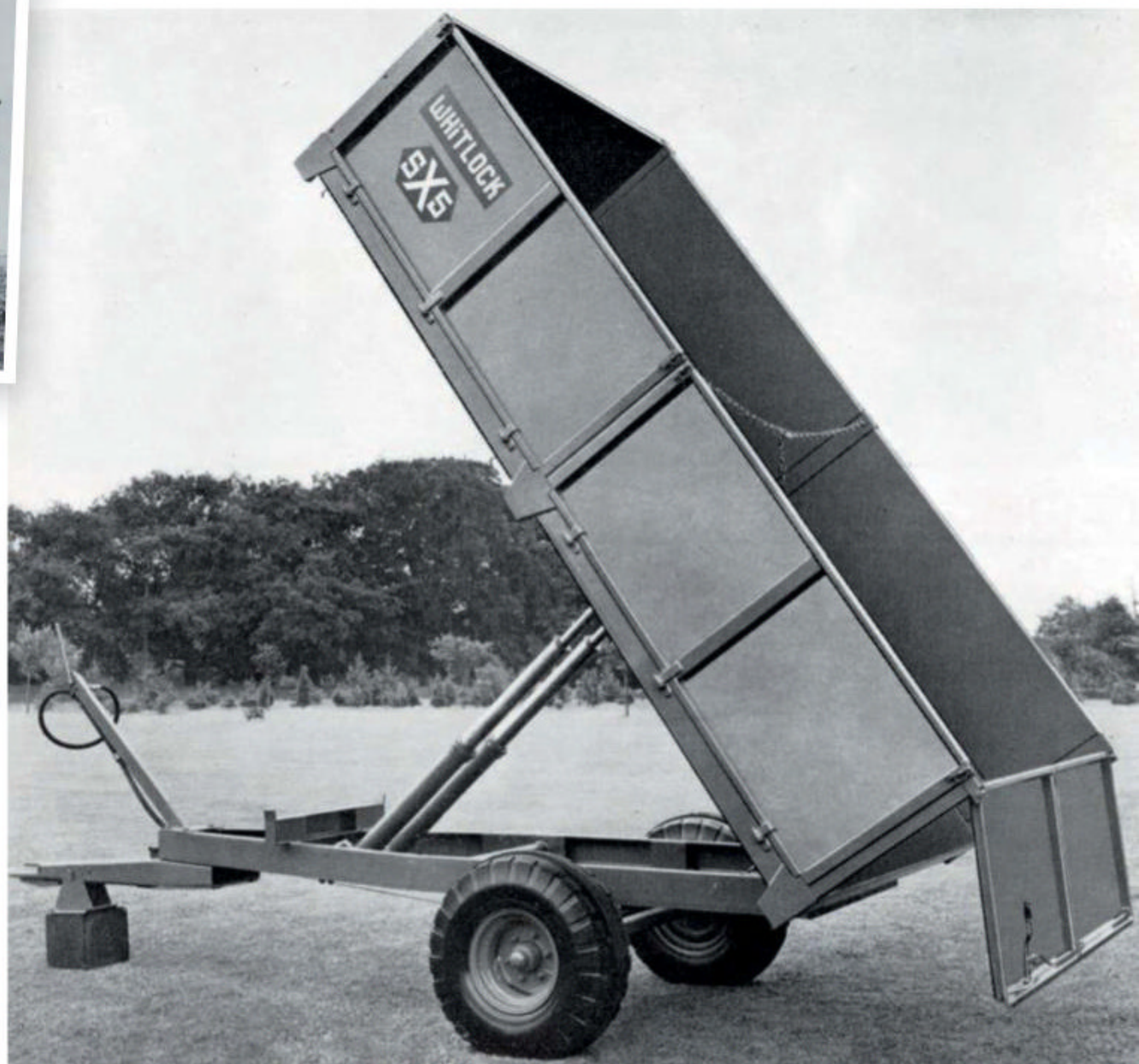
Whitlock Bros. Ltd., of Great Yeldham in Essex, was perhaps best known for its excavators, but the company also produced other agricultural equipment – such as the SX5 and SX6 trailers. With a 5-ton load capacity, the SX5 had a 7x13ft body, with sides 2ft 6in high. Tyres were 12.5x15 8-ply, with the wheel hubs mounted to a 2 3 / 4 in solid steel axle.
