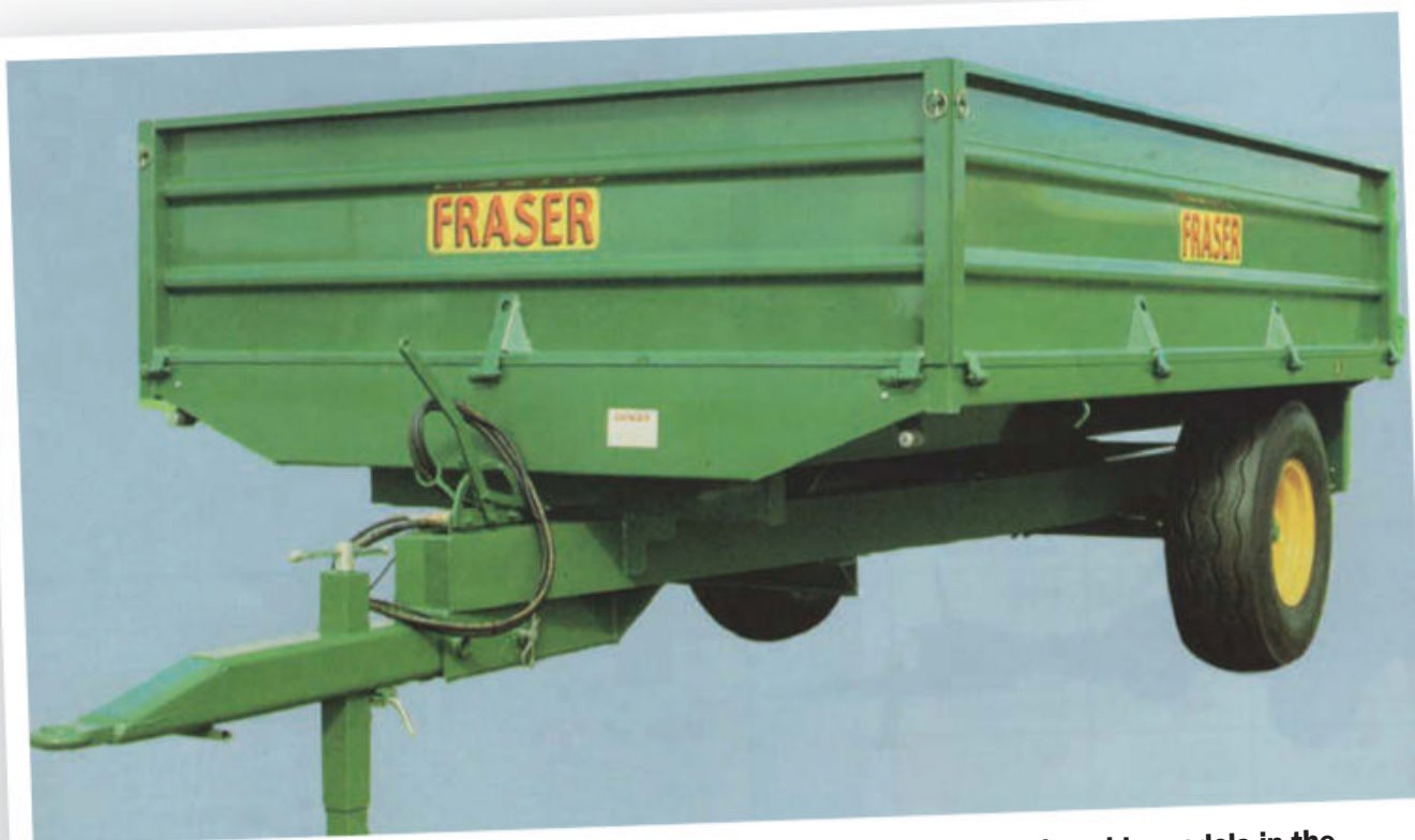
Aberdeenshire-based Fraser Agricultural (Rothienorman) Ltd.'s single-axle dropside models in the style shown spanned four to seven-and-a-half tonnes and could be specified with floor and sides made from hardwood or steel. The F68 shown was a 4.5-tonne model with an unladen weight of 860kg.
