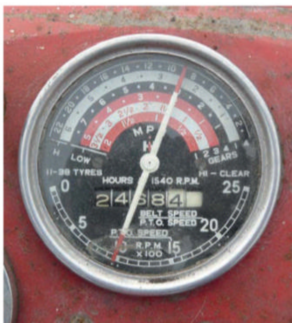
A genuine Hi-Clear tractor is distinguished by its tractorometer. Photo: Scott Lambert.
