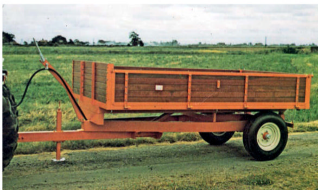
T&F Equipment Ltd. had a slogan that claimed 'trailers of distinction' and it's fair to say that its 21135 and 21140 models certainly cut a dash. With striking orange steel frames and Malayan hardwood secured with galvanised nuts and bolts, these 3.5-ton and 4-ton trailers looked the business. The company was based in Sutterton, Lincolnshire.
