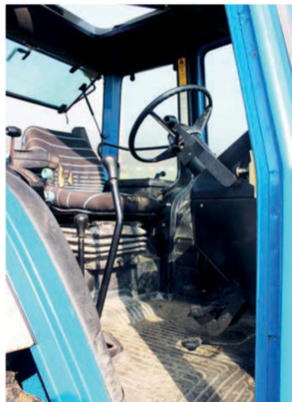
A view into the Super-Q cab of a 7710, showing the new seat and two floor-mounted gear levers.
