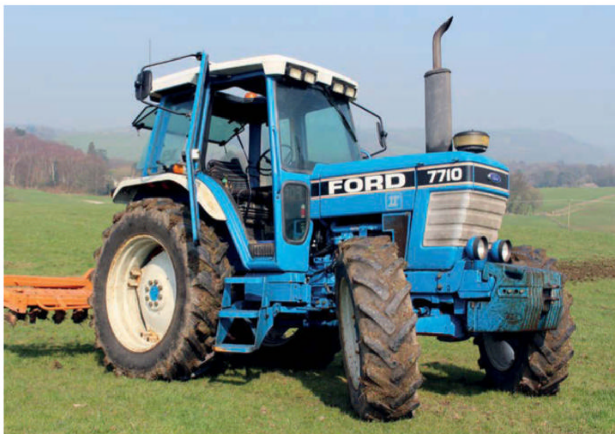
The Ford 7710 Force II remained the same as the earlier version, except for the fitting of the Super-Q cab.
