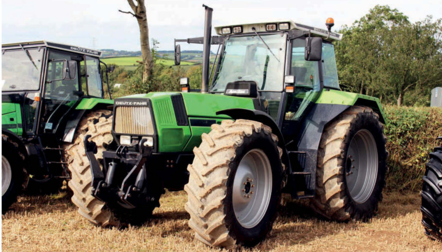
Say hello to the AgroStar 6.81! It's an 185hp monster, powered by a Deutz seven-litre, six-cylinder engine and fitted with either an 18- or 27-speed transmission.
