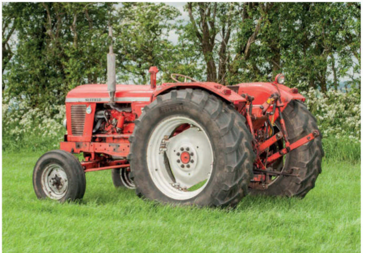
The business end of the 4/65 differed from its predecessor, thanks to a change of hydraulic pump from Dowty to Plessey and an increase in lift capacity to 3,350lb.
