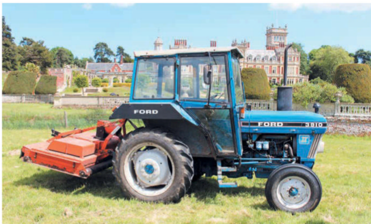
The 3910 was the smallest Series 10 tractor offered in the UK after the launch of the Force II range. This three-cylinder 50hp tractor was only produced with the Sekura LP cab.
