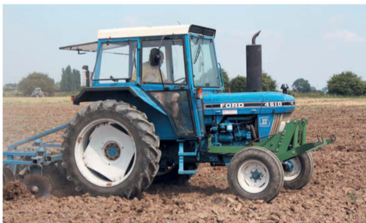
The 64hp 4610 continued to be a popular machine after Force II was introduced. This three-cylinder, 64hp tractor was never available with the Super-Q cab and was fitted as standard with the Sekura-built AP cab.
