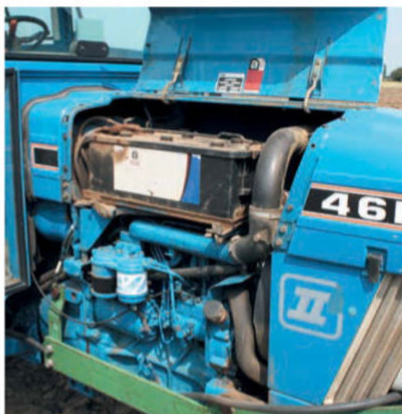
The bonnet retained the excellent access points as had been established on the original Series 10 models of 1981. Note the Roman numeral 'II' on the lower panel which, along with the new style decals, denoted the new range.
