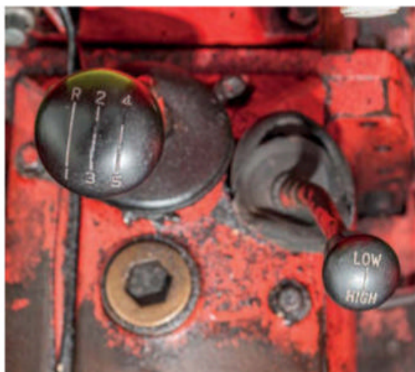
10 forward gears and two reverse were available to the operator.
