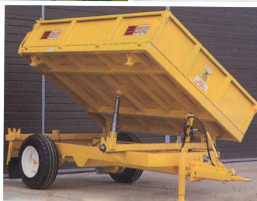
A S Trailers, based at Marston – near Grantham, Lincolnshire, produced a wide range of trailers in the company's traditional blue livery. This 3.5-tonne, three-way tipper was from its 'Local Authority Range' and featured a sprung axle and overrun brakes.
