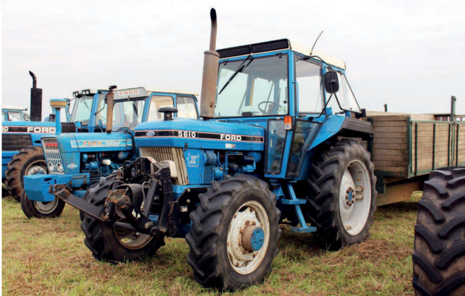
The 5610 was originally only offered with AP or LP cabs. The smallest of the four-cylinder models to be offered in the UK, the 5610 was a 75hp machine and not many would have been fitted with a front linkage like this one.
