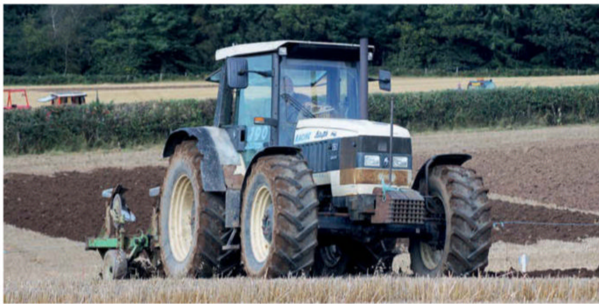
Jim Hedges powering up the hill with his Lamborghini Racing 190 and Dowdeswell reversible. This tractor was the largest produced at the time and was powered by a turbocharged six-cylinder, six-litre engine of 189hp. The transmission was a full powershift, 27-speed unit that was also sold for use in large Renault tractors for a time.
