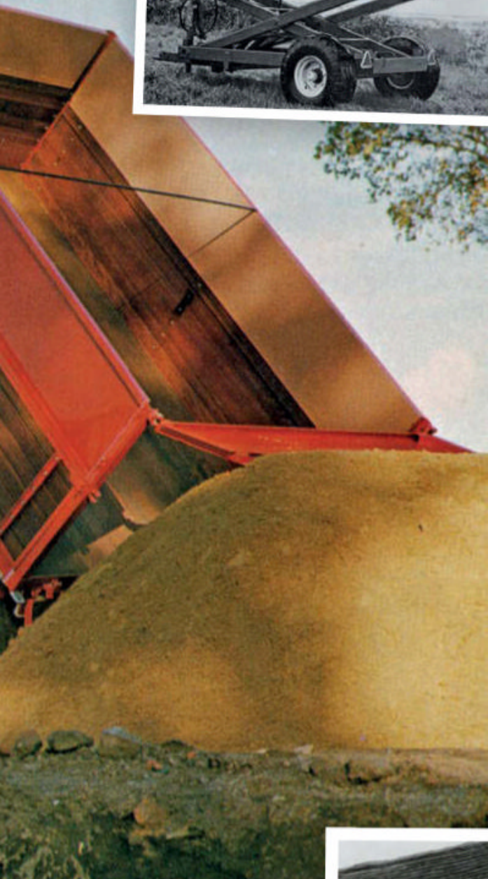
Whitlock Bros. Ltd., of Great Yeldham in Essex, was perhaps best known for its excavators, but the company also produced other agricultural equipment – such as the SX5 and SX6 trailers. With a 5-ton load capacity, the SX5 had a 7x13ft body, with sides 2ft 6in high. Tyres were 12.5x15 8-ply, with the wheel hubs mounted to a 2 3 / 4 in solid steel axle.
