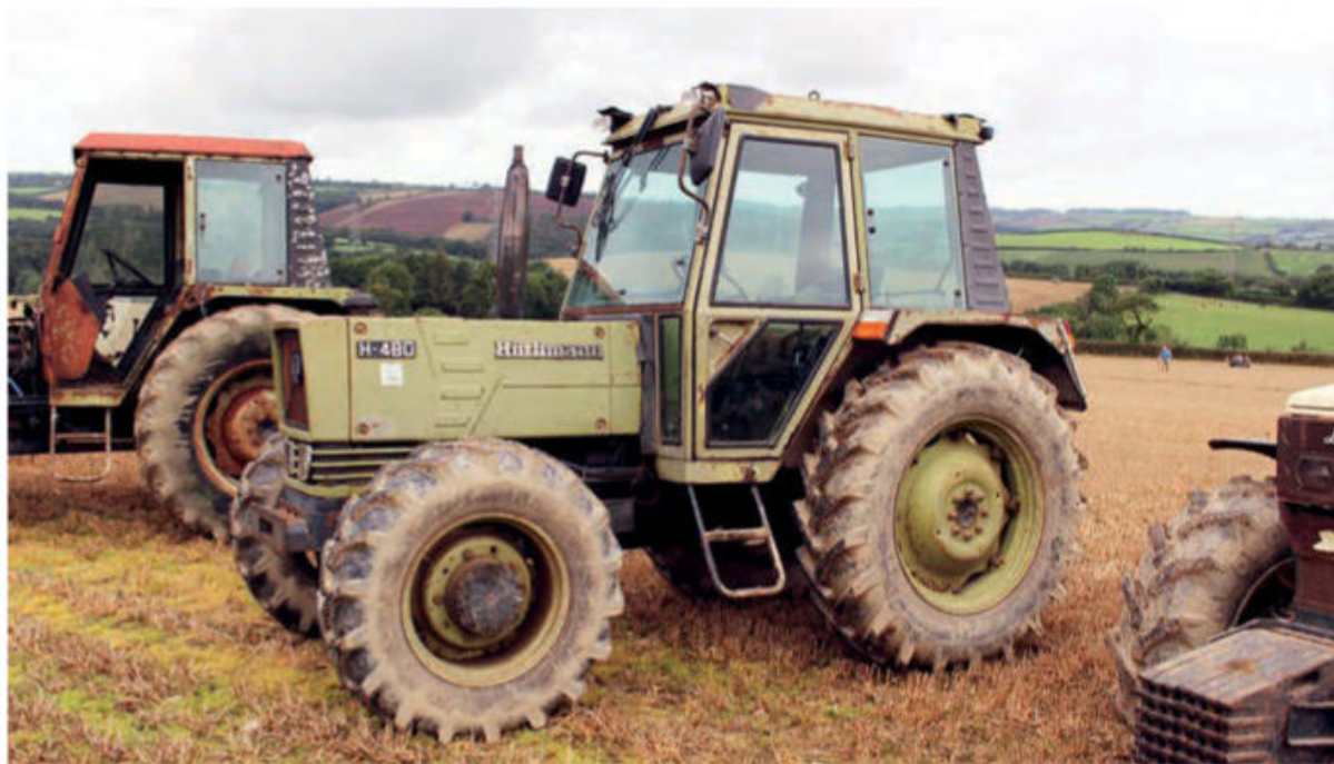
A slightly larger Hürlimann; this H-480 is fitted with the same cab as contemporary SAME and Lamborghini tractors and is powered by an 82hp SAME 4.6-litre, four-cylinder engine.
