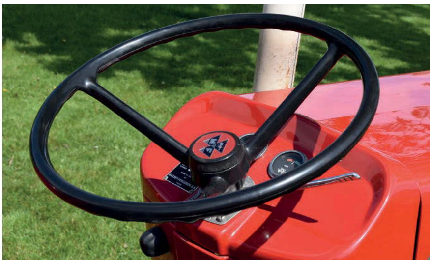
RIGHT: As an 'Economy' variant, Norman's MF 130 simply has an oil pressure gauge and ammeter.
