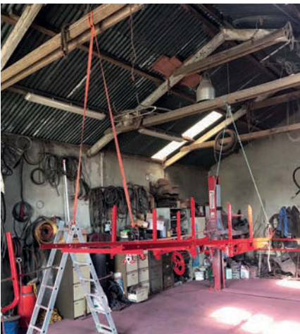
Suspending the frame and individual components ensured full coverage when spraying paint.
