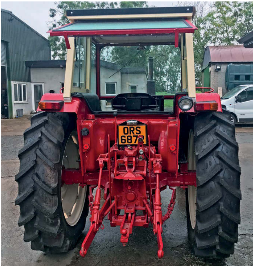
The 'saddle' fuel tank added additional ballast over the rear axle.
