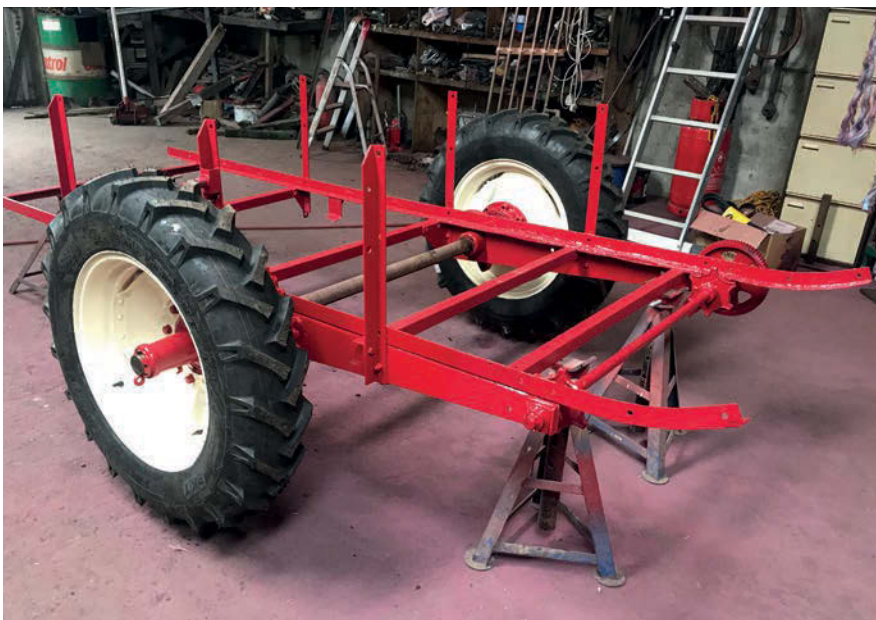
The frame, complete with axle and wheels shod with BKT 7.50-20 tyres.
