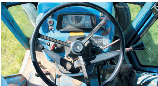
Inside the 'Q' cab of the 4610, the column-mounted gear levers can be clearly seen. The lever on the left changed the range, while the right-hand lever selected the ratios within each range.
