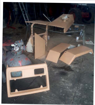
The new and original panels were painted with buff primer prior to receiving top coats of Orchid White.
