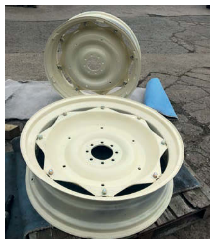
A good finish was achieved with the spray gun. Note the Bettinson cage/dual wheel lugs.
