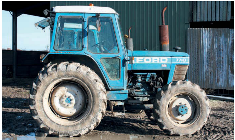
A side view of the 7710 shows the higher bonnet line, with only the new Series 10 decals changing the appearance of the bonnet from the earlier 7700 model. Four-wheel drive was now a factory-fitted option on the 7710.
