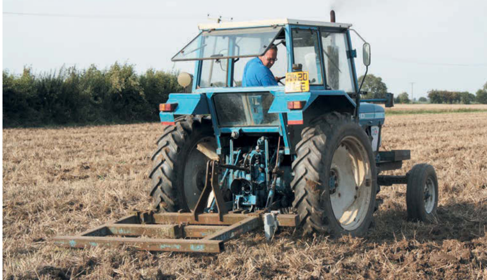
A 76hp 5610 cultivating stubble, fitted with the original LP cab sourced from Sekura.
