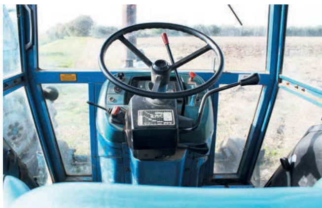
Inside the LP cab visibility is excellent, with plenty of glass area. The only blight on the landscape, according to many drivers, was the awkward gear shift provided under the steering column.
