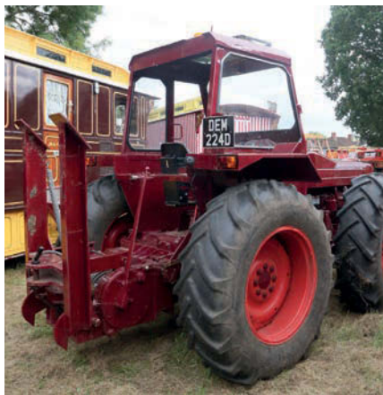
At the rear there's a substantial winch to enable rides and living vans to be moved, should Kevin's traction not be sufficient.
