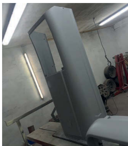
Other than the mudguards, the remainder of the panels were in good order and needed very little attention before primer went on.
