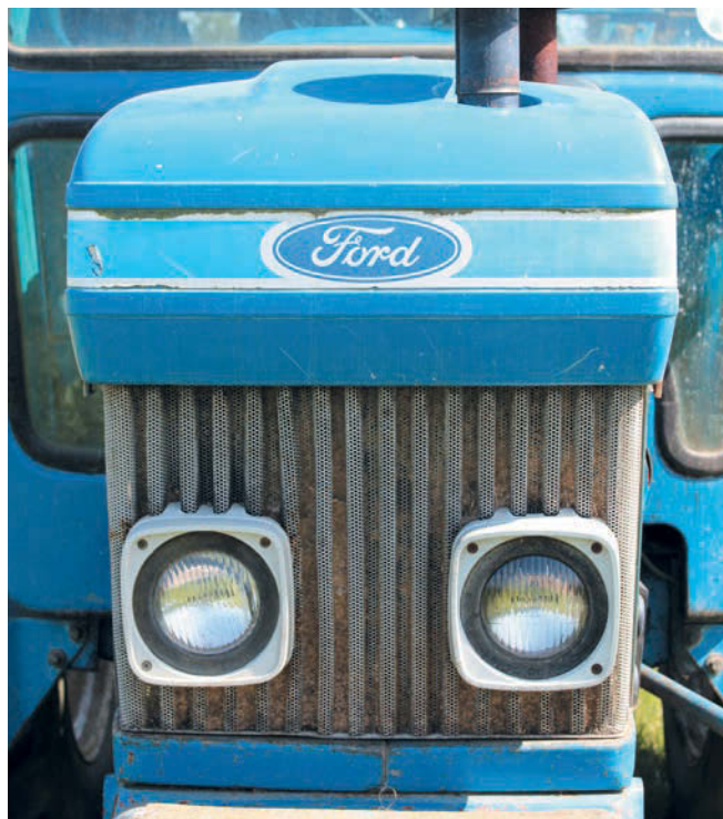
The front bonnet treatment was the main new external feature of Series 10, with headlights fitted into the front grille and a nose cone at the top that could be hinged out of the way to gain access to the air cleaner.
