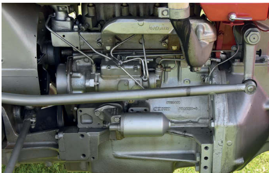
The 30hp, four-cylinder A4.107 engine was built by Perkins to MF specifications.
