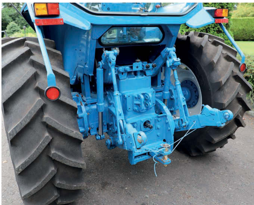
The tractor is fitted with two assistor rams and two double-acting spools.
