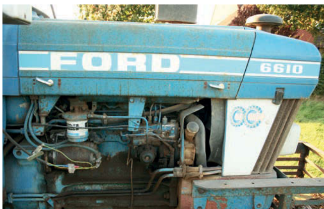
A side view of an original 6610, showing the four-cylinder engine, bonnet decals, including the Synchroshift logo, and the hinged bonnet and front nose cone.
