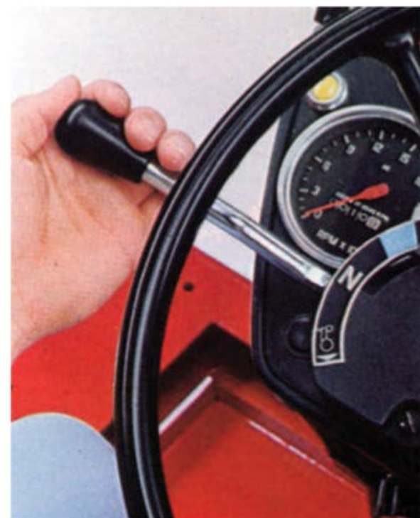
The Speed Ratio Control Lever on a 74 Series tractor. The light blue area on the quadrant indicates the range for best performance. Image from IH literature.
