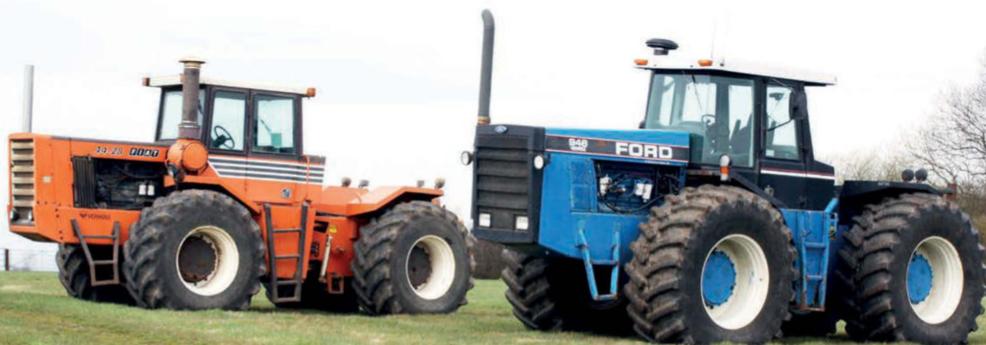
The Ford Versatile was based on a new range of Versatile machines known as Designation 6 and comparing these two models, that are around 10 years apart, shows that the cab is probably the main difference. Note the position of the exhaust at the front of the bonnet – a Versatile trait.
