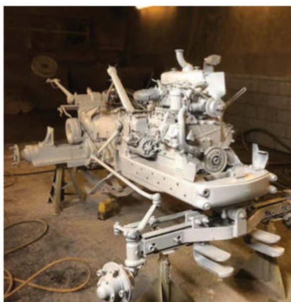
While awaiting replacement parts, Paul sent the Nuffield 4DM for shot blasting and priming.
