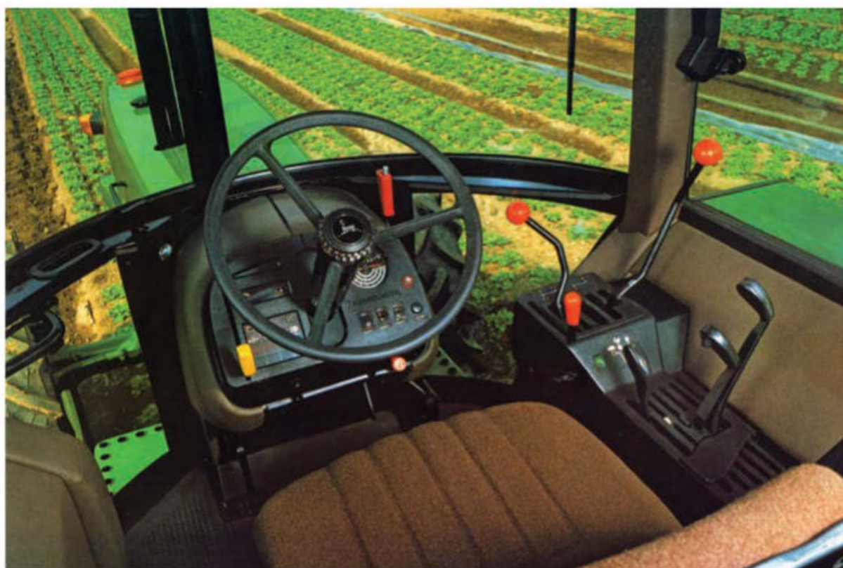
The interior of the SG2. The right-hand console meant that all of the major controls fell easily to hand.
