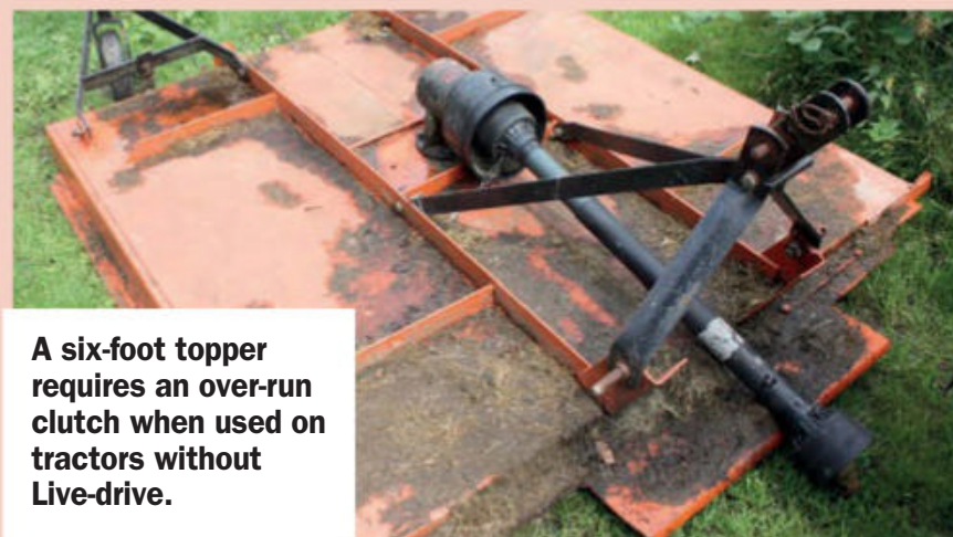
A cheap option is an aftermarket over-run clutch, such as this type.
