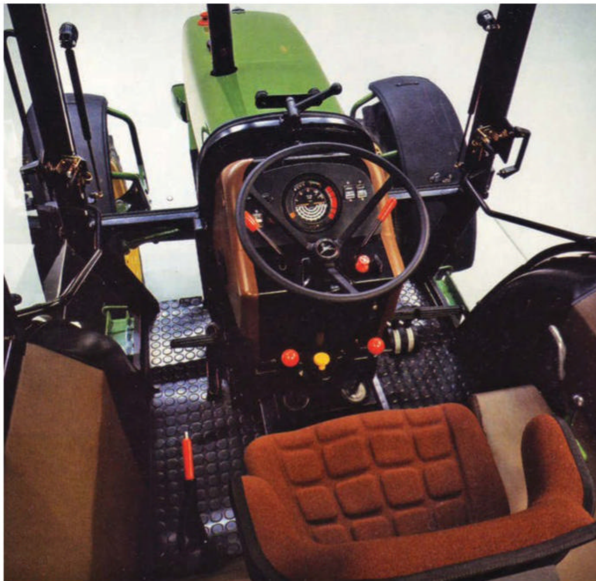
The interior of the John Deere MC1 cab. Note the floor-mounted gear levers and lack of pendant-style pedals.
