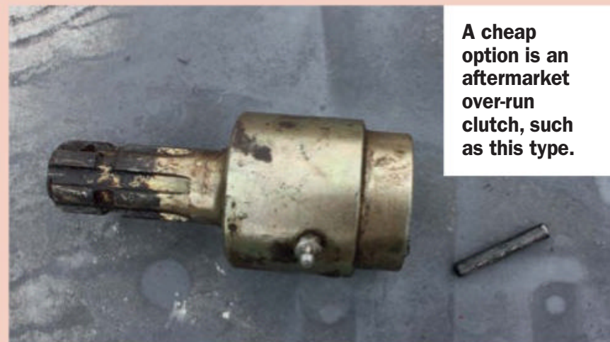
A six-foot topper requires an over-run clutch when used on tractors without Live-drive.
