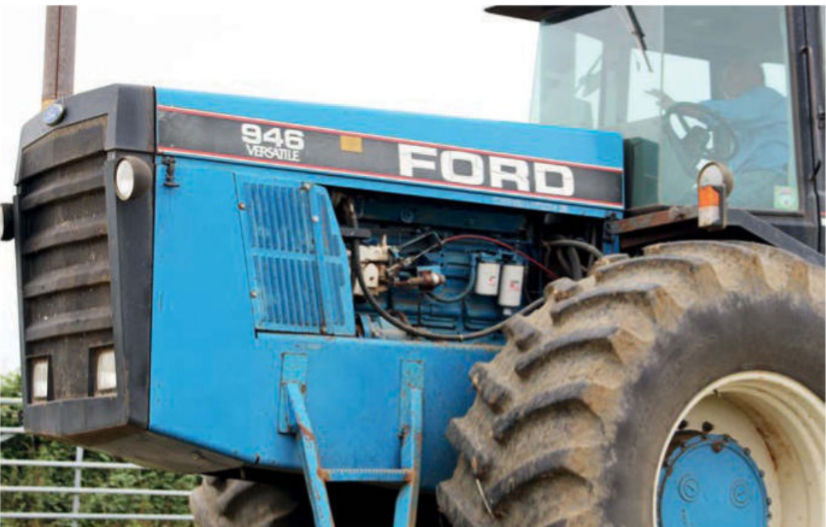
Cummins provides the grunt for this Versatile product – a six-cylinder engine featuring a turbocharger and aftercooler.
