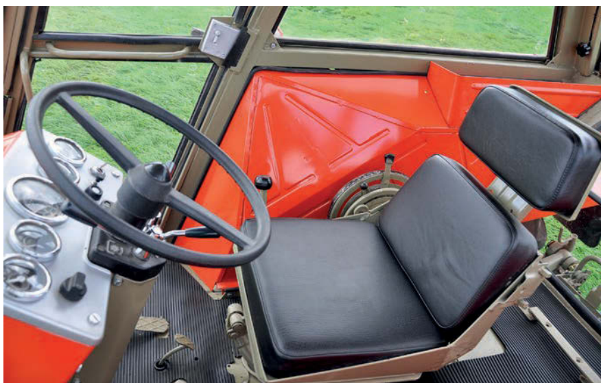
The cab was a trendsetter, but let down by the fact that the seating position made pick-up hitch visibility difficult. Photo: T&M archive.
