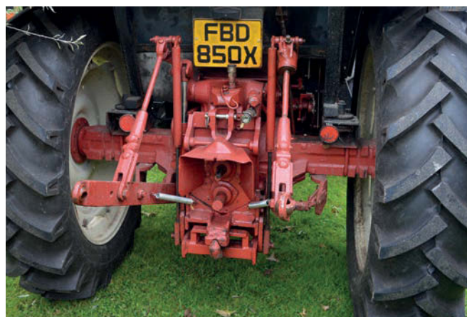
Standard lift capacity was 2,000kg across the bulk of the range, but 2,380kg with the optional assistor (seen here).
