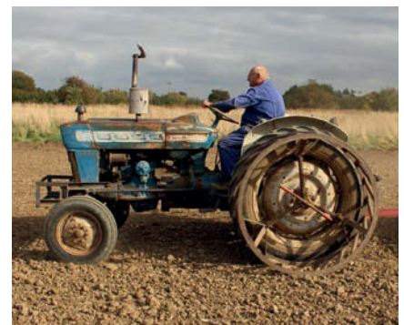
Also rated at 55hp, the Ford 4000 used a 'square' engine design.
