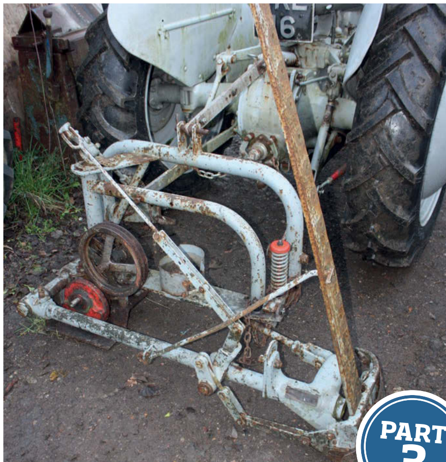
Work on the cutter bar is about to begin with the removal of the paint applied years ago by a previous owner.
