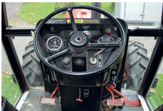
The dash panel was simple and well laid out, but some of the warning lights were difficult to see in bright light.
