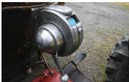
Ford's optional Select-O-Speed system was convenient, but not particularly smooth. Photo: Peter Henshaw.
