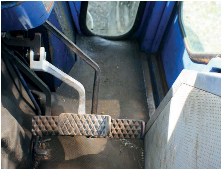
The tractors in the range are fitted with a three-pedal braking system. Photo: Howard Sherren.
