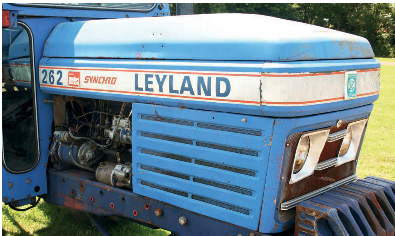
The side grille panels are retained by springs and allow access to the battery and radiator. Photo: Jonathan Whitlam.
