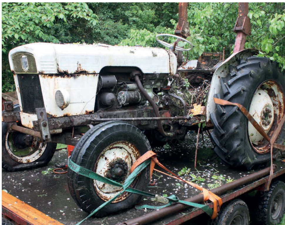
The extent of the rust in the bonnet can clearly be seen in this photograph. It has been the most challenging task on the project so far!
