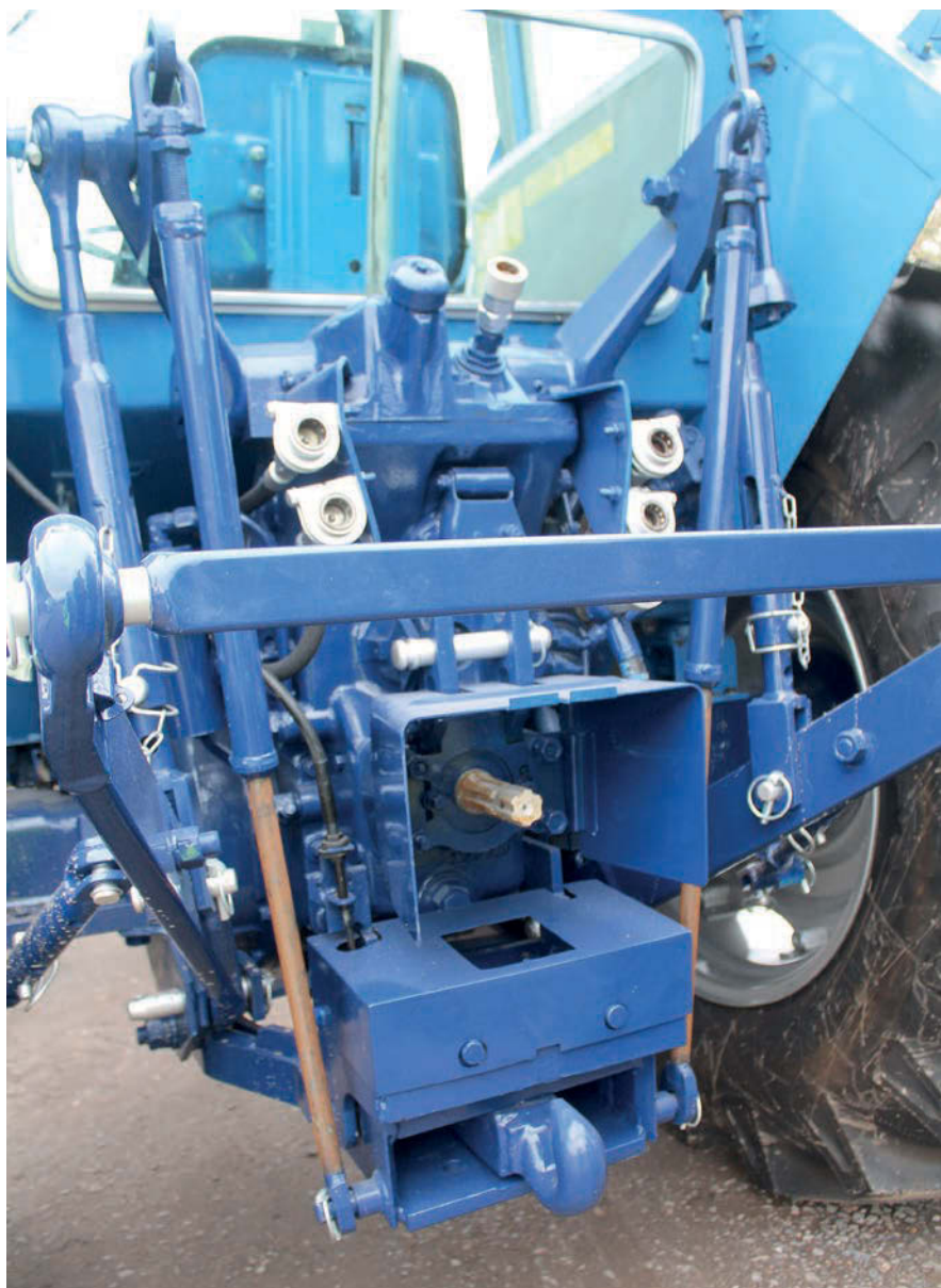
The three-point linkage, PTO and pick-up hitch arrangement. Photo: Joseph Lewis.
