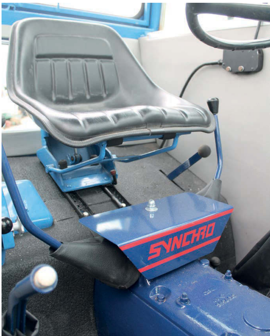
This shot shows the two gear levers to advantage. Gears on the driver's right and ranges on the left. Photo: Joseph Lewis.
