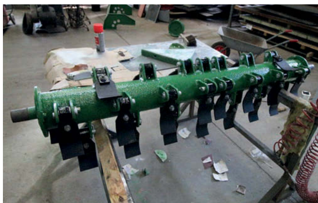
The completed rotor with new pins, bushes and flails.
