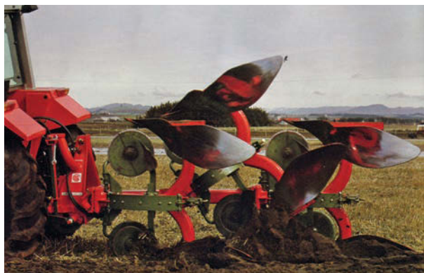
The Kverneland Automatic Reset System was available for mounted and semi-mounted conventional ploughs, as well as reversible models.
