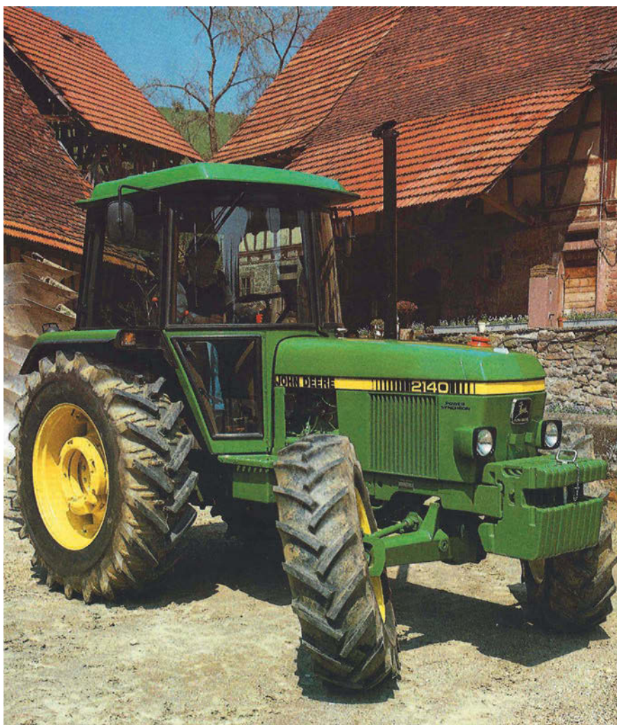
The four-wheel drive model was famed for its 'Caster angle' steering.
