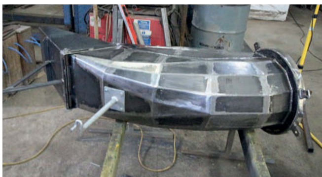
This photograph provides an insight into the construction of the top spout and adjustable flap. This element was one of the most time-consuming and intricate parts of the build.
