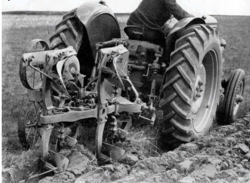
The TS 50 (two-furrow) and TS 51 (single-furrow) ploughs were produced by Ransomes Sims & Jefferies.
