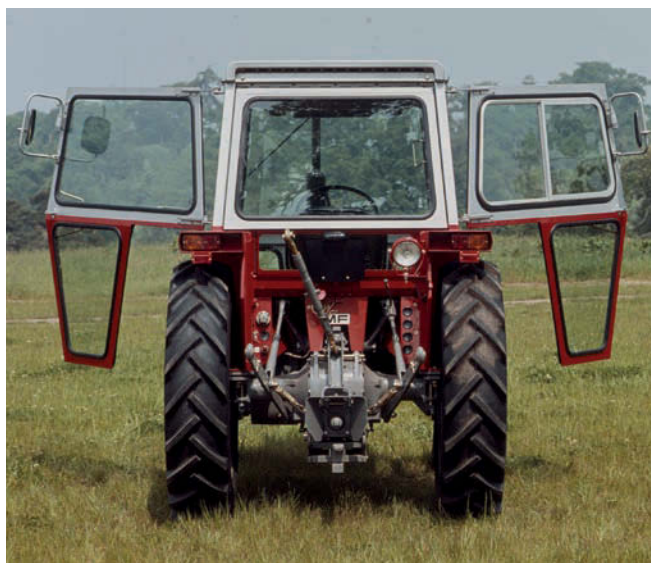
The second incarnation of the 550 (and the three other Coventry-built models) featured a two-door cab with sliding side window.
