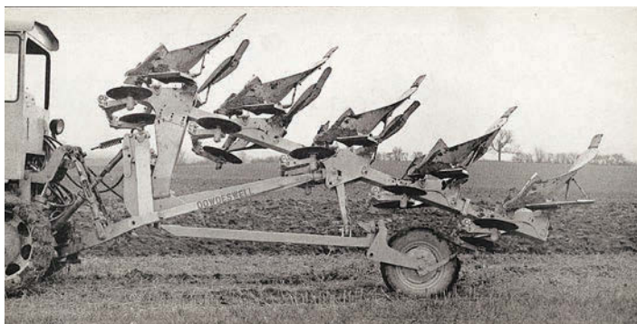
Roger Dowdeswell's DP1 plough, the first mounted reversible plough for crawler tractors, was awarded a silver medal at the 1970 Royal Show. The depth/transport wheel remained on the ground while the plough was reversed.
