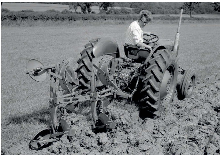
The Massey Ferguson 797, introduced in the 1950s, was one of the first reversible ploughs to use a hydraulic turnover mechanism. Photo: AGCO.
