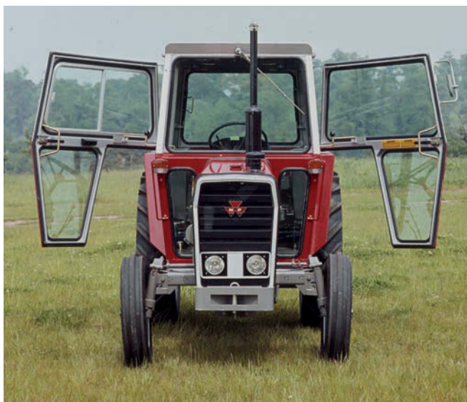
The second incarnation of the 550 (and the three other Coventry-built models) featured a two-door cab with sliding side window.
