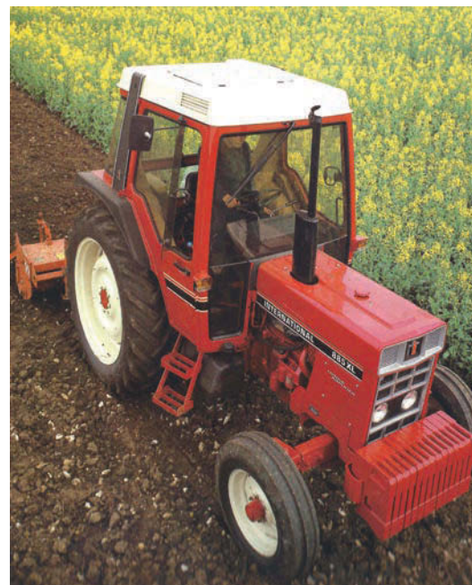
The dual-shaft PTO meant switching from 540rpm to 1,000rpm was simple.
