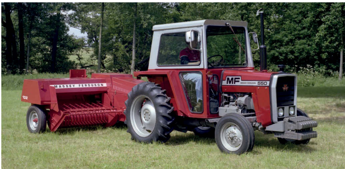
Many 550s were fitted with 6.00-16 front tyres and 12.4/11-28 rears. List price for the standard tractor in June '76 was £4,100.
