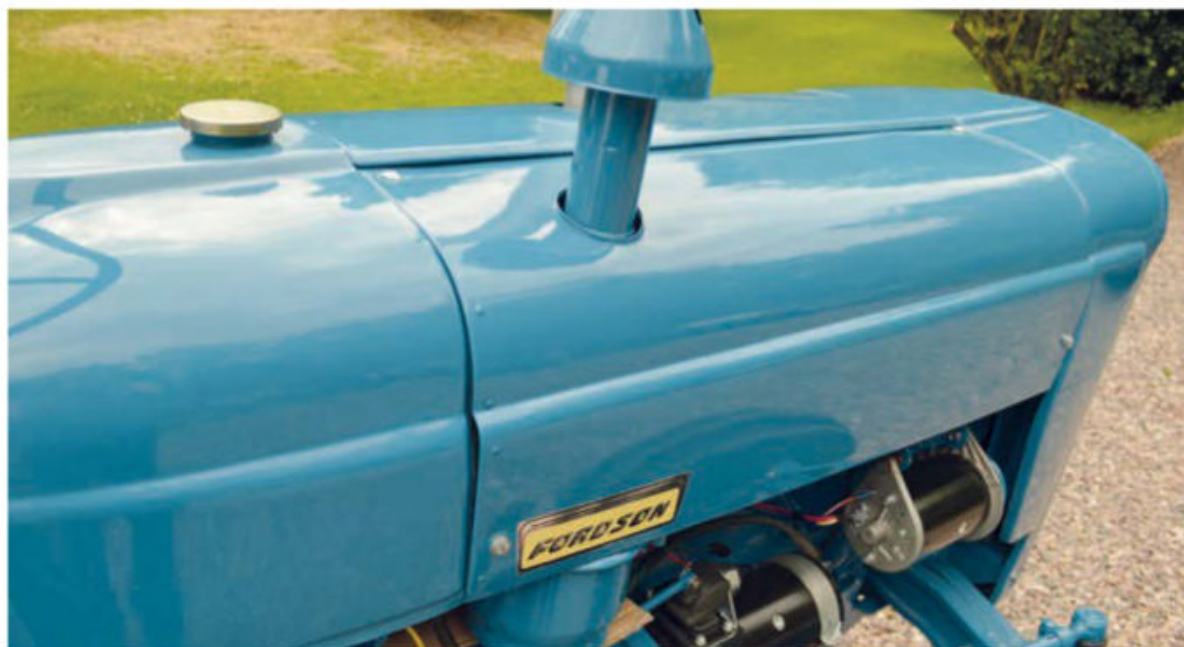
Another change in tinwork was the bottom line on the Super Dexta, which was now straight compared to being stepped down at the rear.
