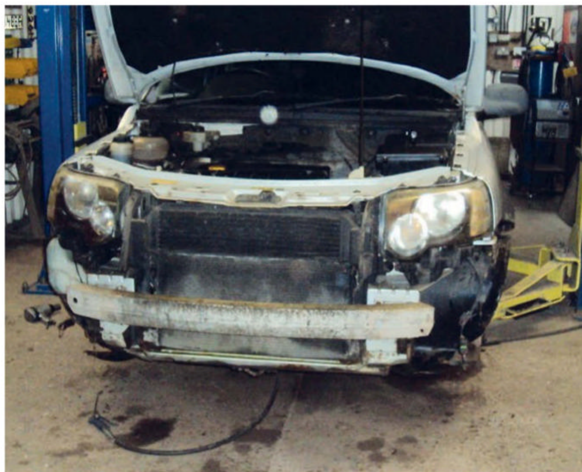
The front bumper has to be removed from the Freelander before I can get the intercooler off.
