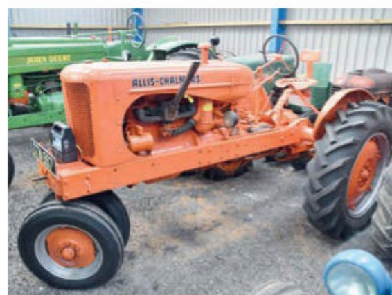
Mike's Allis-Chalmers CA. The live PTO on the tractor was because of a hand clutch that "broke" the rear axle, causing the differential to spin freely.
