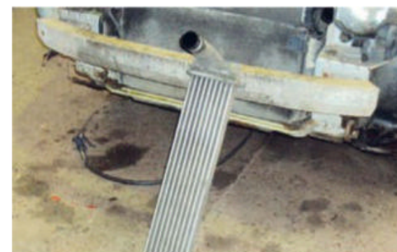
There was quite a bit of oil in the rad when I tipped it up, it got a good wash out with petrol.
