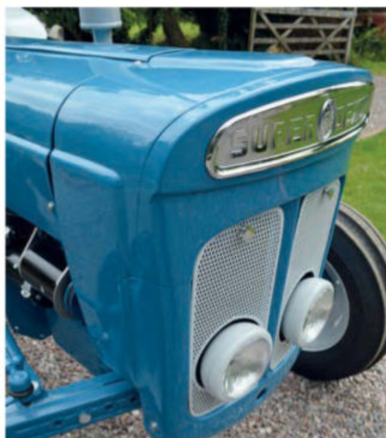
The front cowl was one of the most visible differences from the earlier Dexta models. The design was very different to what Fordson had produced previously.
