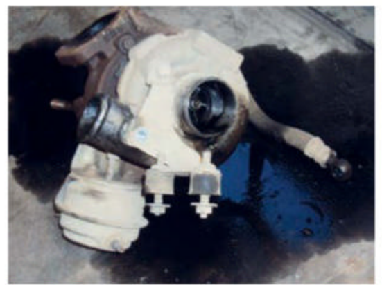
Oil had got in to all sections of the turbo, this was not good.
