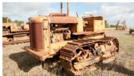
Looking so clean showing its West Coast, US is the 1945 Allis-Chalmers HD10 with the four-cylinder GM 4-71 two-stroke diesel were good crawlers for their time.
