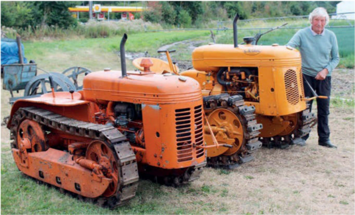
Robin fitted rubber pads to the HG 42 an option when built. The original nose cone on the HG 42 has been replaced.
