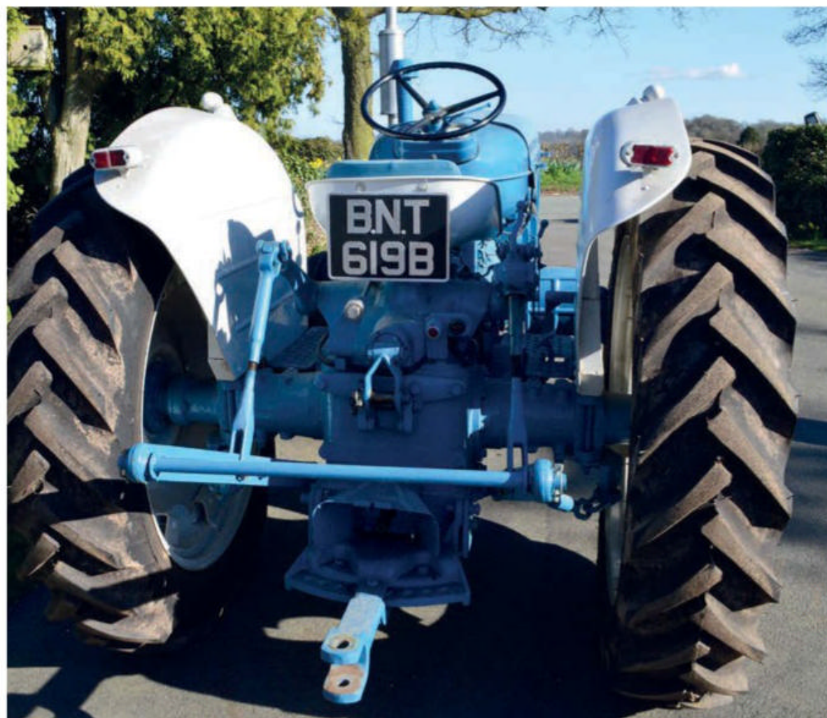
The hydraulics on the Super Major were said to be "A great advance in tractor design" thanks to the dual flow control. Having good hydraulics was important.
