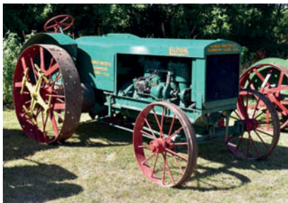
Very rare in the UK is the Illinois Super, which was known for its sprung rear wheels.
