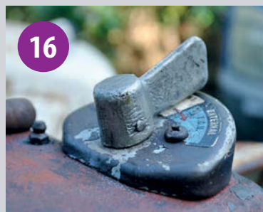
I replaced the broken roll pin with a solid pin.
