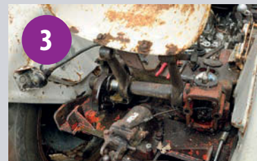
3 The whole lift arm has to come with the housing until it is clear of the bearing.
