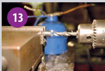
Using the mill to bore the end of the shaft, as I couldn't fit it in the lathe.
