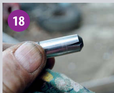
The dump valve body after polishing with 1500 wet and dry.
