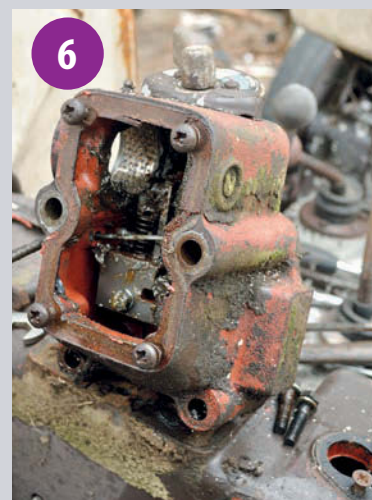
6 At first look, it appears to be a mess, but it's just old grease inside the housing.
