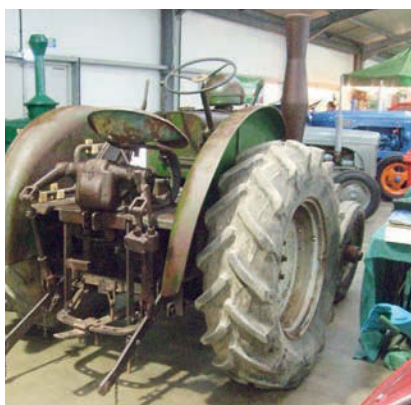
John Stephenson's Series 2 on the Marshall Club stand at Newark tractor show 2021. This tractor has been fitted with an Adrolic power lift and linkage. Photo courtesy of the Marshall Club.
