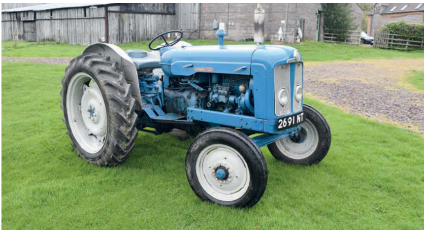
The 55hp New Performance Super Major was introduced in July 1963 (08C-960337-F), with a new colour scheme of New Performance Super Major blue, matched with grey-painted, pressed-steel wheels and mudguards.
