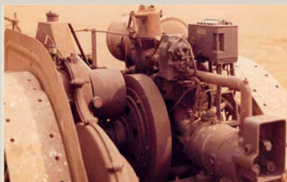
The opposed two-cylinder engine on the Moline Universal - who has this tractor now?
