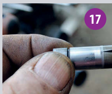
The dump valve body as removed.
