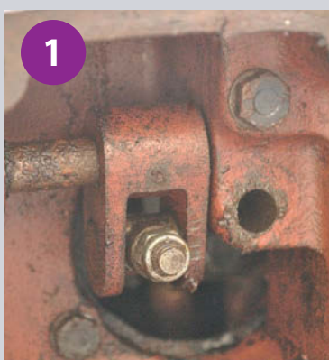
1 To extract the valve block, the control rod needs disconnecting first.
