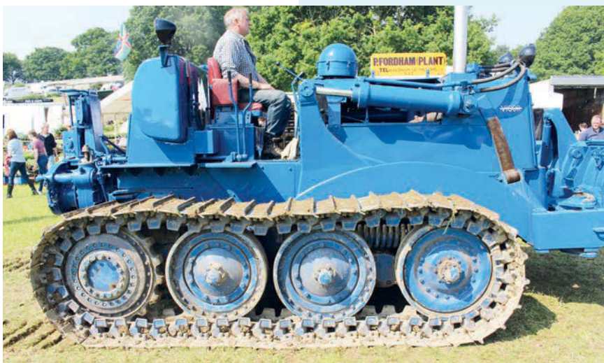
A unique feature of the Vickers crawler is the track running gear.
