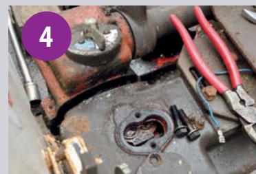
4 I discovered both valve covers need to be removed to get the assembly through the hole.
