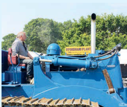
The straight pipe chrome exhaust makes for a unique engine note from the 190hp 12.14 litre Rolls-Royce six-cylinder, supercharged, diesel engine.
