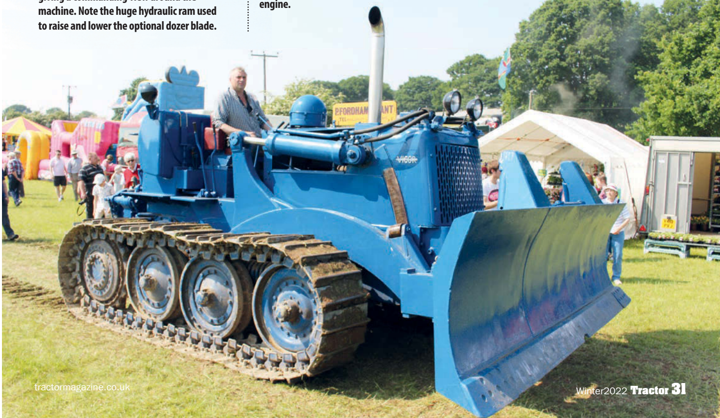
The straight pipe chrome exhaust makes for a unique engine note from the 190hp 12.14 litre Rolls-Royce six-cylinder, supercharged, diesel engine.
