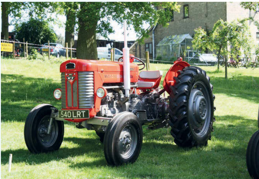
The first 50hp Massey Ferguson 65 arrived in 1957 and was based on earlier North American designs. It was fitted with the same six-speed gearbox as the smaller 35.
