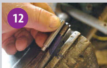
Measuring to determine where to cut the shaft with the replacement end.
