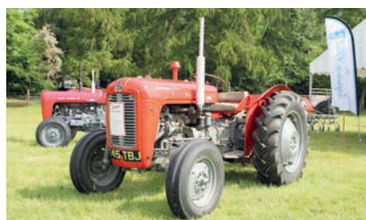
Fitted with the Multi-Power transmission, as proudly proclaimed on the side of the bonnet, this tractor had the benefit of 12 gears to choose from.
