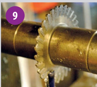
Cutting the slot on the mill for the valve rod roll pin to engage.
