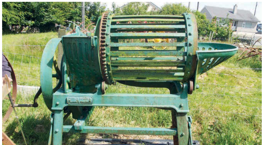
Built by Harrison, McGregor & Co this unusual root chopper is more elaborate than most and features a barred rotating cylinder which lies horizontally between the hopper and the blades.
