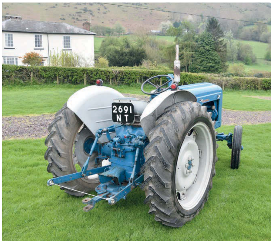
By the time of introducing the New Performance Major, the design had finally reached its potential. Extra goodies included disc brakes, a differential lock and draft control.
