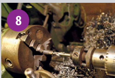
Boring the hole for the lowering speed repair piece.
