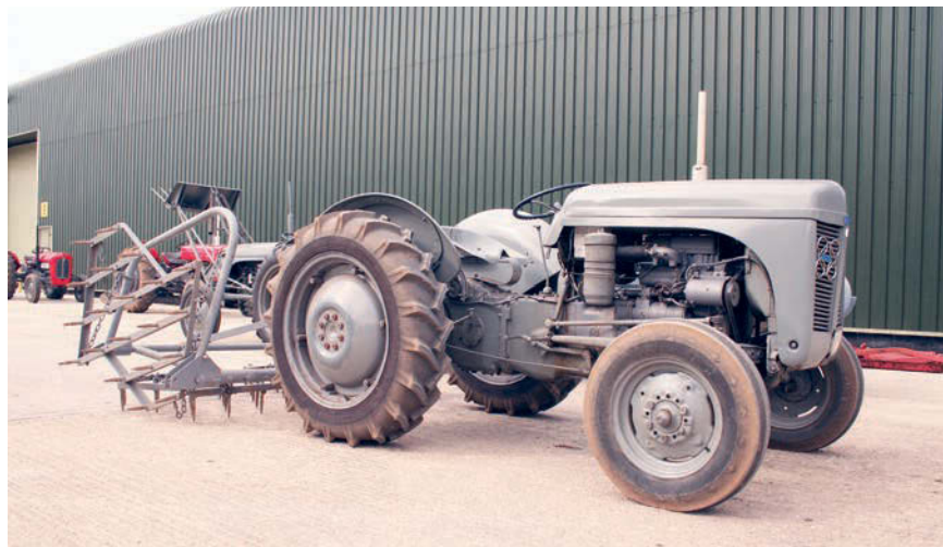
Before the TE-F20 version arrived in 1951, many owners upgraded their petrol powered 'Fergie' to diesel power by fitting a Perkins P3 diesel engine. Note how the bonnet had to be raised significantly to accommodate the taller engine, which also led to stability issues.
