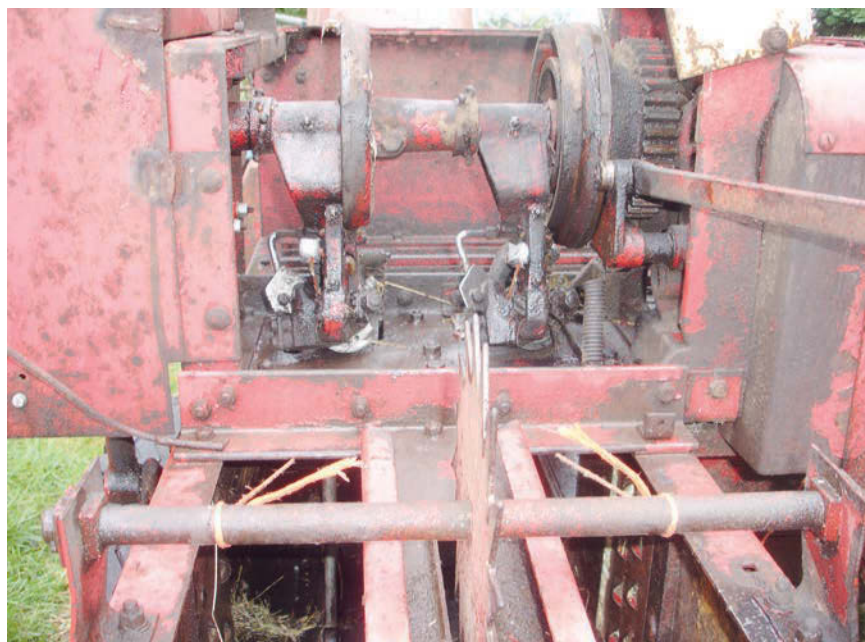
Once all the muck was blown away, I sprayed all the knotter mechanism with "duck oil".
