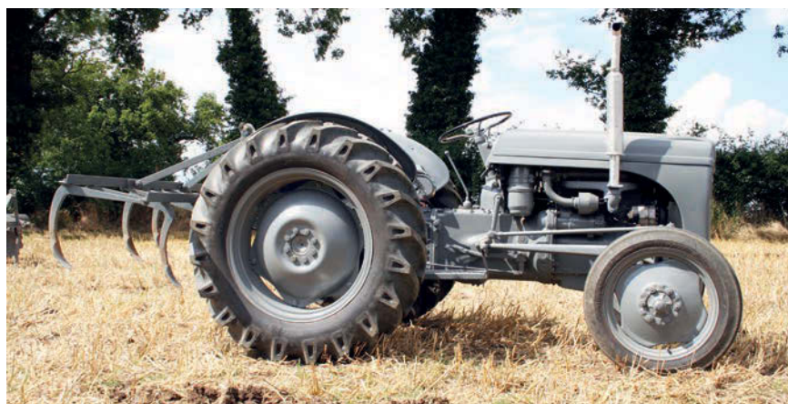
Despite a four-cylinder diesel engine being fitted, the Ferguson TE-F20 retained the same sleek lines of the earlier TE-20 tractors.
