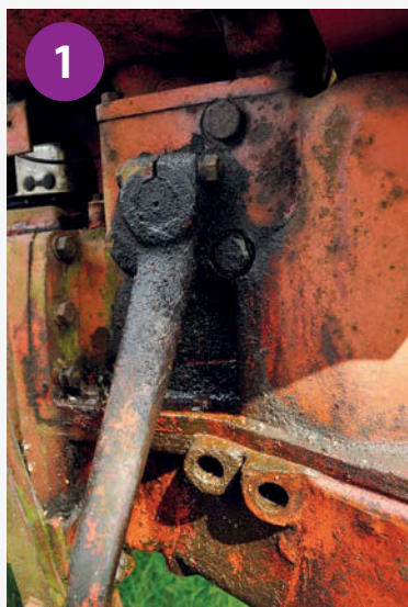
The oil leaking from the steering box is getting worse.
