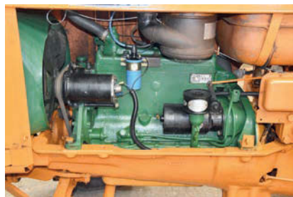
The 2383cc side-valve engine was rated at 30hp and was mated to a five-speed gearbox.
