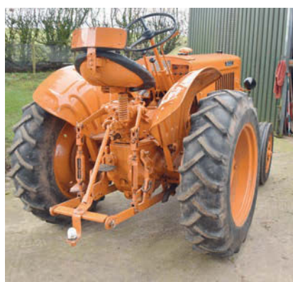
Standard equipment included a two-speed PTO, hydraulic lift, and adjustable tread.
