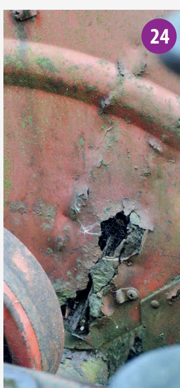
The other wing is nearly as bad and will need similar remedial treatment.
