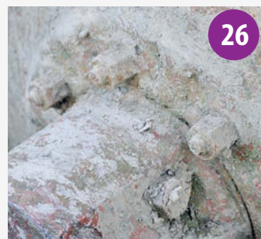
The rear wheels will need to come off, the nuts may need some heat to shift as they have not been touched for a while.
