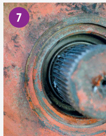
Before replacing the seal, the housing is cleaned out with brake cleaner.
