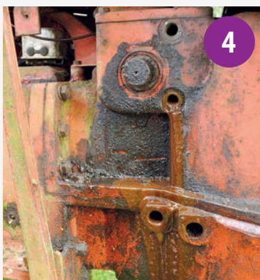
With the arm out of the way, I drained the oil (into a suitable container).
