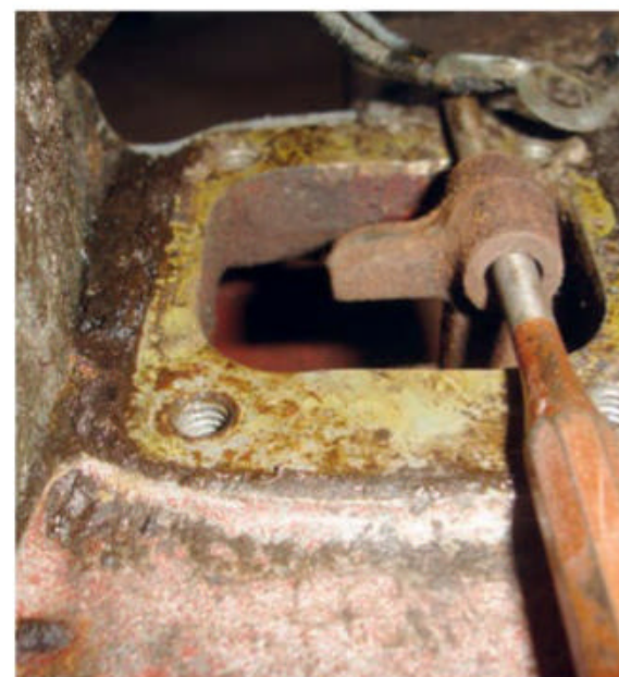
Graham left the punch in, so the linkage did not drop.
