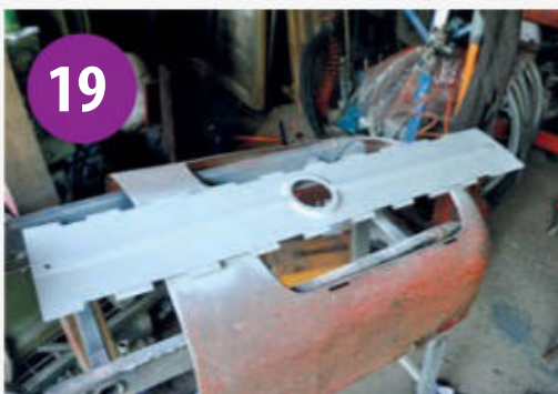
The central bonnet panel needed a fair bit of filler as well.
