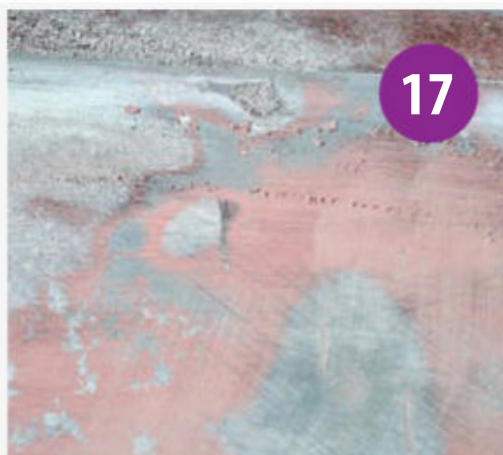
You can now see the low spots, including the scratches of the coarse paper used as the dark paint is left in the hollows.
