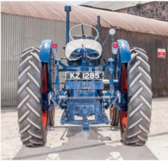
The hydraulic pump was replaced and the three-point linkage had new parts fitted.
