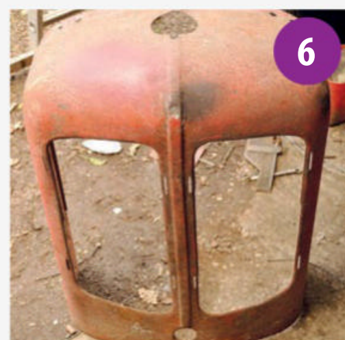
After knocking out some dents the nose cone is ready for sandblasting.
