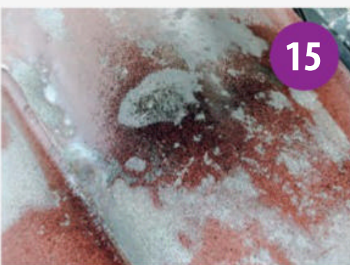
Using a contrasting colour, spray paint lightly over the spray area, let it dry...
