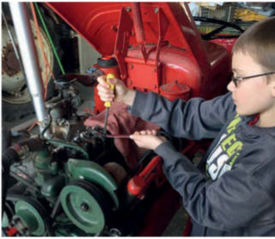
Cole McCloskey, Allen's grandson, adjusting the valves on the Fifties Volvo. Cole is keen to learn how things were done in the old days, but he is also the most internet-savvy member of the family.
