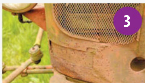
This is obviously not the original panel as it had a hole for the steering arm from a three-wheel model.
