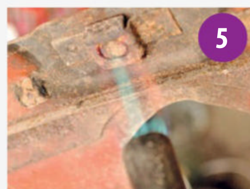
Using some heat, I managed to free the bonnet holding screw from the retained nut.
