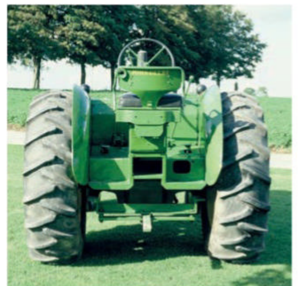
The rear end of the Model R featured a generously padded seat and independent rear wheel brakes.
