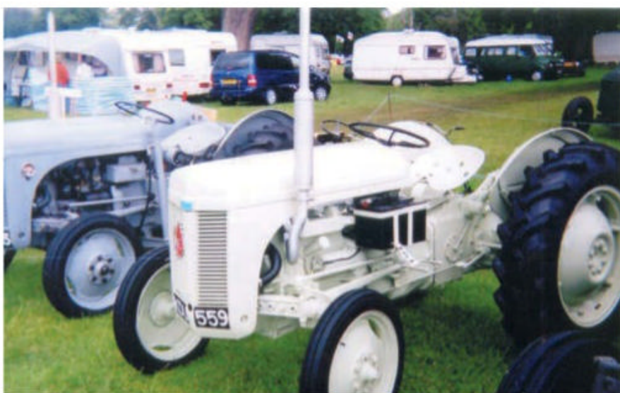
The grey Ferguson is fitted with a two-cylinder Meadows engine whilst...
