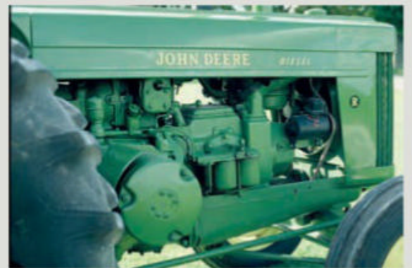
The Model R diesel engine was based on the John Deere twin-cylinder series.
