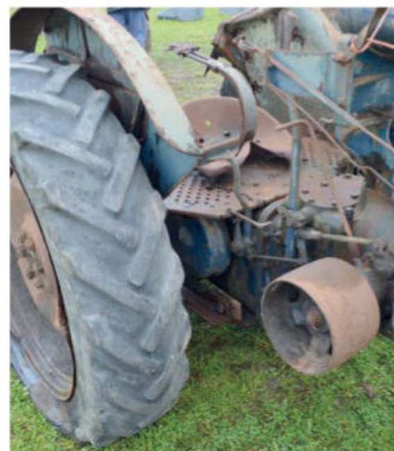
The other rear tyre was a more modern pattern and in slightly better condition. The rim, on the other hand, was very bent and buckled.
