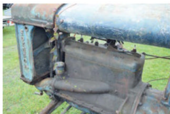
On this side of the engine on E27Ns is where they're prone to cracking, however, this one wasn't which was a bonus.
