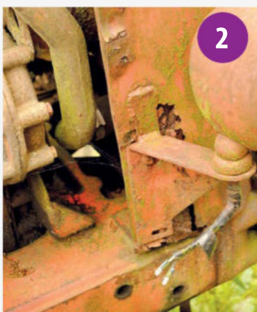
The headlamp bracket has been welded to the nose cone as it has rotted away.
