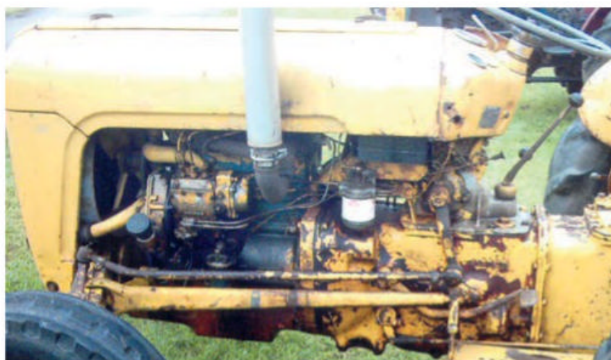
...the yellow Ferguson 35 is fitted with a three-cylinder diesel engine as fitted in a Ford Dexta tractor - note the industrial tractor style accelerator quadrant.
