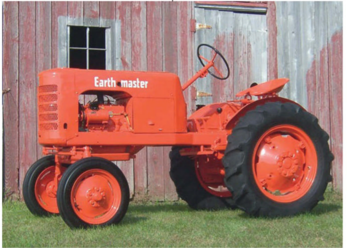
The 1948 Earthmaster is another lesser-known American tractor. Built in California, these were small, low-cost tractors. The company produced a range of tractors and equipment throughout the Forties, but they never sold in large numbers.
