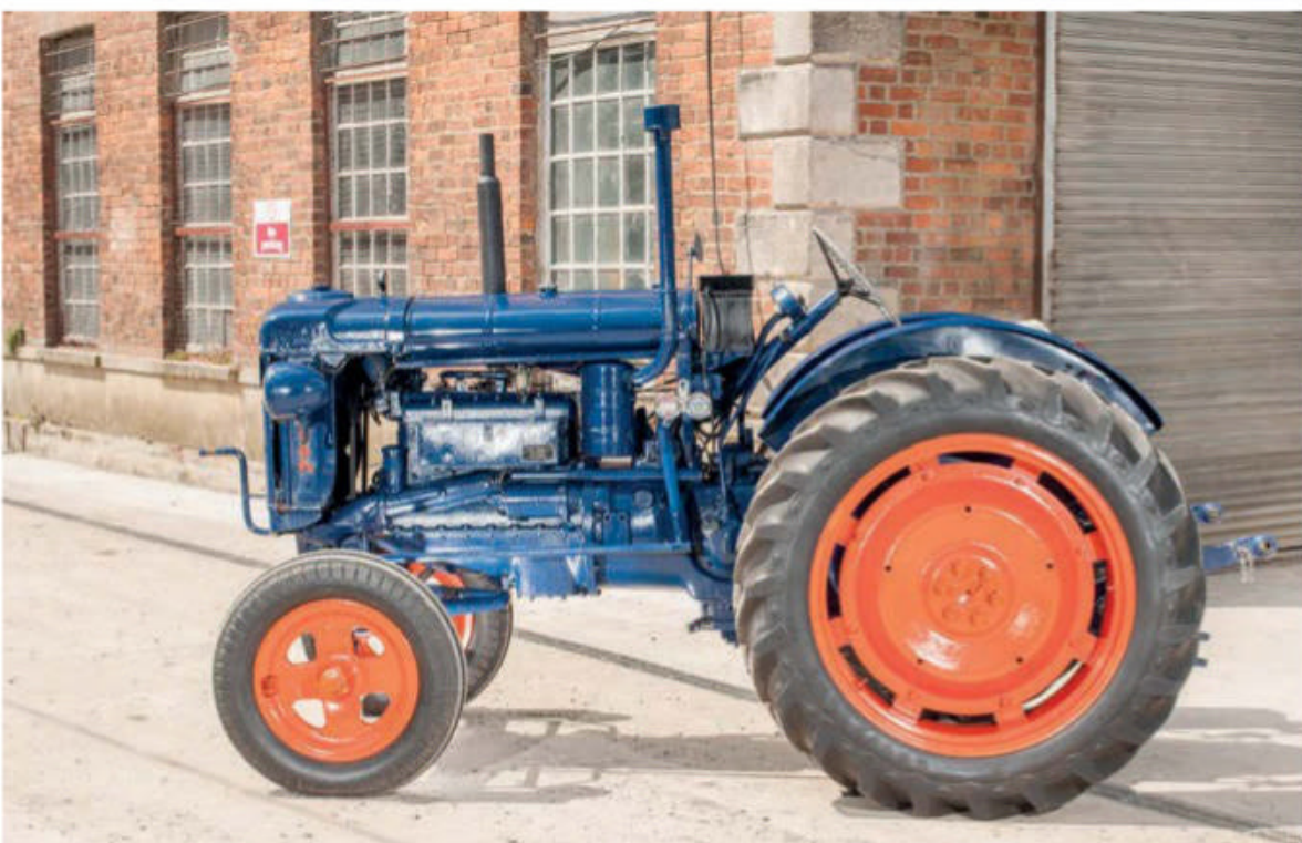
New mudguards, and new tyres on the original rims brought the E27N back to life.
