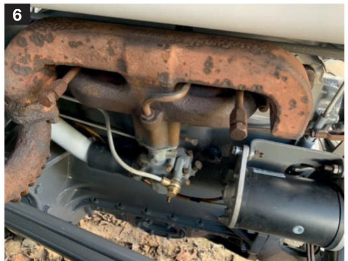
6 I soon found this carburettor leaked on the threads in the union so another solution was needed
