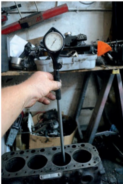
The long shaft allows measurements to be taken at the bottom of the cylinder.
