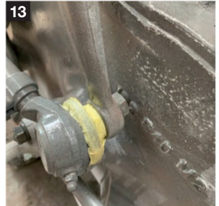
I even masked off the tire rod rubber boots as I hate these painted it's a fiddly job but worth it
