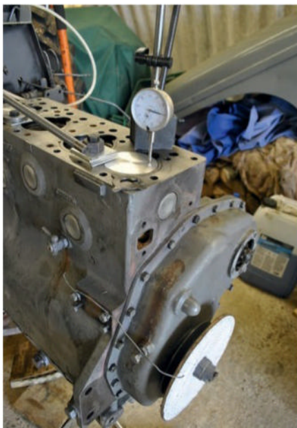
A DTI being used to find TDC while setting up timing.
