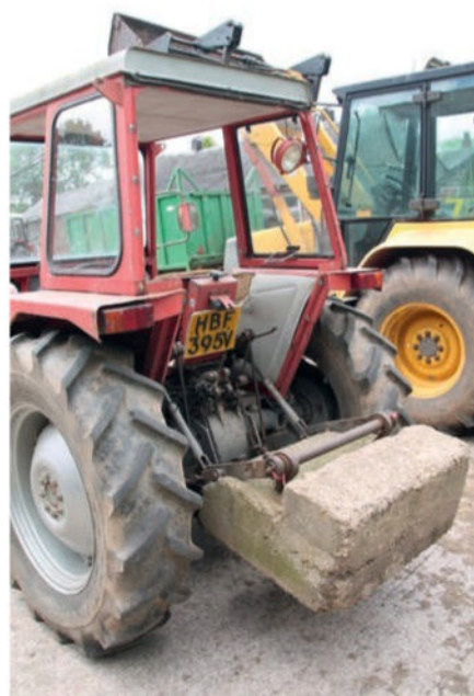
The rear view shows the considerable concrete rear weight in the 240
