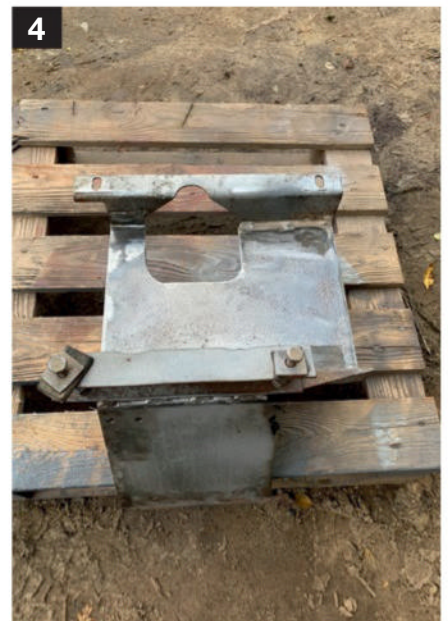
4 A quick grinding of the welds and a skimming of filler and this battery tray was finished
