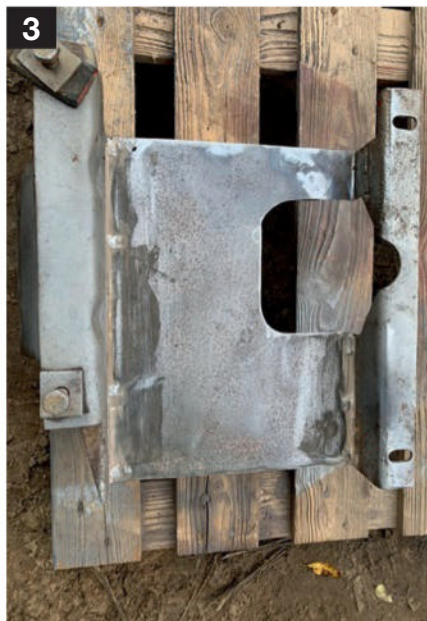
3 This tray now had a double bottom so was more than strong enough to take a battery
