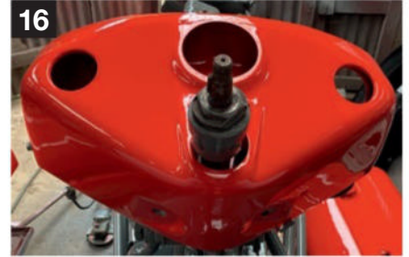
16 The dash here is bare and only fitted temporary to stop it being damaged until the gauges could be fitted
