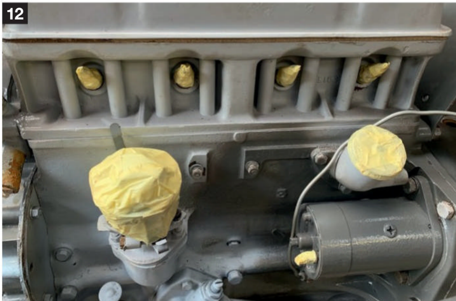
Here I am masking the engine up in preparation for it to be sprayed, some items have been removed
