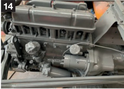
14 A few final coats of paint with a nice glossy one to finish and the skid unit was sprayed
