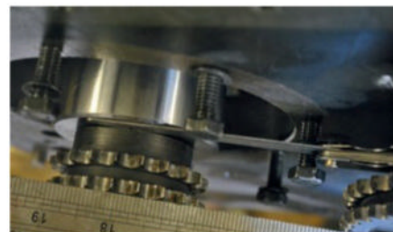
The lowly feeler gauge has its uses when on a rebuild: here it is checking the crank chain wheel clearance.
