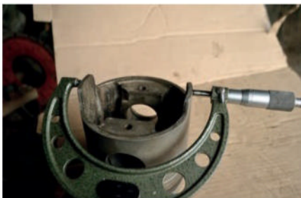
A micrometer measuring the base of a new piston: it was 0.002in larger at the base.
