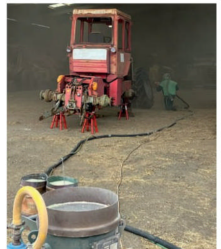
Keeping the sandblasting pot topped up takes some concentration, in order to keep up with the blaster up front!
