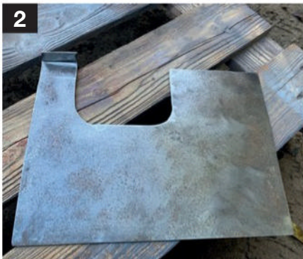
2 I cut this simple section of metal to weld into place, the right angle part was bent to cover that rotten bit
