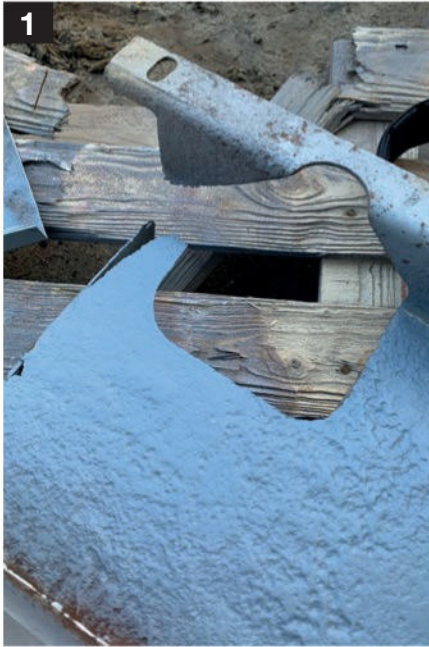
1 This battery tray was slightly rotten so a repair was needed, I believe the bonnet had been removed for a while so this was open to the weather
