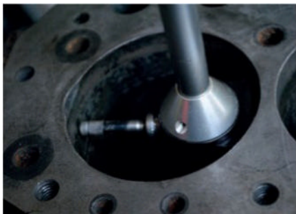
Measure below any ridge left by the top ring.
