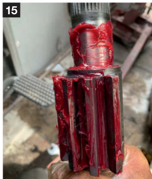
15 Even though the steering box would be refilled with oil once reassembled, I still coated the working parts with grease.
