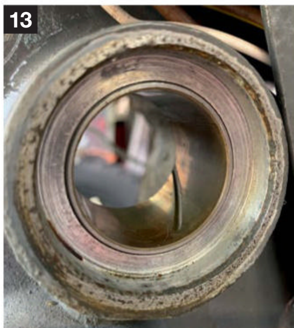
13 I treated the faces onto which the seal located to a good clean; the aluminium came up quite shiny.
