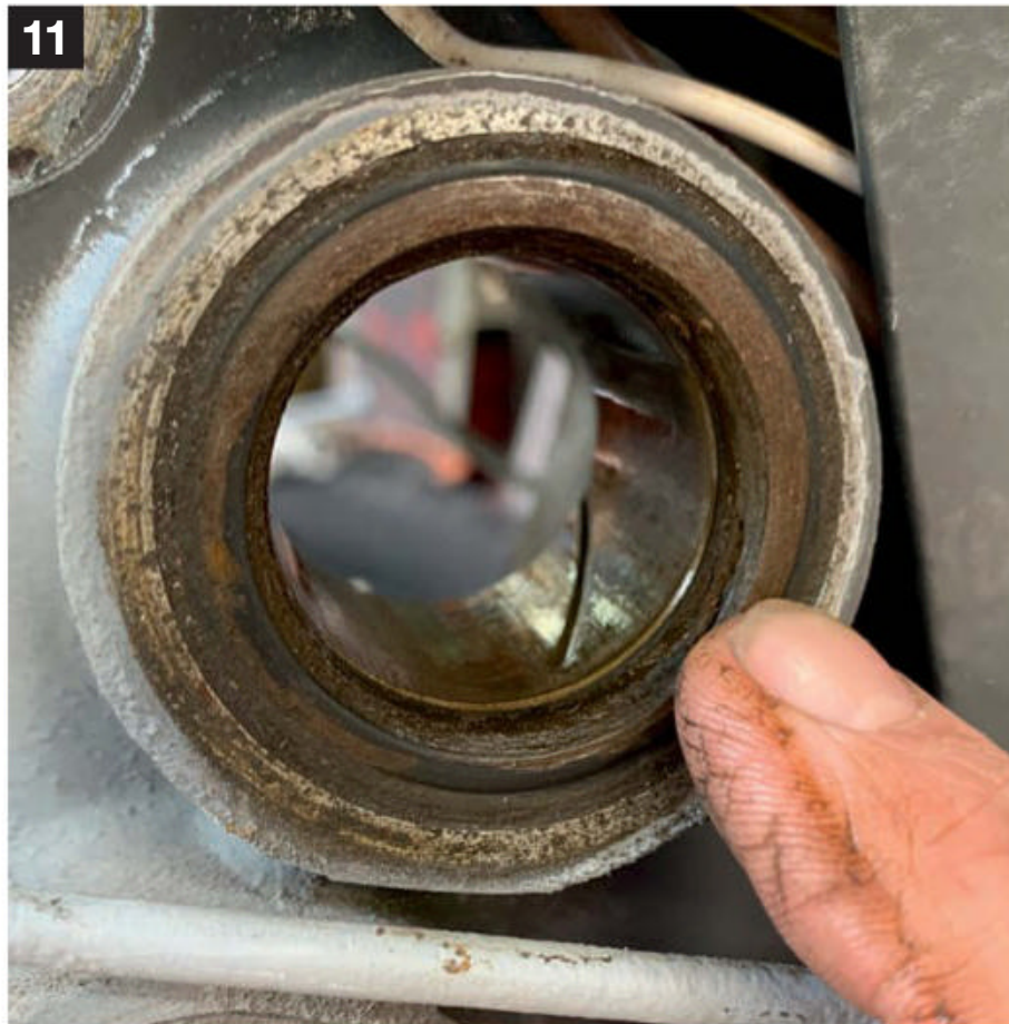
11 This oil seal was slightly worse than the other one, although the bushes in both were found to be in good condition.
