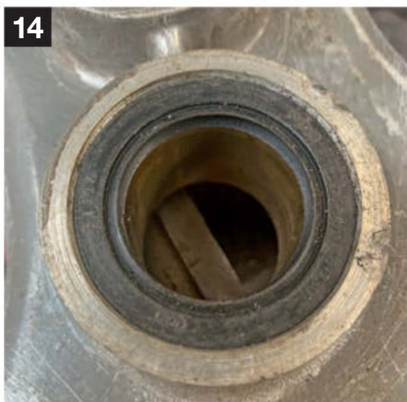
14 That looks much better; a nice new seal was gently tapped into place.
