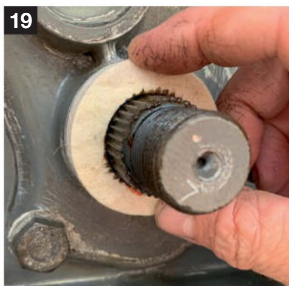
19 This felt seal – replacing the original, flattened example – protects the main oil seal and completed the job perfectly.
