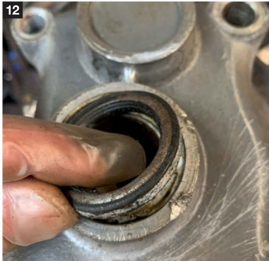
12 Removing the seal was quite easy as it wasn't a ridiculously tight fit. A good, flat-headed screwdriver was all that I needed.
