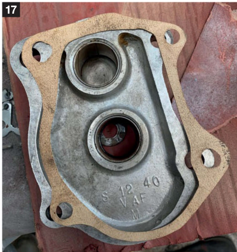
17 The old gasket was the cause of the leak that had prompted this whole rebuild. Here's the new, slightly thicker replacement I made.
