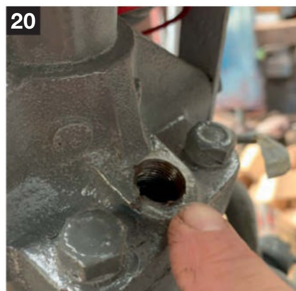
20 The reconditioned steering box is re-filled with oil via this hole that's located at the bottom of the steering column.
