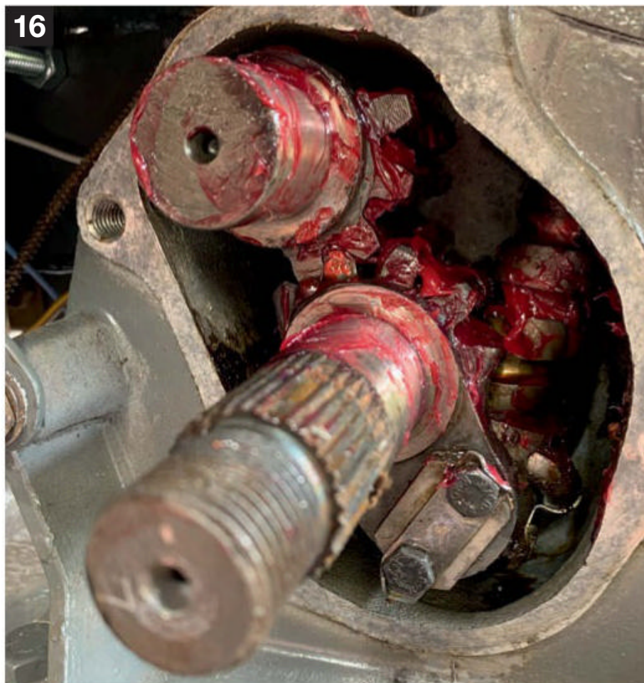
16 As you can see, I applied a fair bit of grease to most of the moving parts as some extra protection before the new oil got around and did its job.
