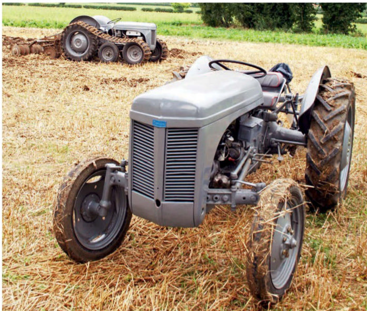
Here's a petrol TE-A 20 (foreground) with a TVO TE-D 20, launched in 1949 (complete with Bombardier tracks). With farmers wanting a cheaper alternative to petrol, the TE-D 20 was introduced. The engine started on petrol then, once warmed, was switched to TVO running.
