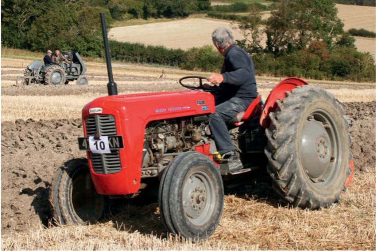
An early version of the MF 35 showing the ‘Ferguson’ badge on the bonnet, as carried by its predecessor, the FE 35. The 35 was a versatile farm tractor when new, and now makes an ideal ploughing match machine. It delivers enough power from its diesel engine (here a four-cylinder Standard unit), to make ploughing easy while, at the same time, being compact enough for straightforward transportation and storage.
