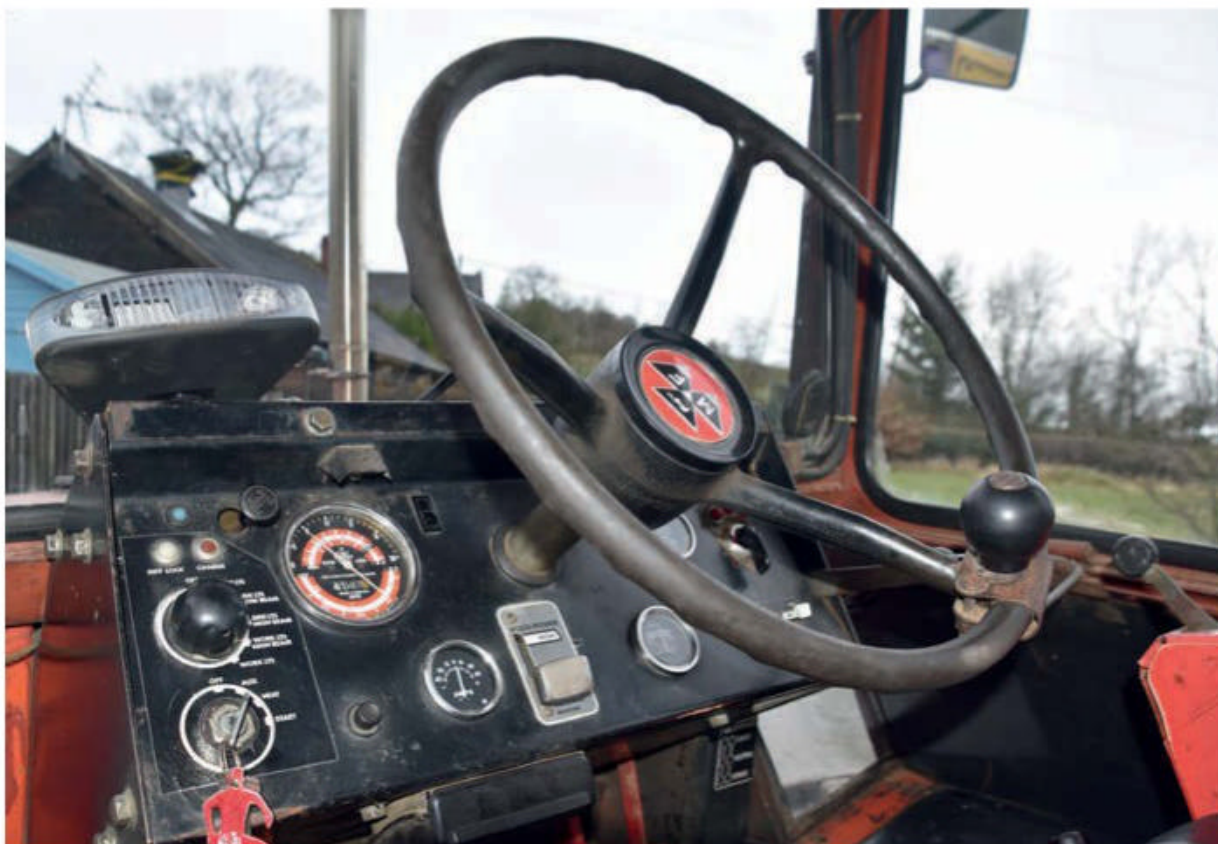
All the controls are straightforward and fall easily to hand, and the instruments were made by familiar names like Smiths Industries.
