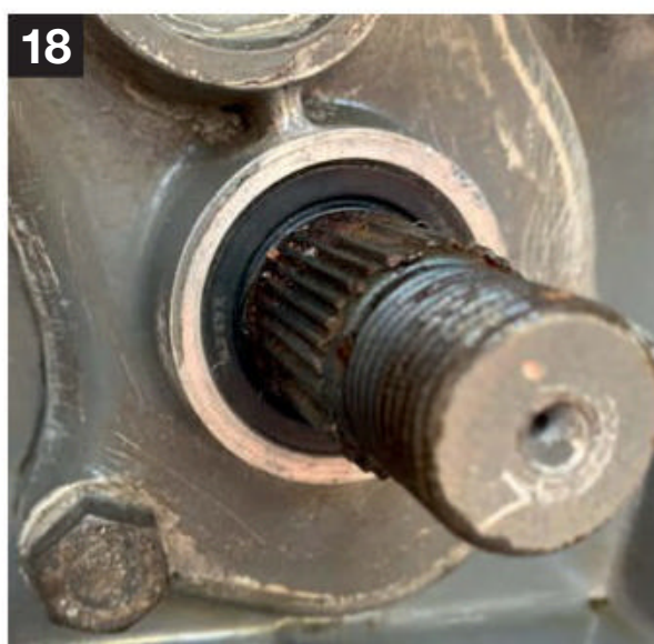
18 With the plate re-fitted and the new seal clearly visible, I was pleased that the whole assembly looked so clean and tidy.
