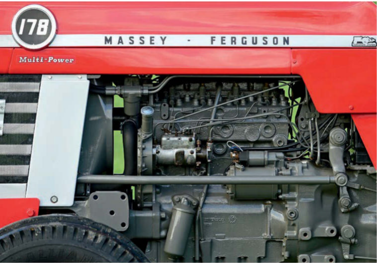
The Perkins engine benefitted from a nut-and-bolt restoration. The crankshaft was re-ground and new cylinder liners were fitted.
