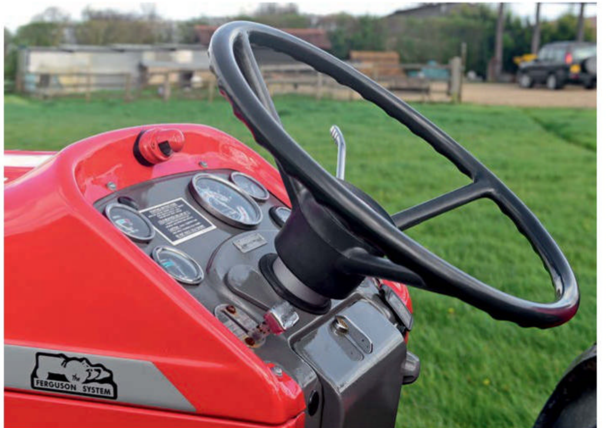
All the instrumentation is original and, once Simon had fitted a new wiring loom, everything was found to be operational.
