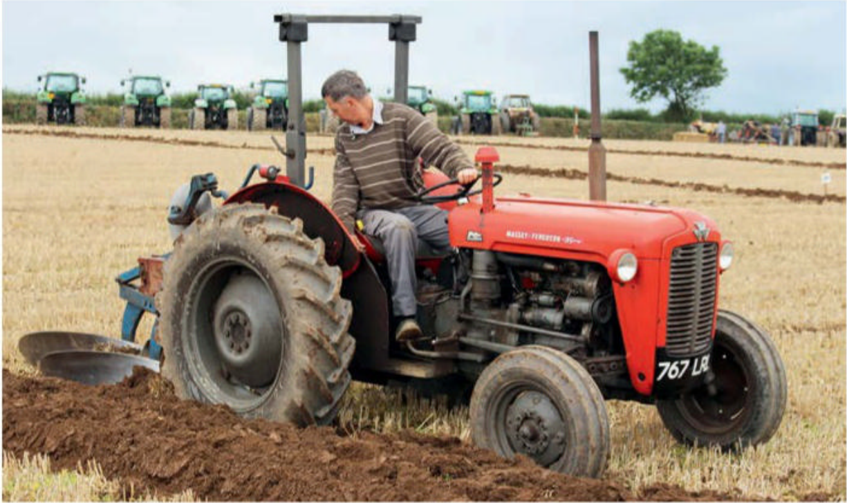
The later Perkins three-cylinder engine, which replaced the earlier Standard power unit, increased the popularity of the MF 35 still further. Following the safety cab legislation of 1970, older tractors such as the 35 were often fitted with a rollover frame to make them legal for use by employees. Although very practical, such additions did tend to distract slightly from the classic lines of the tractor.
