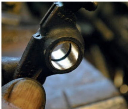
New bronze bearings fitted to the rockers...
