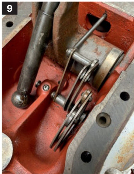
All the good reusable parts were stripped out from the old top cover and put in the new one.
