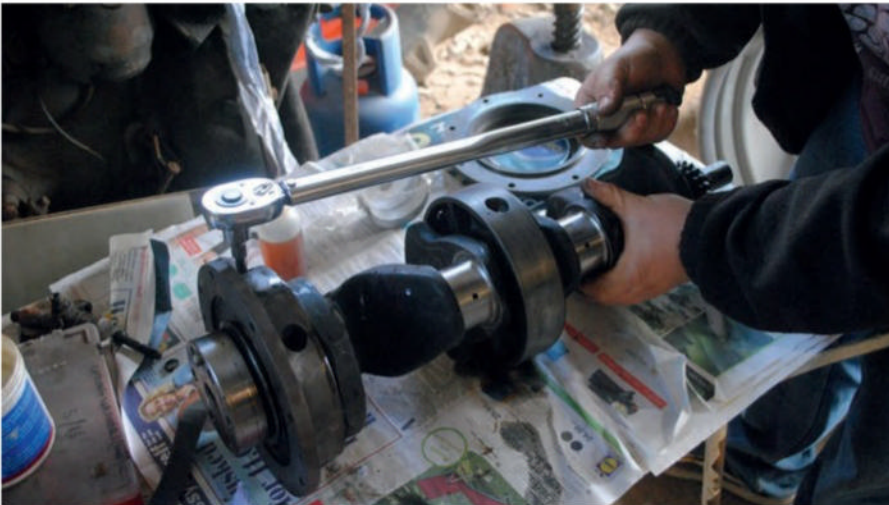
Torquing up the main bearing caps.
