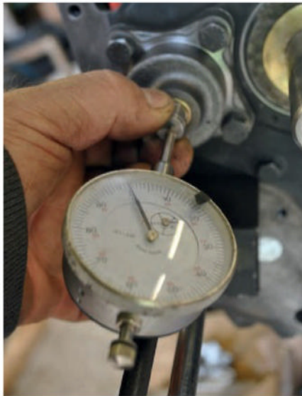
Checking the end float on the oil pump shaft.
