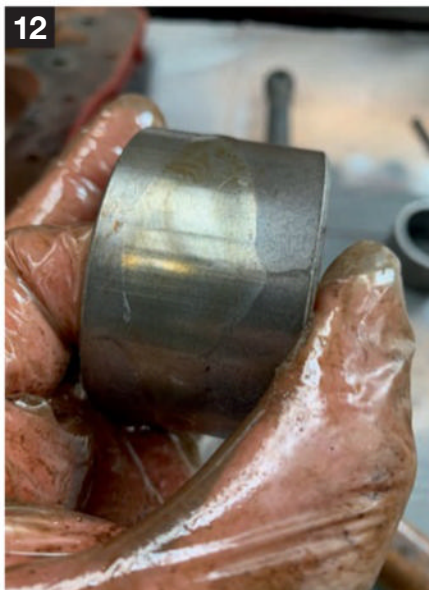
I had bought these bushes new; there were four to be fitted into the top cover.
