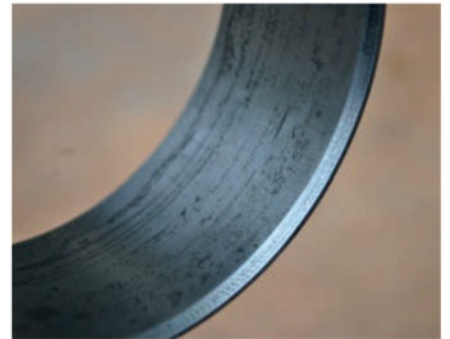
A chamfer was cut to assist the rings being compressed.
