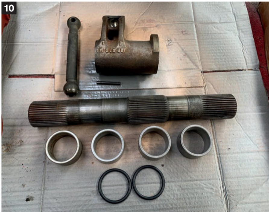
The main shaft, conrod and lift arm were from the old cover, and underneath there were four new bushes and two new seals.
