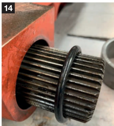
This rubber seal went in next and just slipped over the cross shaft, followed by another bush.
