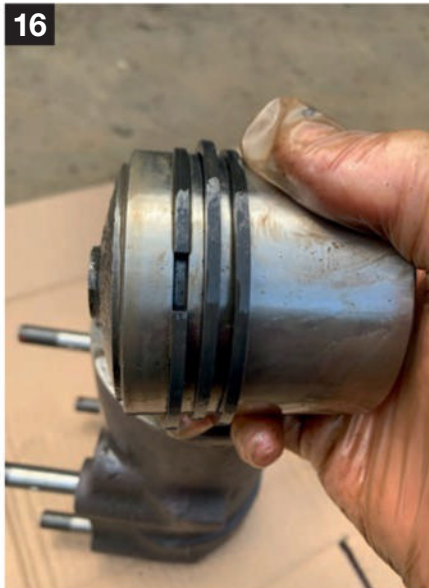
16 As you can see there's a complete set of three rings fitted; assembling this was similar to an engine piston.
