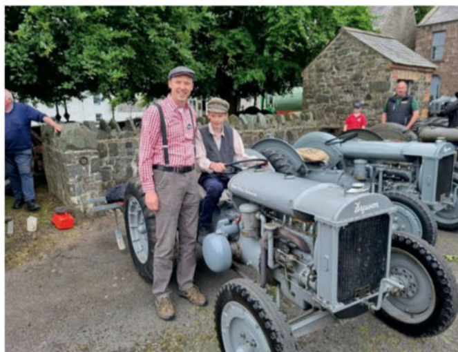
All in the family: the Ferguson Brown A with electric start mechanism fitted.
