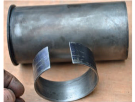
The home made ring compressor with cut out for fitting the gudgeon pin.
