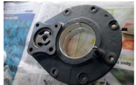
The front main bearing housing with the new shells fitted.
