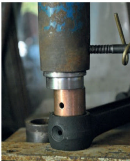
Pushing in new little end bushes; make sure the oil hole lines up with the hole in the conrod.
