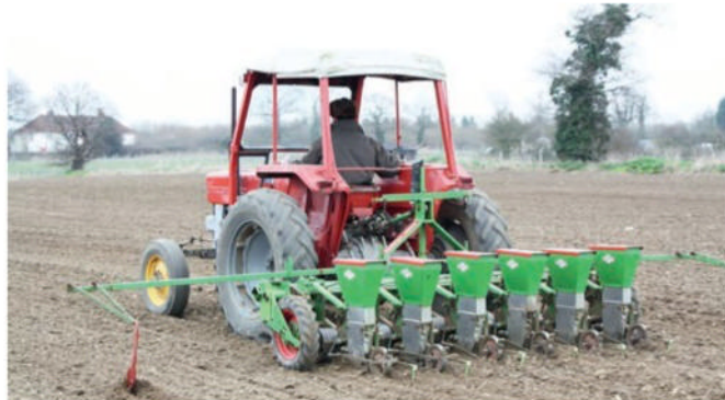
Many 135 tractors are still used on farms in Britain, including this one seen sowing sugar beet with a David Thomas precision drill in Suffolk. Most of the cladding on the cab has disappeared, as have the doors, but the roof, front windscreen and frame remain intact after six decades on one farm.
