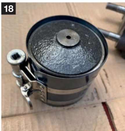
18 The piston ring compressor that I use for engines came in useful here: it's the smallest piston it's had to wrap around.
