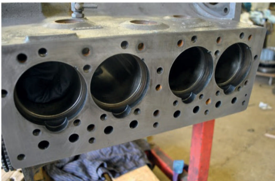
Make sure the seats for the new liners are spotlessly clean before reassembly begins.
