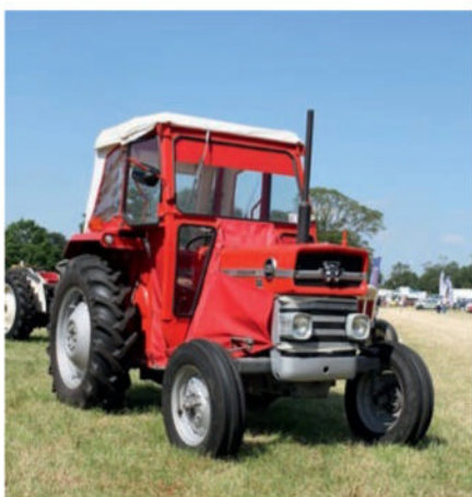
A superbly restored Massey Ferguson 135 complete with flexible clad cab, the version most often chosen given it was cheaper than the rigid alternative. This was probably the most familiar version of the 135, produced from 1971 to 1976.
