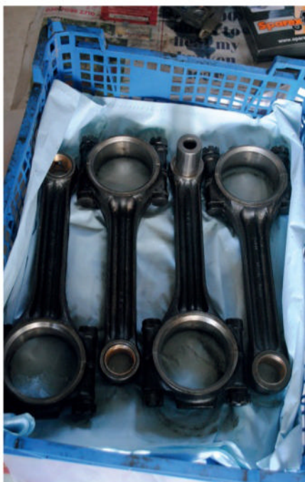
All four conrods fitted with bronze bearings and reamed to size.
