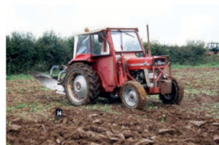
The 148 had extra power from an uprated Perkins three-cylinder engine and a long 6in wheelbase that made it more stable when lifting heavy implements on the rear linkage. The 148 was a superb tractor, but never sold in the huge numbers of the 135, mainly due to its increased cost, thanks to all its luxury features that came as standard.
