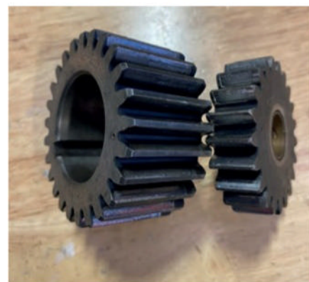
Rodney replaced the timing gears, which were making that worn noise.
