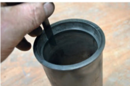
Using a new liner check the piston ring gaps are within spec.
