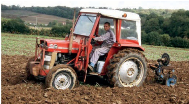
The 148 was a new version of the 135 introduced in 1972 as part of a new Super-Spec range, and fitted from new with either the Flexi-cab or rigid clad cabs. This very original example is fitted with the frame for a front loader and was being used at a ploughing match in southern England. (Photo: Kim Parks)
