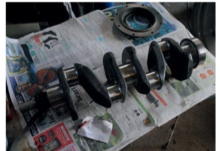
A polish of the crank journals with very fine emery cloth will help bed the new bearing shells.
