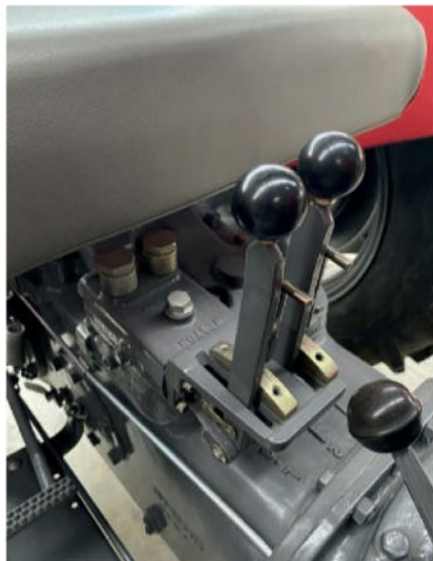
The dual spool valves: looking perfect after the overhaul.
