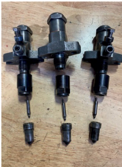
The injectors carried the wrong bodies.
