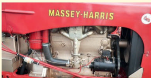
The Continental E206 engine certainly has a long stroke.
