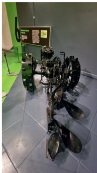
The back end of the 'Black Tractor', which features a four-piston hydraulic pump. Photo: Aaron Taylor
