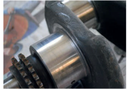
The crankshaft front main bearing in good condition.
