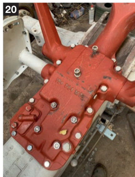
20 Jumping forward this was the replacement top cover all complete and working on the tractor. This part was set up by a Massey Ferguson expert.
