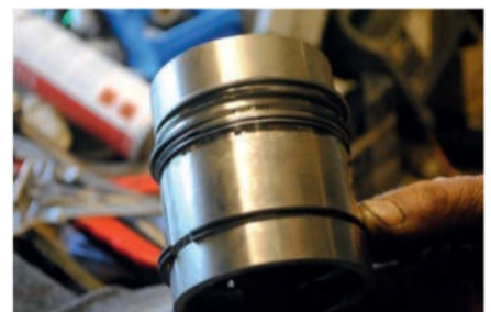
New piston with all the rings fitted: ensure the top compression rings have the 'T' facing upwards!
