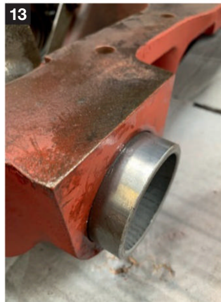
These bushes tapped in with ease. I had bought new as the old ones were rusty and took some removing.
