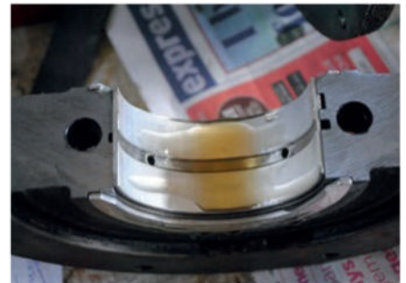
Always use plenty of oil when reassembling on a clean surface.
