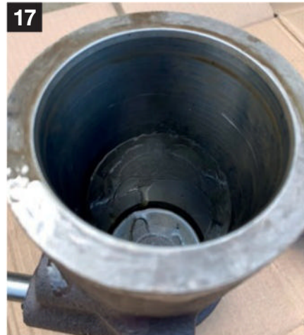
17 Also, like an engine, the cylinder received a good dose of lubrication before the piston was slipped in.
