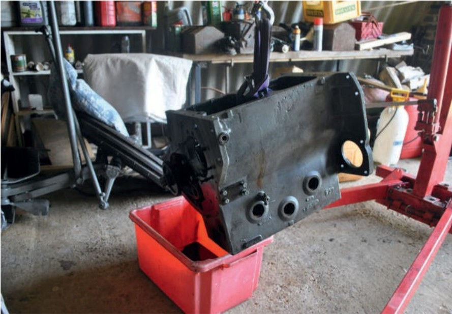
A good wash out of the engine block before rebuilding.
