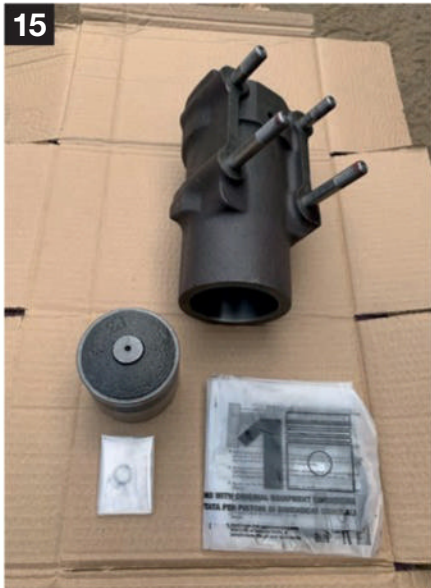
15 A new hydraulic cylinder, piston and rings await assembly – also note that a set of specially made studs are installed in the cylinder.
