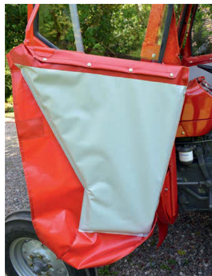
The door cover is double-skinned, with a section of foam between the layers of plastic, as per the original design.
