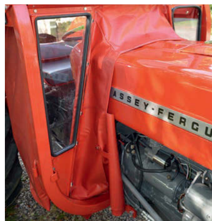
At the other end of the bonnet, the cab surround hugs the dash as it should do, to help protect the driver from draughts.
