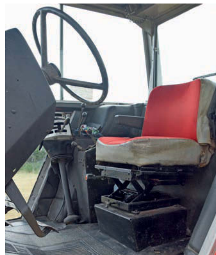
The 2640's cab was a market leader when the model was introduced. Once inside, the operator was completely sealed away from noise, dust and the elements.
