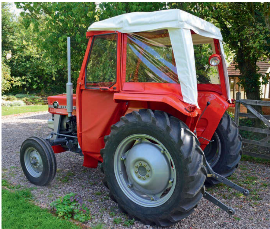
The cab on Alan's 135 was known as a flexi cab, and offered quite good weather protection. The cover was made new and I consider that the quality is outstanding.
