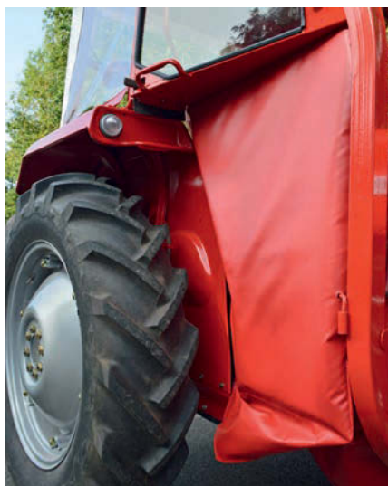
The cover extends down the full length of the door, over a frame to give it rigidity.
