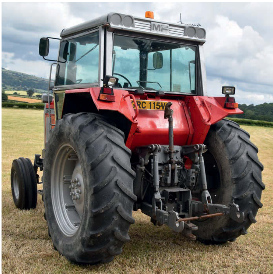
The back end of Richard's 2640 is in decent shape, although he's had to replace the blocks used to guide the hydraulic arms up and down.
