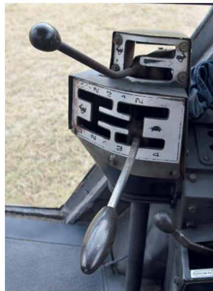
The 2640's eight-speed gearbox was used in combination with a two-ratio power shift speed-reduction unit.
