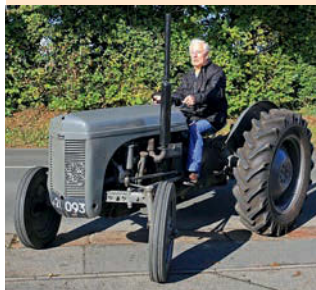
Lyndon Pallot on his Ferguson TE-20 which was fitted with a Perkins P3 conversion by Central Motors.
