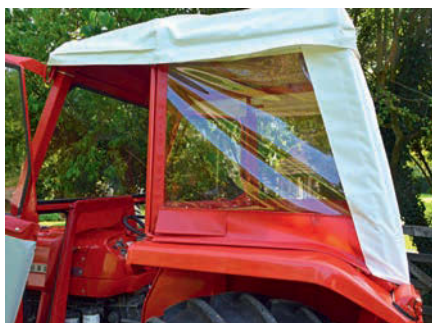
As the cab covering is new, the side window is lovely and clear, ensuring great visibility. Note the red flap below, for hand signals!
