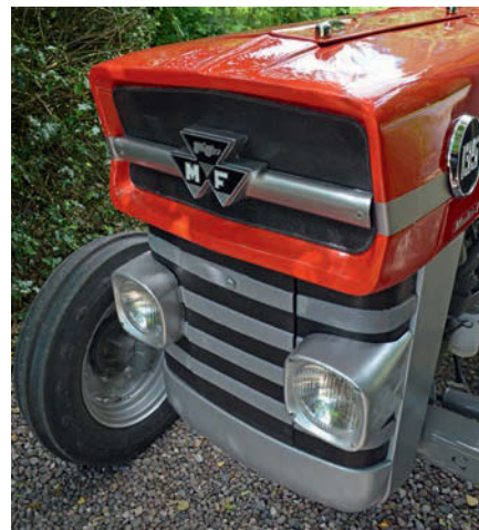
The familiar front end of a Massey Ferguson 135; new headlights and cowls, plus the upper badge bar, were fitted.
