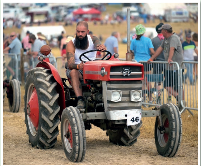
▲ You don't see too many MF 130s around, so it was good catch sight of Gary Cresswell's 1965 vineyard model that's powered by a Perkins P4 diesel engine.
