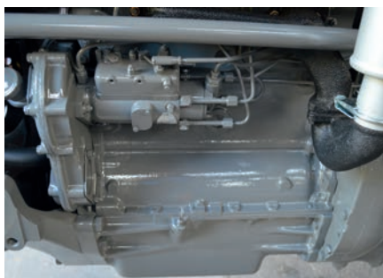
This Perkins AD4-203 engine has been the subject of an extensive rebuild.
