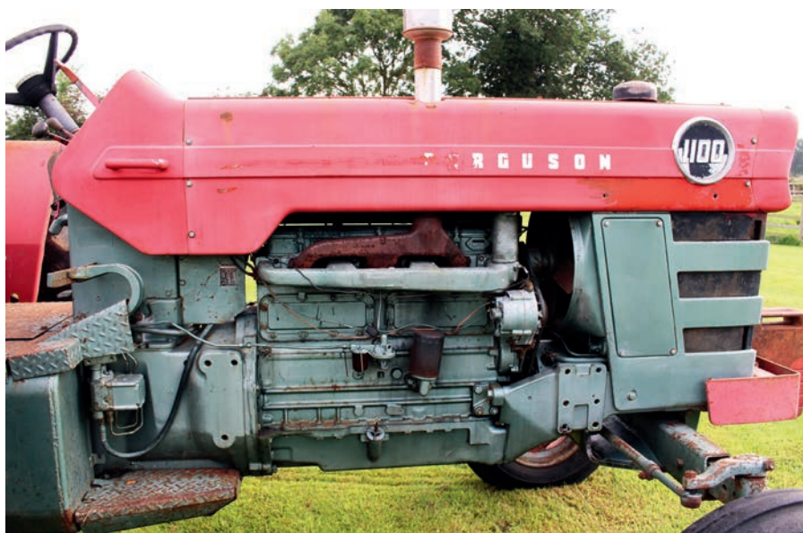
The 105hp engine that powers the 1100 is a Perkins A6.354 six-cylinder diesel unit, with a 5.8-litre capacity. In North America this model could also be specified with a petrol- or LPG-fuelled engine.
