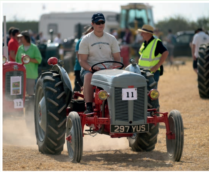
▲ This tractor was listed in the programme as Mick Jones' 1957 Massey Harris Ferguson FF30DS. It's said to have been built in France, and is powered by a French engine from the Standard-Hotchkiss Co.
