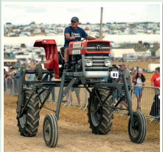
▲ This is a very rare machine; it's a 1973 MF 135 Flamingo High-Crop. Only 10 examples were built by Kent-based Lenfield Engineering, having been designed for spraying and dusting bean fields. This example was new to Chalk Valley Contracting in Bowerchalke, and was entered by Tim James from Child Okeford, Dorset.
