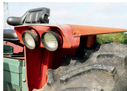
Twin headlamps were mounted in the leading edge of each rear mudguard – or fender, as they’re called in America – and provided plenty of illumination from this position. These lights were replaced by a pair in the radiator grille for the 1100s that were built to be sold in the UK market.
