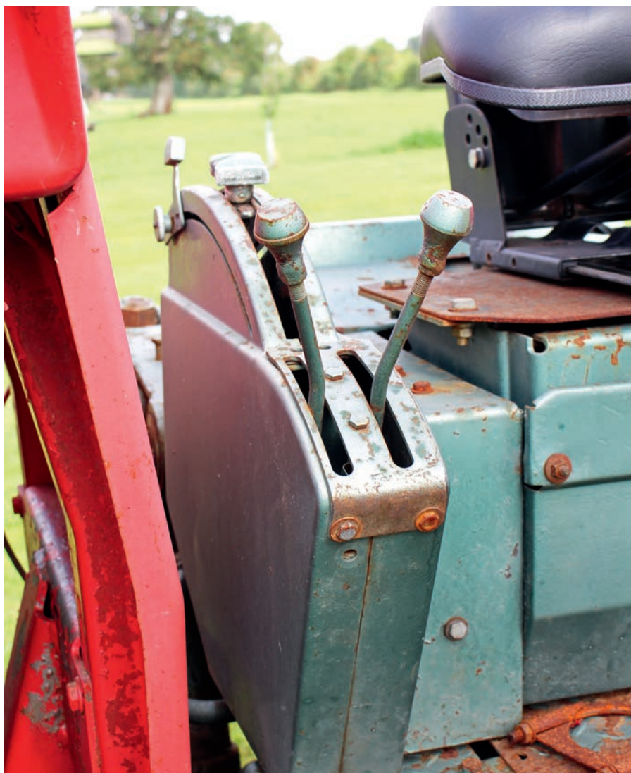
The easy-to-use hydraulic controls for the rear linkage were conveniently positioned in a quadrant to the right of the driver's seat.
