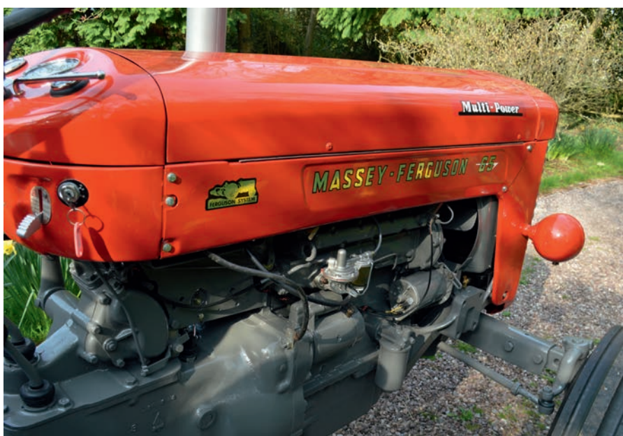
The repainted and re-hinged bonnet looks great with its new decals.
