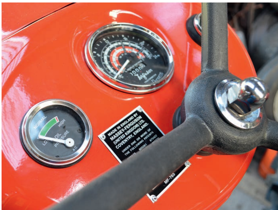
The upper dash was fitted with three new dials and a commission plate. The new steering wheel got a replacement chrome nut and washer, too.
