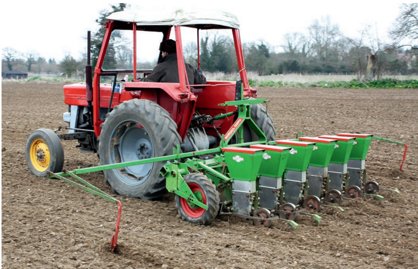
The low driving position and excellent visibility of the rear-mounted David Thomas precision drill made the Massey Ferguson 135 ideal for planting this Suffolk farm's crop of sugar beet every spring.
