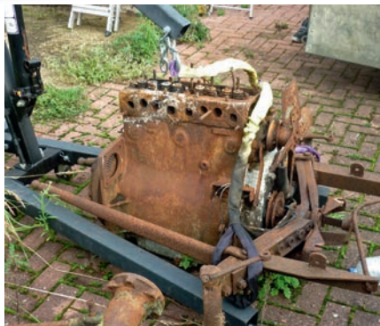
The cylinder head was a real struggle to remove. The valves are all free in their guides, which means it will play another day.
