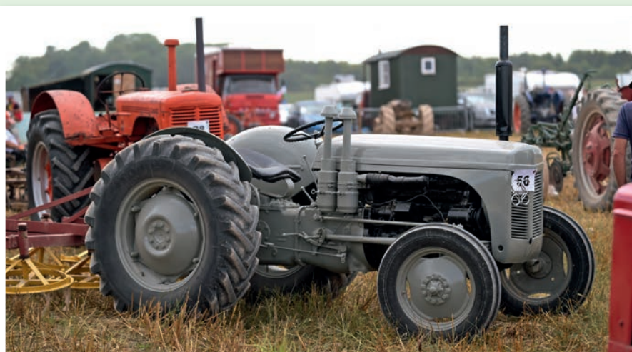
▲ You don't see too many MF 130s around, so it was good catch sight of Gary Cresswell's 1965 vineyard model that's powered by a Perkins P4 diesel engine.
