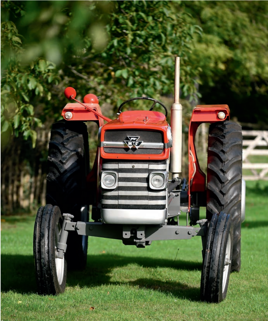
The headlights and their housings are original, although they're sitting on a new radiator grille assembly. For the future, Richard is considering having the exhaust sprayed white.
