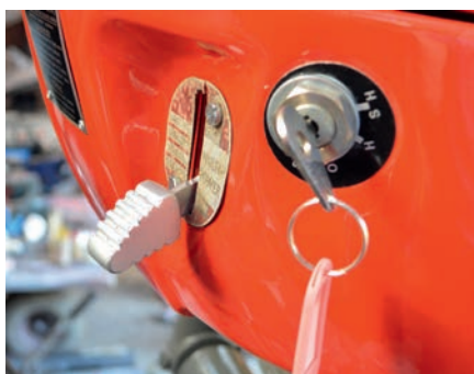
The lower part of the dash includes the ignition key switch, relocated due to the inclusion of the Multi-Power control lever, which occupies the key's normal place.
