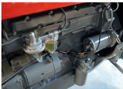
It's obvious from this photograph that the fuel lift pump, the dynamo and the wiring loom are new.
