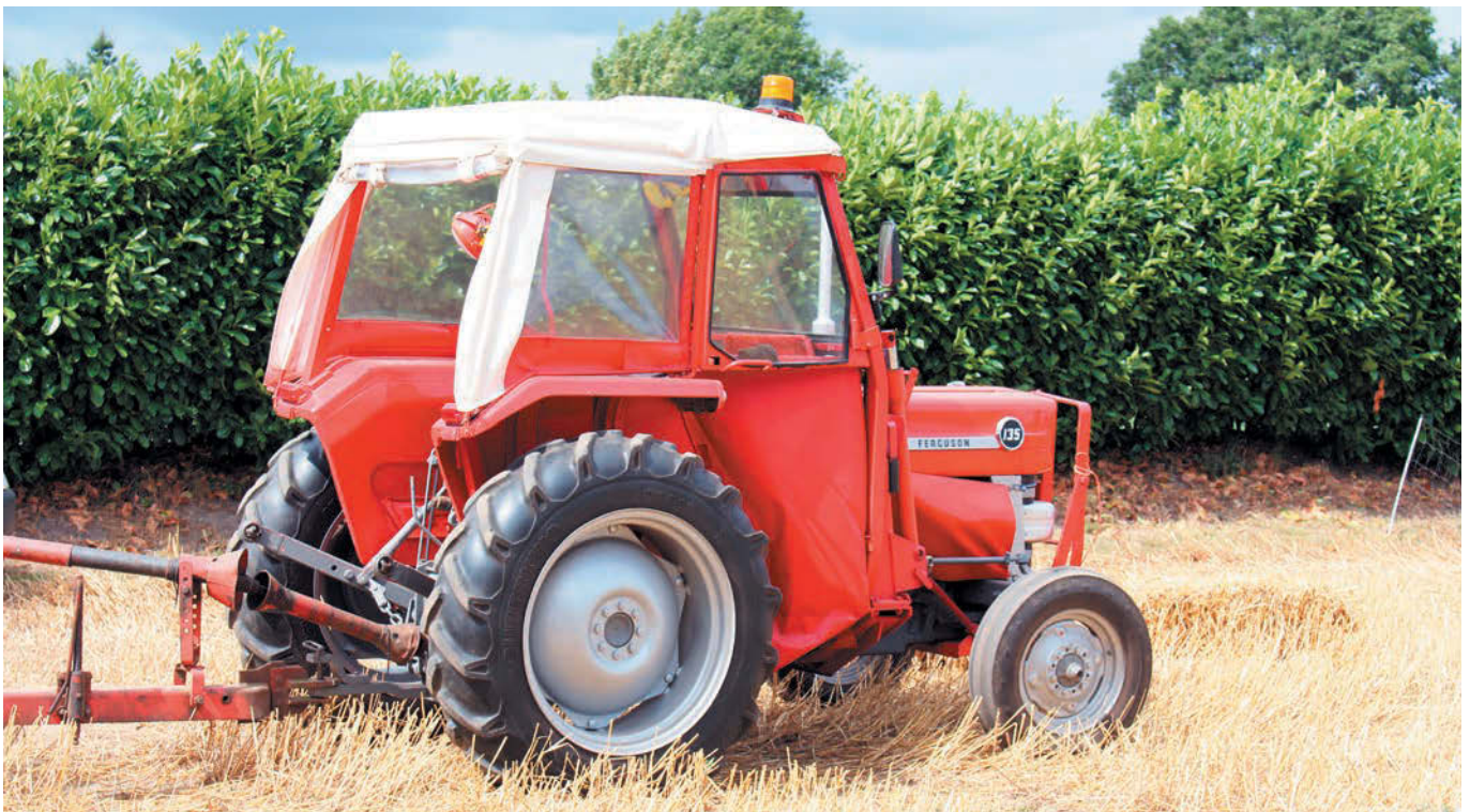
This rear view shows a common feature of most early safety cabs; the open rear. This was ideal for keeping an eye on the implement behind, but was chilly during cold weather. A fold-down clear sheet was provided, and can be seen rolled neatly at the rear of the cab roof. But once this got dirty, rearward visibility became more limited!
