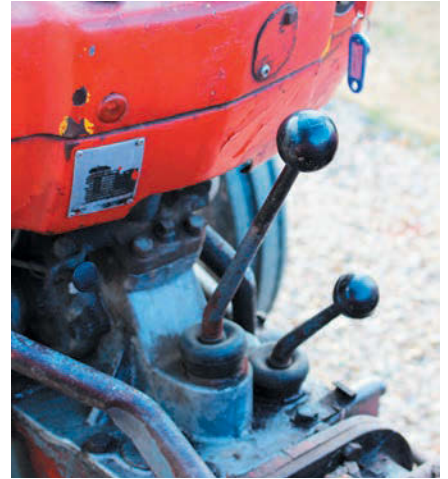
The transmission is easily controlled using these two gear levers, plus a switch on those tractors fitted with Multi-Power.
