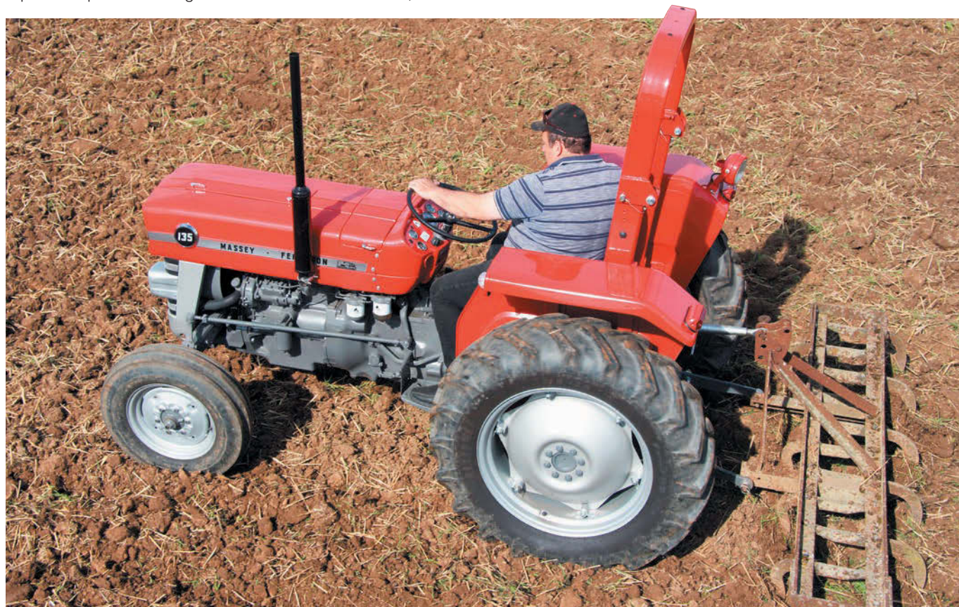
The simplest way to make a cabless 135 meet roll-over regulations was to fit an aftermarket roll-over bar, as here on this restored example seen cultivating in Lincolnshire.
