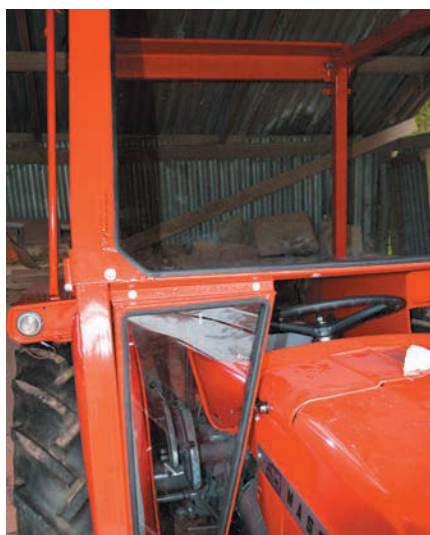
Here the screens are being fitted into the cab frame. They looked so much better with the new rubber seals fitted.
