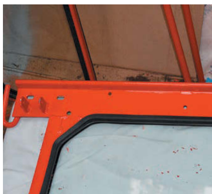
It took quite a bit of work to get the screen looking right. Here I'm refitting the glass, complete with new rubber seals.
