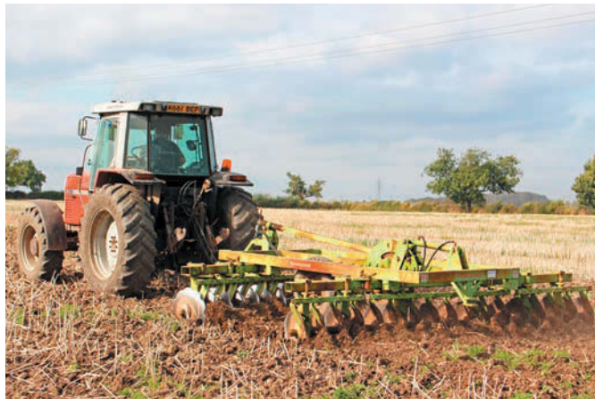
A heavy set of Dowdeswell disc harrows cause no problems for the 126hp 3125, which showed superb traction for its size, even during its second decade of use.
