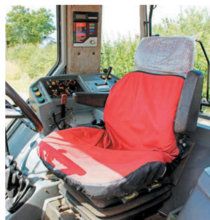
The interior of this 3115 is typical of what greeted the 3000, 3100 and 3600 Series driver. Cab interior was spacious, light and airy. The controls were easy to use and, on top-spec models, the Dataronic terminal was mounted on the right-hand side cab pillar.
