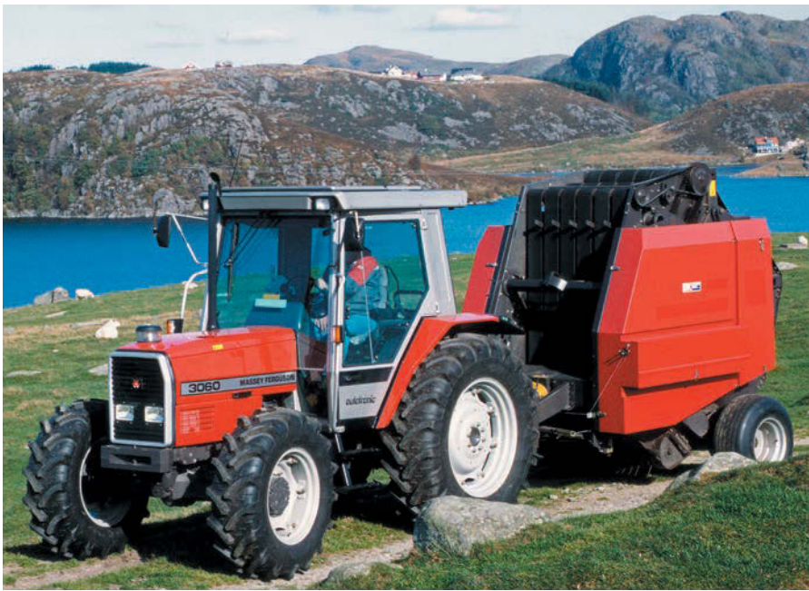
The 3060 was an original model of the 3000 Series launched in 1986, and was rated at 77hp. This is a later example, as it has the centrally-mounted 'MF' badge on the radiator grille. The 3060 was a popular model, but struggled to represent MF in the 80hp bracket, so was later joined by the 85hp 3065 (Pic: AGCO)
