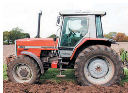
The 3125, with a Perkins 126hp engine, was the largest model in the 3100 range, but was still lighter than the 3610 that it and the 3115 effectively replaced
