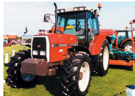
The look of the new order in 1995, when the 3000 family was entirely replaced by the new 6100 and 8100 models. Note the new cab design and new bonnets with larger radiator surround on this 100hp 6160.
