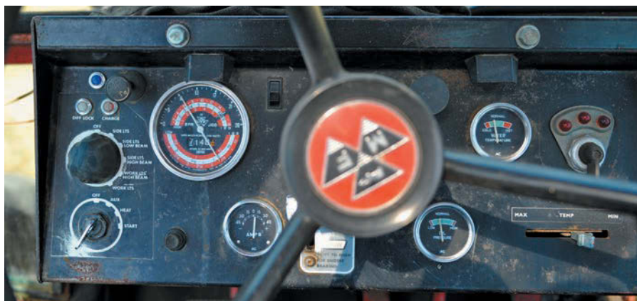
A well-equipped dash offered the MF 1200 driver plenty of information, apart from fuel level. However, a simple sight glass was provided elsewhere in the cab.
