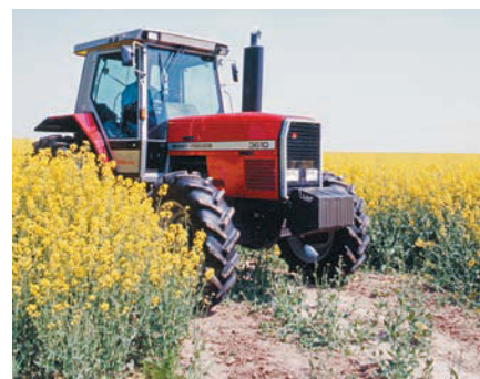
With 113hp under its large bonnet, the 3610 was the smallest of the original 3600 Series line-up, but proved unpopular due to its large size and weight combined with a modest power output. It was the first of the new models to be dropped. (Pic: AGCO)
