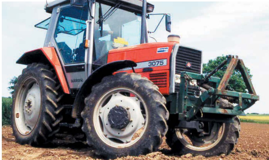
The last of the all-new 3000 family models was the turbocharged 3075; an excellent machine offering lots of power in a lightweight chassis. It also benefitted from the option of the Dynashift semi-powershift transmission.
