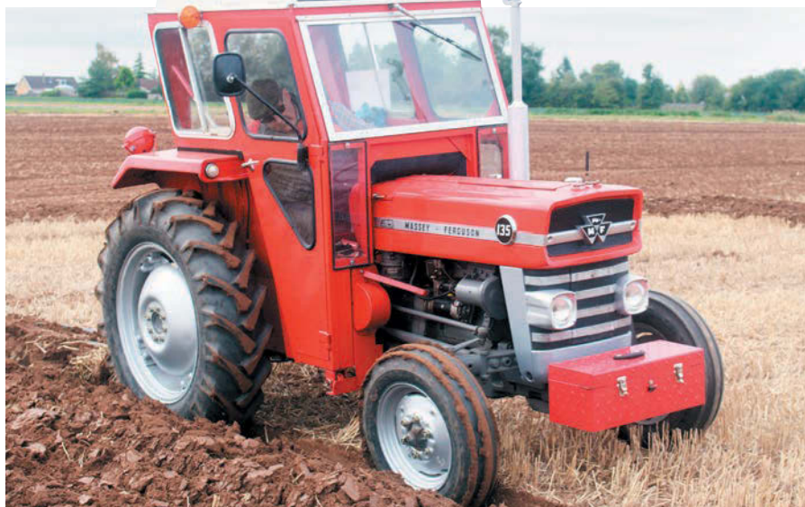
This Duncan cab not only met the safety cab legislation of the time, but also the later, 'quiet cab' requirements. It was a popular retro fit among budget-conscious farmers.
