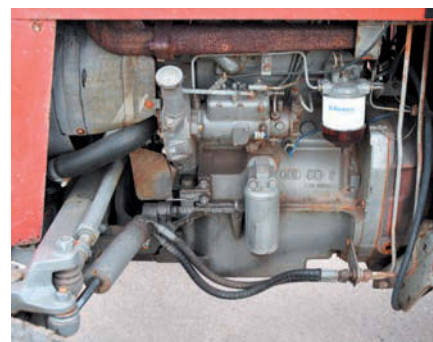
The Perkins AD3.152 that powers this MF 550 was a popular and reliable engine.
