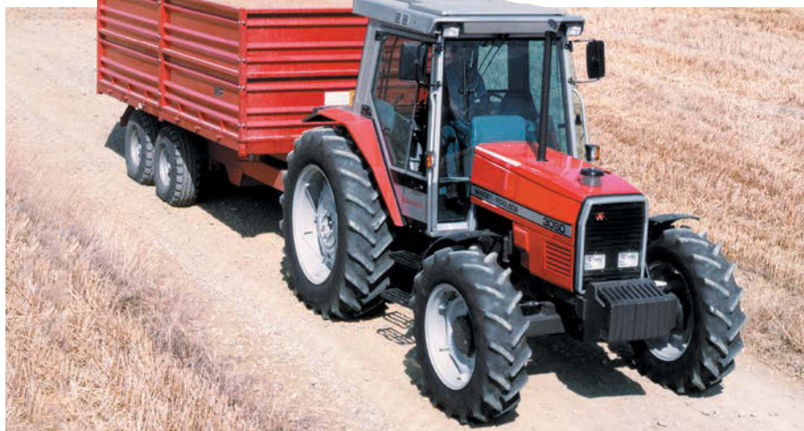
Top model in the original 3000 Series of 1986 was the 107hp 3090, which took power levels beyond the 600 Series that these tractors replaced (Pic: AGCO)
