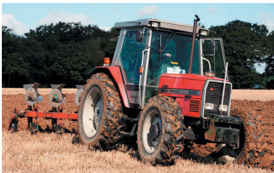
The 3080, with its 100hp six-cylinder Perkins engine, was a very popular model in the original range, and sold extremely well (Pic: Kim Parks)
