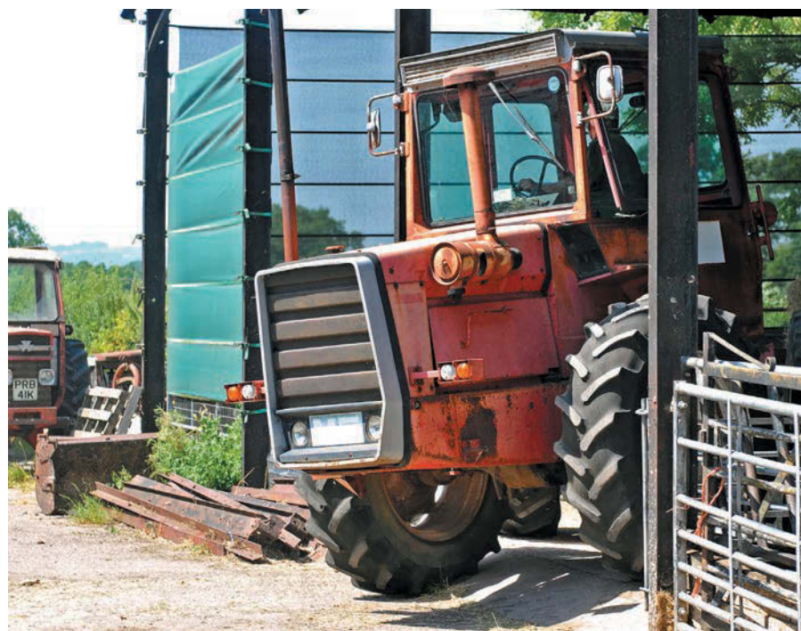
Storing an MF 1200 requires plenty of space, but the tractor's articulated layout makes it easier to back into spaces than you might imagine.
