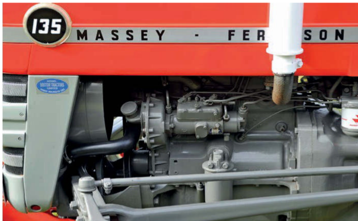
This is the extremely reliable, 45.5hp, Perkins AD3-152, 2.5-litre, three-cylinder, diesel engine that powered most MF135s. A petrol-powered model was available with an engine provided by the Standard Motor Company, but most of these went for export.
