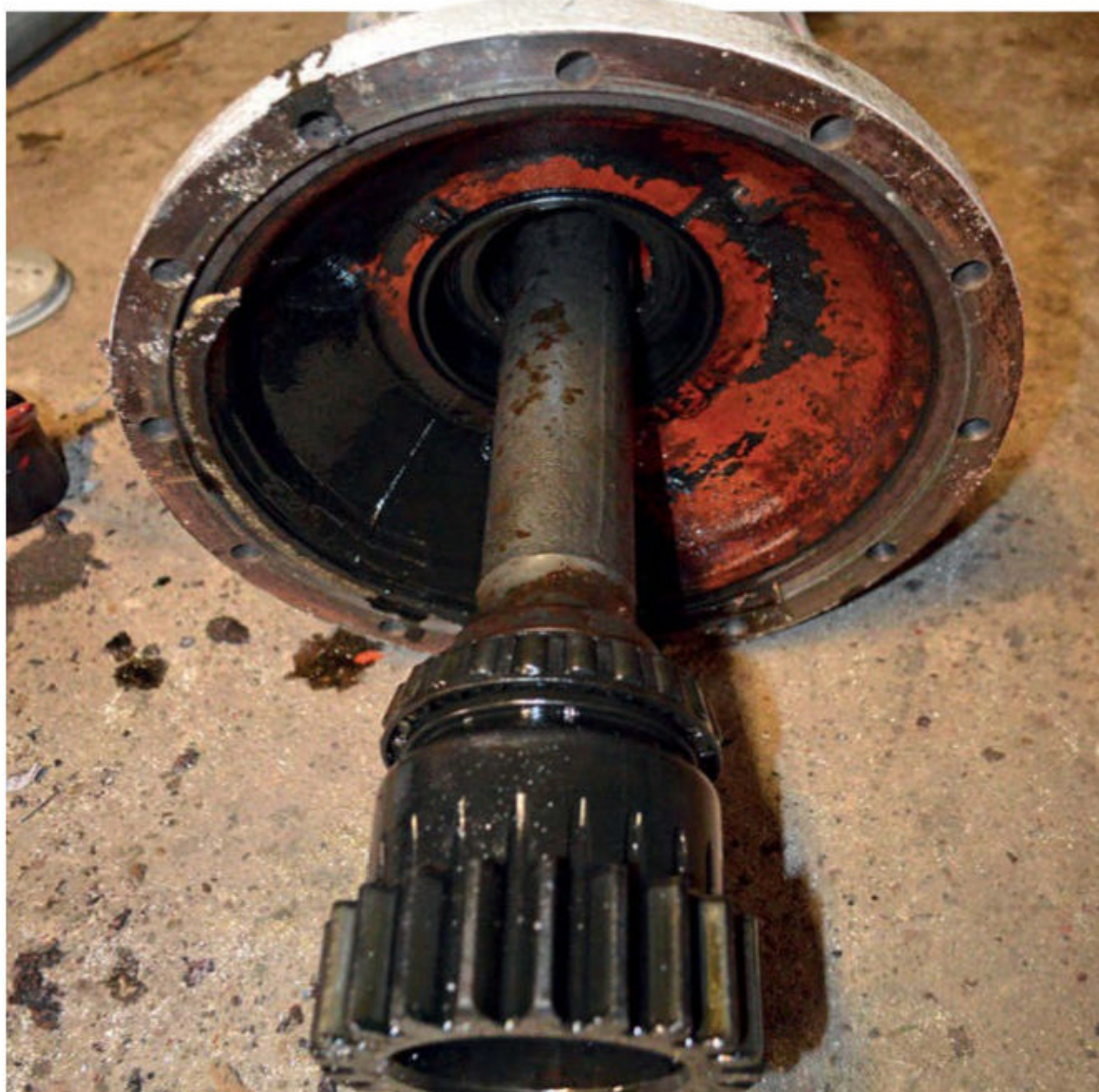
... after which the reduction hub could be removed, allowing me to slide out the half-shaft.
