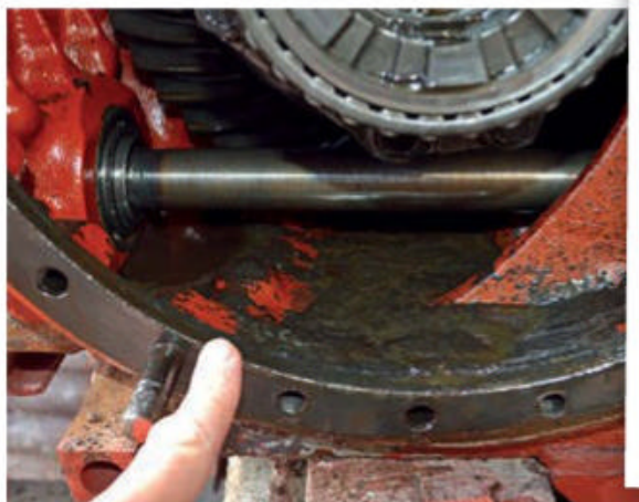
While the axle was off, I took the opportunity to remove all the accumulated sludge from the back-end of the tractor.
