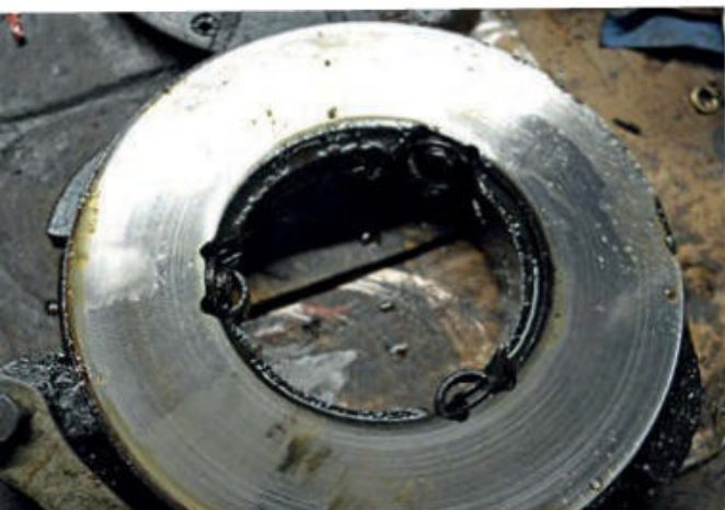
Sandwiched between the discs is this actuator that, when pulled, pushes the discs against the plates.
