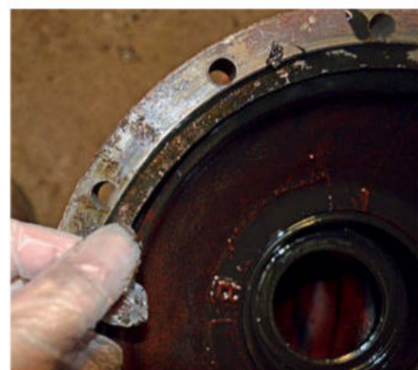
Careful and thorough cleaning is required around this edge, to ensure that the cork gasket seals properly.
