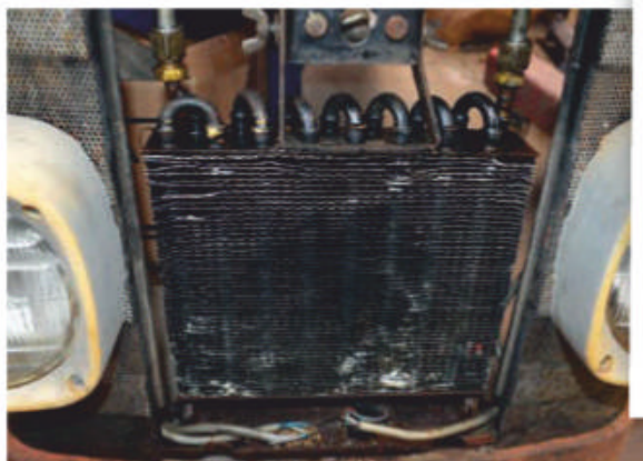
With the tractor back in the workshop, the first job was to remove the bonnet. This oil cooler is fitted behind the front grille, on Multi-Power models.
