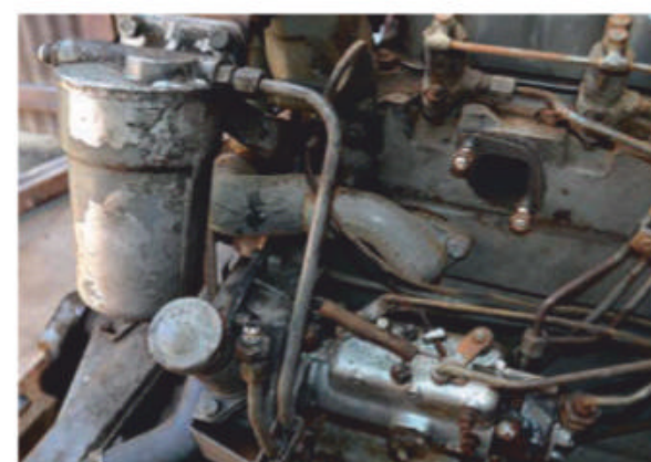
Another Multi-Power feature is this oil filter that's linked to the oil cooler, a new filter was on the list of things to replace.
