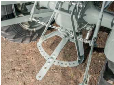
This early style drawbar is an alternative to the nine-hole drawbar.
