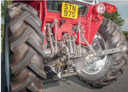
The improved hydraulic system gave a maximum lift capacity of 3120lb (1415kg).
