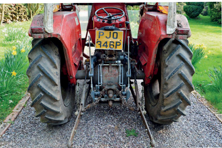
The rear of the tractor was pretty standard; Alan had bought the new pick up system, which is in the lighter grey colour.
