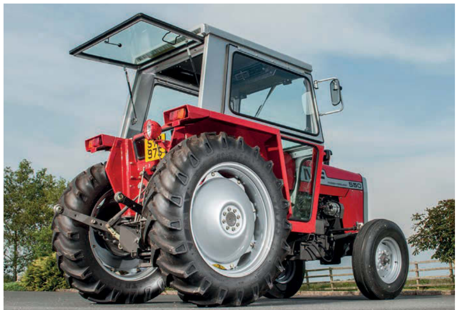
The opening rear window was a big improvement over the roll-up flexible arrangement on the 100 series cabs.
