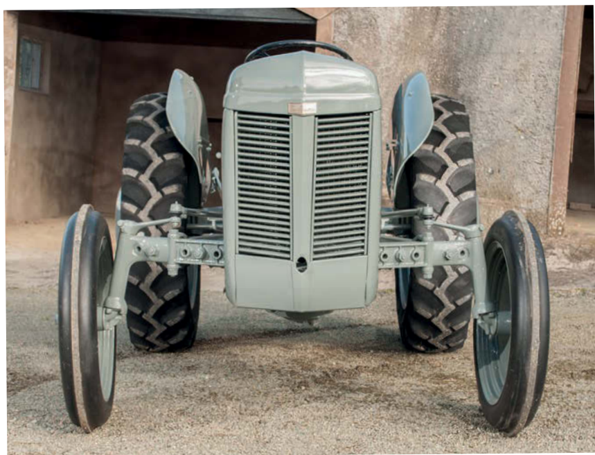
Raymond has set the wheel track to 48in, as it would have been when it left the factory.
