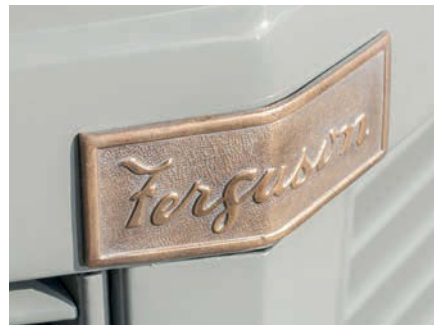
Brass grille badges were fitted to TE 20s during the early period of production.
