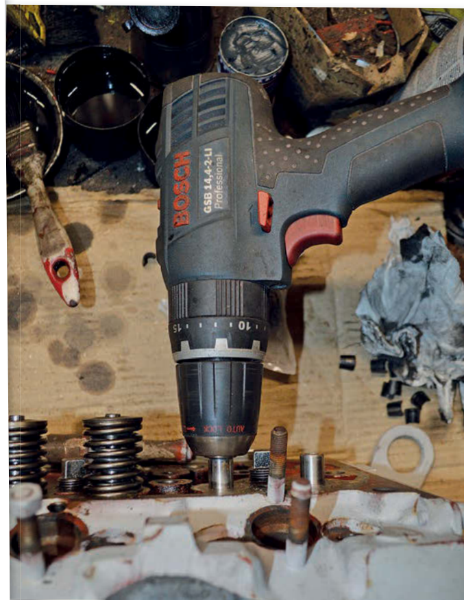
I keep this 14-volt cordless drill purely to grind in valves; the motor isn't powerful enough to drill a hole but is perfect for doing this job.
