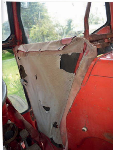
The interior of the cab featured the soundproof cladding, which meant the doors were double lined with foam padding in between.
