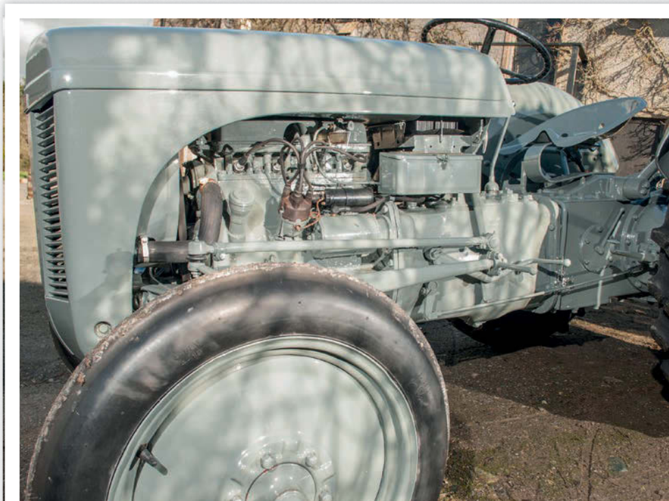
The Continental Z120 engine had an 81mm bore, very similar to the Standard engine in the TEA 20.
