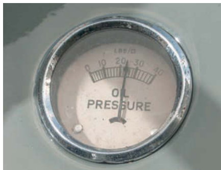
The engine has a healthy oil pressure, as shown on the original 40 psi gauge.
