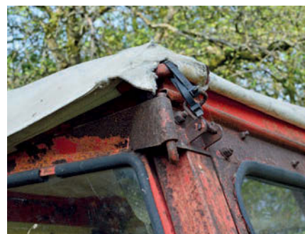
The other section of the roof was no better, as it was ripped in various sections and held on with cable ties.
