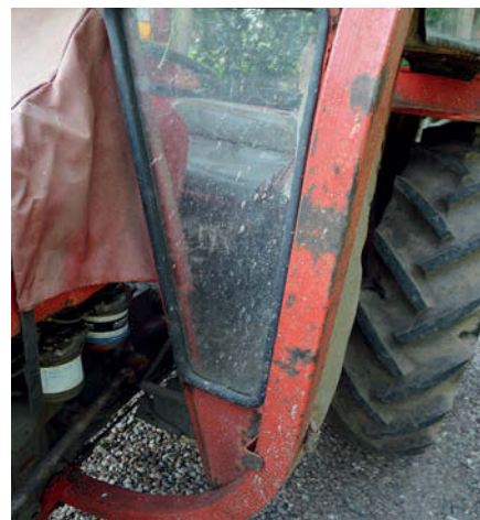
All of the glass in the cab would need removing to do the best possible restoration; I would probably replace the rubbers, which were perished.
