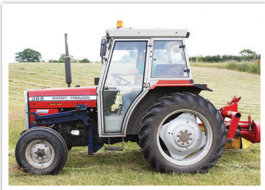
Plenty of glass in the cab: thin cab pillars and an exhaust stack mounted to the side of the engine provide excellent all-round visibility from the driver's seat.
