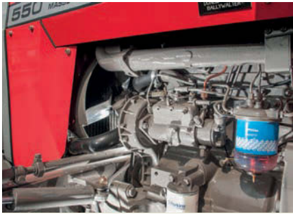
Inheriting the Perkins AD 152S engine from the MF 148, the MF 550 produced 47 DIN hp.
