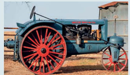
Showing the rowcrop design of the Wallis Cub, which was well advanced for the time.
