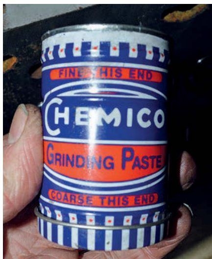
If you're overhauling a cylinder head then you'll need a tub of grinding paste like this; it has coarse at one end and fine at the other.
