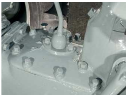
On later models the steering box was held down by studs and nuts.
