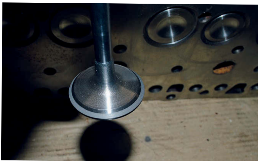
The drill gets the valves into perfect condition; it didn't have to work hard as they were new.
