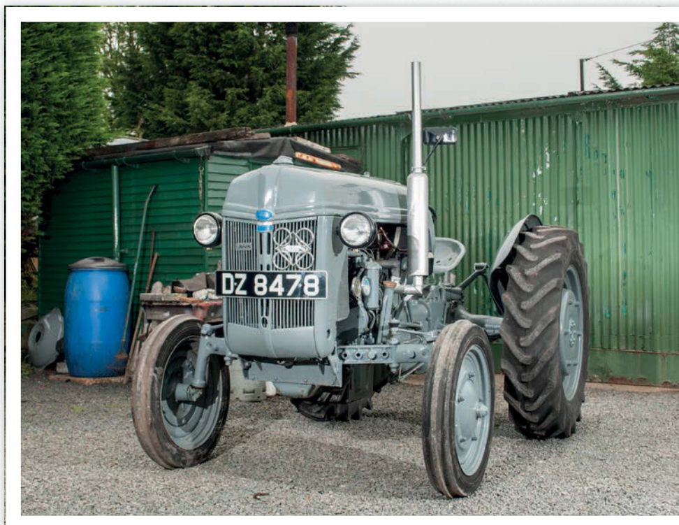
Wartime austerity meant that DZ 8478 left Dearborn with a magneto, a starting handle and no lighting kit.
