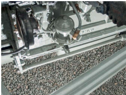
Original strengthening rods from a Z120 add support to the BMC pressed sump.
