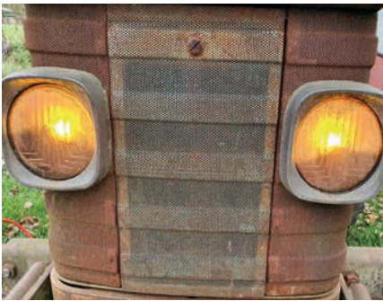
A replacement grill has been purchased from a donor tractor that was imported and broken for parts.
