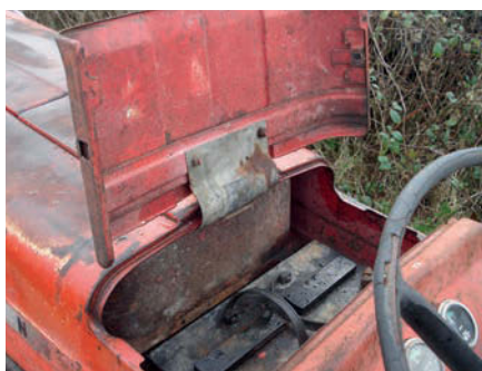
The battery compartment is fitted with a hinged cover, like an early Coventry made MF 135.
