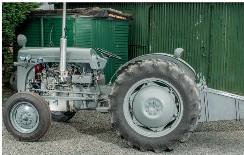
Ferguson dealer approved P3 conversion gave many petrol and TVO models a new lease of life in the 1950s.
