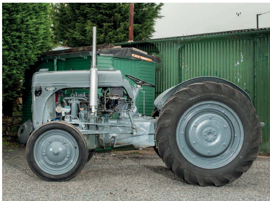
The distinctive raised bonnet line creates space for the Perkins diesel conversion.
