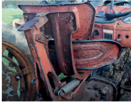
Although the suspension adjustment mechanism is not quite complete, I believe it is similar to items used on MF combines.
