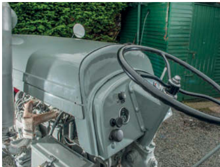
The bonnet riser was an essential component in the conversion kit.
