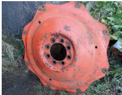
I initially bought row-crop wheels with David Brown centres thinking they would fit, but the stud hole size is different.
