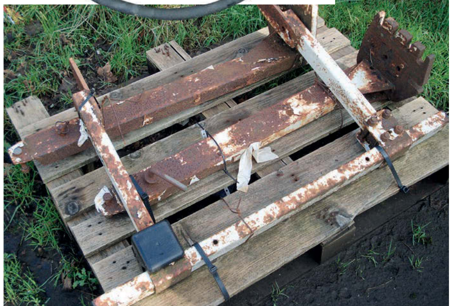
A roll frame has been purchased to fulfill the legal requirements for a working classic tractor.
