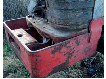
Once again, the weight frame looks like a standard item, but note the lugs to the rear.
