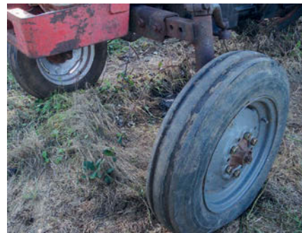
Here you can see the kingpin posts are substantially longer than a standard clearance model.
