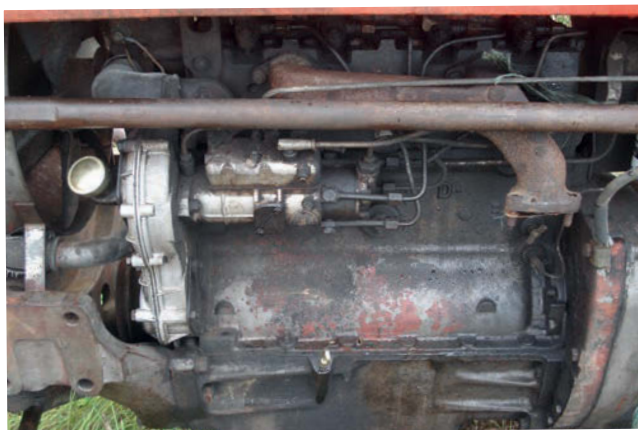
Fortunately, the Perkins AD4.203 engine was not seized, although it took some patience to bleed the injection system.
