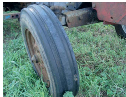
For comparison, the top of the kingpin post on a standard model is far below the level of the tyre.
