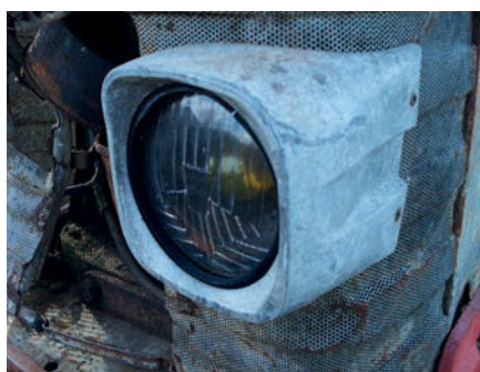
Alloy light cowls house larger diameter lights than the Coventry built equivalents.
