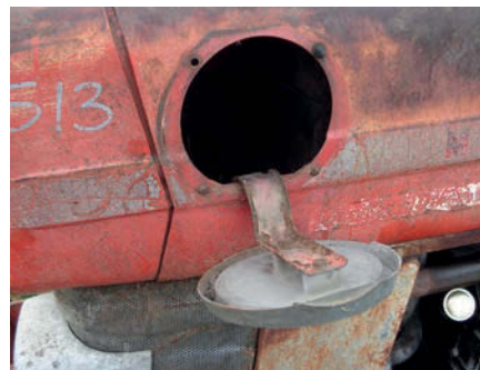
Strangely, a hinged down medallion is fitted as per much later models, with a dry air cleaner arrangement.
