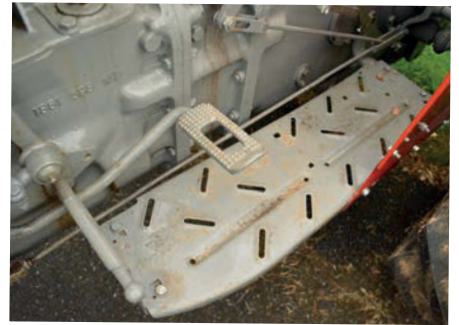
A longer gearbox calls for longer footplates; Alan commented on how much easier it is to get on and off the tractor because of this – and he's right.
