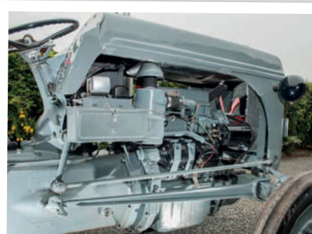
The fixing straps on the starter motor mark this out as an early Perkins P3 engine.
