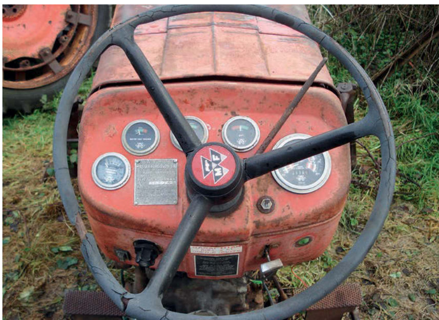
The dashboard on this early French built Mk1 MF 165 is more akin to that of a MF 130 than a UK built 165.
