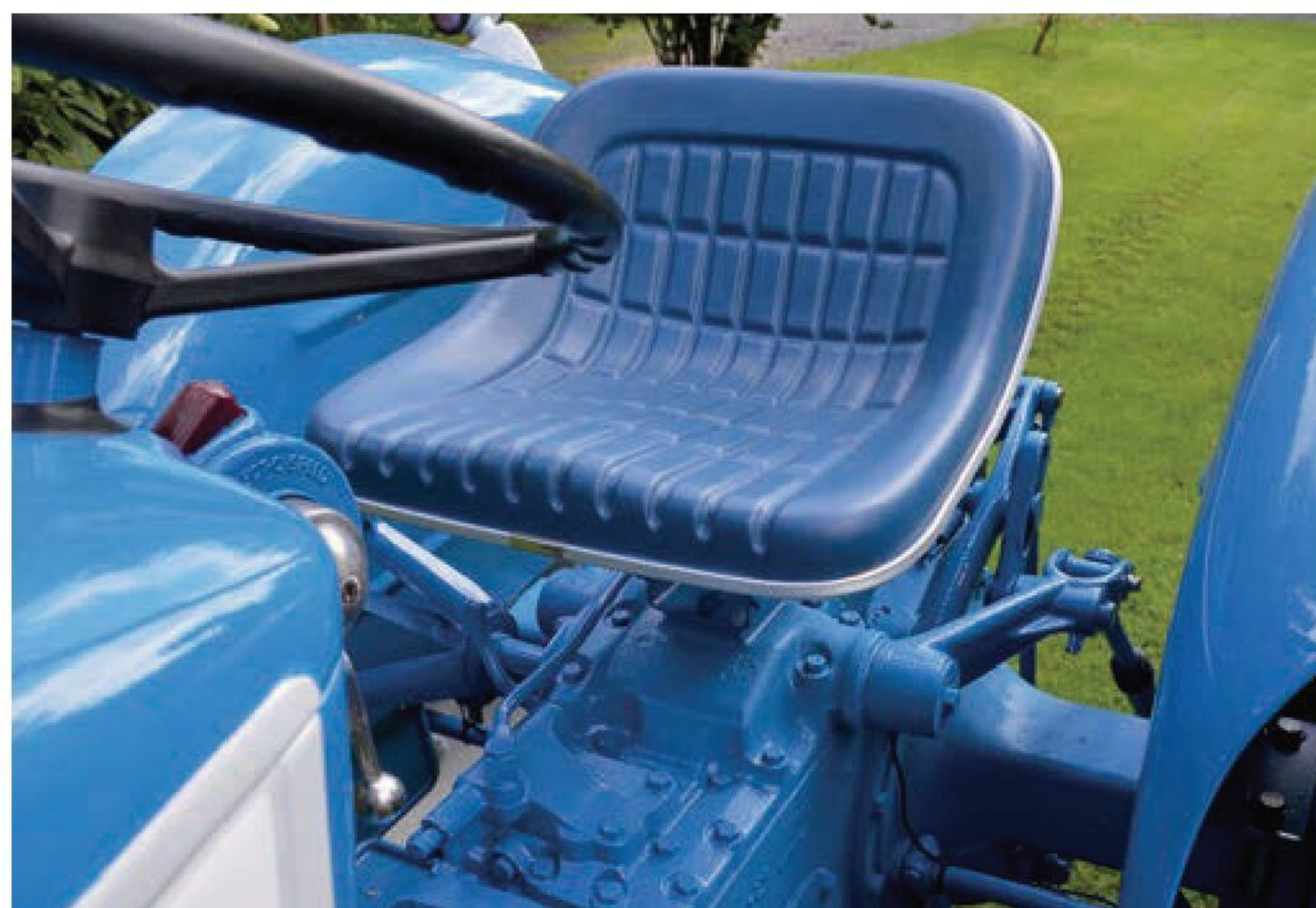
The plastic-covered Ford seat did tip slightly, but it was hard to sit on in comparison to the 165's so not as comfortable for prolonged periods of use. The design also allowed drivers to slide around more, which wasn't ideal.
