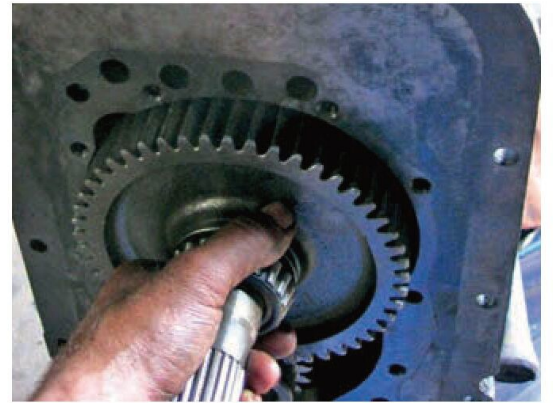
The reduction box output shaft is refitted, followed by the rear cover.
