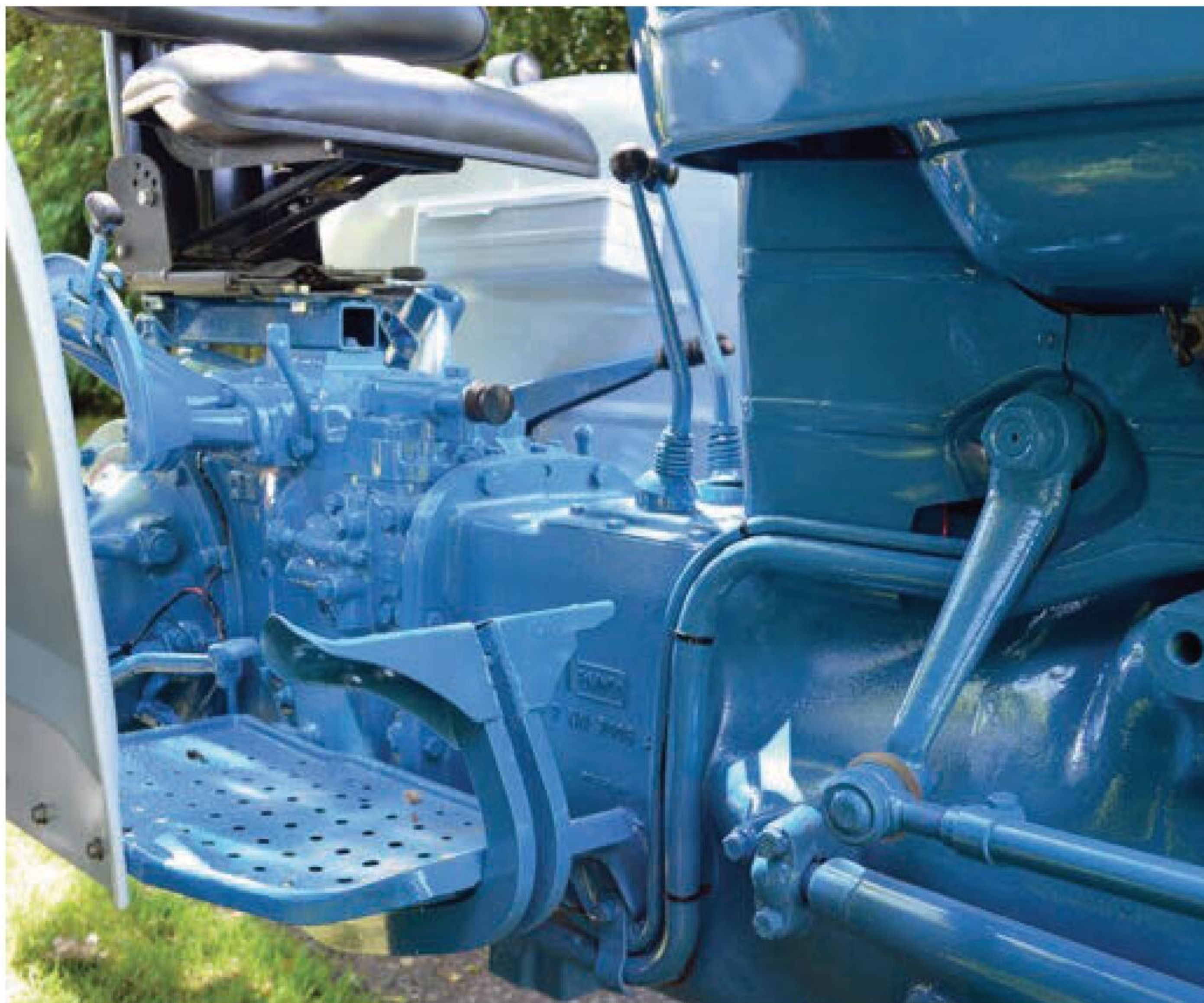
The repaired foot plates looked OK and, when located to the wings via the three bolts, made a sturdy place to step on to the tractor.
