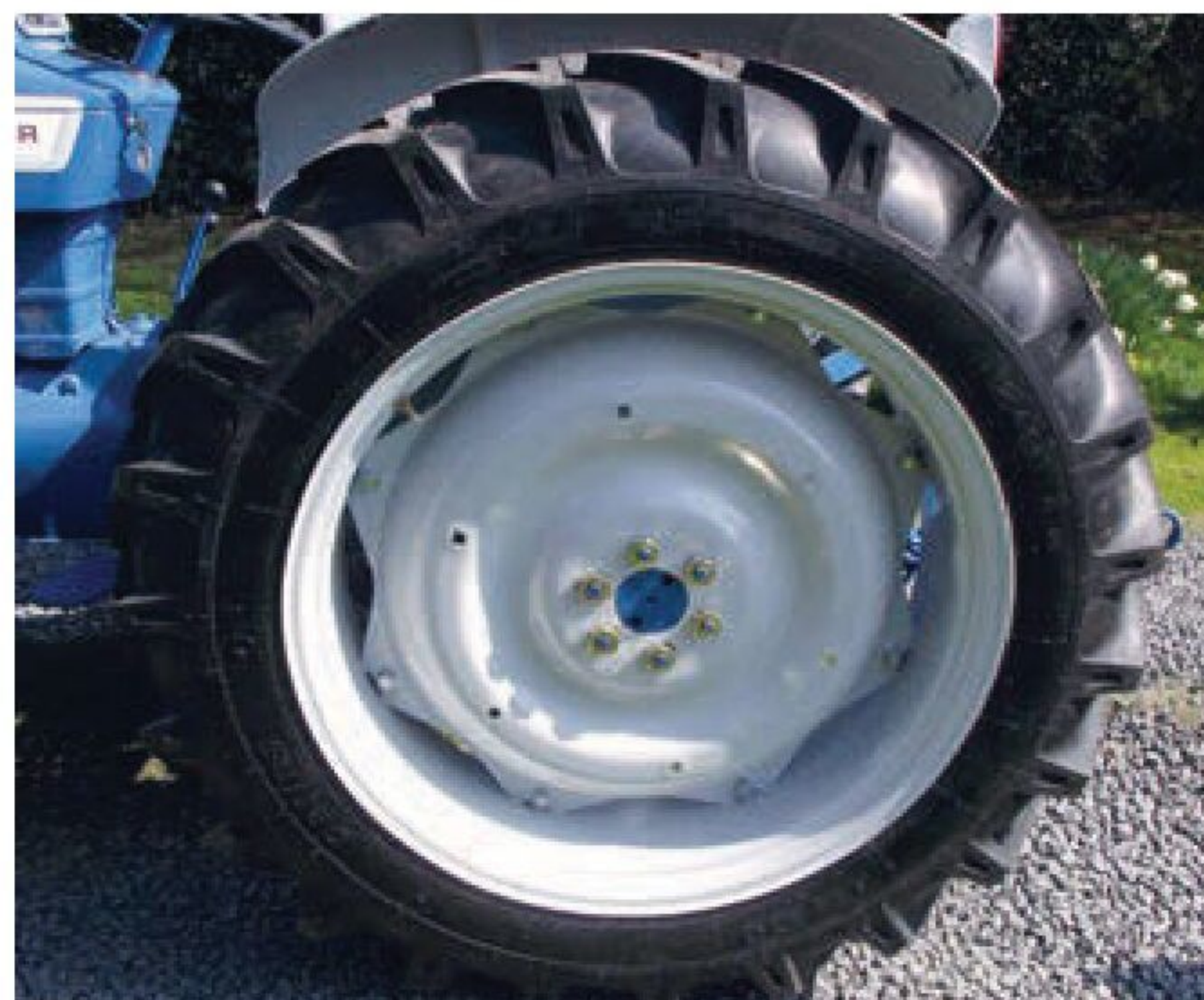
The Ford had one, solid centre dish; the rims were 36in, which were 4in larger than those on the 165.
