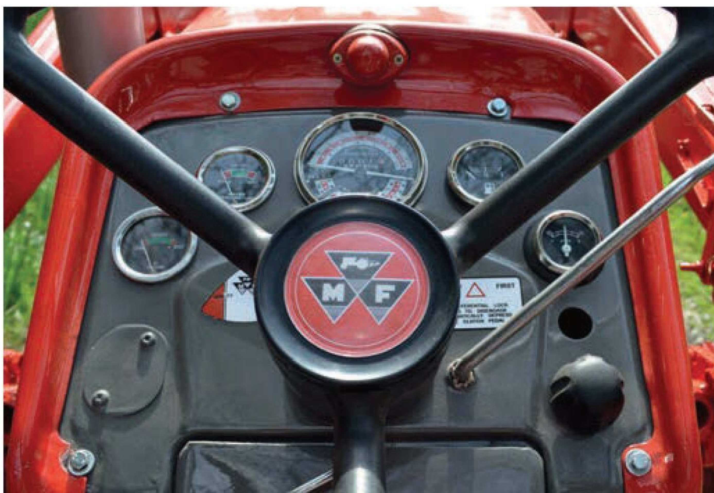
The Massey Ferguson 165 had a well-equipped dash featuring five useful gauges; tractormeter, fuel level, ammeter, water temperature and oil pressure.
