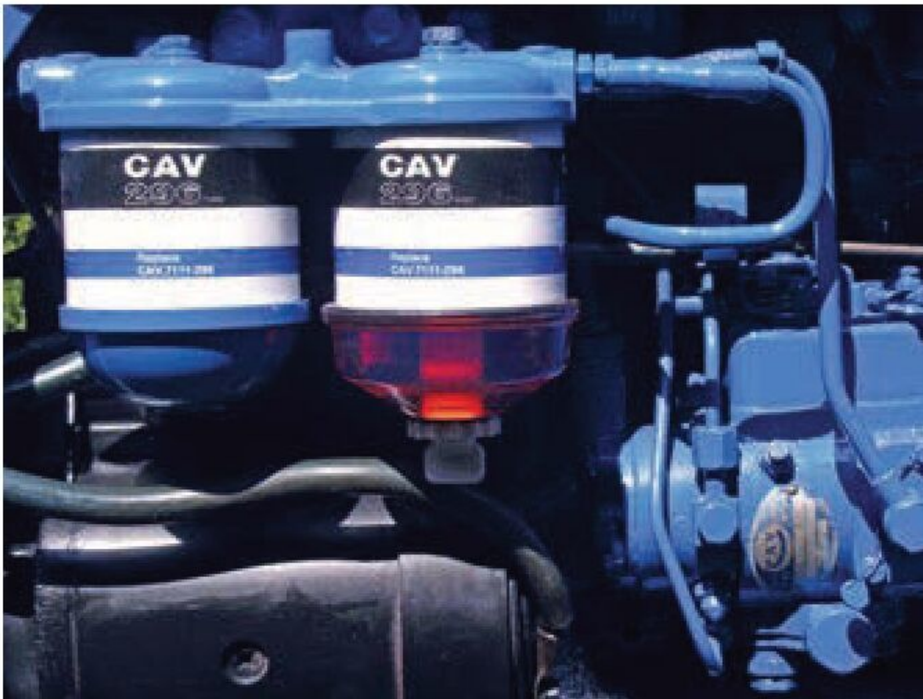
Trying to remove the starter motor on the Ford is a tricky job due to the close proximity of the double fuel filters and injector pump.
