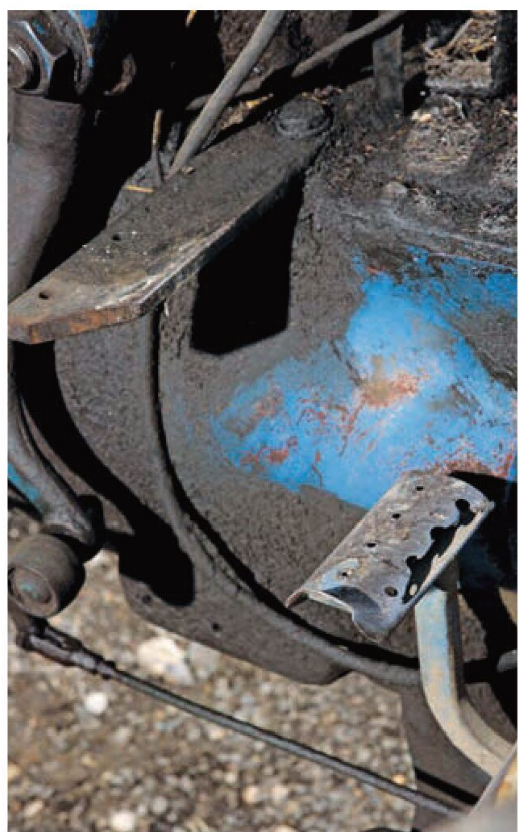
The Lambourn cab, which was on the tractor when new, was fitted to the angled plate just ahead of the gearbox, seen here.
