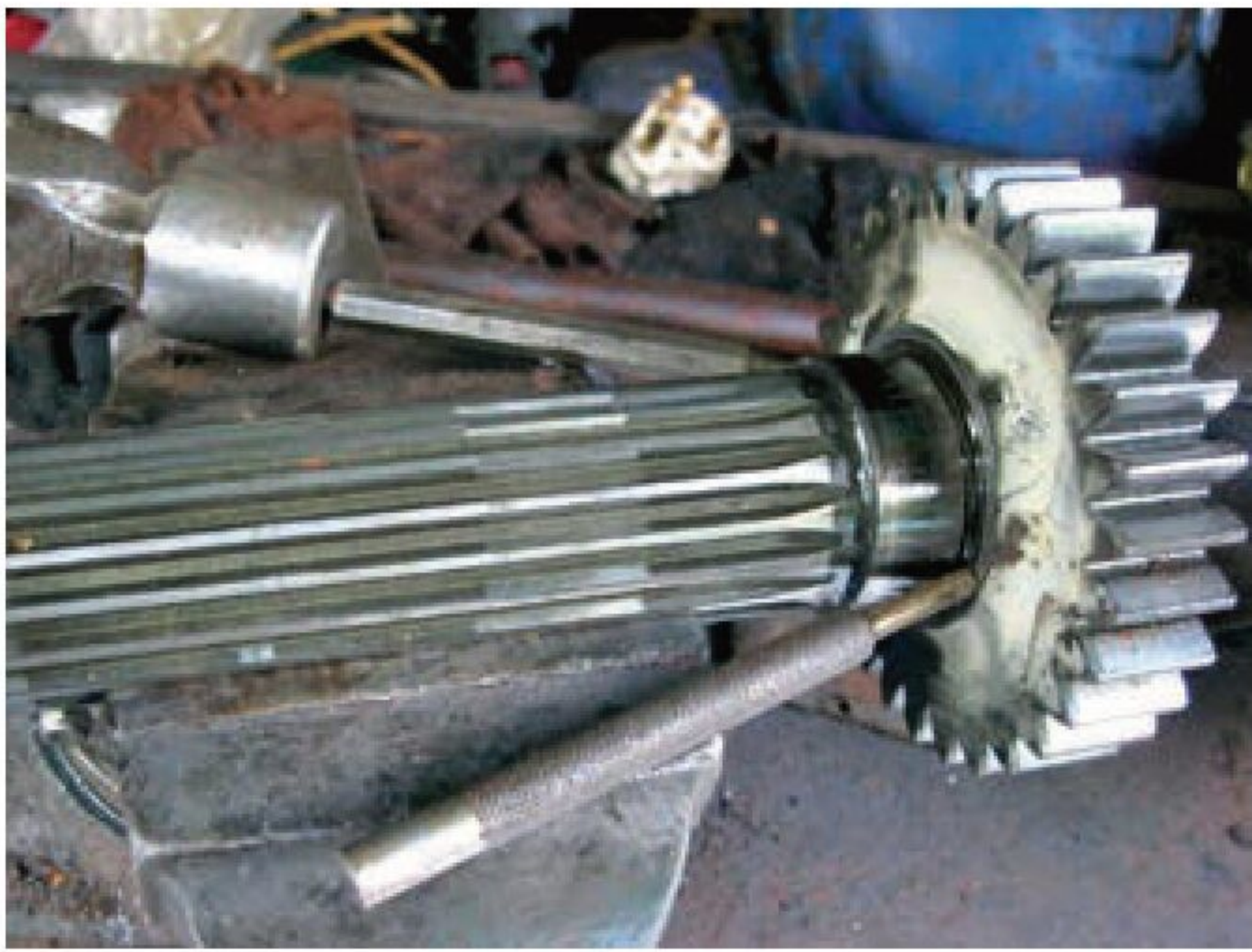
LEFT: Driving out the bearing cup from inside the end of the output shaft, with two punches.
