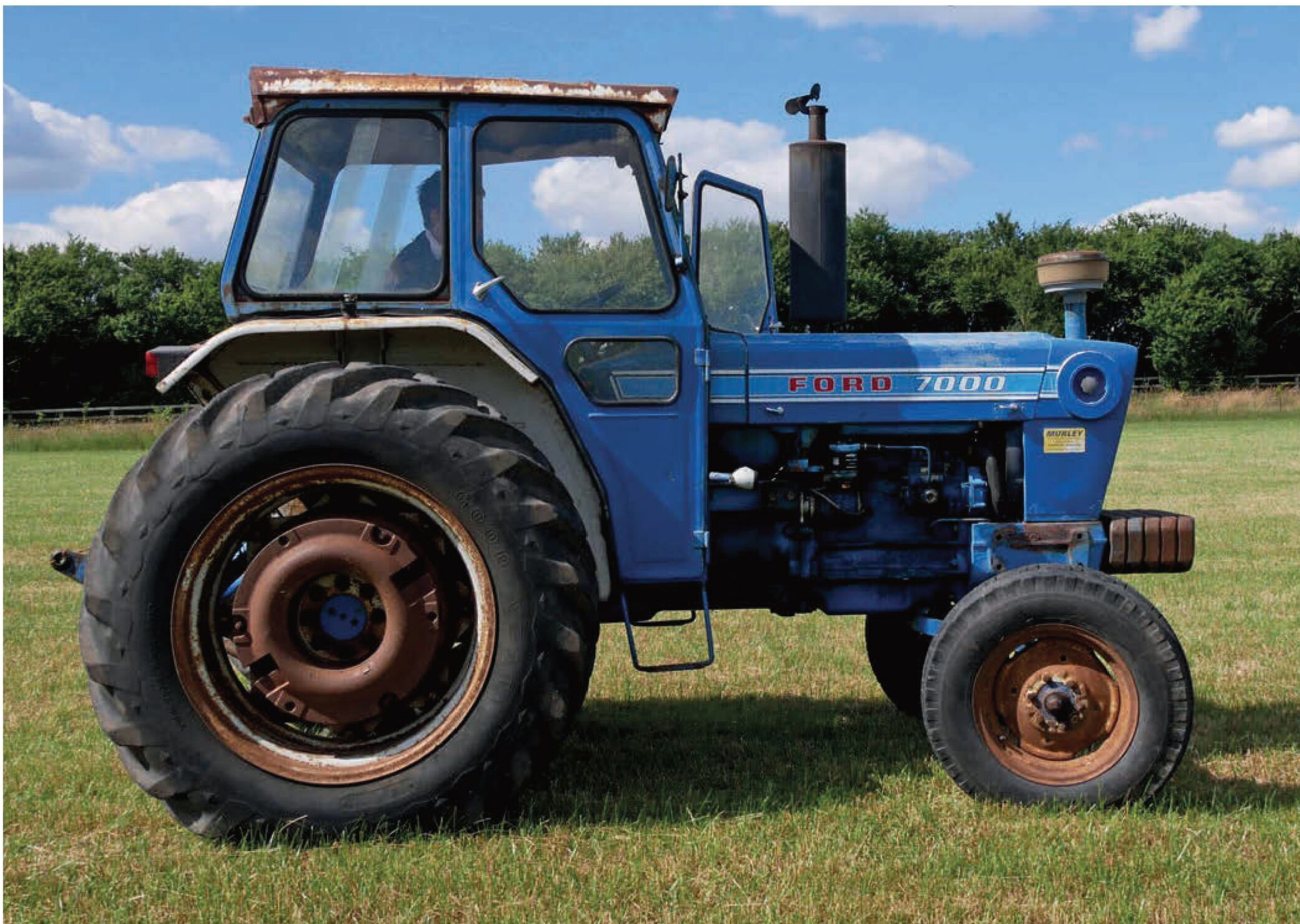
Steven Brooks' 1974 Ford 7000 is a completely original and standard, eight-speed tractor, with no optional extras. Being a short wheelbase tractor, it really needs a set of weights on the front for heavy fieldwork.
