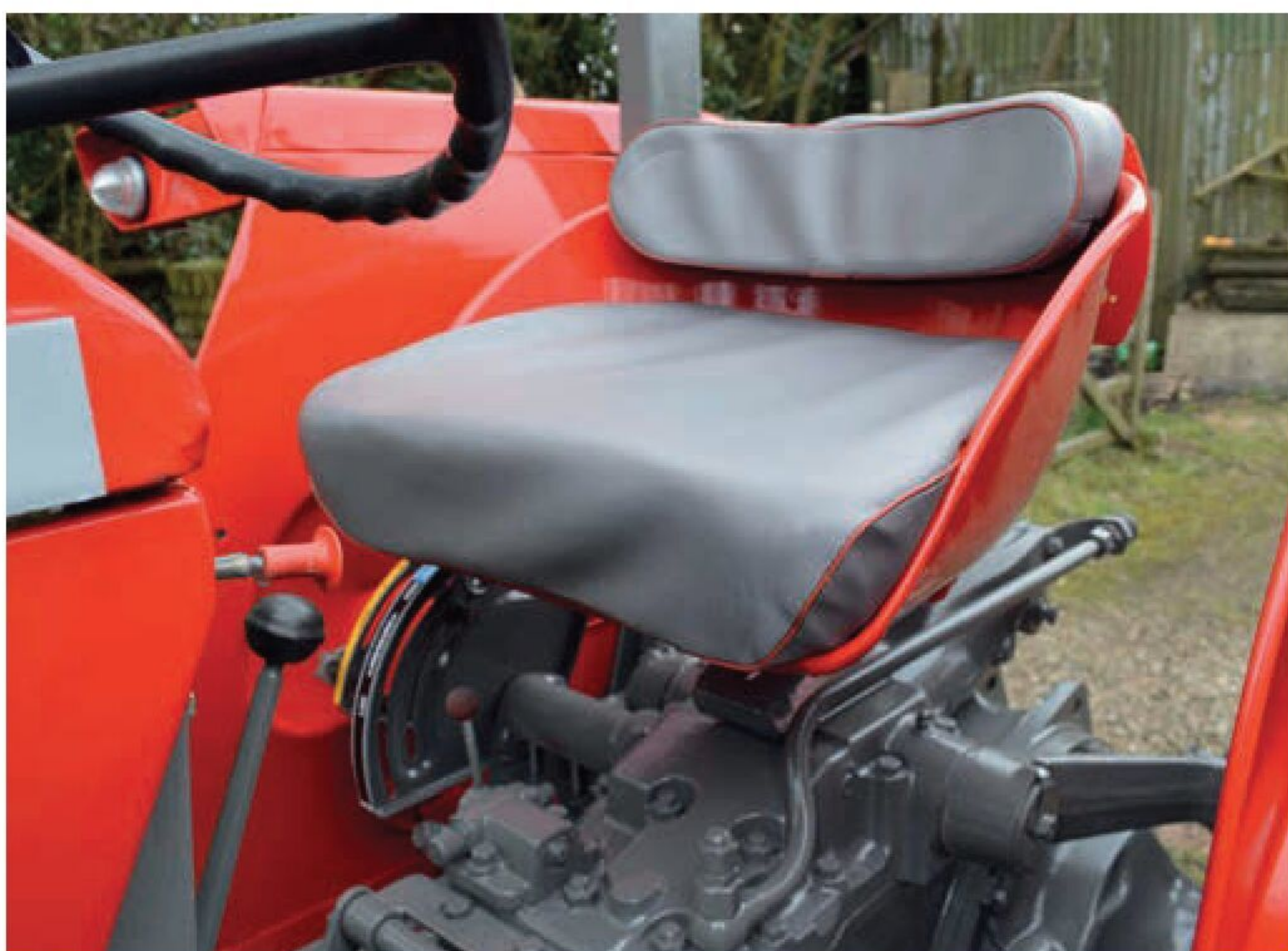
The Massey Ferguson's bucket seat could be tilted or tipped, and featured relatively comfortable cushion pads.
