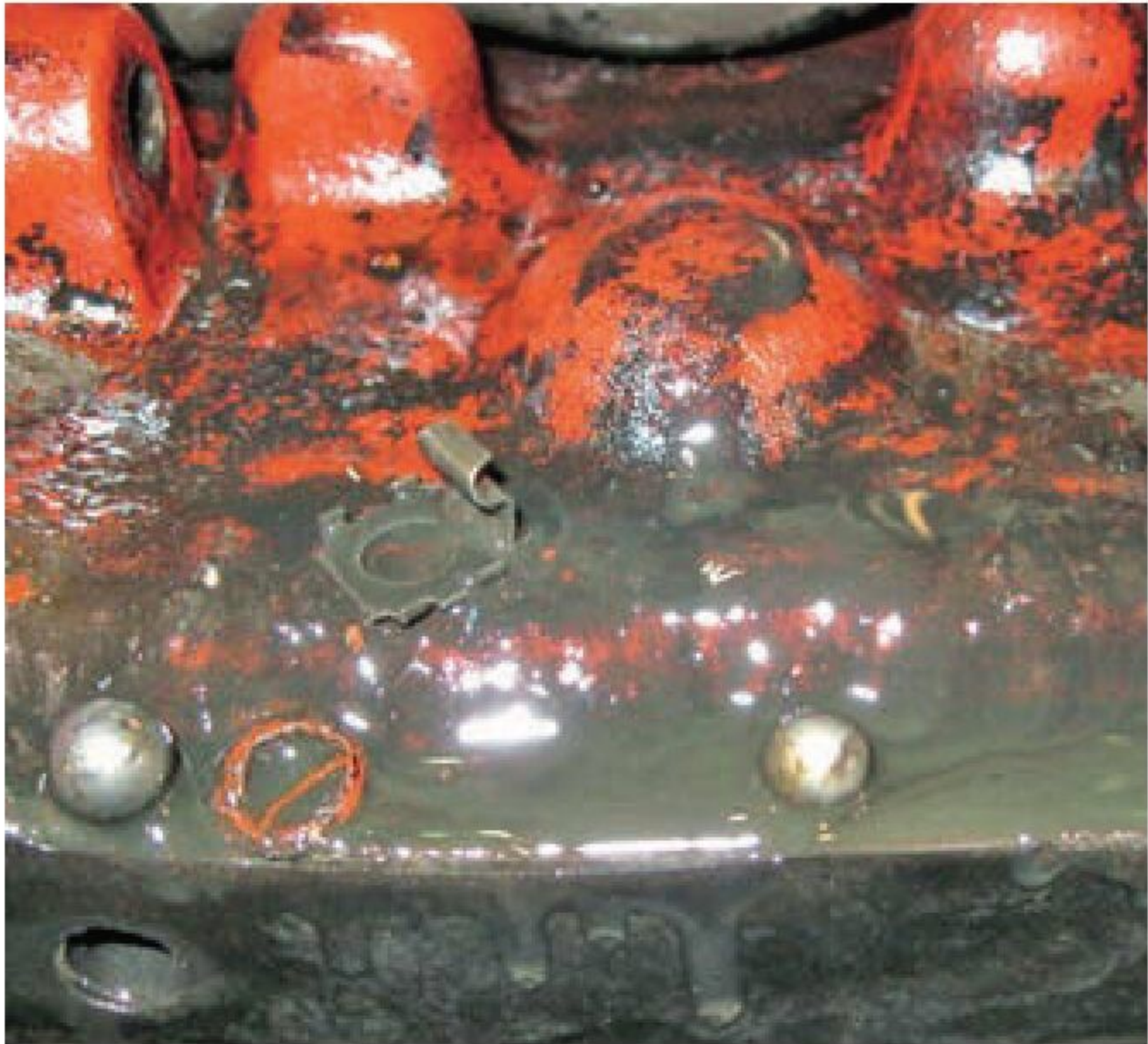
Two different-sized steel balls and the broken clip of a captive nut were found in the bottom of the differential casing, after splitting the gearbox off.
