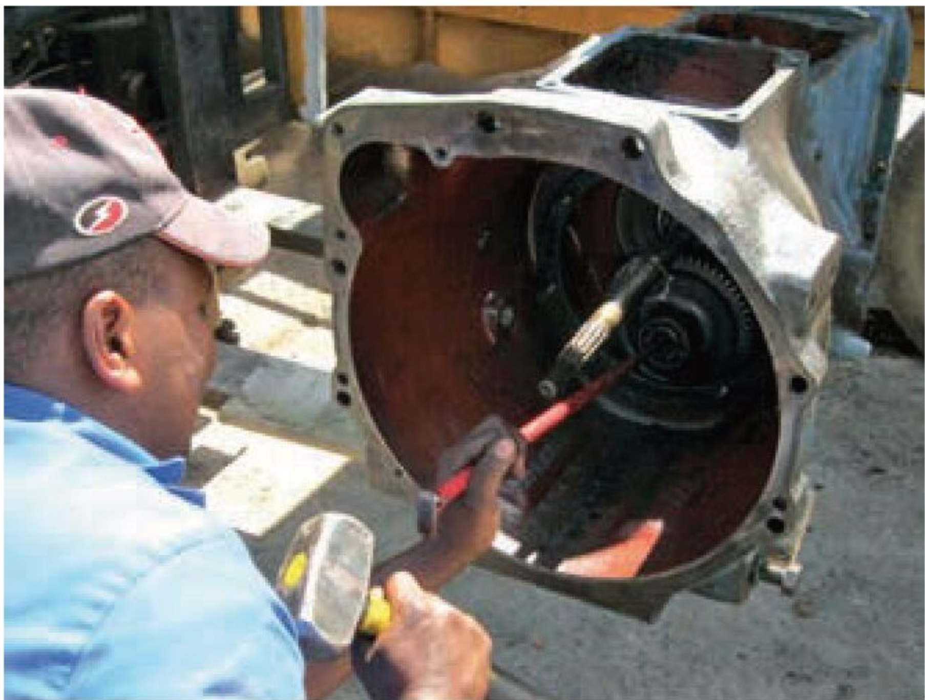
Driving the front PTO shaft out towards the rear, leaving the large input gear and bearing behind.
