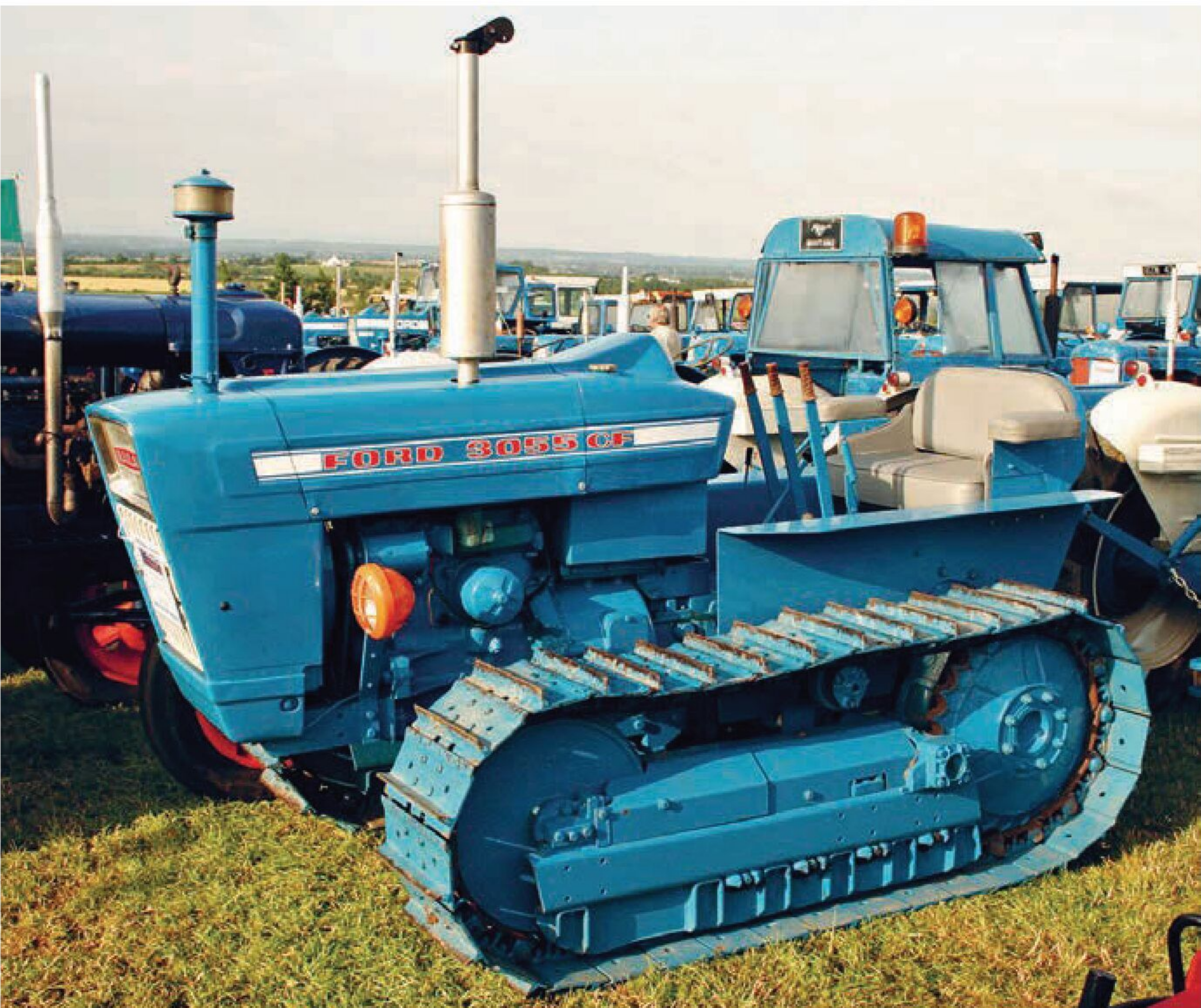
An unusual crawler conversion based on the 3000, by Mailam, from Italy.
