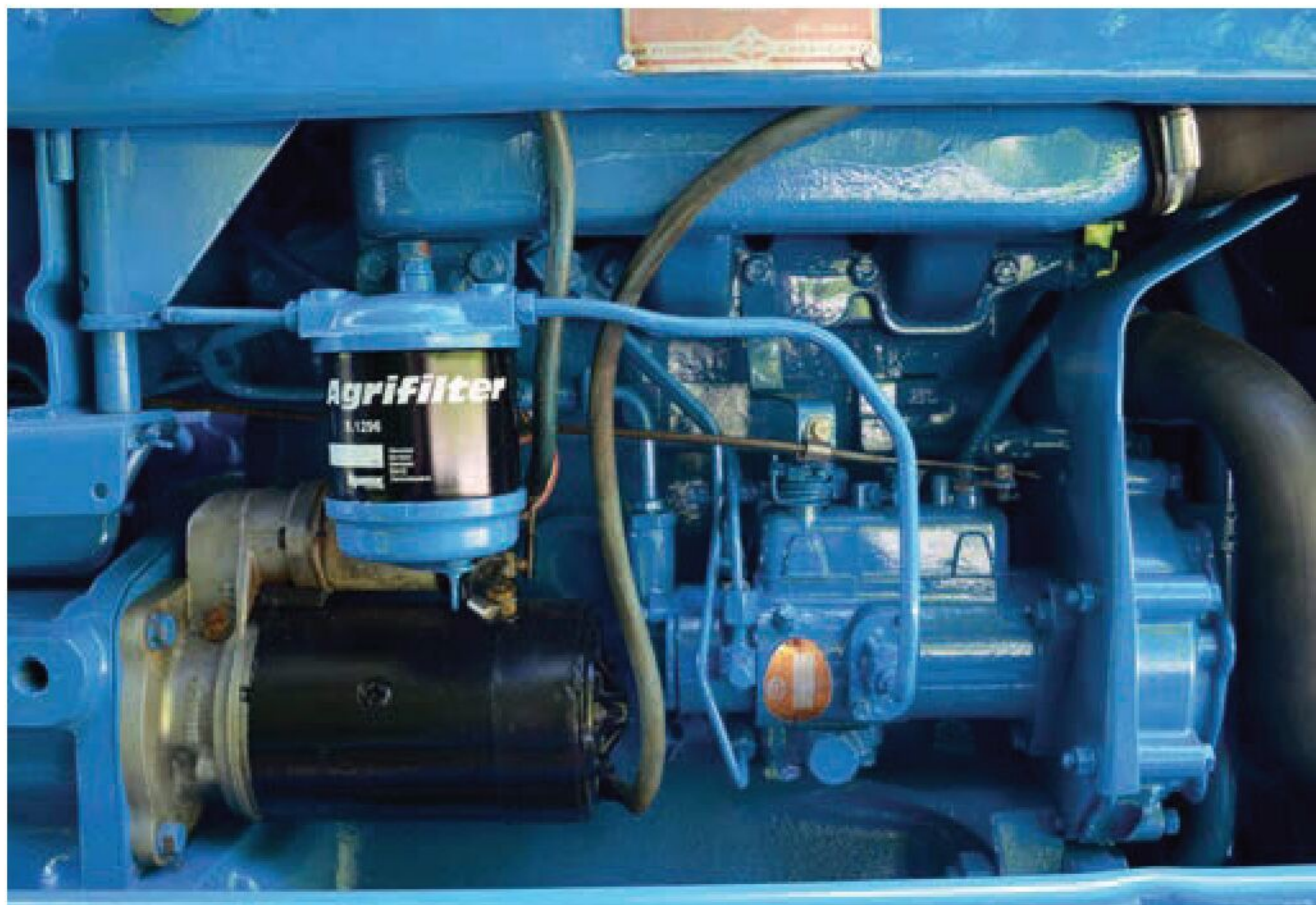
A CAV rotary pump replaced the Simms unit found on the early 3000s, and this one only had a single fuel filter.
