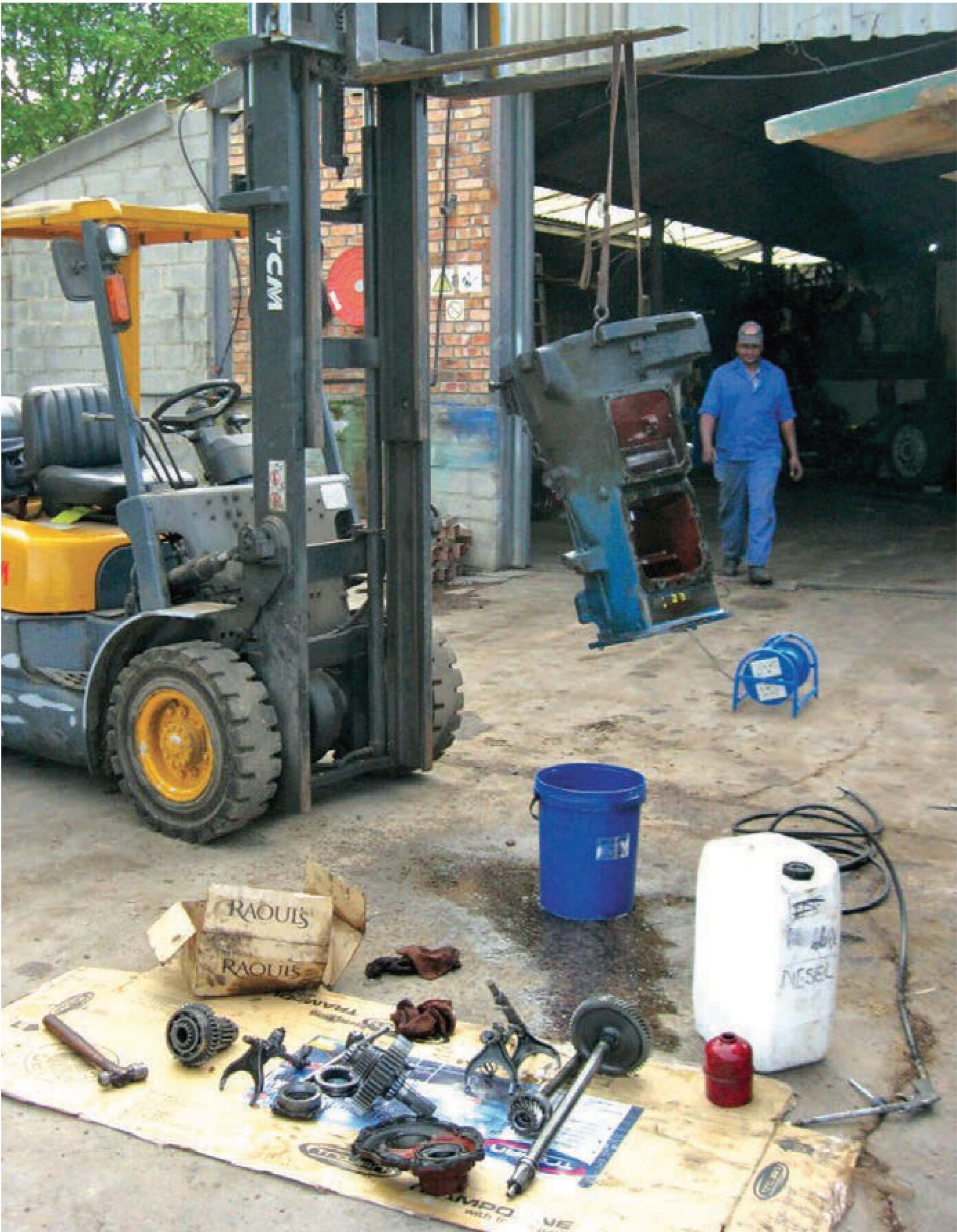
The whole gearbox is hanging from the forklift, with a bucket underneath to catch the remainder of the old oil and the paraffin we used to wash it out thoroughly.
