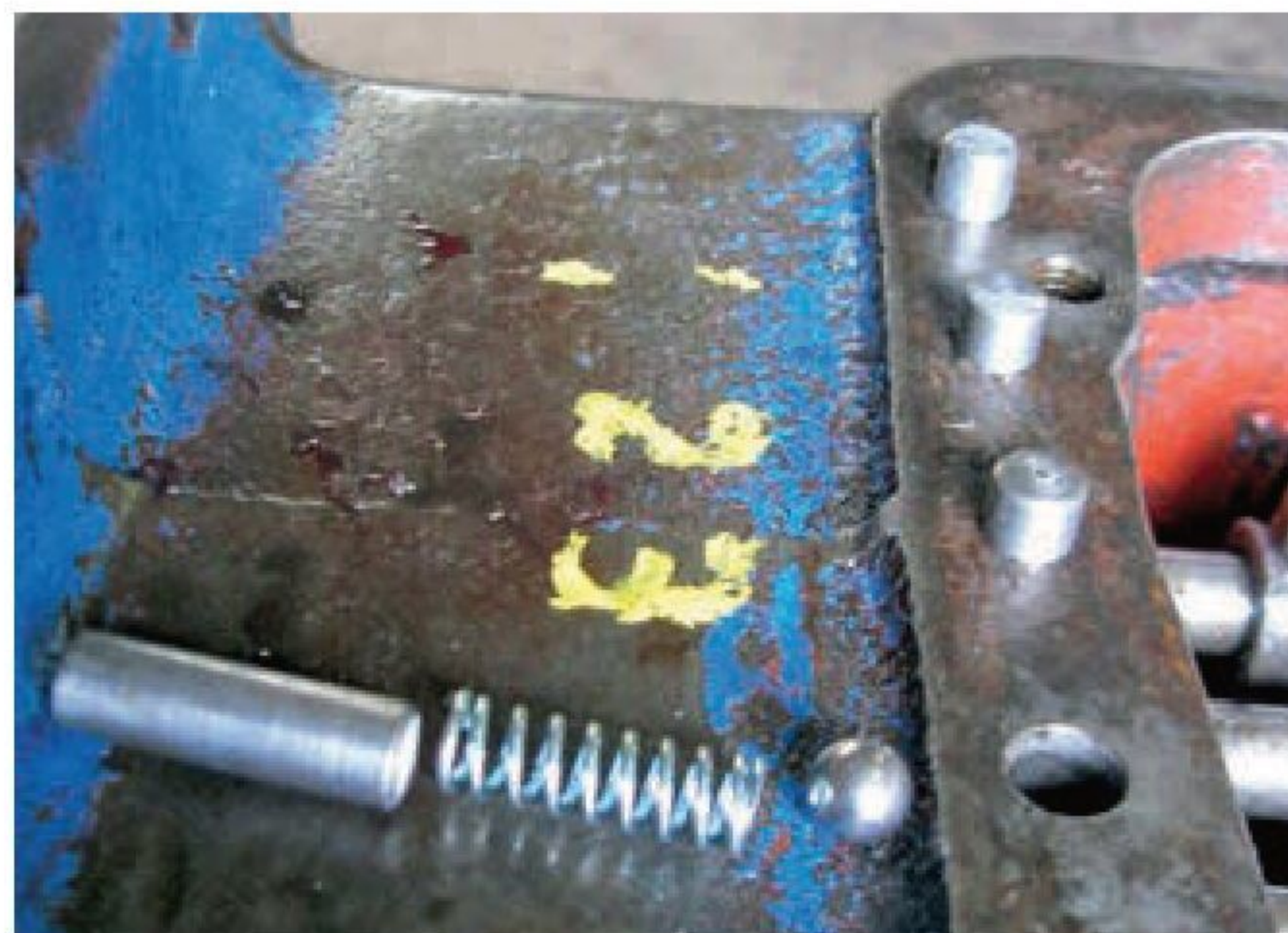
New balls, springs and spacers will ensure the correct amount of resistance on the selector rods.
