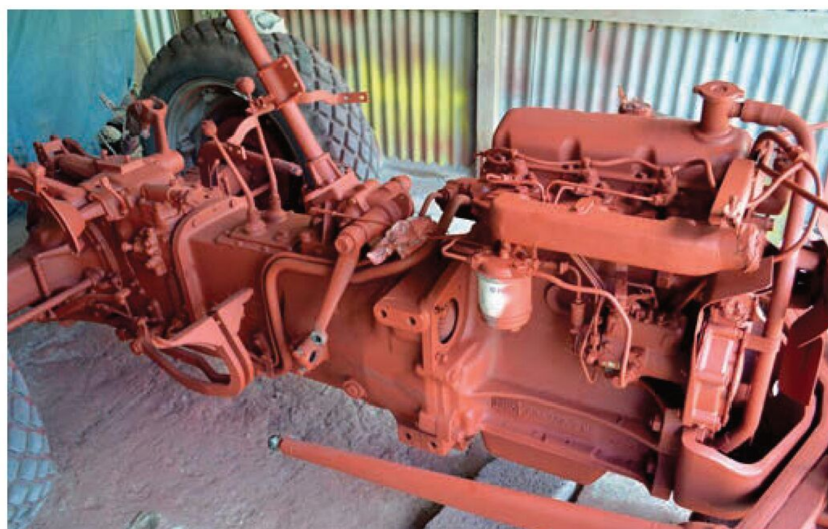
Red oxide is a perfect primer coat to start with. Be prepared, though, to use a lot, as a good coat around all the awkward areas is essential.
