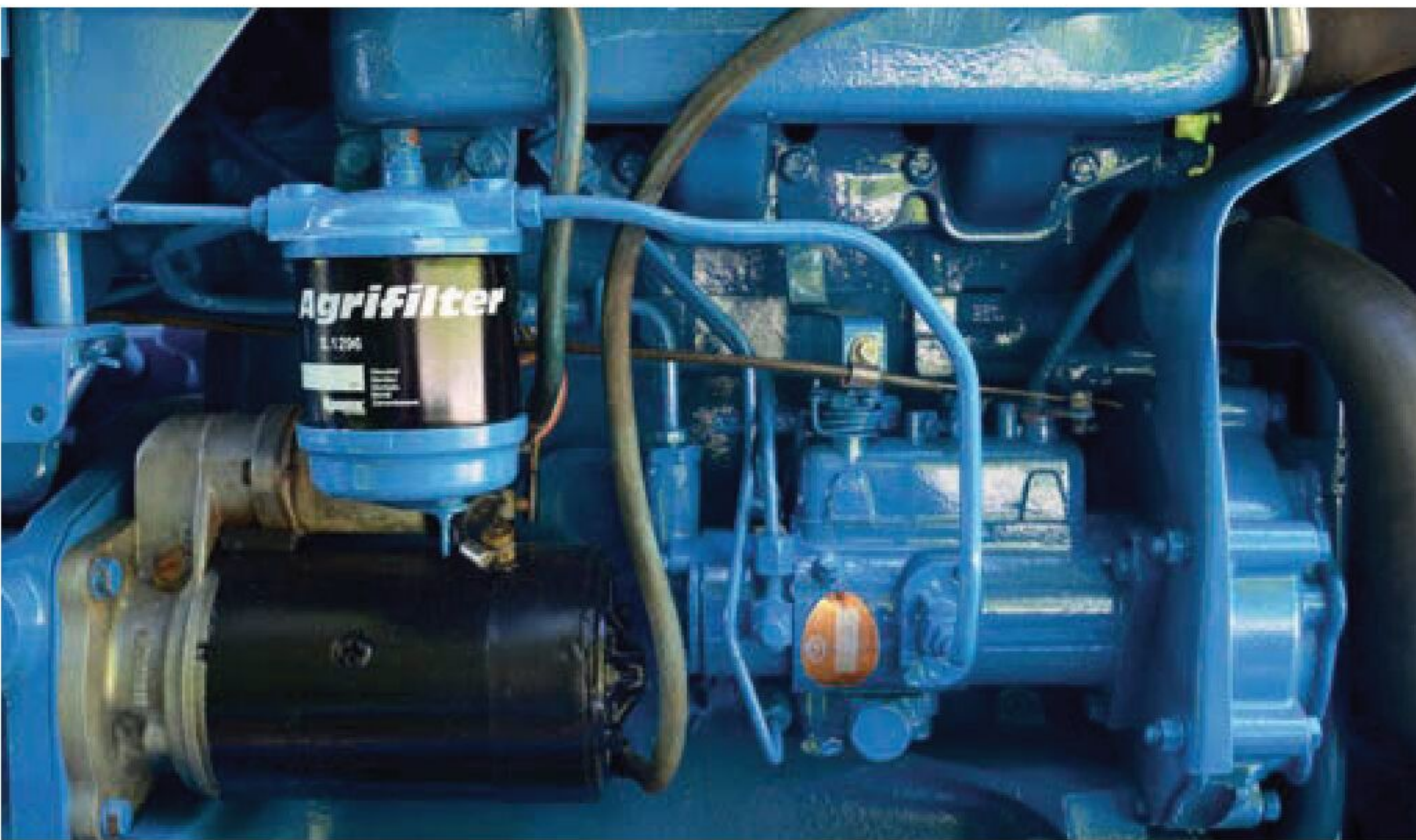
A new Sparex fuel filter was fitted and, like the dynamo, the starter was painted black. The CAV rotary pump had replaced the Simms unit found on the earlier 3000.
