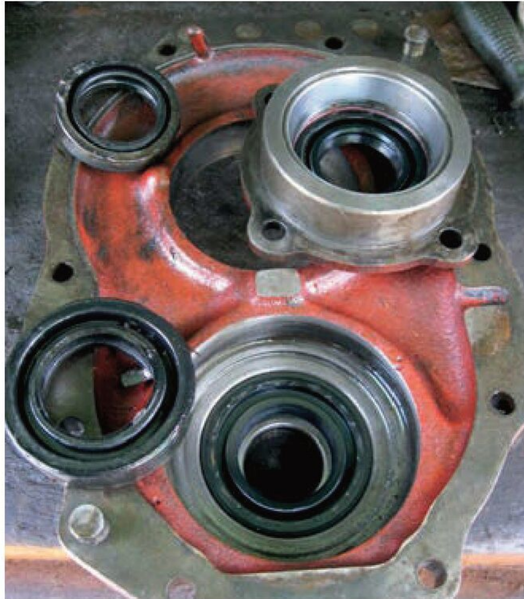
The old, back-to-back seal on the upper housing has to come out towards the larger of the two bearings. It cannot pass through the smaller bearing.
