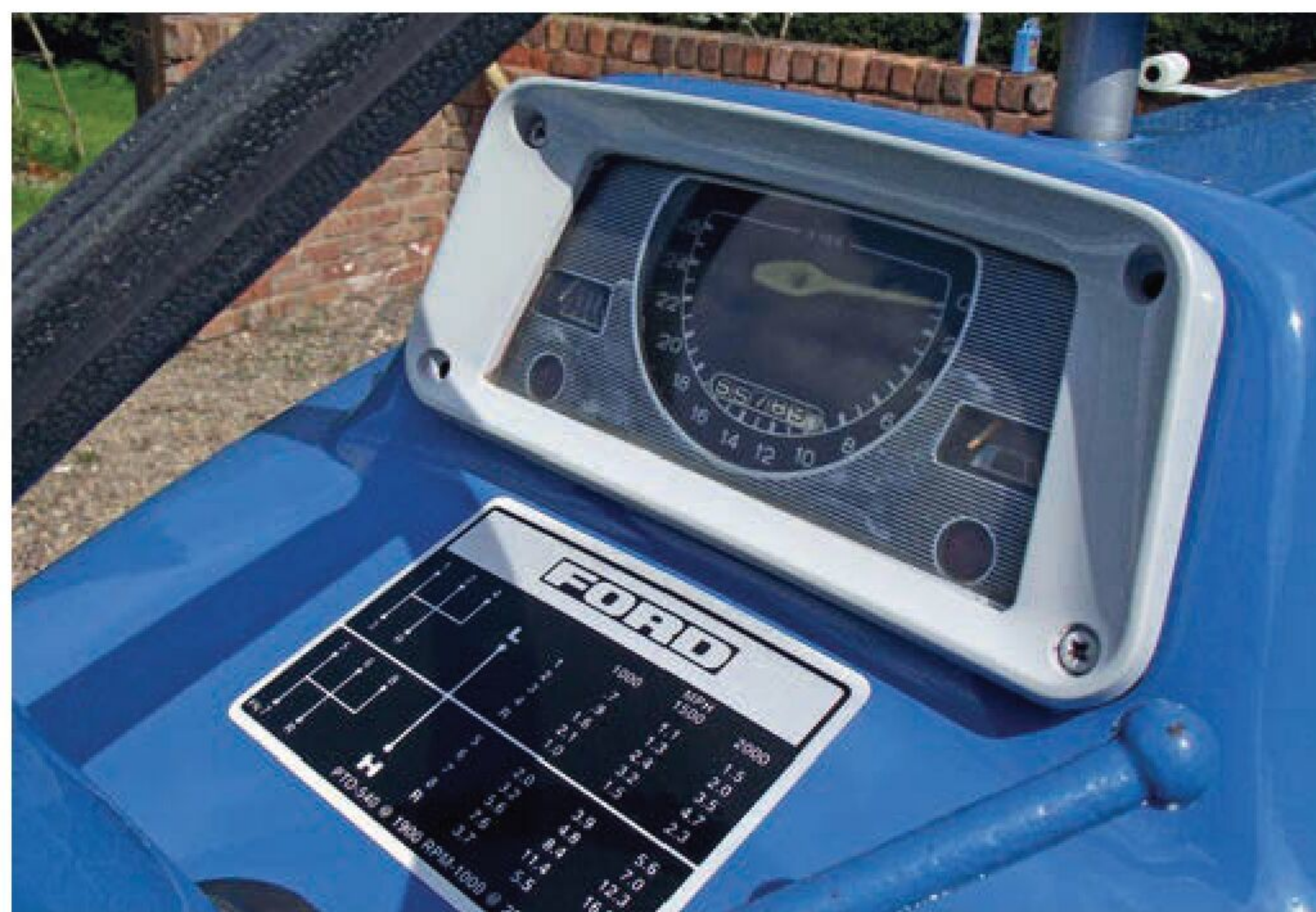
The Ford 4000 had a rectangular dash with tractormeter, fuel level and water temperature gauge, the oil pressure and charging circuit was catered for with warning lights.
