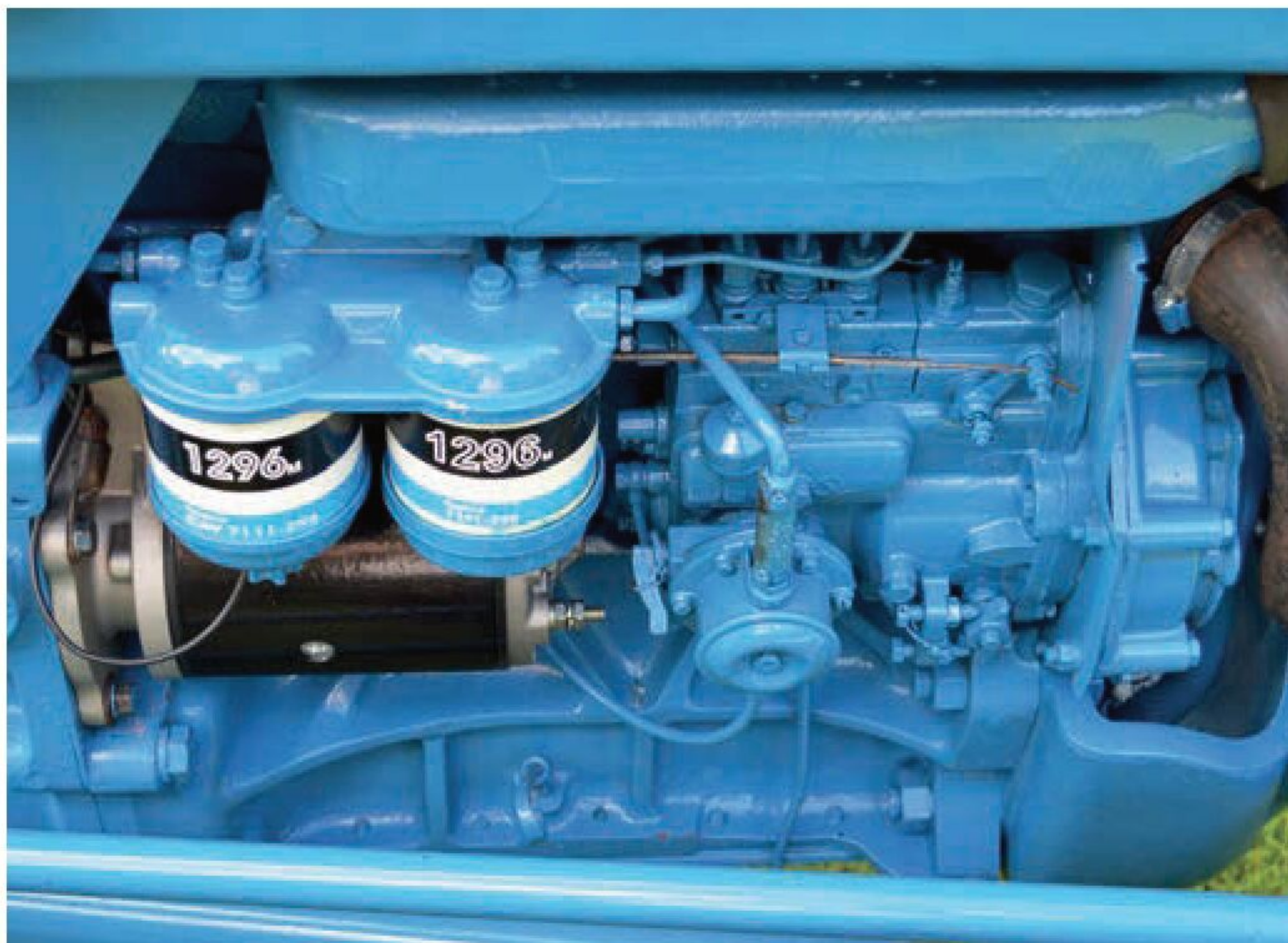
The original, Pre-Force 3000 engine blocks suffered with well-documented problems, which Ford eventually got to grips with. This side of the engine was rather cluttered.
