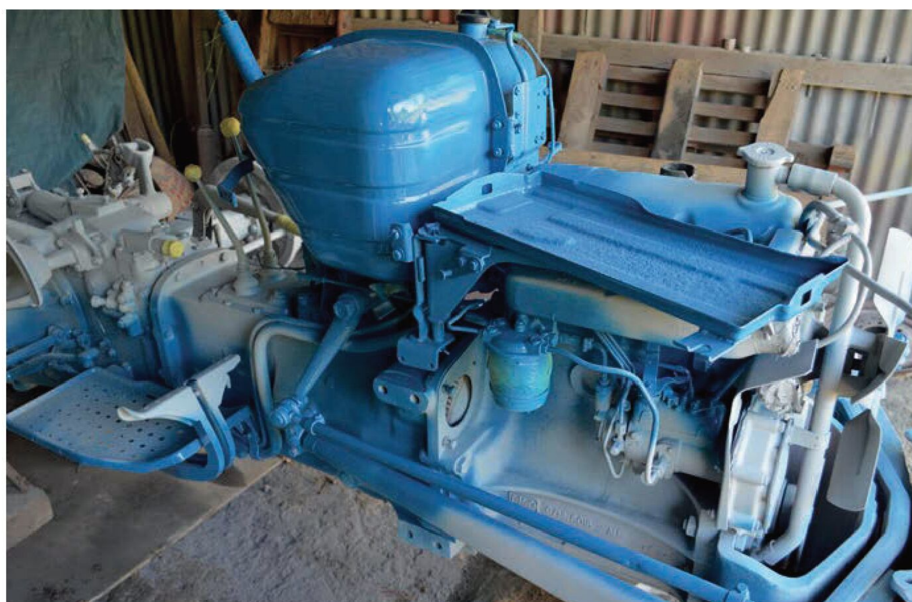
Grey undercoat followed the red oxide and, as soon as it was hard, the final colour was applied so that components could start being refitted.
