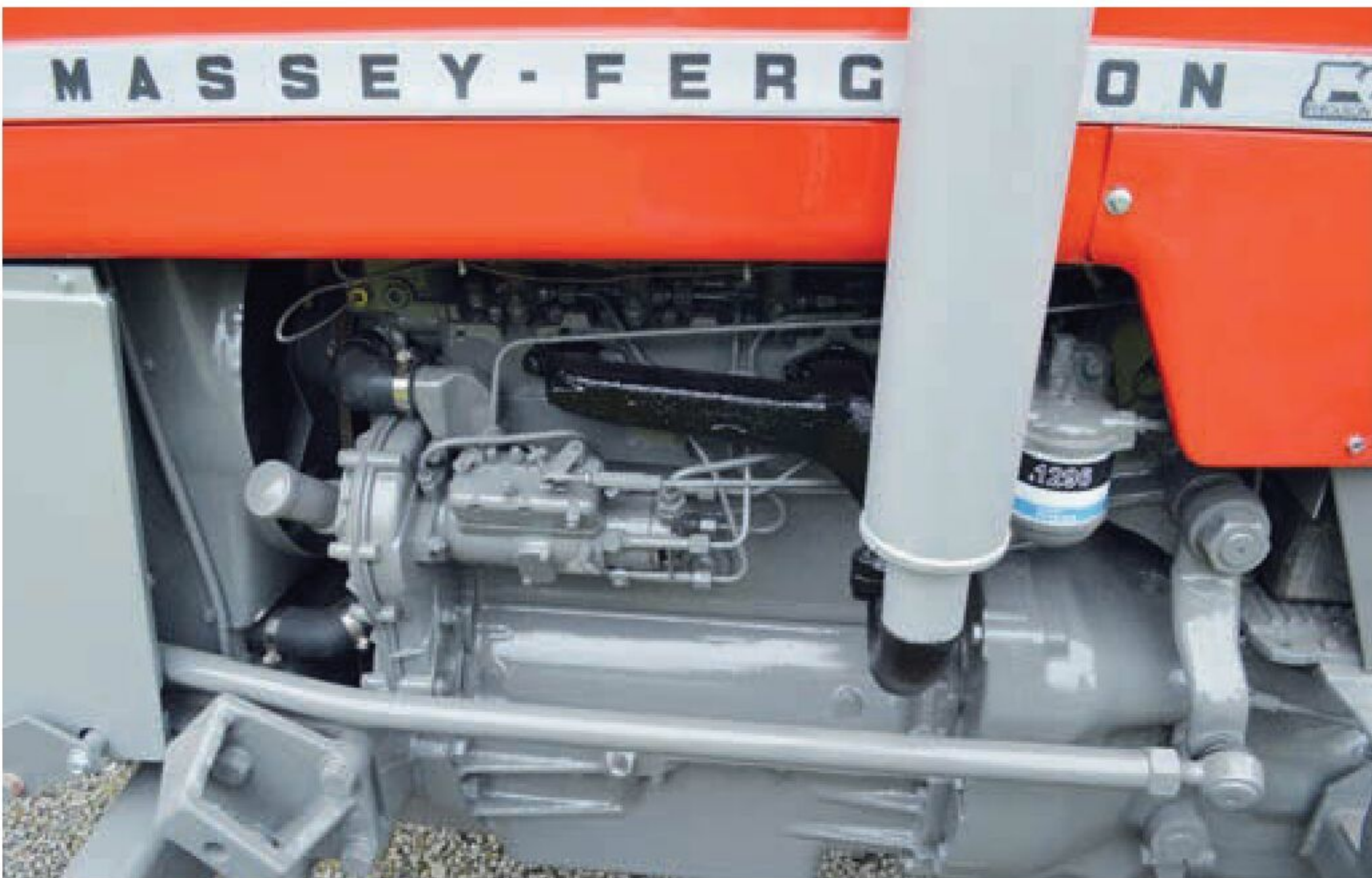
The early Perkins A203, four-cylinder diesel engine was tried and tested and proved reliable in the 165. It provided the benchmark for tractor engines at that time.
