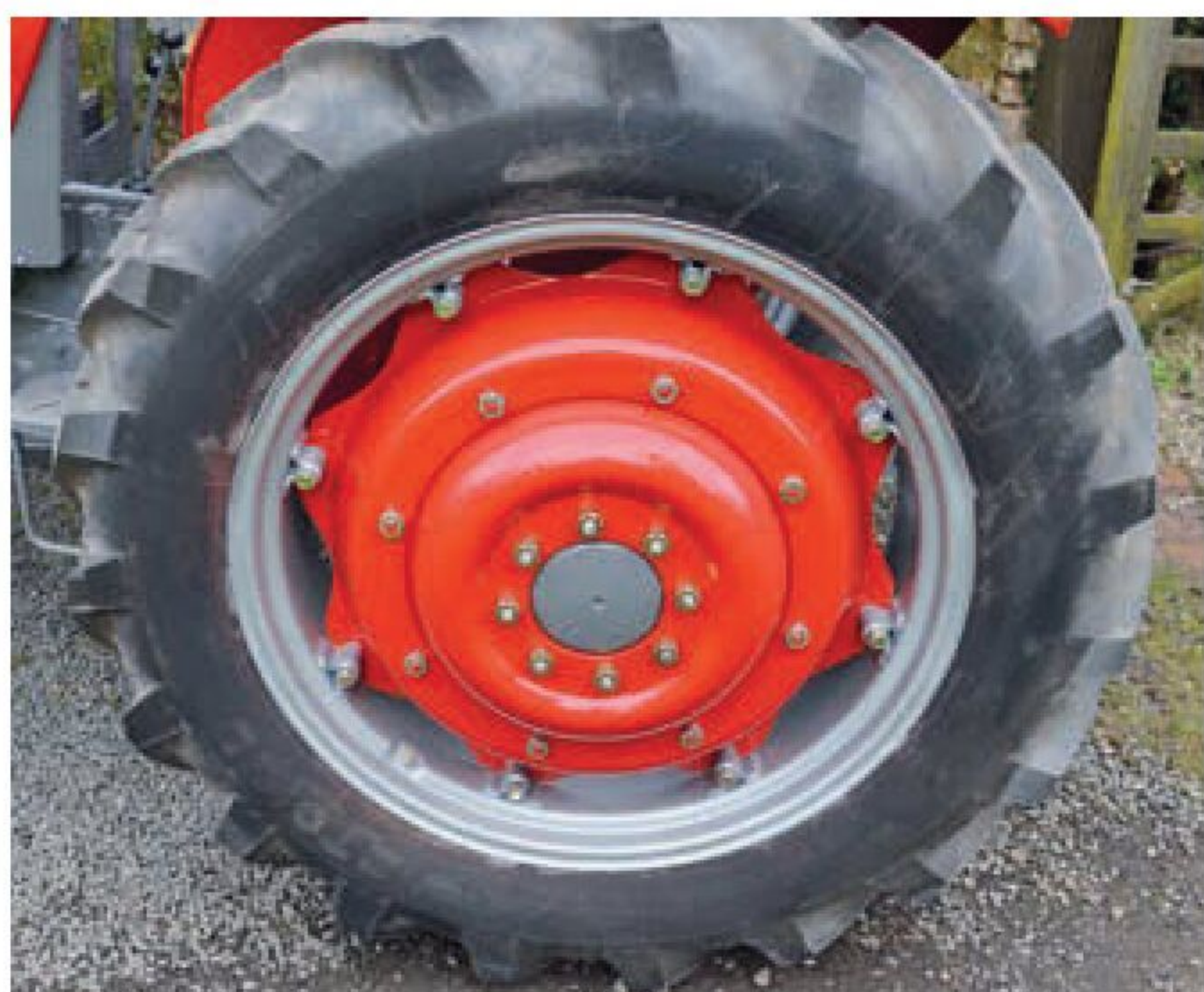
The rear wheels on the 165 featured centres that had dishes that could be split, allowing for a greater variety of widths.
