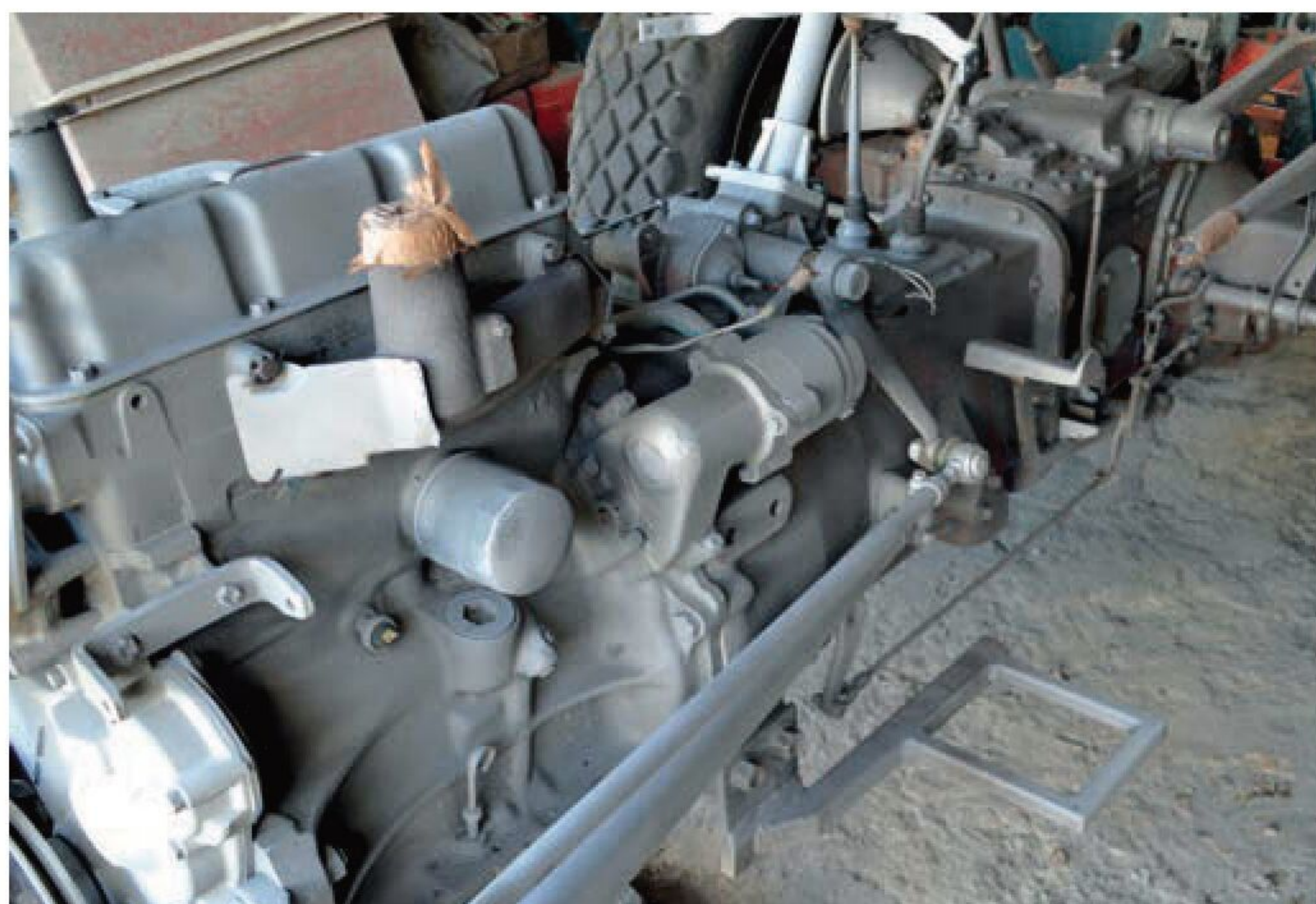
Sand-blasting effectively removed all the old paint and surface rust.
