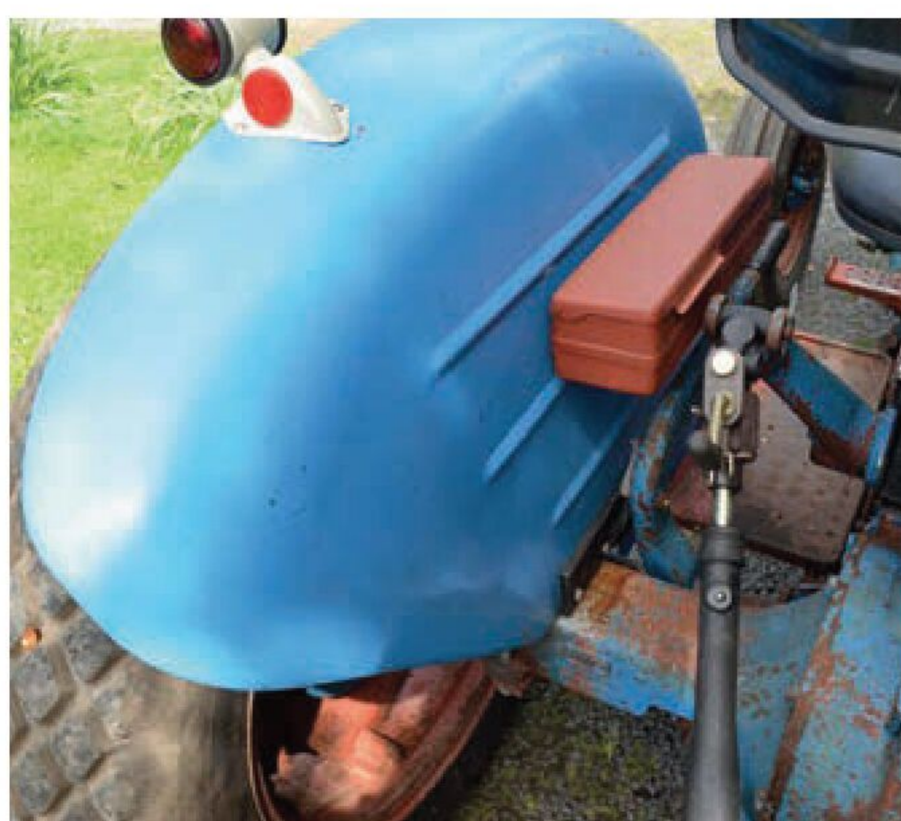
These reproduction wings were of reasonable quality and fitted well. The toolbox was also a good copy of the original.
