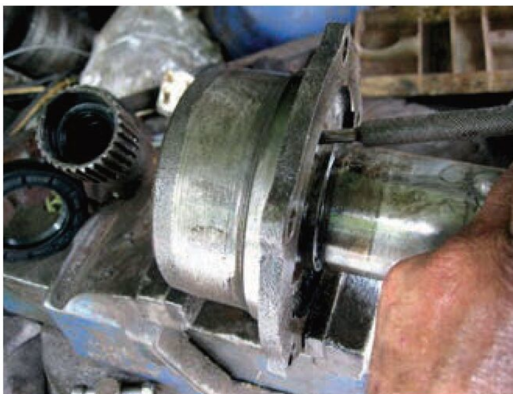
The tell-tale hole to show when the outer seal in the release bearing support tube housing is leaking, is handy to punch the old seal out.
