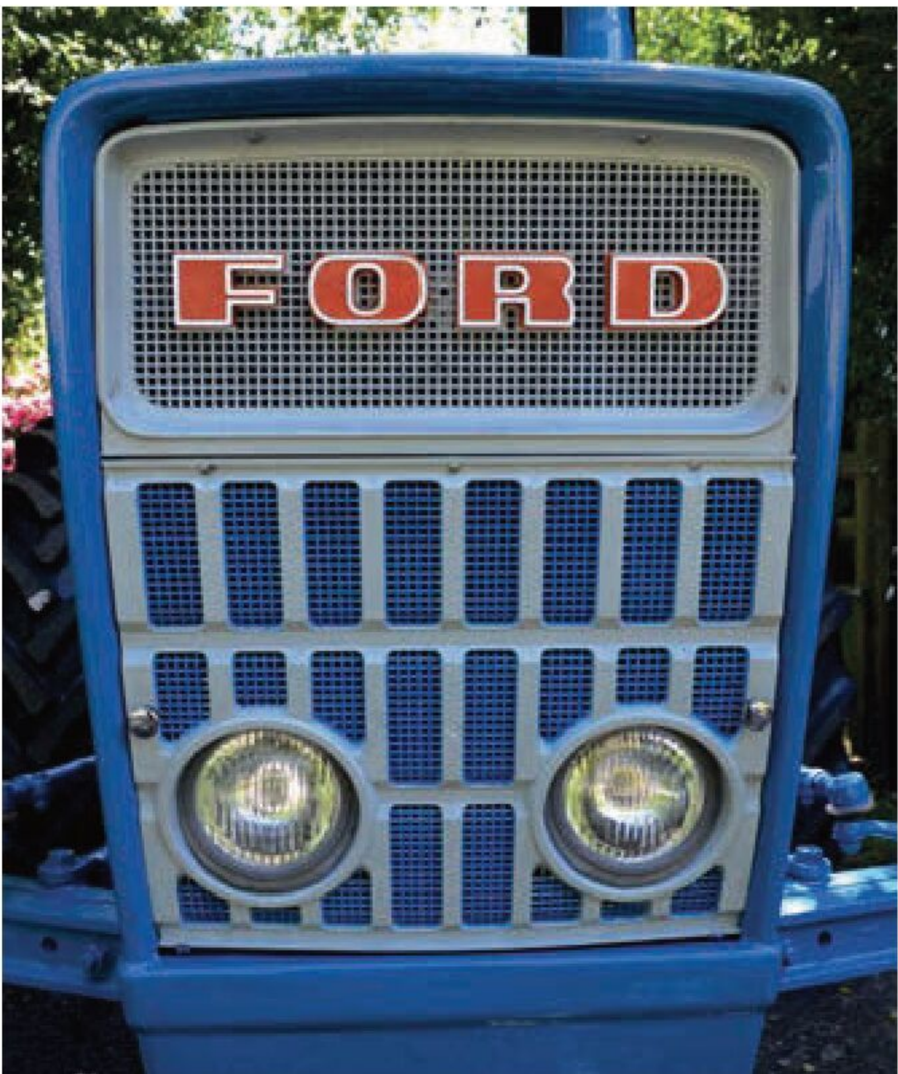
The new cowl, headlamps and grille make for a great-looking front end. The lower towing point (see pic on page 87) was left on as it helps anchor the tractor when on a trailer.
