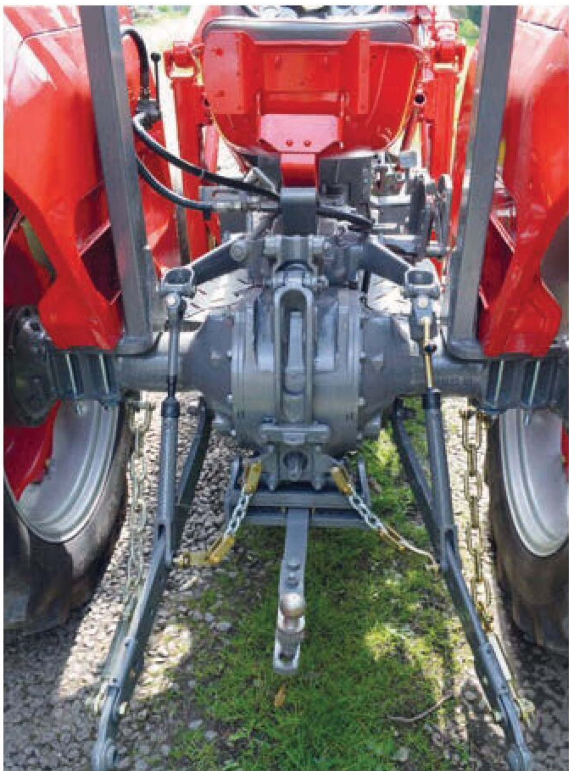
The hydraulic system on the 165 was a continuation of the one Harry Ferguson had developed years earlier.
