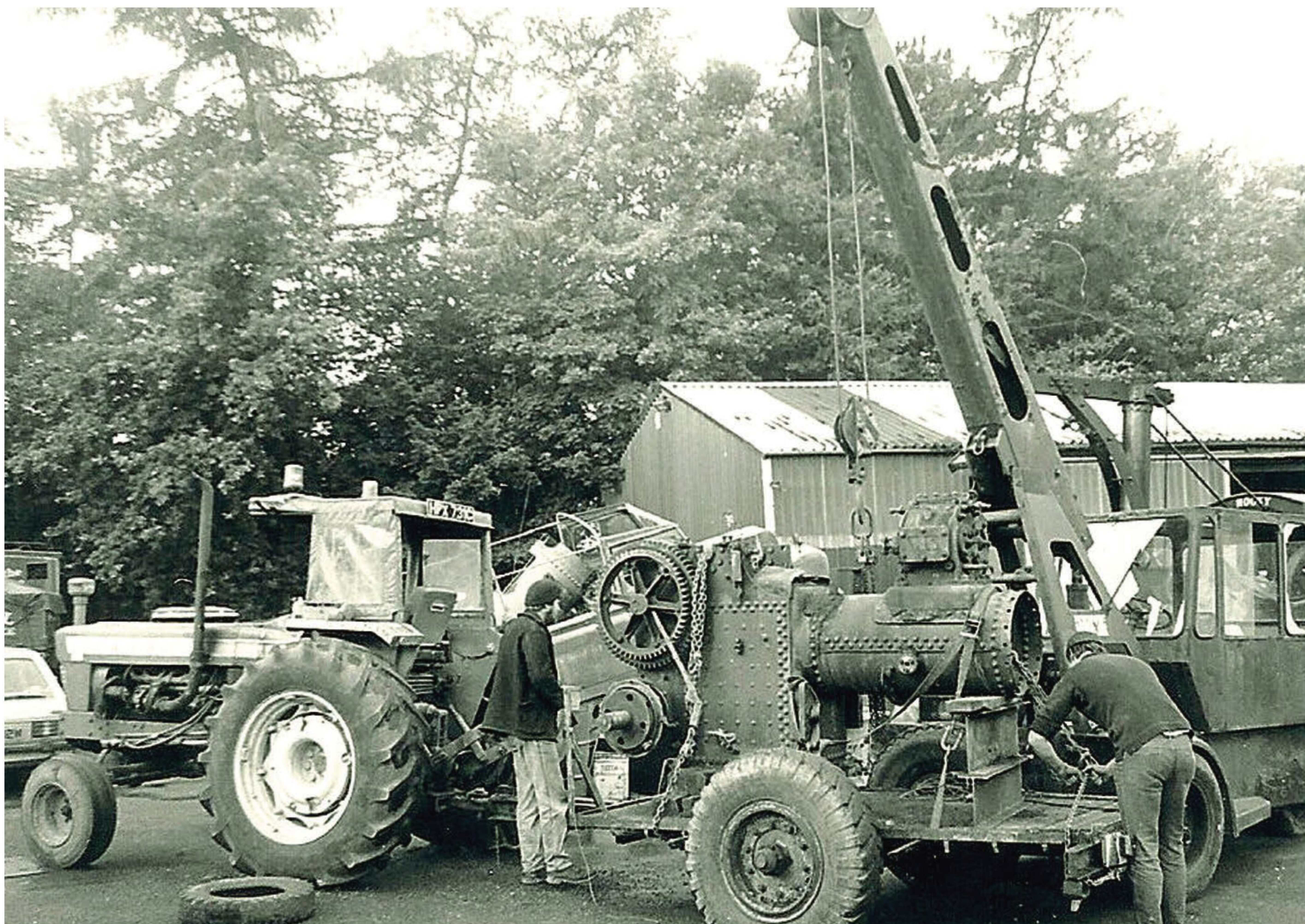
The old, WW2 searchlight trailer holds an Aveling & Porter steam tractor boiler assembly, which has just been collected by the Hybrid.
