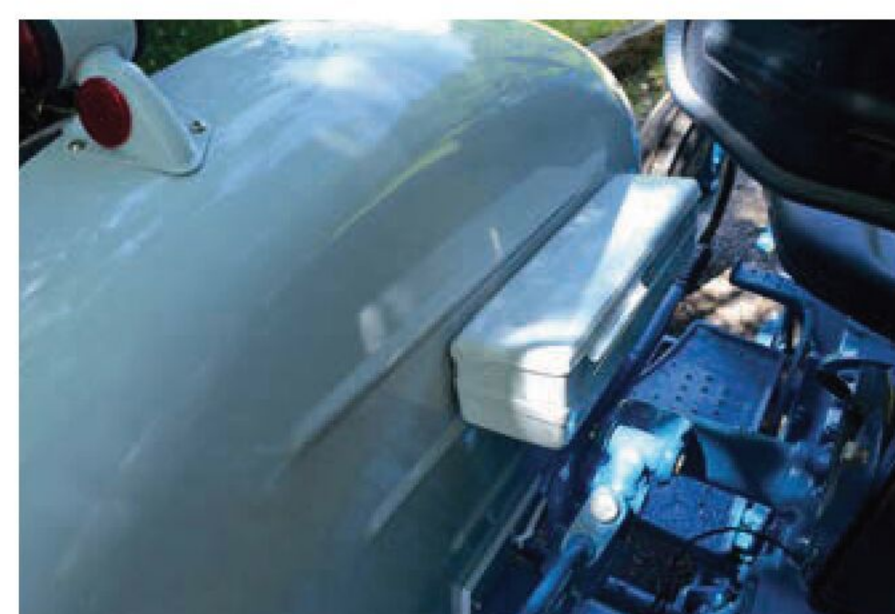
The wings needed very little work once they'd been sand-blasted. Four coats of paint got the finish looking right. The lights are exact copies of the originals.
