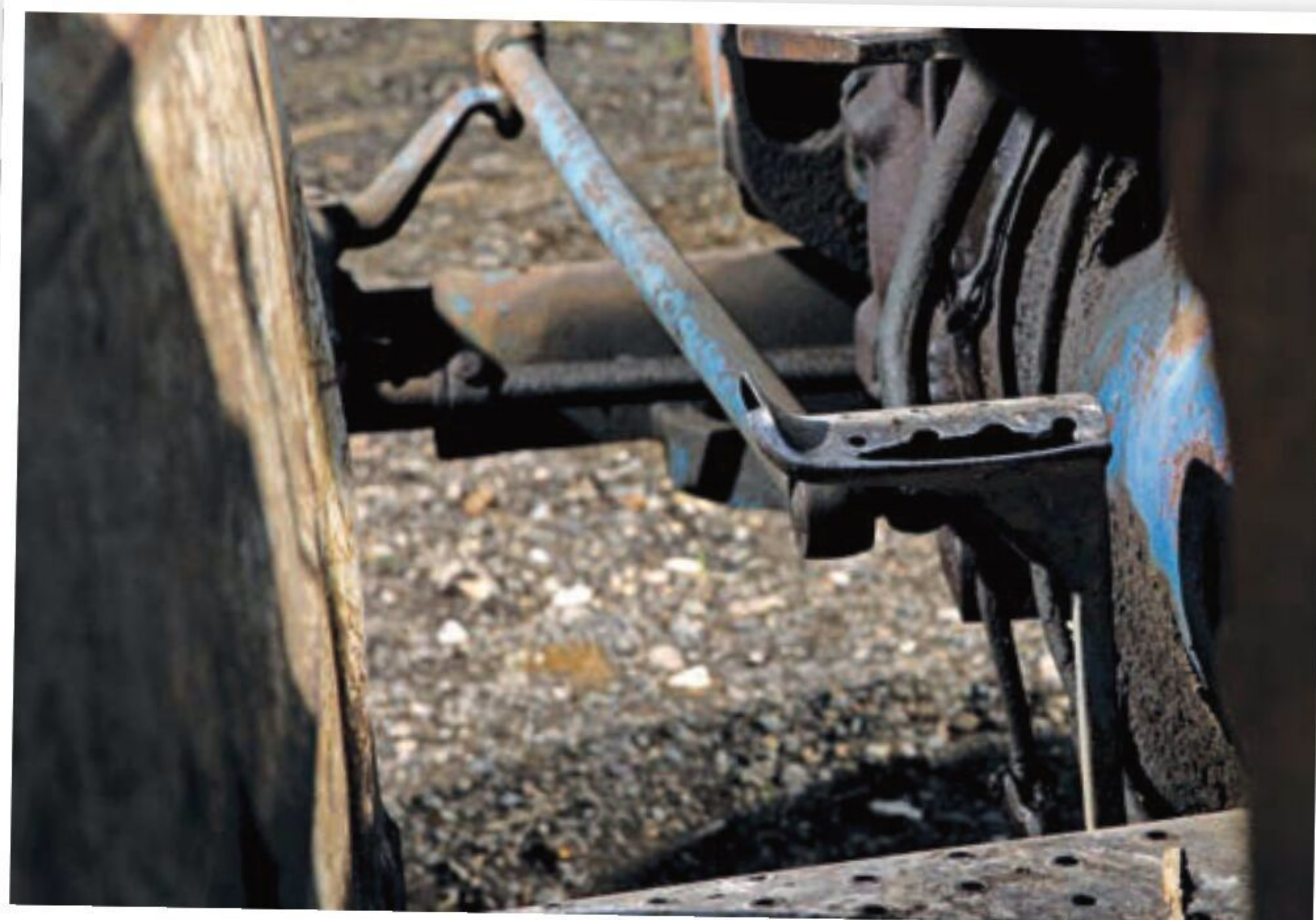
BELOW: The clutch pedal shows what years of left foot pressure can do.
