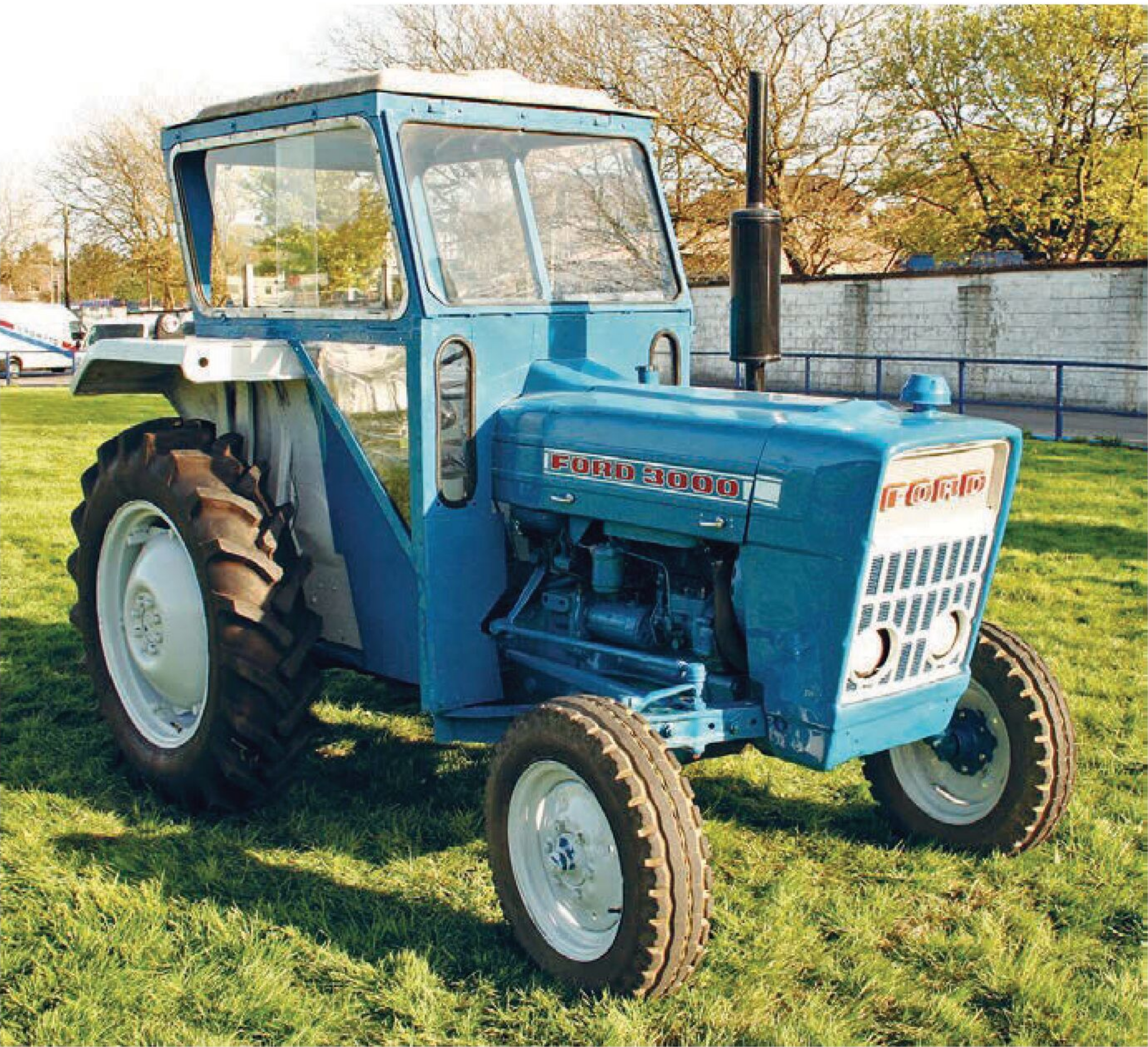
This Irish example is fitted with a Duncan cab.
