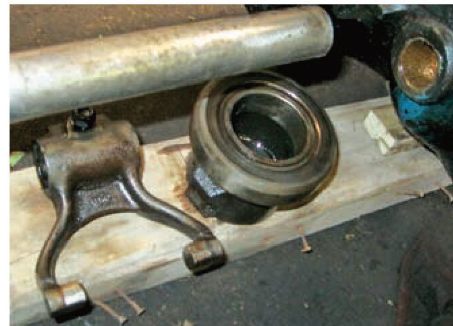
New bushes were fitted to the bell-housing before refitting the clutch shaft, fork and release bearing.
