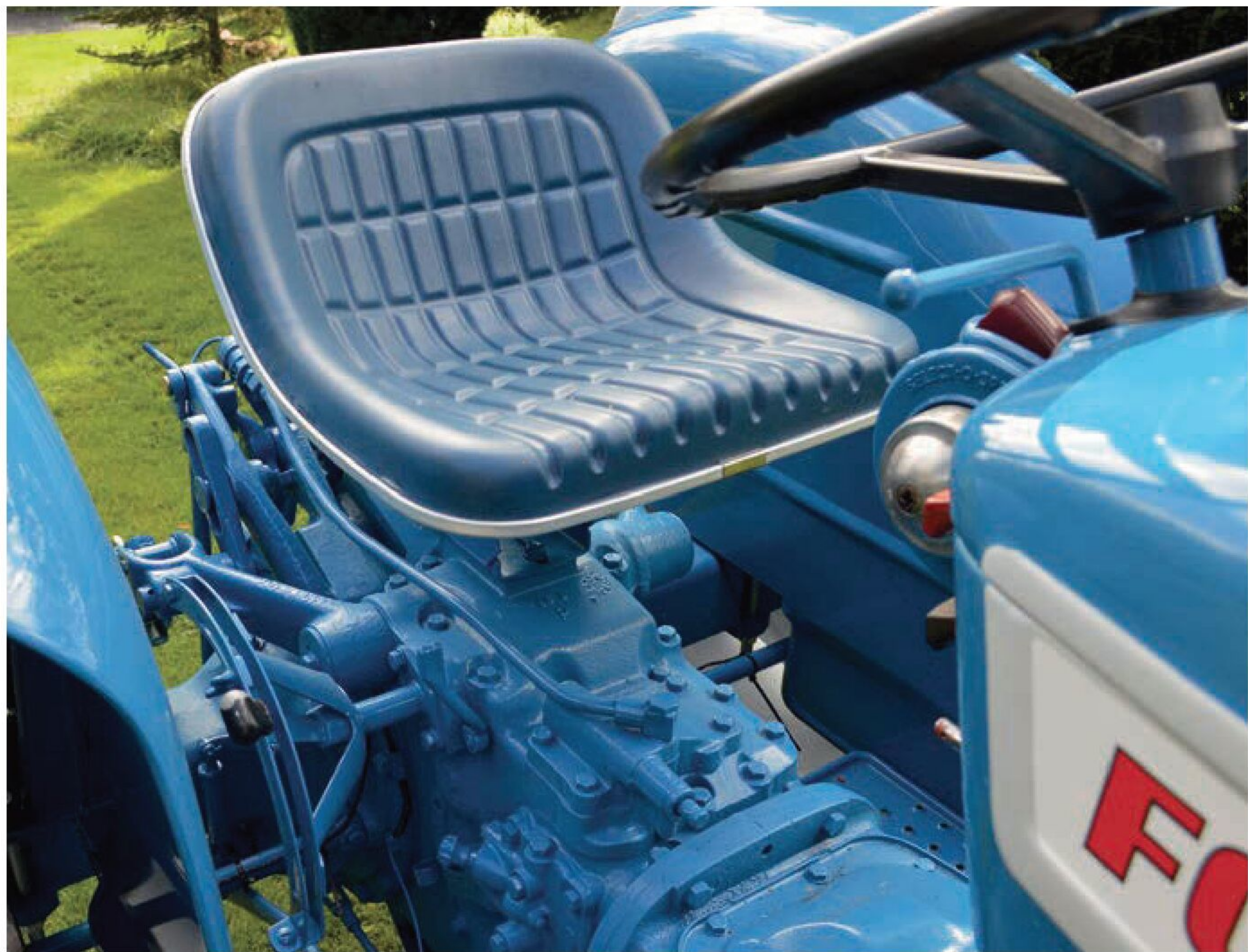
Both Pre-Force and Force 3000s used the same seats, which had a degree of adjustment and a one-piece, ribbed cover intended to help stop water puddling.
