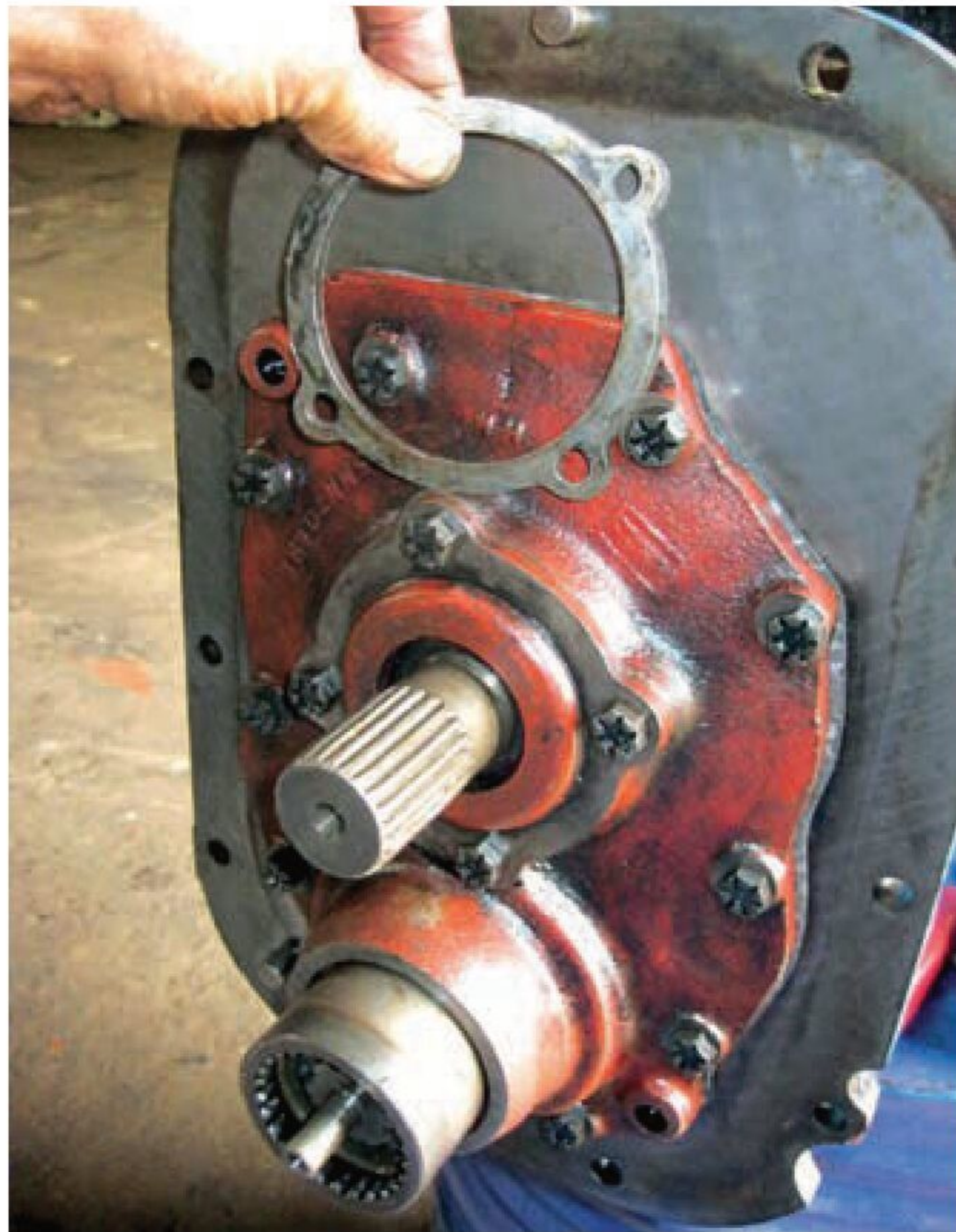
The upper bearing flange has shims with which the play on the output shaft bearings is set. In this case, with all the shims removed, the bearings felt just right! The PTO front shaft could be refitted, remembering first to fit the large gear into the bell-housing, followed by the output driving dog and circlip.
