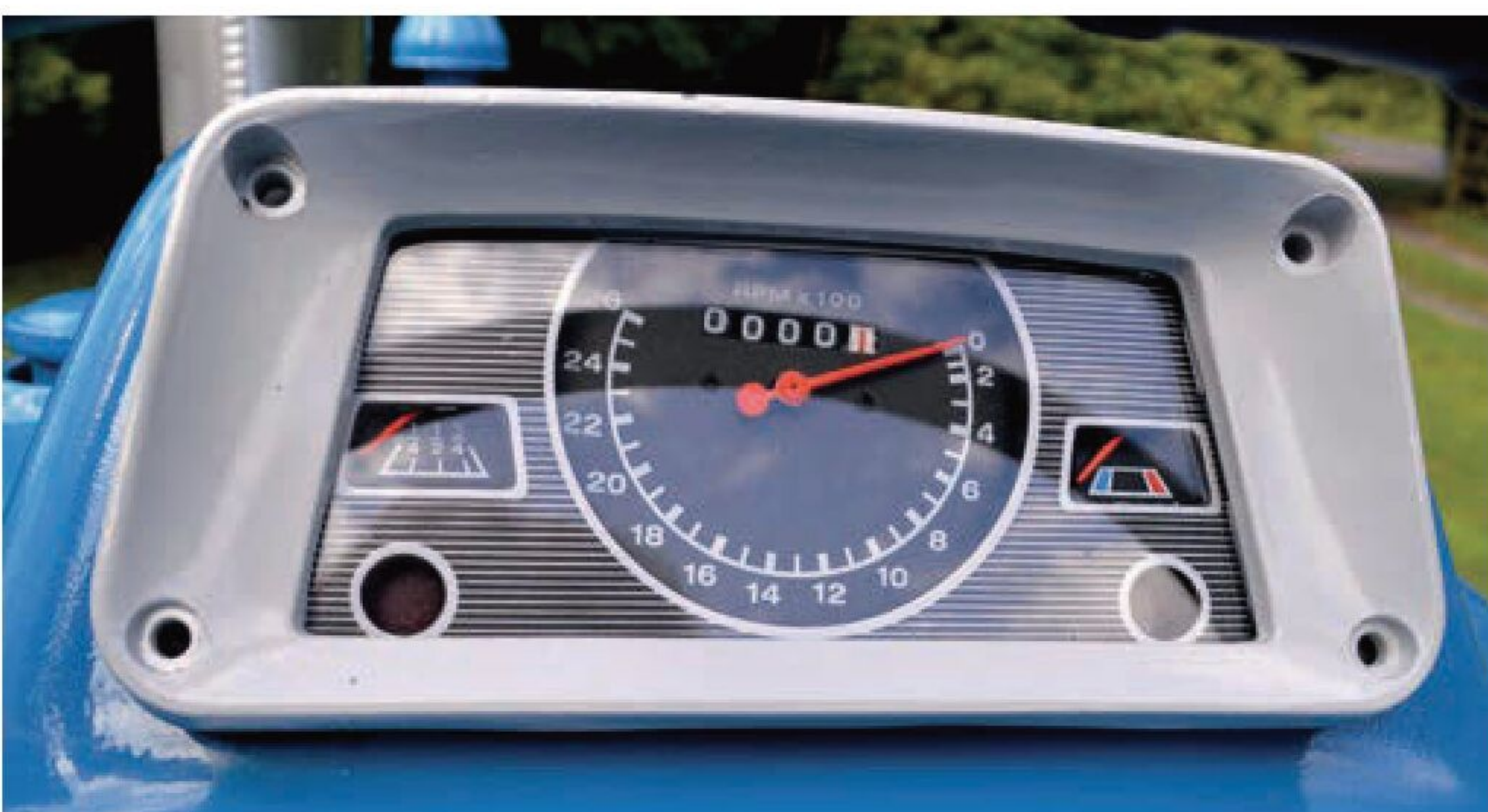
ABOVE AND RIGHT: The instrument clusters used on Pre-Force and Force 3000s were largely the same, featuring a tractormeter, fuel and water temperature gauges, plus warning lights for the charging system and oil pressure.
