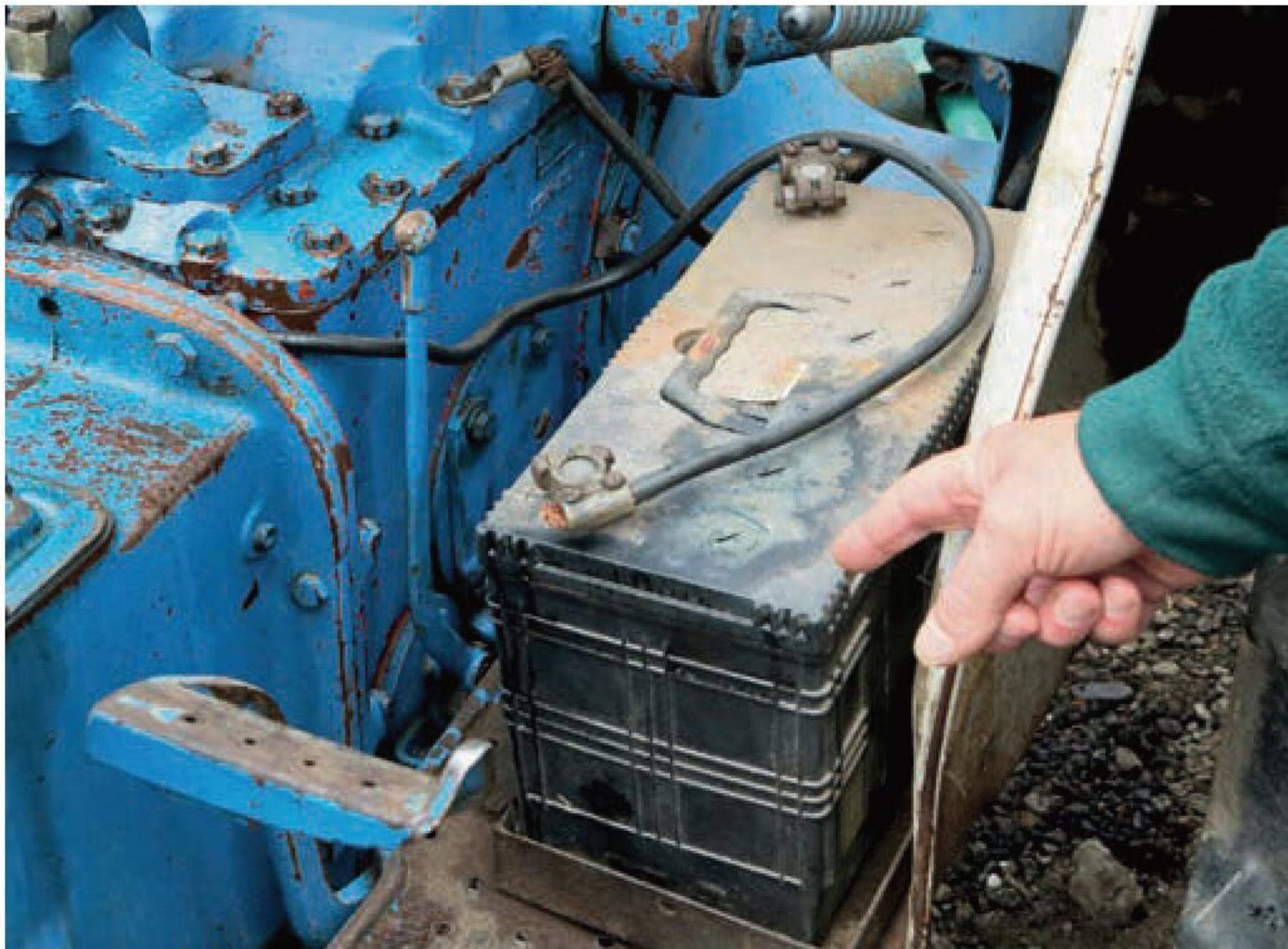
The battery was moved to the left-hand footplate.
