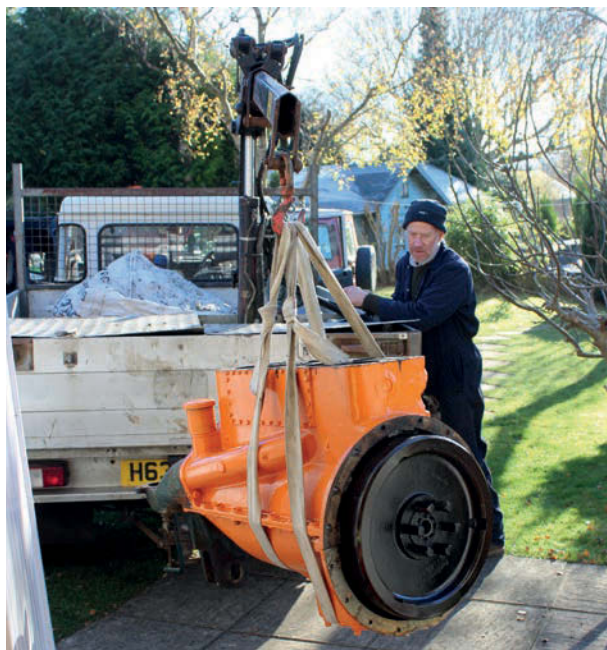
The engine, minus its cylinder head, is easily brought into the workshop using Nigel's hydraulic crane.
