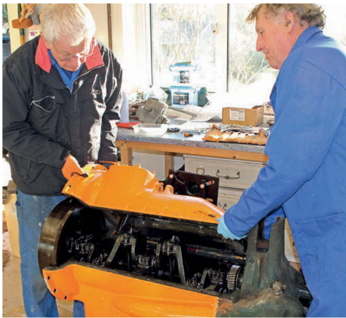
Bill and Bob (right) lift off the heavy sump assembly to reveal the big end and main bearings.
