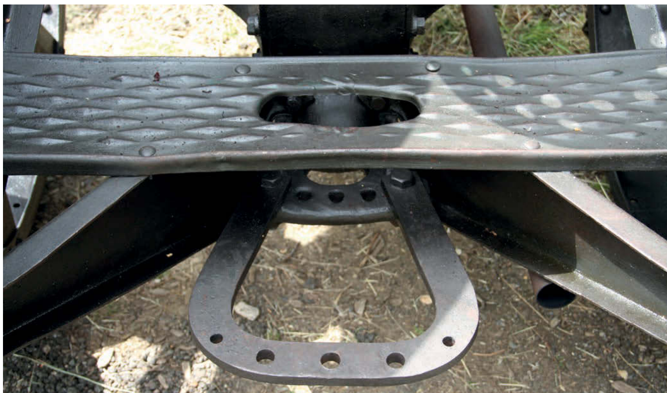
A drawbar showing virtually no wear is another of this tractor's amazing features.
