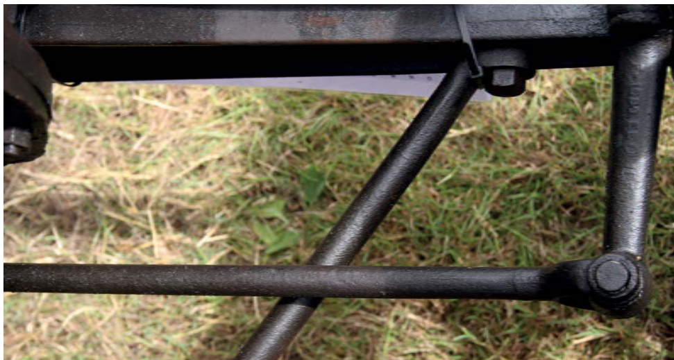
Luckily, the pins and bushes in the steering system were all found to be in remarkably good condition on this machine. Another indicator that its working life in southern France wasn't a particularly hard one.
