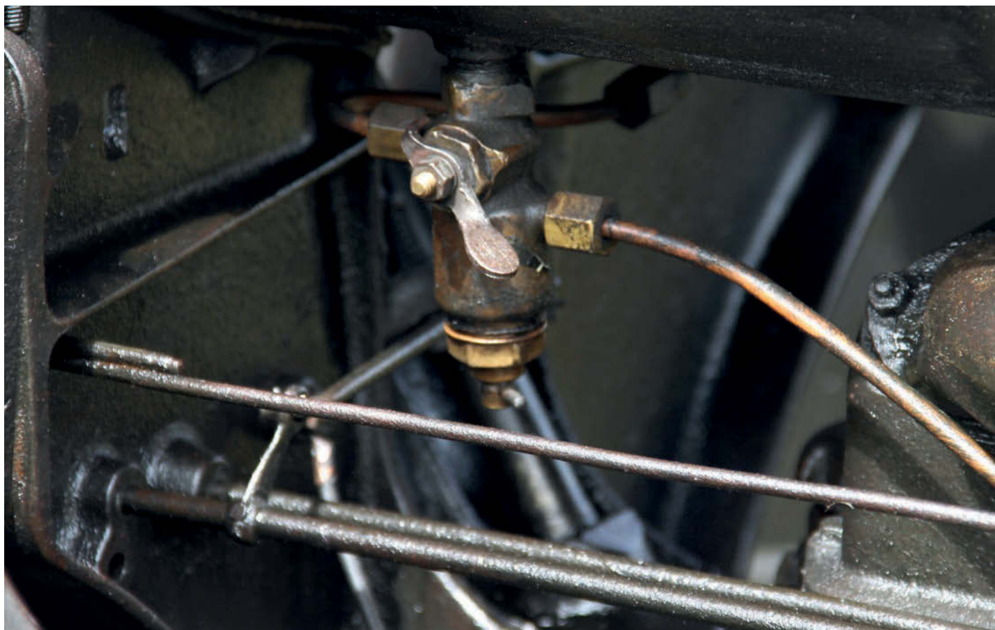
Even the fuel tap doesn't leak on this superb example; many do on both Model F and N tractors.
