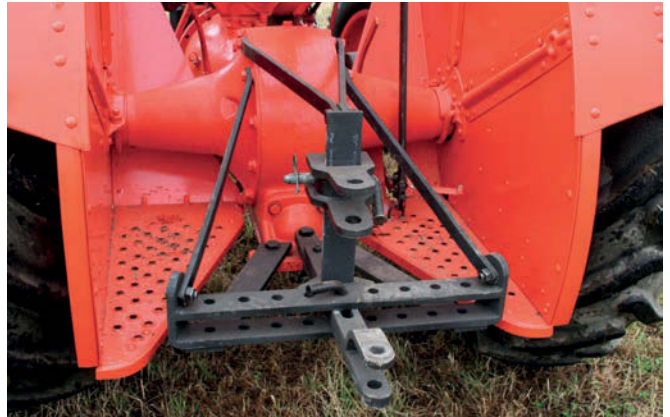
Peter Gillet fabricated the two-level drawbar himself, to replace the winch that came with the tractor, but he wouldn't do it again!
