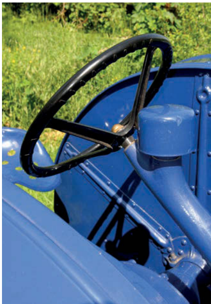
The hollow steering column acted as an air passage between the air pre-cleaner and the bowl.
