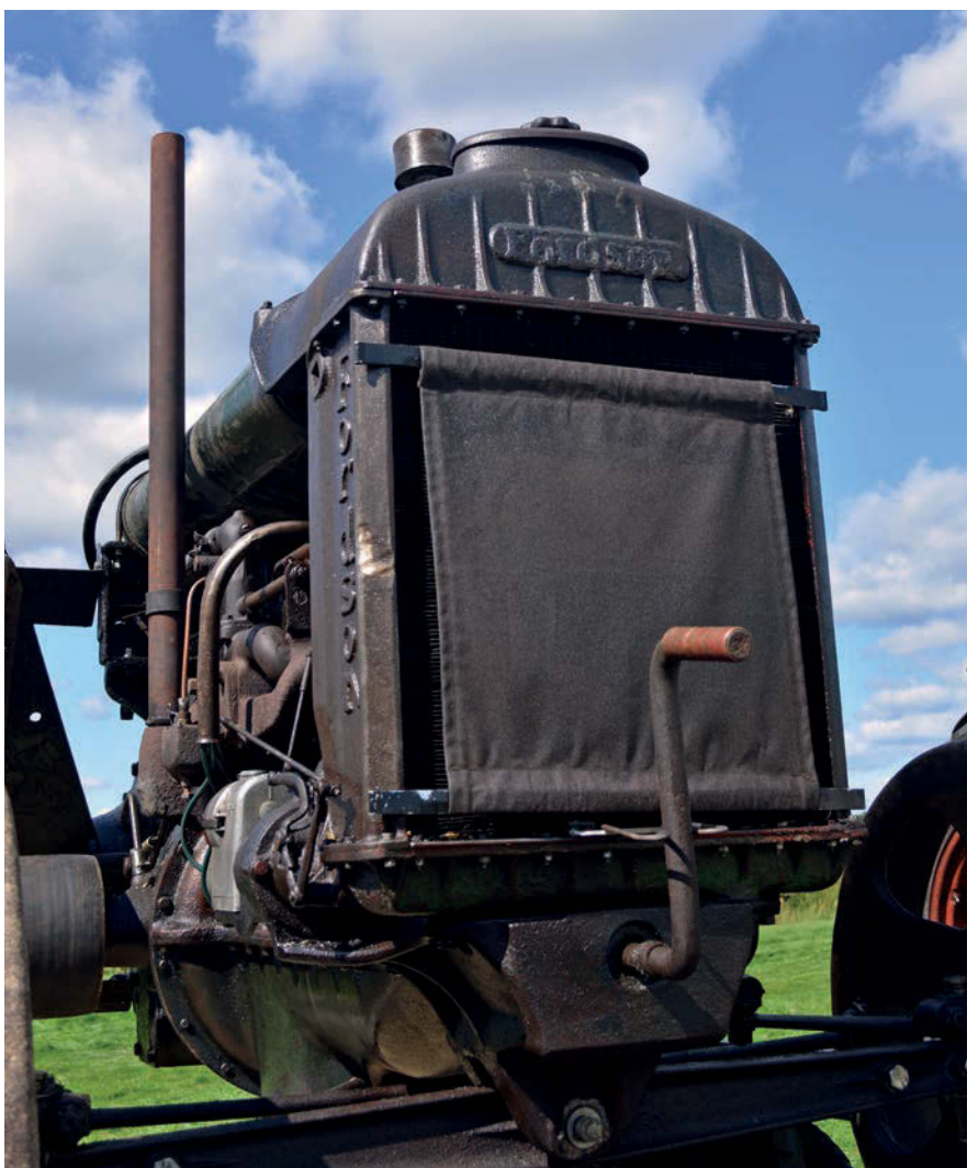
The radiator needed soldered repairs to some of the cores to deal with fluid leaks.
