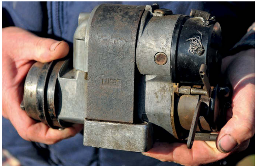
This is the Lucas GJ4 magneto that was fitted to the Model N following the outbreak of World War Two. In practice, it wasn't a great performer, perhaps due to its exposed position.
