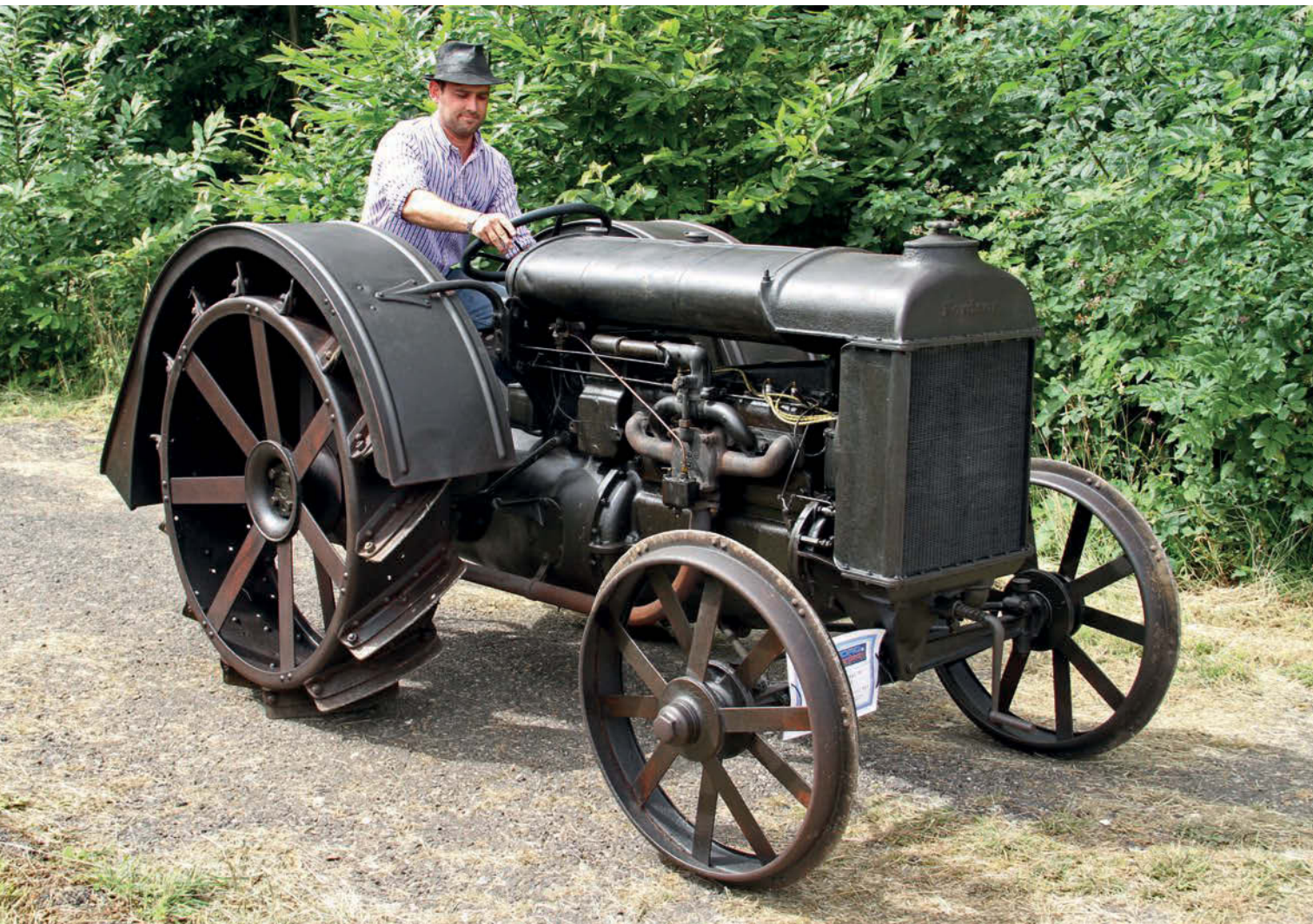
Adjustments are made to the Holley 295 carburettor, to control the engine's slow-running performance, from the driver's seat.
