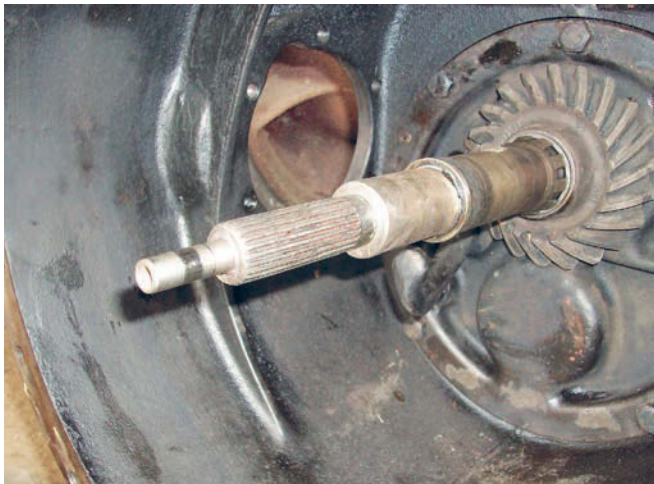
New spigot shaft in place and ready to receive the Sherpa clutch.
