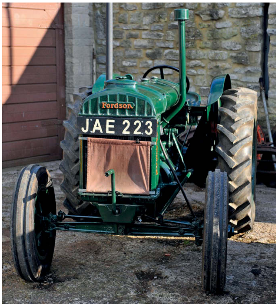
Narrow wings were a wartime economy measure, to save as much steel as possible for the war effort. The radiator blind was a common feature designed to speed engine warming.
