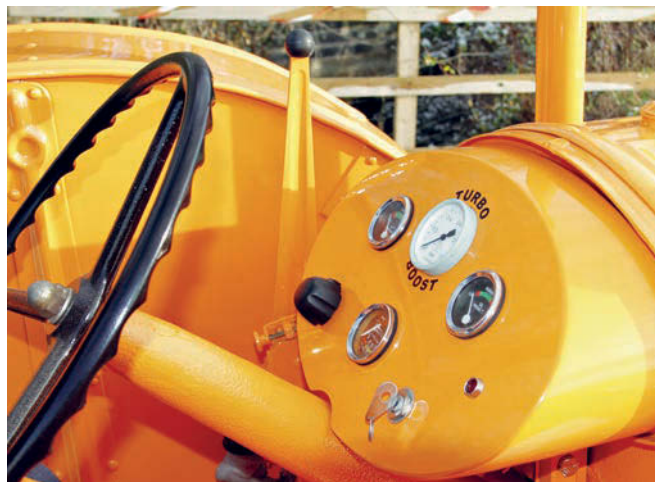
The new dash panel in place and painted, complete with all the gauges.
