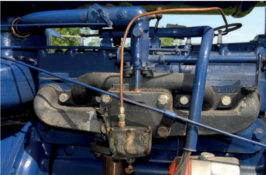
Despite some cracks, Thomas was able to retain the original manifold.
