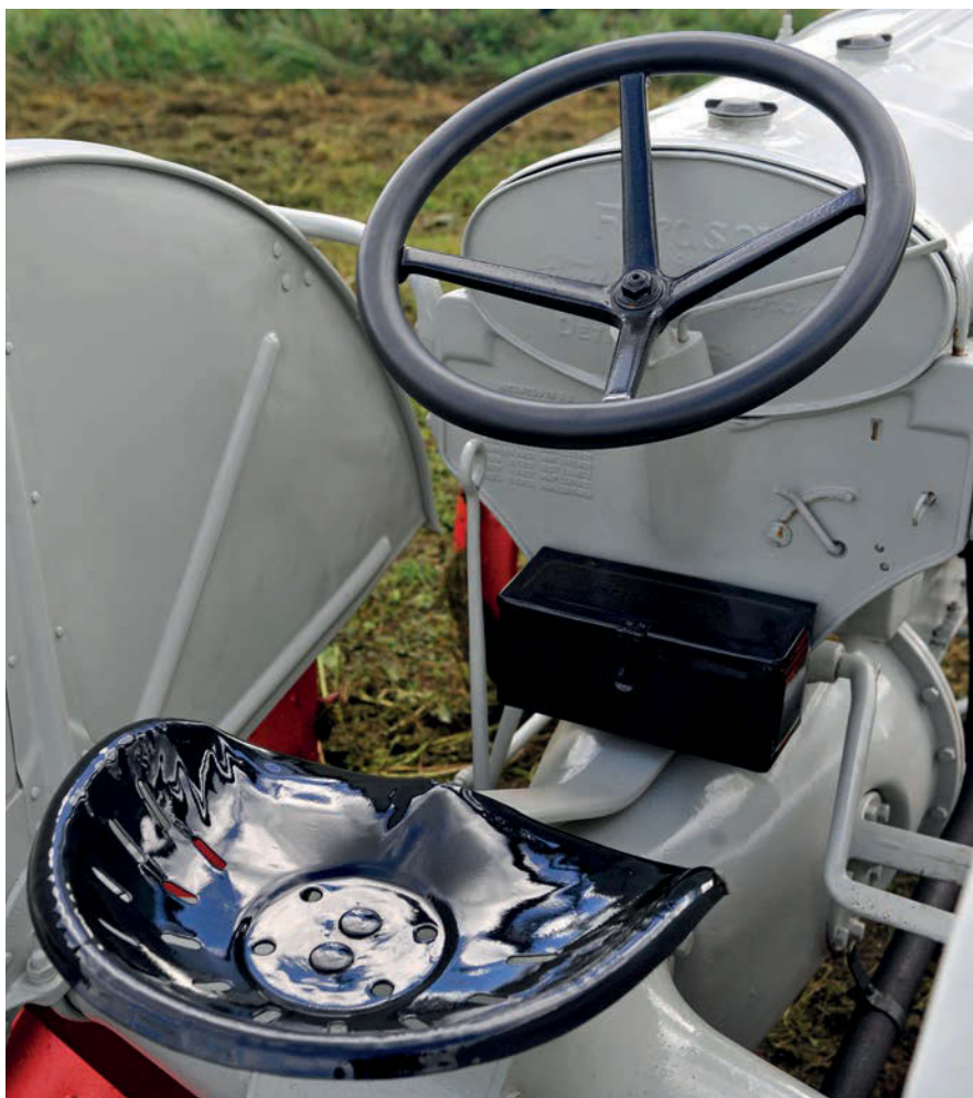
Model F controls are rudimentary. There's a clutch/brake pedal on the right-hand side, a spindly gear stick on the left, an ignition advance/retard control on the bulkhead and a throttle lever immediately beneath the steering wheel.
