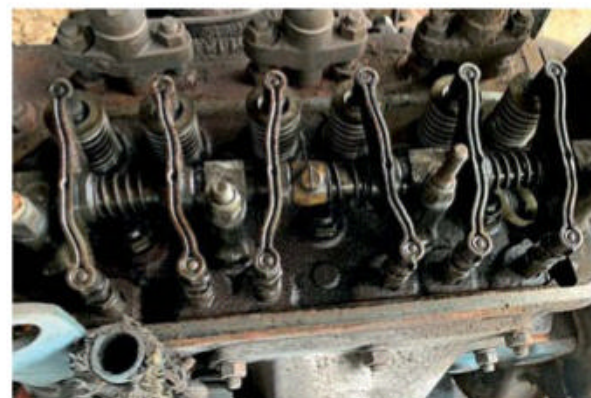
With my first clear view of the roster shaft, I was pleased to see that, although dirty, the overall condition didn't look too bad.
