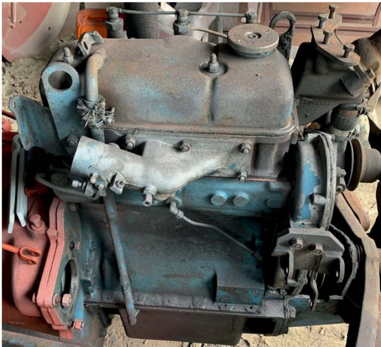
This side is relatively bare; I'd already removed the starter motor, the wiring loom and the alternator.
