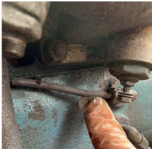
Knowing that I'd soon need to remove the cylinder head, the next job was to undo the other end of this oil feed pipe.
