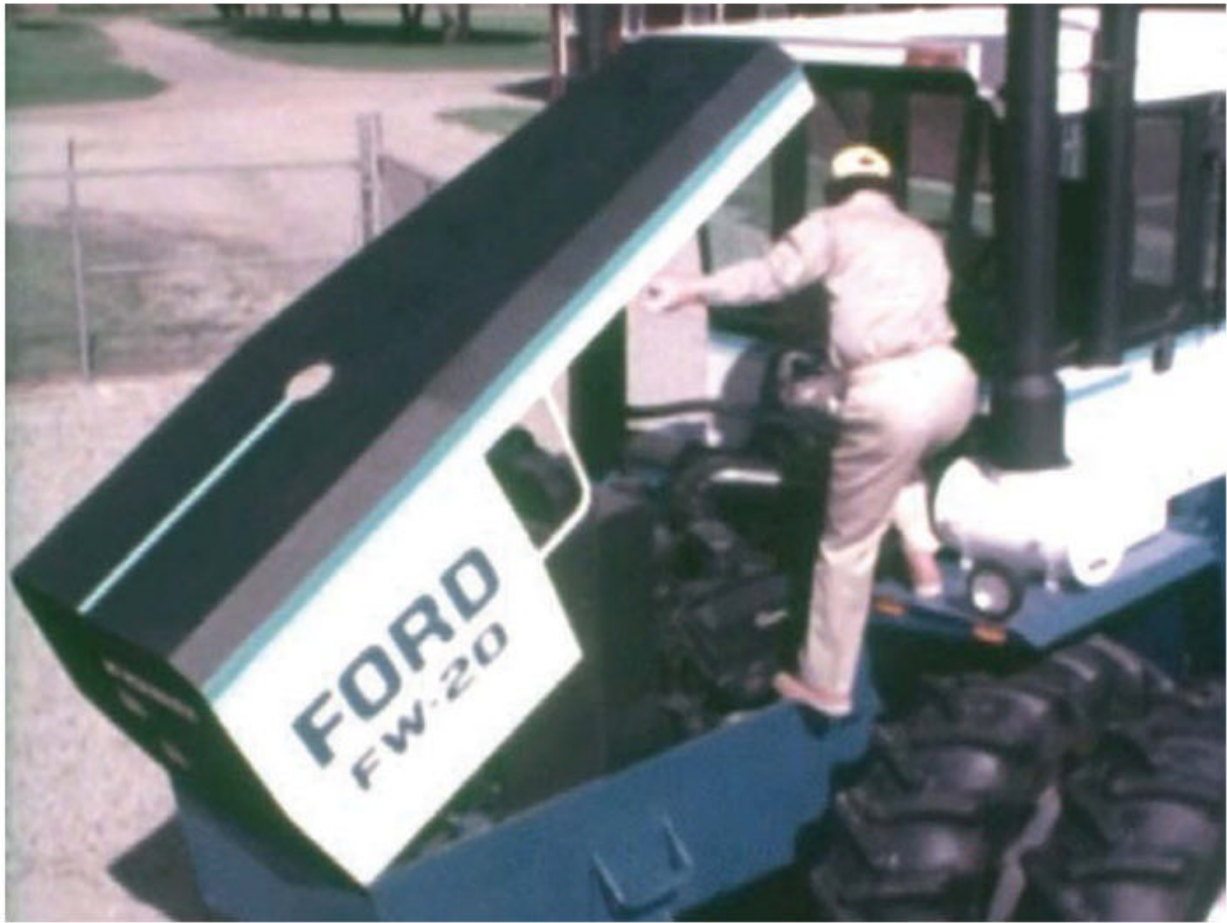
The top of the FW’s bonnet was painted black to reduce glare from the sun affecting the driver. The whole, massive bonnet could be hinged forwards to gain access to the engine for routine maintenance.
