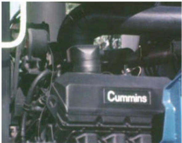
Many truck components were used on the FW tractors, as had become the norm for big, articulated, 4WD tractors in North America. These included Spicer transmissions and Cummins V8 engines. This FW-20 is powered by a V-555 9.1-litre motor.
