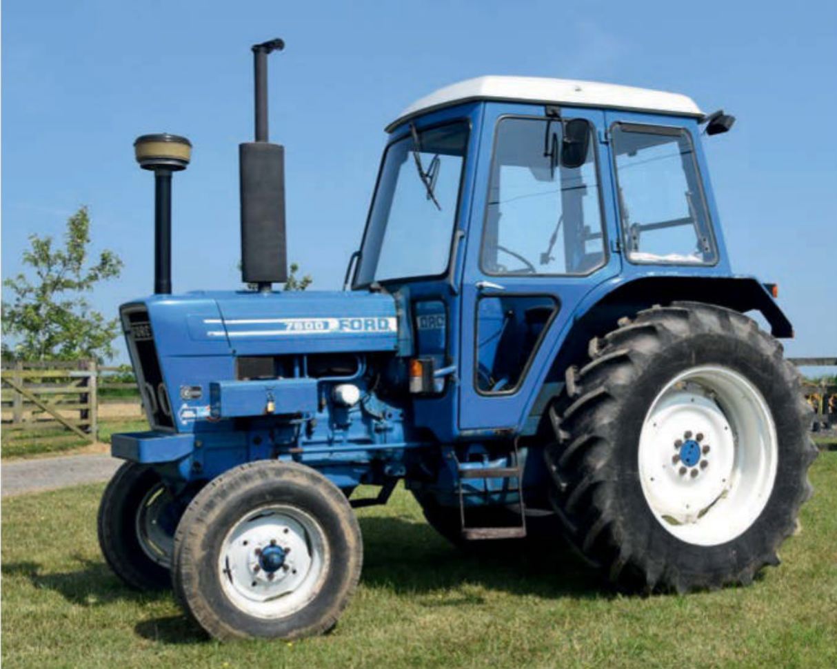
Early models like Dave's used a 4.2-litre engine delivering 96.7hp. A turbo provided most of the grunt.
