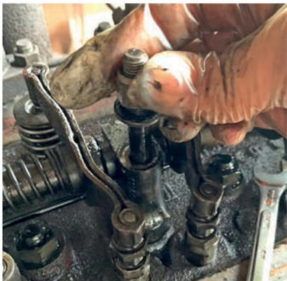
Removing the nuts on the rocker shaft signalled the start of this engine's strip-down.
