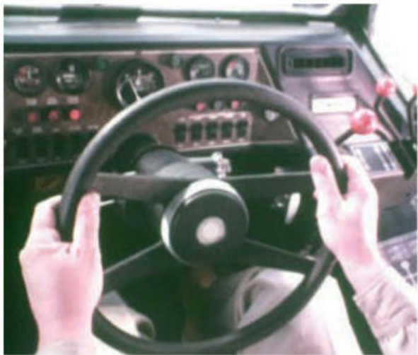
The steering wheel is fully adjustable, both in terms of tilt and height, giving car-like driving ergonomics. The instrumentation is uncluttered and easy to read.
