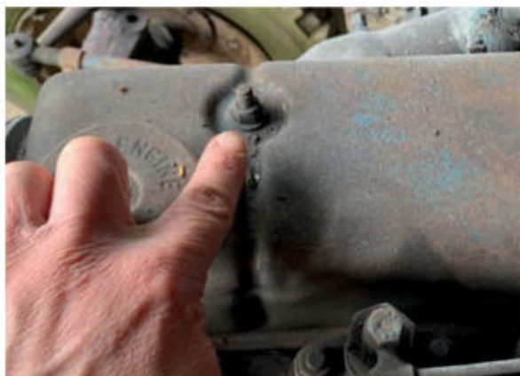
These two nuts on the rocker cover needed to be undone to remove the cover and reveal the top part of the engine.
