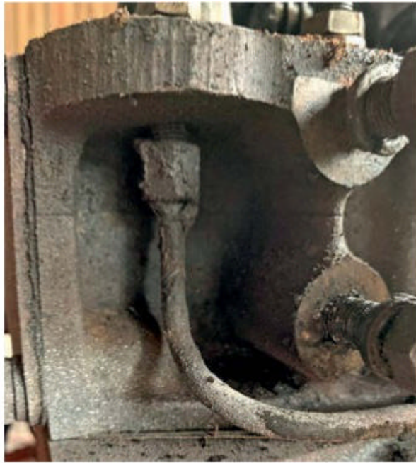
Once I'd undone that rocker shaft oil pipe, I followed the pipe down and removed this union, also.
