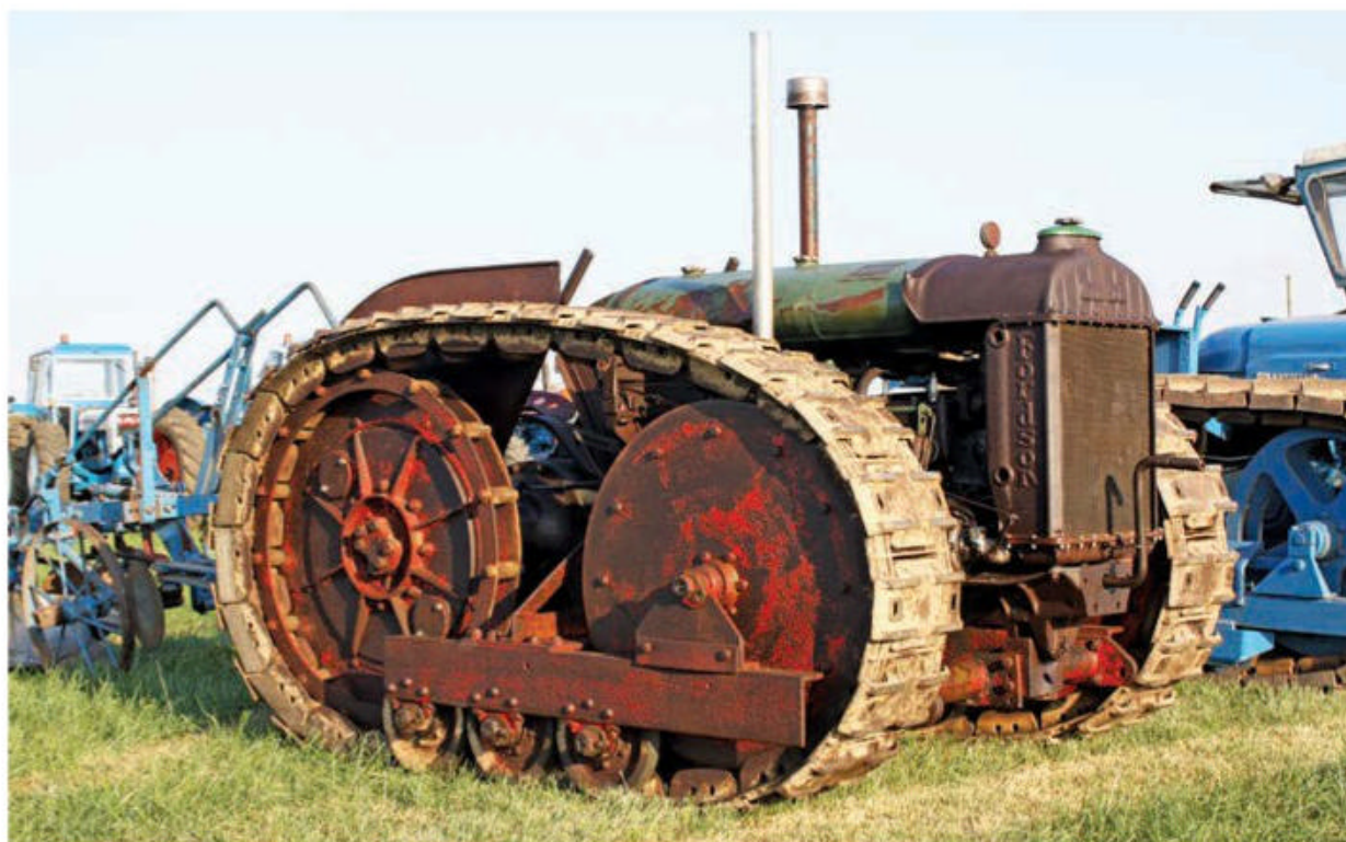
The Roadless Model N crawler was found to be unstable at speed, when in the hands of the military, during the run-up to WW2.
