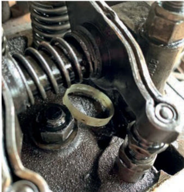
Someone had obviously lost the plastic collar from an oil bottle while topping-up. Luckily it wasn't able to travel far inside.
