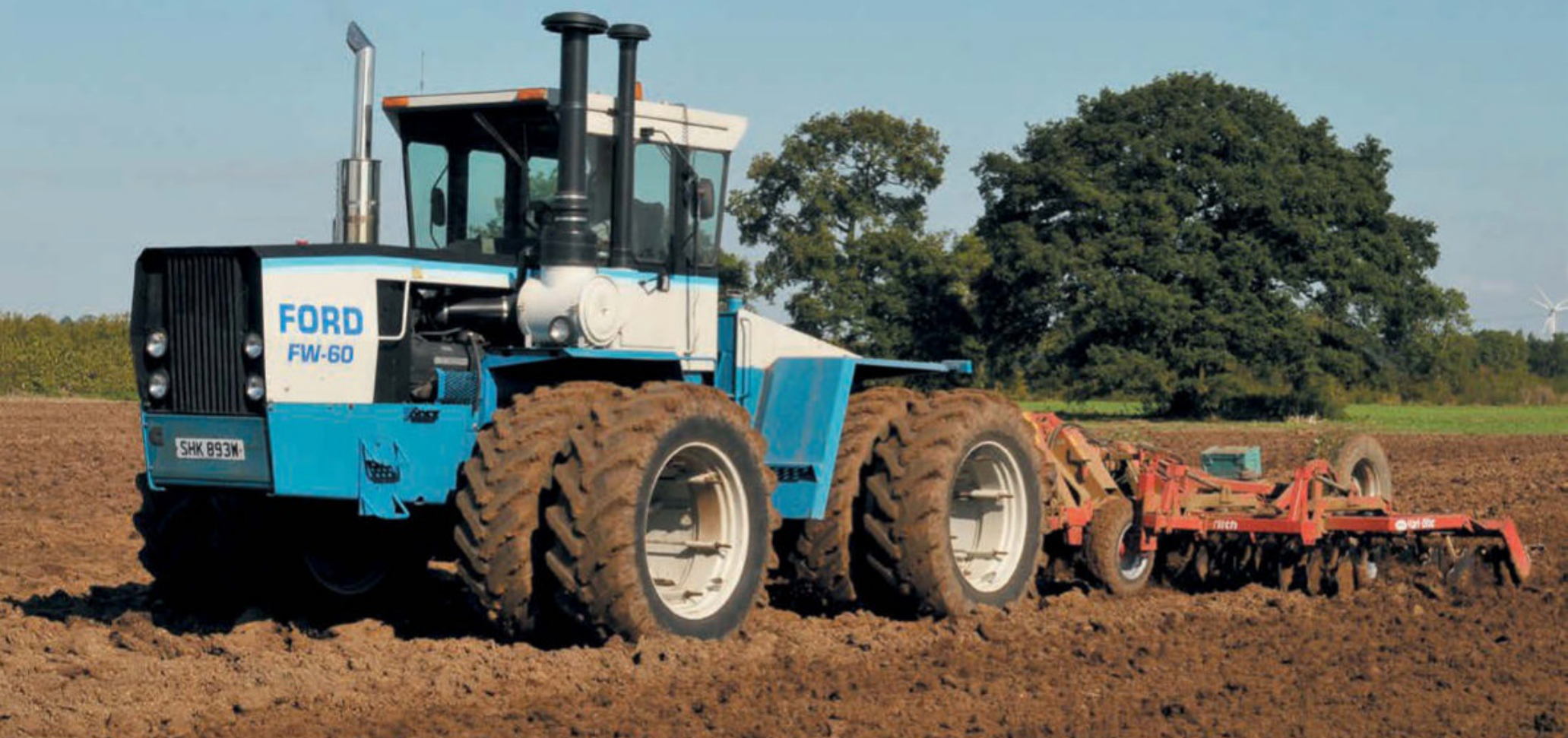
The range-topping FW-60 was an impressive beast, with 335hp on tap from its turbocharged V8 Cummins engine. This example was one of the first to be exported to the UK, and was the machine used in the publicity material for the UK launch.
