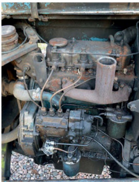
The Perkins engine ran but not smoothly, so I didn't leave it going for longer than was absolutely necessary. It will undergo a complete overhaul as part of the restoration.
