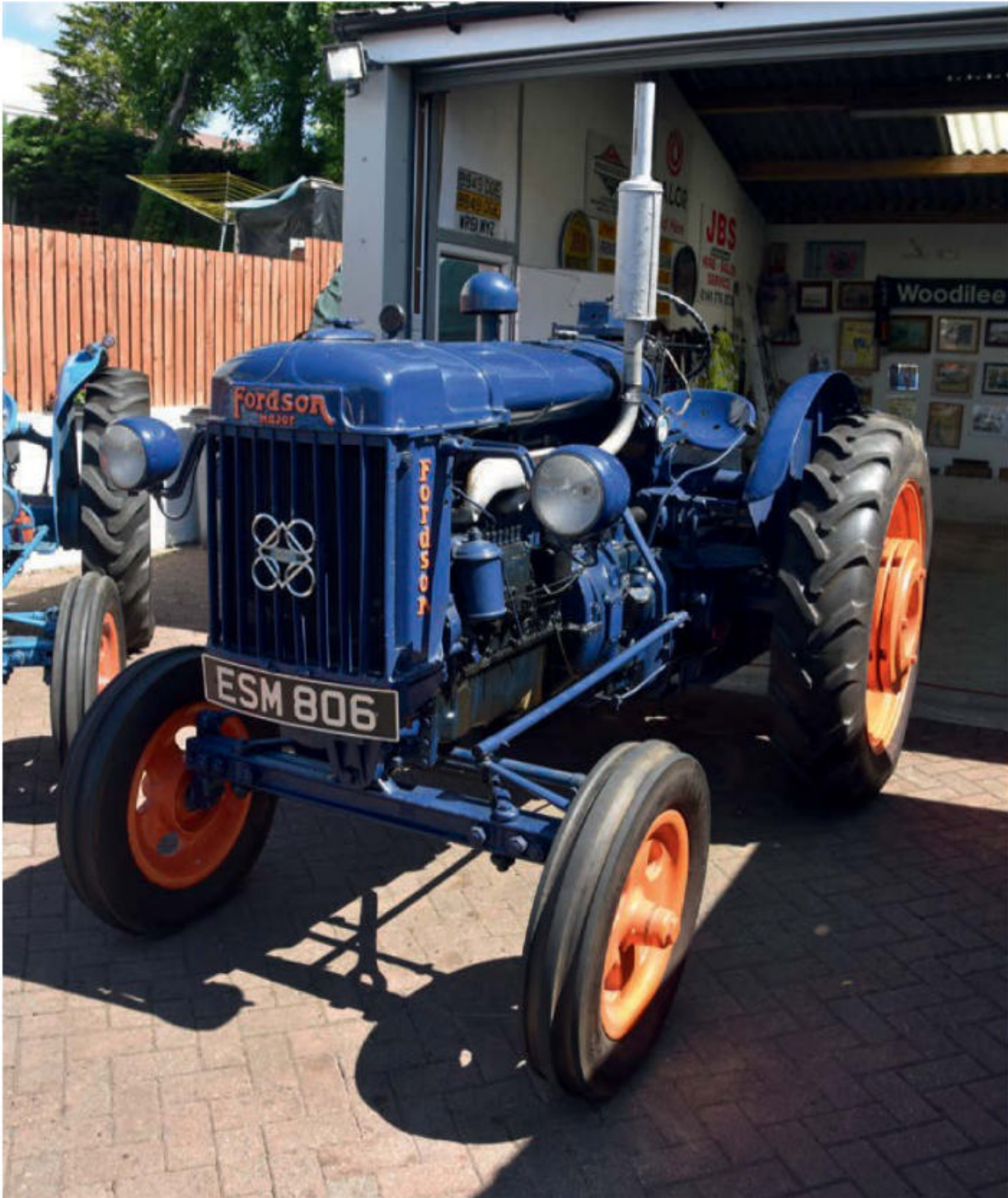
Early factory E27Ns all ran on petrol/paraffin and the venerable Fordson engine was underpowered and prone to wear and tear. Things changed when Ford came to an arrangement with Frank Perkins in 1950.
