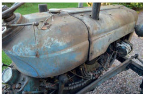
It was good to discover that the fuel tank and bonnet are in good condition. Note the string on the throttle lever, which is being used as a primitive way of regulating engine revs.
