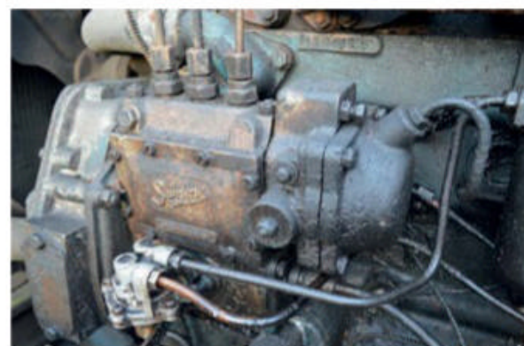
The Simms fuel injection pump will require specialist attention, as will the injectors themselves.
