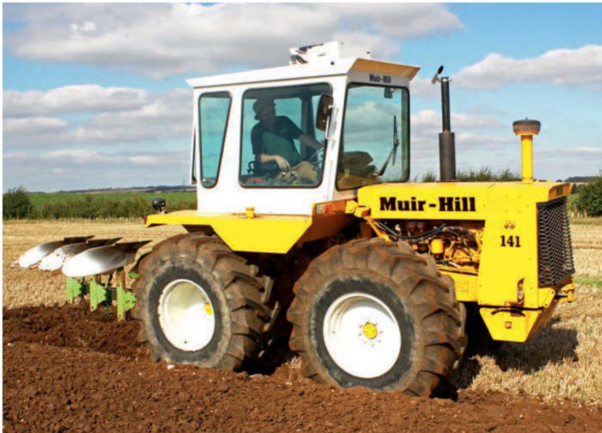
The new model introduced with the launch of the Series III range was the 141 which, uniquely, could be purchased with the choice of either a Ford or Perkins six-cylinder engine.
