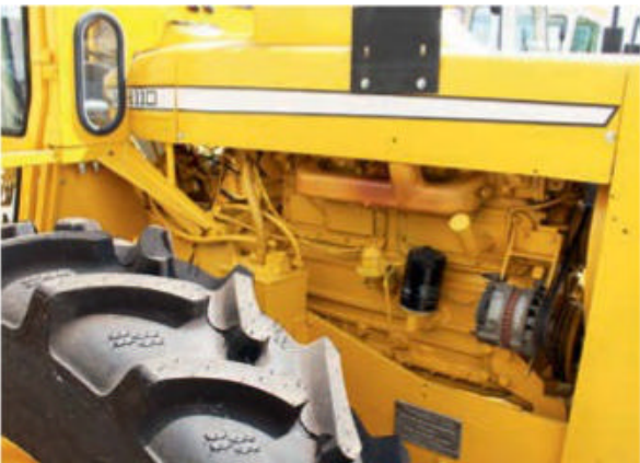
The 110's Perkins engine fitted easily into what was basically the 101 'chassis'. This made the 110 acceptable for many export markets, especially those growing sugar cane, where it proved to be an ideal prime-mover.
