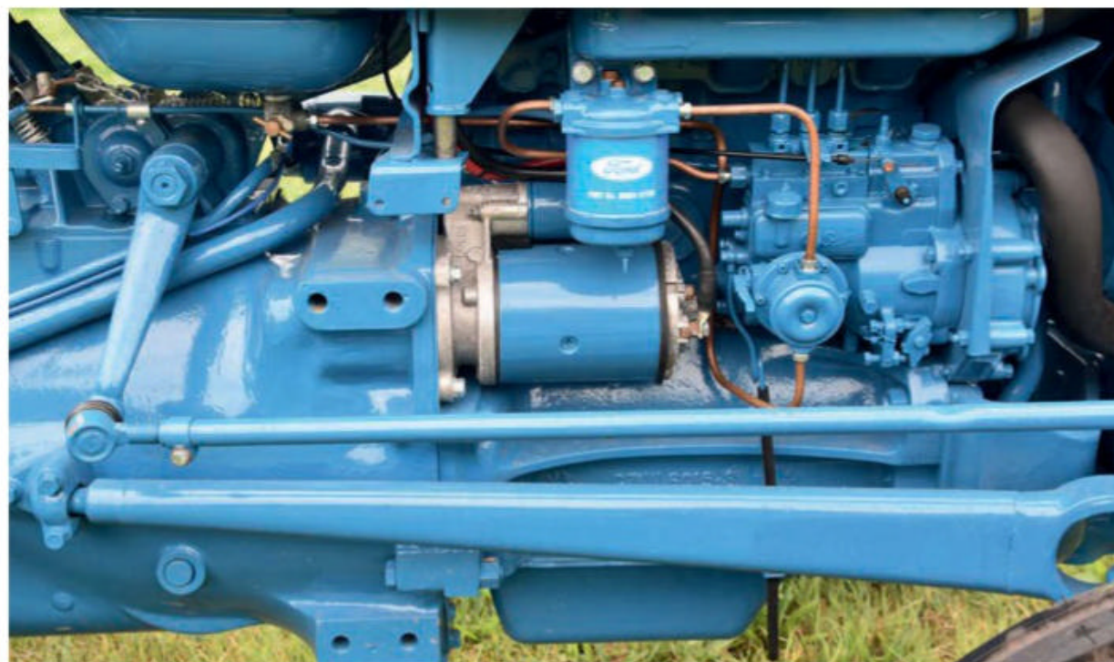
The three-cylinder engine that powered the 3000 was available with either petrol or diesel fuelling.
