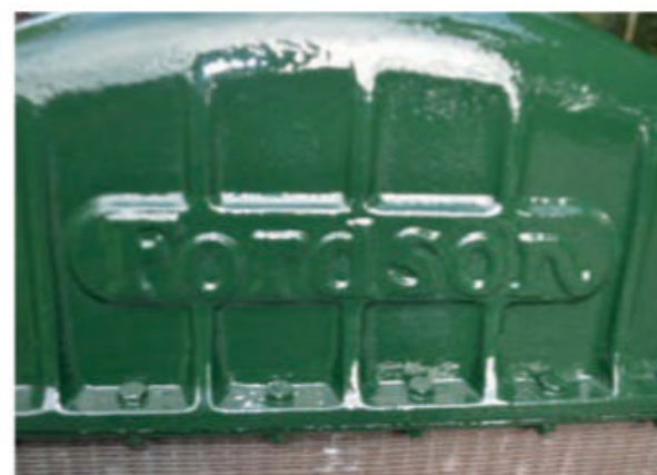
The same rule applied to the embossed 'Fordson' letters above the radiator. These were made more prominent thanks to the sandblasting.
