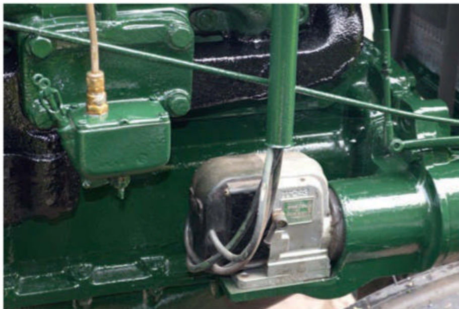
This Lucas SR4 magneto was sent away to a specialist company in northern England for complete refurbishment.
