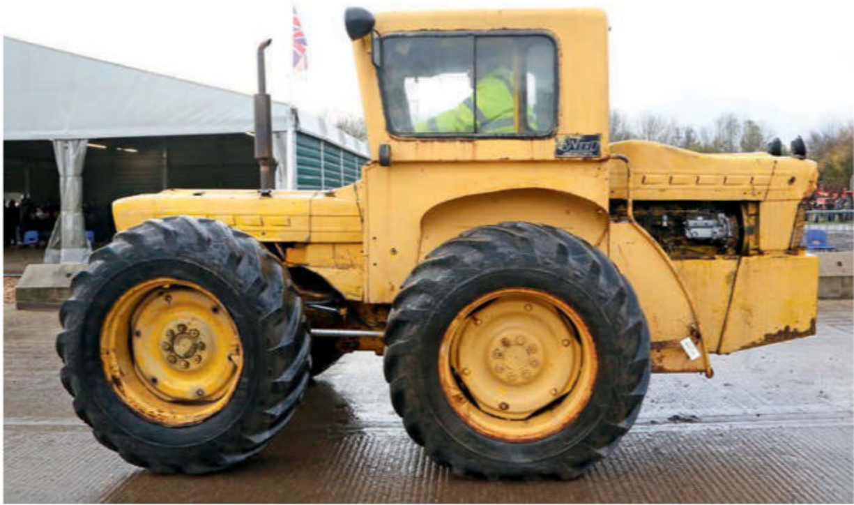
This twin-engined County Pre-Force 1004 spotted at Cheffins is certainly an unusual beast. It's clean for its age and the rear engine is offset to the right.
