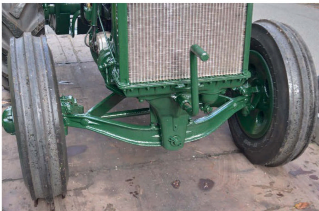
The front axle was specially made for this hop garden conversion. Close up, the detailing is lovely.
