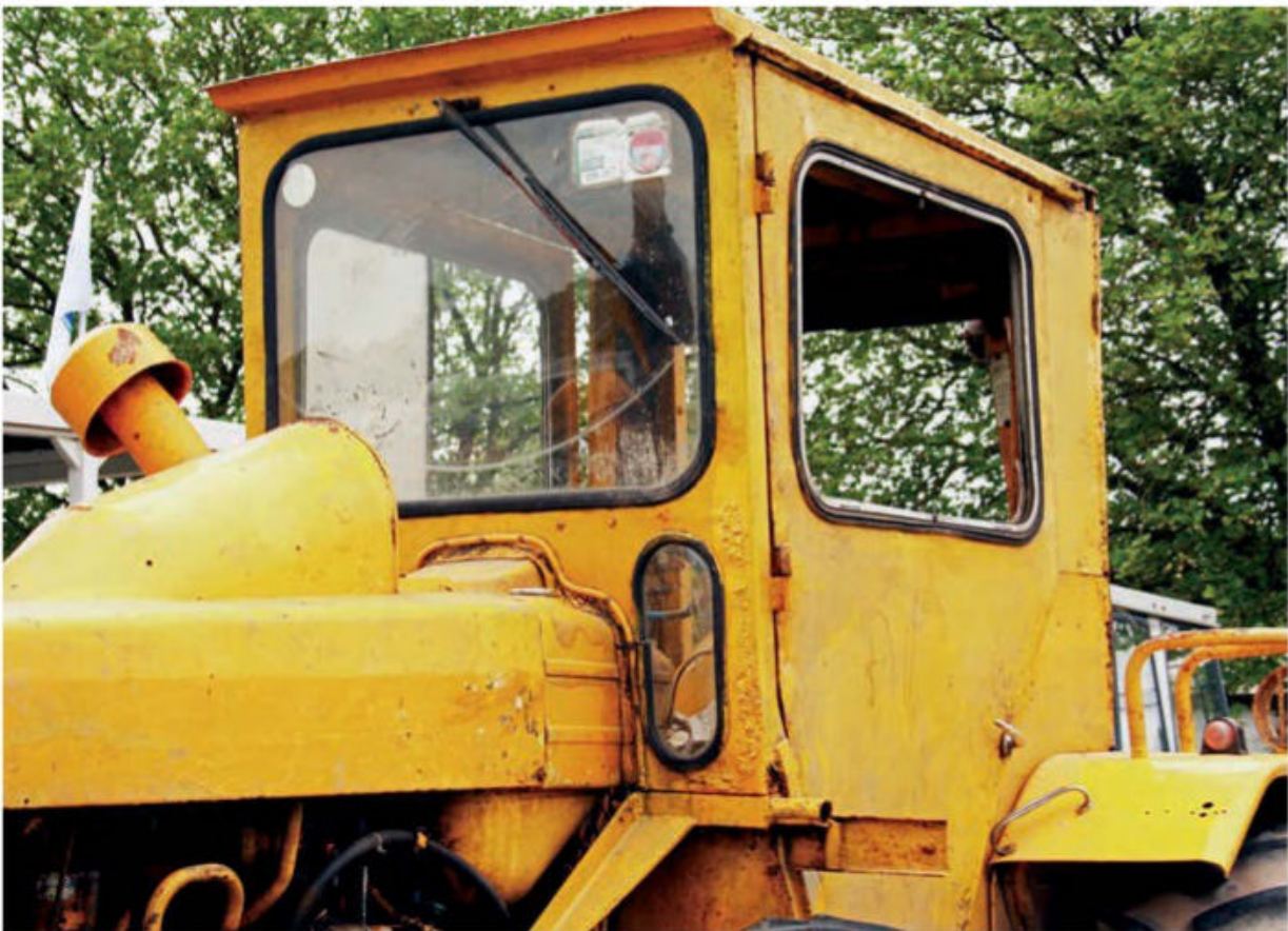
The Perkins engine required a 'hump' to protrude through the standard Muir-Hill bonnet to accommodate the air pre-cleaner and intake. This was the easiest way to tell the 101 and 110 apart at a distance, but it must also have hampered forward visibility – already fairly limited thanks to the design of the safety cab!
