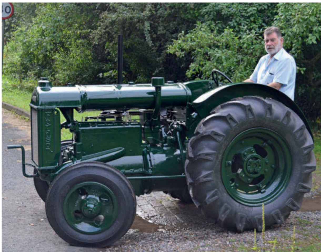
The shorter-than-normal wheelbase is obvious from this side view. It was achieved by the use of a different front axle.
