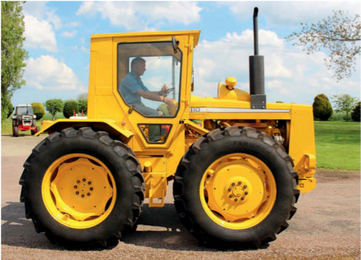
This restored 110 had its safety cab significantly altered by its previous owners – a circus! The much wider, glass-filled doors really helped to give much better visibility from the driving seat. Its current owners, the Riseborough brothers from Suffolk, still hate this cab though!
