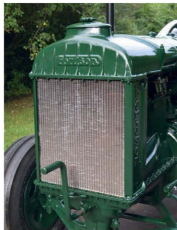
That new radiator core really did look good, and freshened-up the tractor's front end very effectively. The core is soft and easily damaged.
