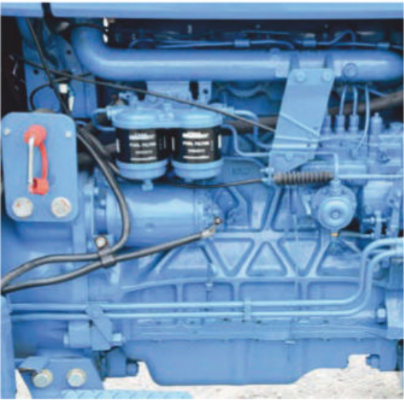
Ford’s 4.4-litre engine was used in the 6610, 6710, 7610 and 7710, with the two smaller models being naturally-aspirated. The 6710 and 7710 both had a longer wheelbase.
