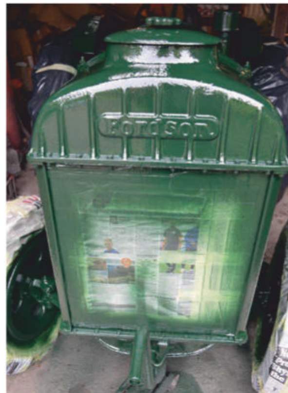
Careful masking-up is essential and always well worth the effort; it was vital to protect the brand new radiator core effectively from the overspray.
