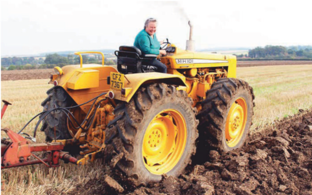
The rear end of the 101 came mostly from the 5000, although it was beefed-up somewhat to cope with larger and heavier implements, and the extra power from the bigger engine.
