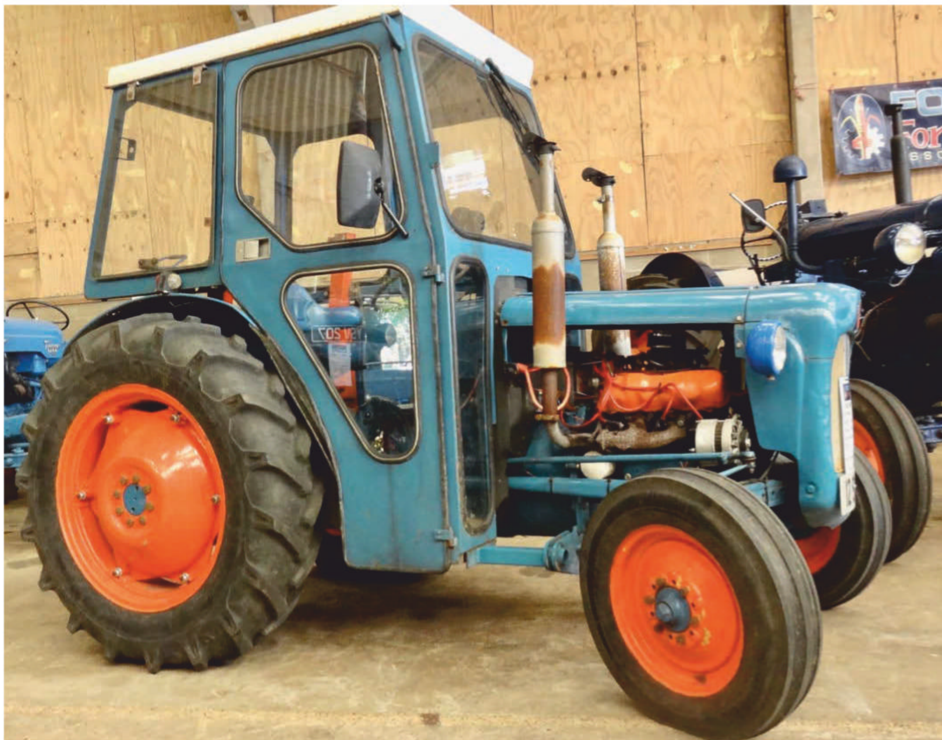
Ray Godwin's Dexta fitted with a Ford V6 2.8-litre petrol engine, at the Eastern Counties Vintage Show.
