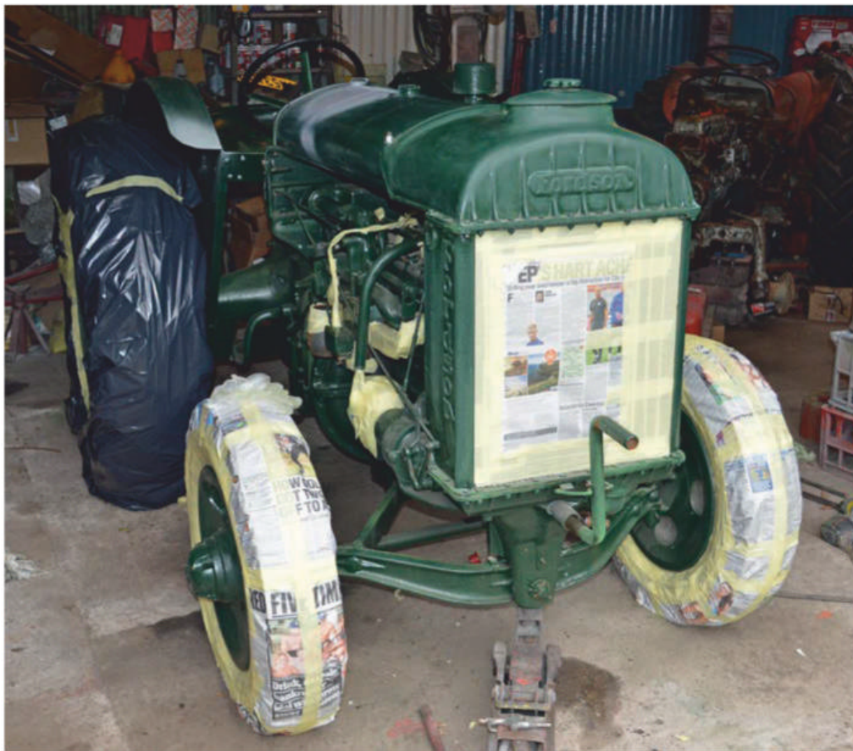
This photograph illustrates how much masking-up was required to cover everything that needed protecting before the final top coat was applied.
