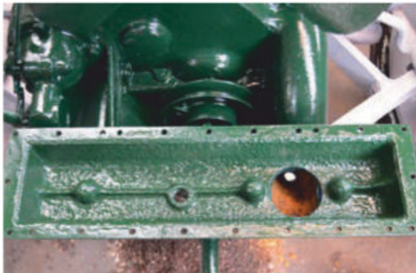
If you remember, this section had been replaced due to the corrosion in the original; it was like a colander in places!
