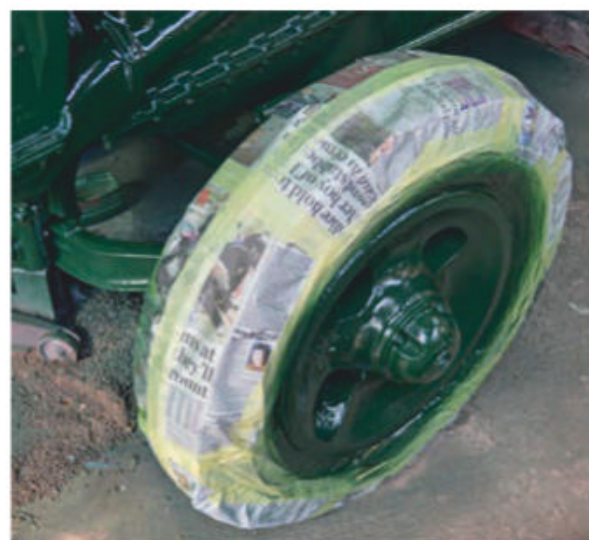
When it came to the paint being applied, I carefully masked-up the front tyres as they were new.
