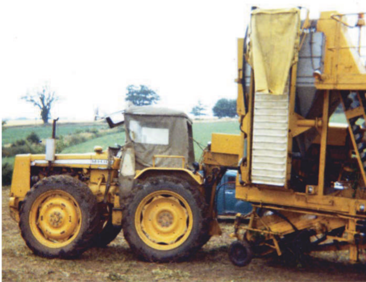
The over-engineered and very reliable front axle was designed and built by Muir-Hill, and was derived from that used on a new range of loading shovels introduced in 1965. This 101 was photographed in Norfolk during the 1970s, fitted with a Fritzmeier weather cab complete with opening front section. This European-built cab was often specified for the 101 before the advent of a safety cab in 1970. (Pic: Paul Reeve)
