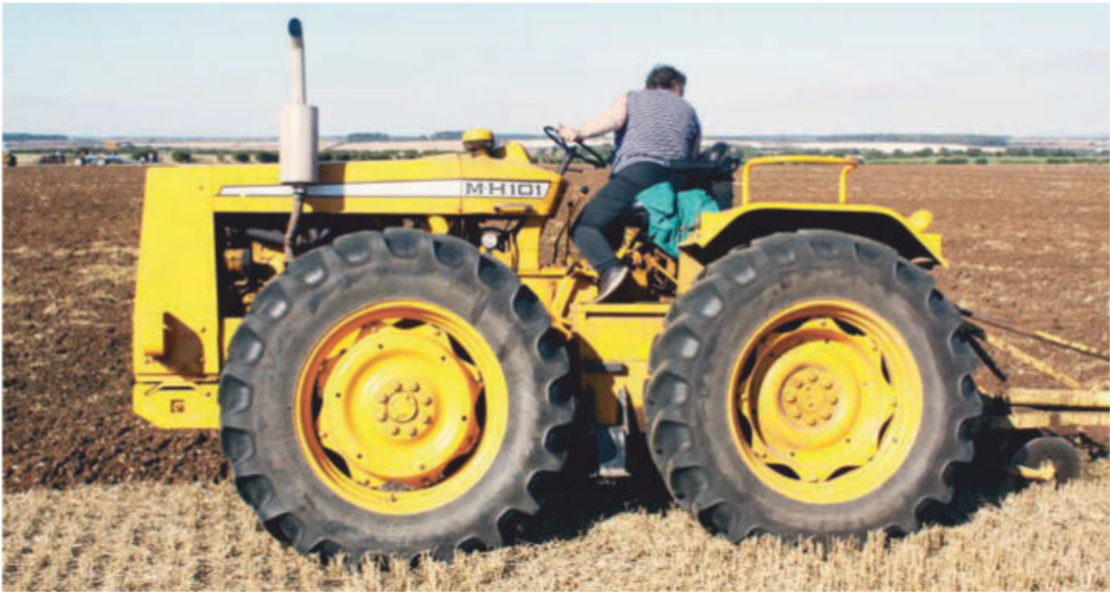
This view highlights the 101’s short wheelbase. A narrow step between the wheels helps the operator with access to and from the driving platform. The model featured a standard Ford eight-speed gearbox, with the control levers placed conventionally below the steering wheel. A drop box took the drive from the transmission then routed it equally to the front and rear axles.
