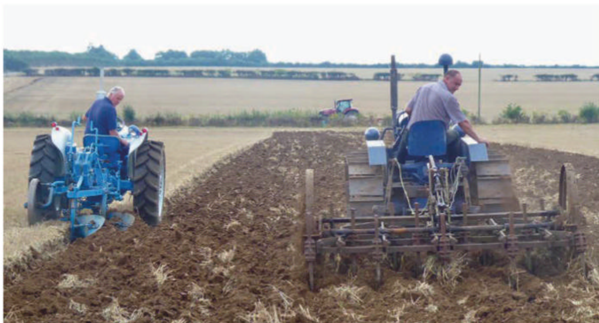
A P6-engined County full track pulling a drag; an ideal combination avoiding compaction.
