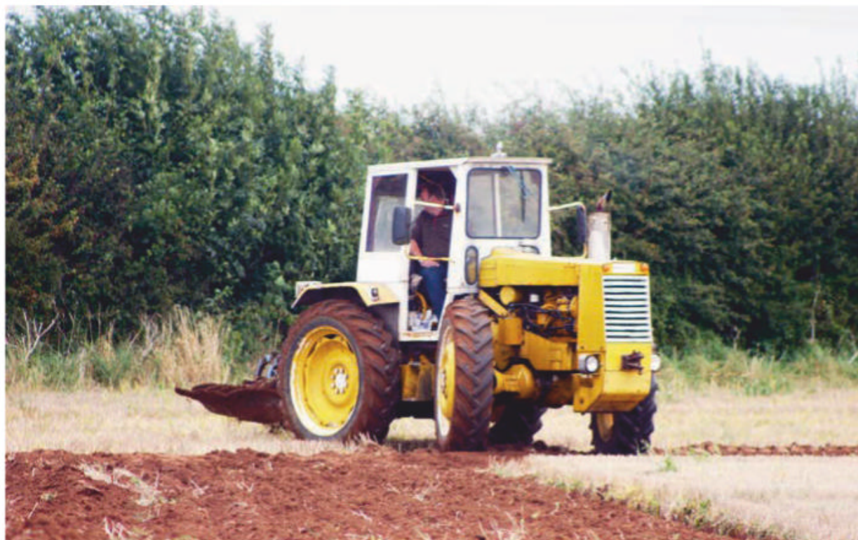
Some of the safety cabs were painted white, although most were yellow. This 101 demonstrates the excellent turning circle of its breed, as it manoeuvres on the headland while ploughing. Power-assisted steering was standard and definitely a necessity!
