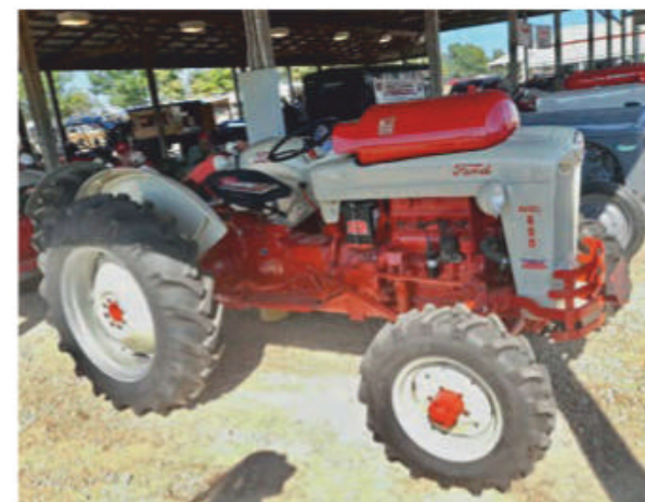
A Ford 600; this model's 'red tiger' engine was LPG-fuelled.
