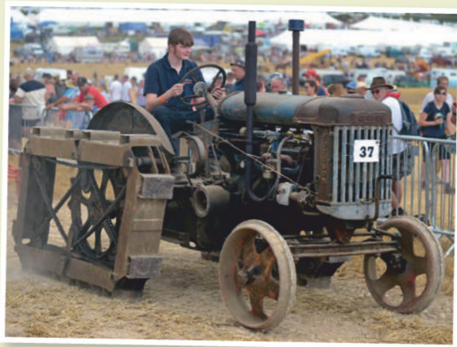
▲ This is Robert Jenkins' 1945 Fordson E27N Halftrack Rotopad. The unusual tracks are fitted in an effort to minimise ground compaction. The tractor is based in Nailsea, near Bristol.
