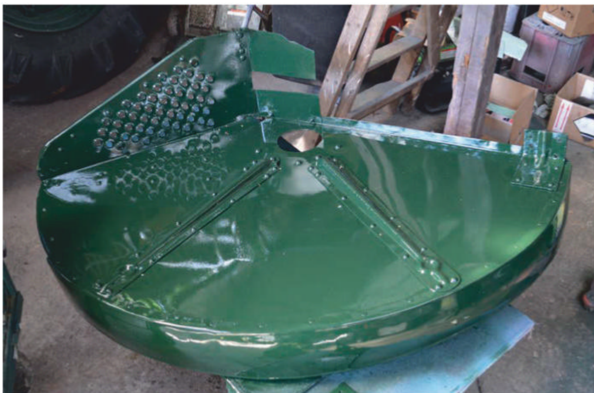
If you remember, this section had been replaced due to the corrosion in the original; it was like a colander in places!
