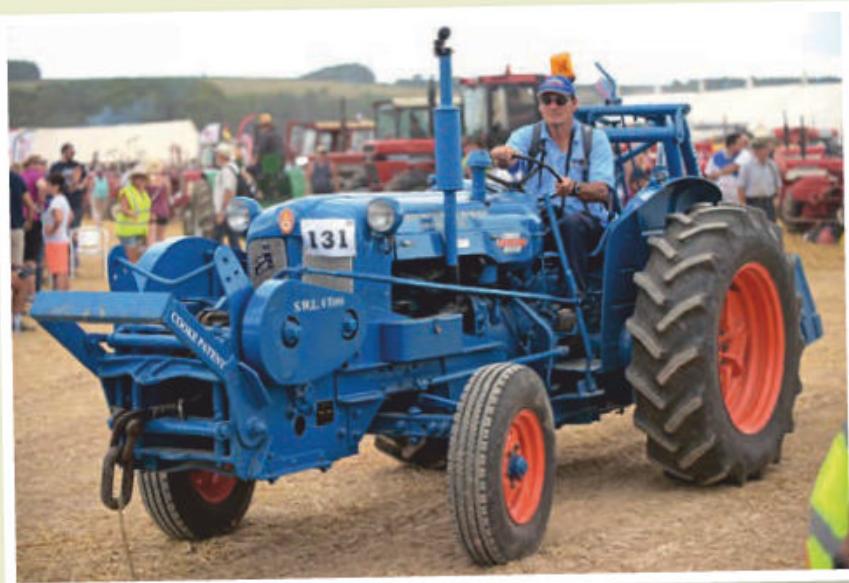
▲ This the the famous Sandbanks Ferry Power Major. Built in 1960, this Fordson was supplied new to F English of Bournemouth, for the Swanage Motor Road Ferry Company. It's fitted with a winch and a Cameron Gardner Rearloada for clearing sand and, today, is owned by Ian Prince from Ramsden Heath, Essex.
