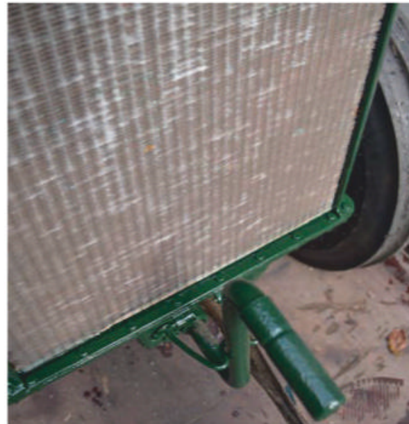
A new radiator core was fitted to the trough, with beautifully straight and dent-free fins.
