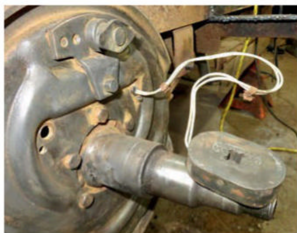
The electro-magnet that's at the heart of the electric braking system commonly used in North America.
