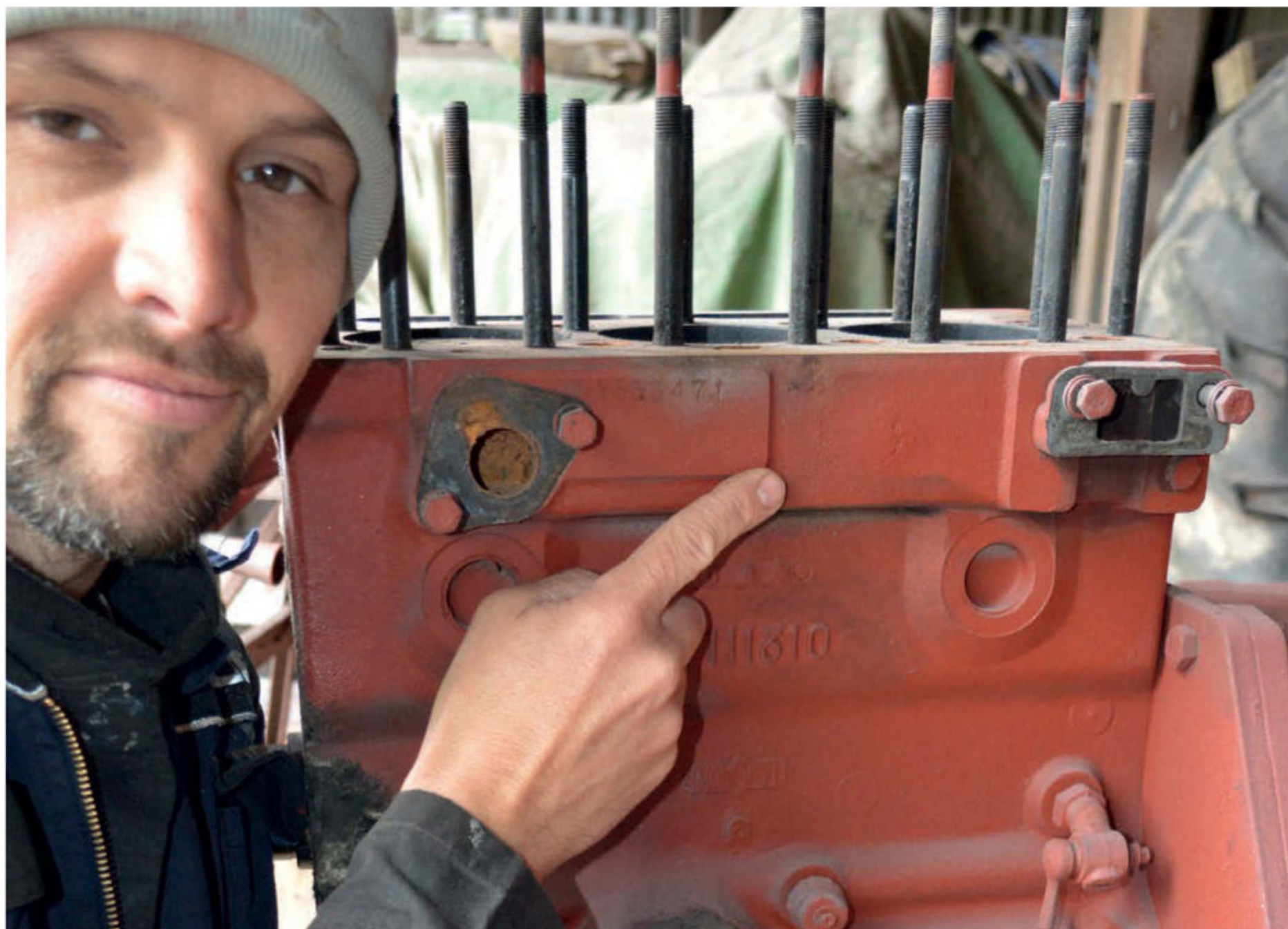
The engine came with the crankshaft already fitted, but these balance weights needed to be swapped over from the old engine.
