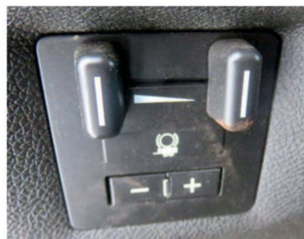
The factory-fitted control unit that's used to adjust the braking force to the trailer's load.
