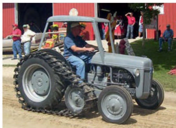
Here's a 9N with a rare, half-track conversion.
