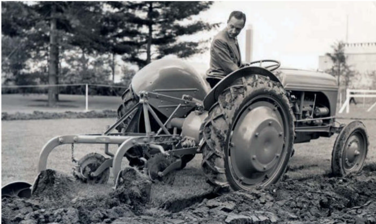
The 9N was powered by a Four, four-cylinder petrol engine that produced a fraction over 23hp.
