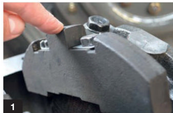
The engine came with the crankshaft already fitted, but these balance weights needed to be swapped over from the old engine.
