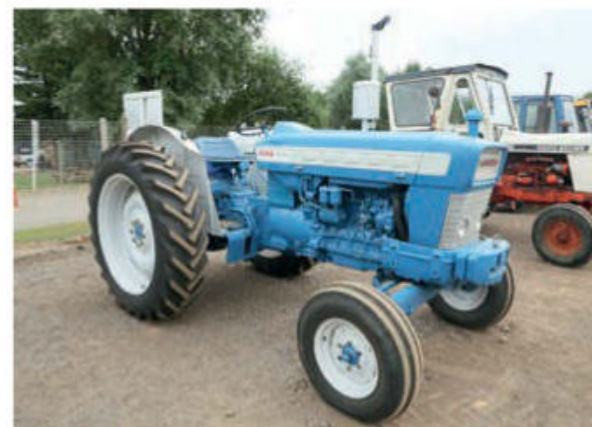
A nice looking Pre-Force 5000, but for the fact that it's fitted with a later engine.
