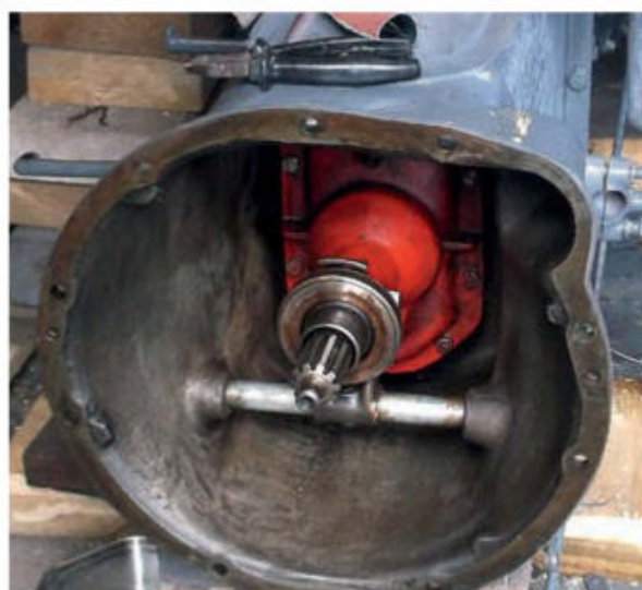
A dismantled gearbox showing the Hi-Lo conversion; a popular modification that boosted the practicality of the 9N's standard transmission.
