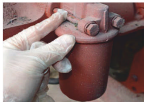
Knowing that the engine needed to be removed, I first stripped off most of what I could from the block, starting with this oil filter.
