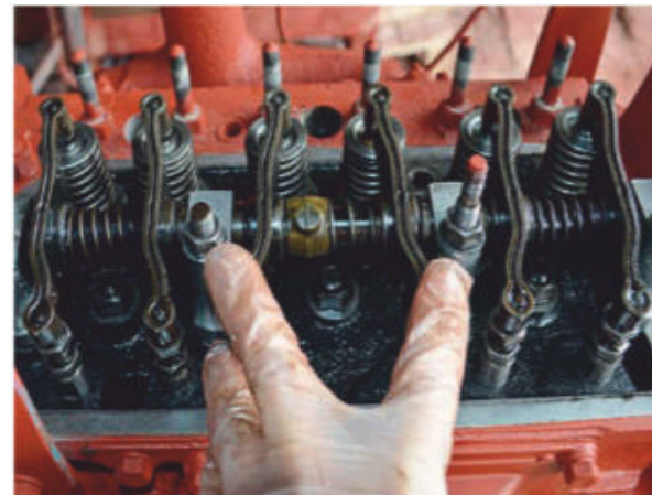
With the rocker cover removed, I could begin extracting the rocker shaft, by first undoing these four nuts.
