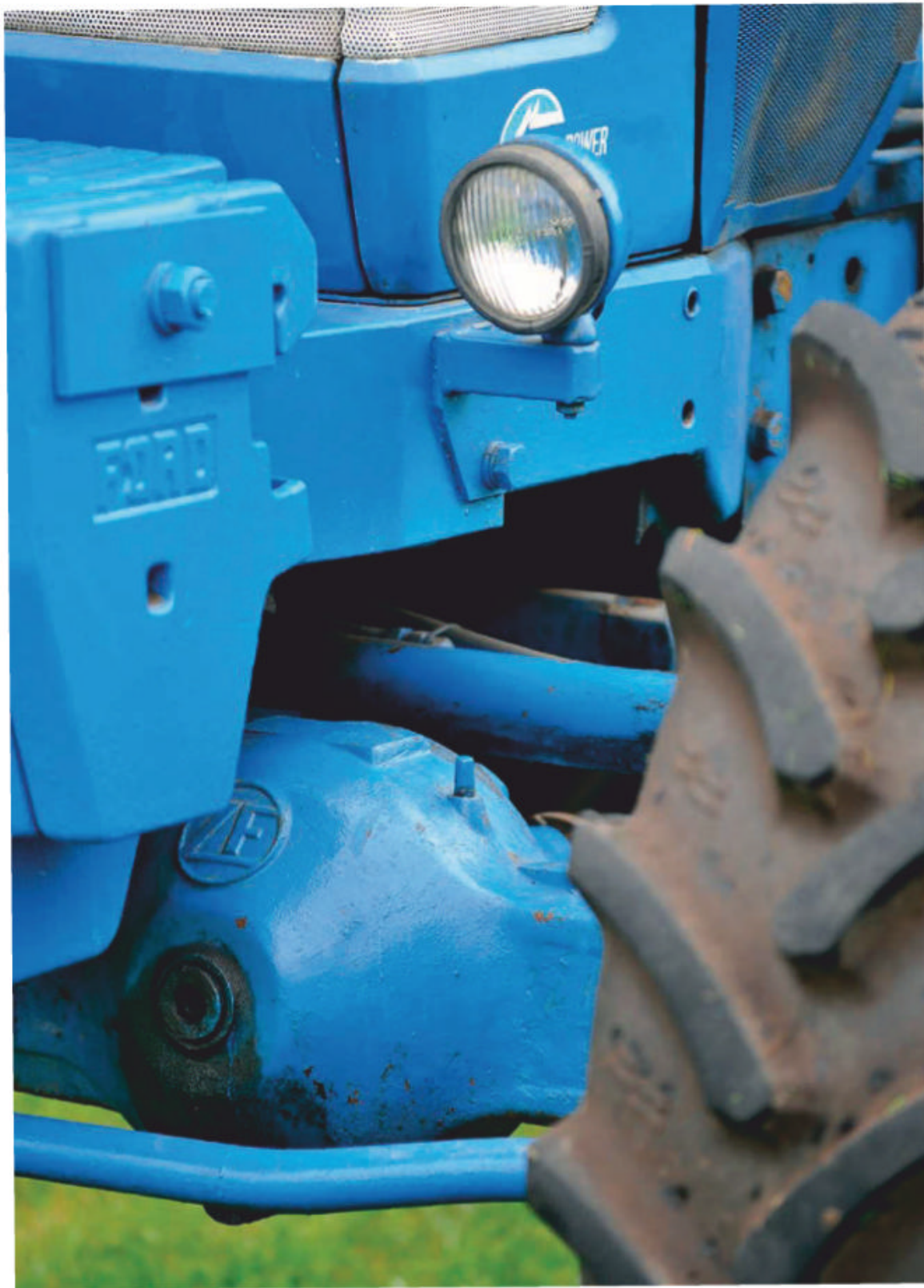
Ford opted for a front axle from German manufacturer ZF, powered by a side-mounted driveshaft.
