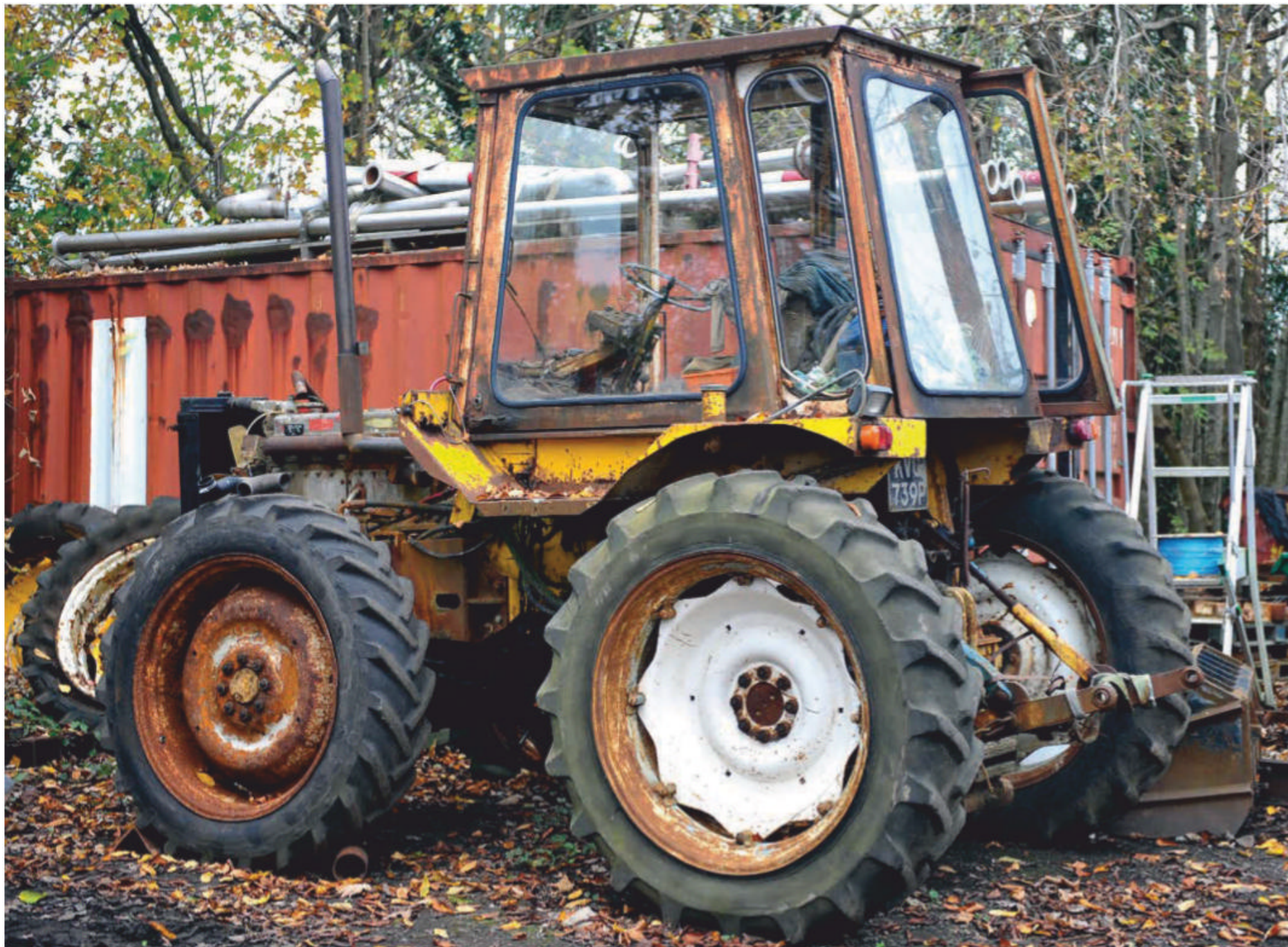
This 1975 Muir-Hill 121 has been fitted with a 180hp DAF truck engine at some point in the past. It's not currently roadworthy.
