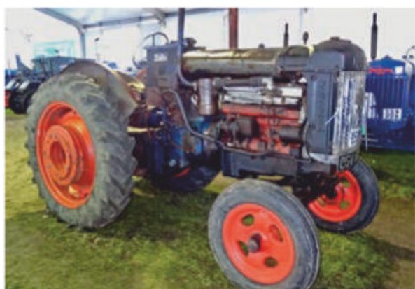
An E27N P6 that's different from the rest; this one has a 'Darlington' solid-axle drive, and is owned by Arthur Musk.
