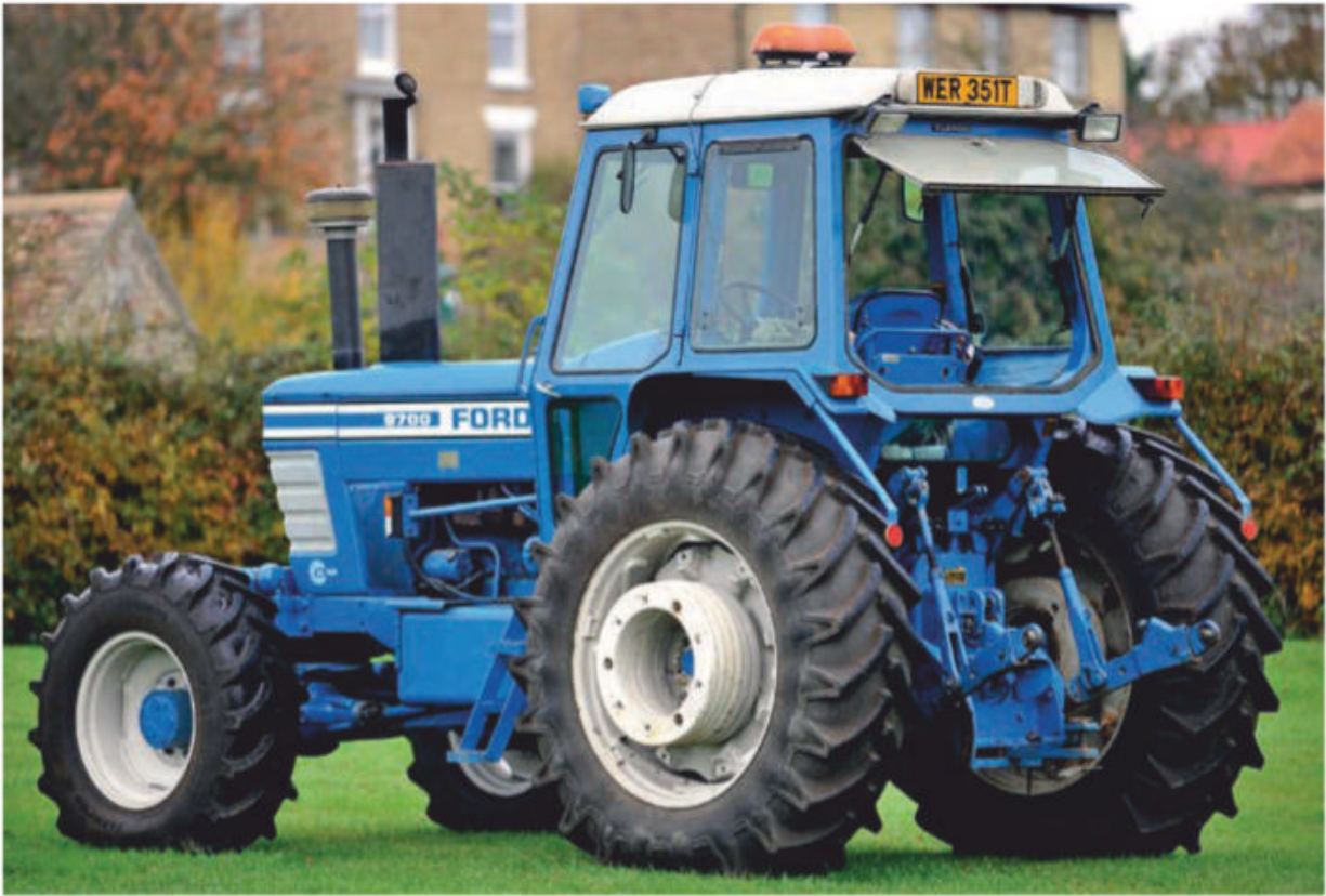
The 9700 operated a lower link sensing system, which wasn’t to everyone’s liking; Edwin isn’t a great fan of this set-up.
