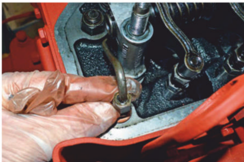
With the rocker cover removed, I could begin extracting the rocker shaft, by first undoing these four nuts.
