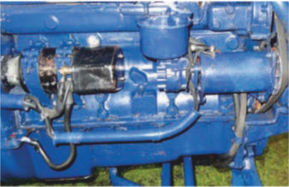
The neatest power steering pump that Phil Gibson's ever seen fitted to an E27N P6, owned by David Thomas.
