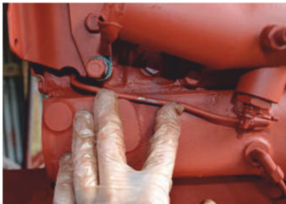
This Perkins-derived engine features a couple of 'hidden' oil pipes that are easy to overlook; this one by the inlet manifold is one of them.
