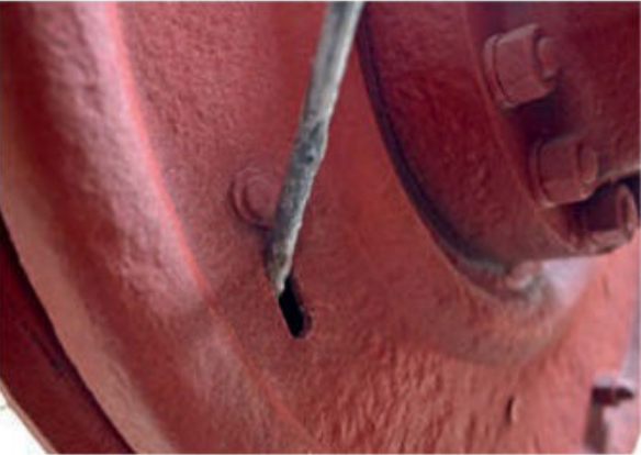
This groove on the backplate is for a screwdriver to fit into, so that the brake shoes can be adjusted. In this case, I'm slackening them off in preparation for removing the drum.
