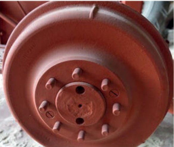
Most tractors of this age and size have drum brakes, and this is what's fitted to the Super Dexta. Always have a good look around the drum for signs of cracks.
