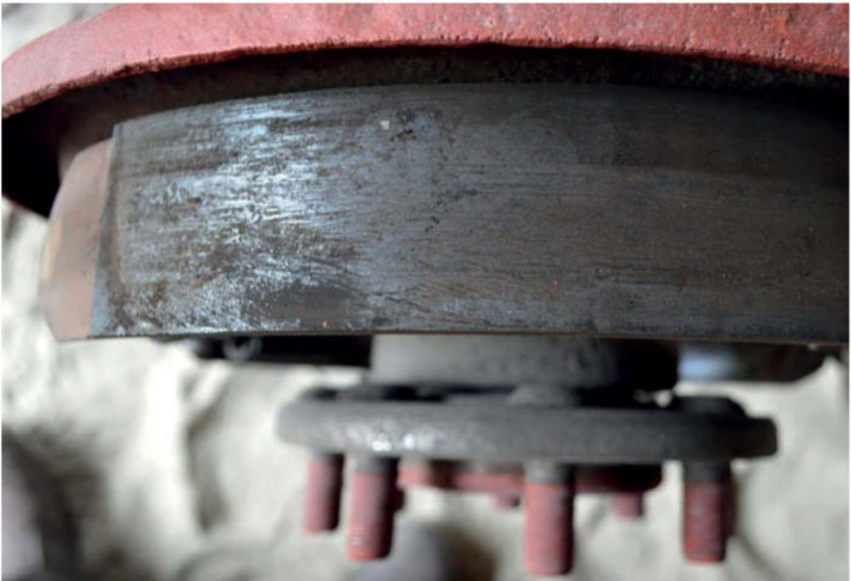
Once the drum was off, I could inspect the shoes which looked to be in good order; just a bit of dust that would be washed off with brake cleaner.
