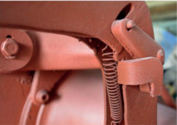
On the handbrake, this is part of the ratchet system; a spring and a toothed pawl are operated by the button at the end of the lever.
