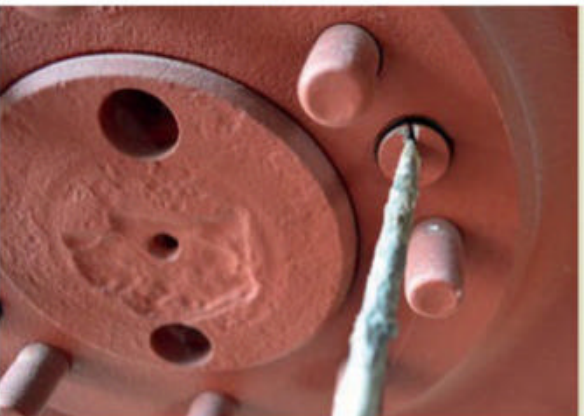
Although the wheels would hold the drum in place, these two countersunk screws are fitted so the drum doesn't drop off when the wheel is removed.
