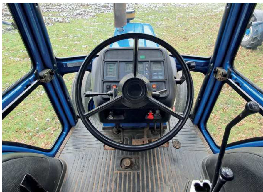
The flat cab floor allowed for conventional gear-change, which pleased operators. The 'digital' dash can be problematic, nowadays.
