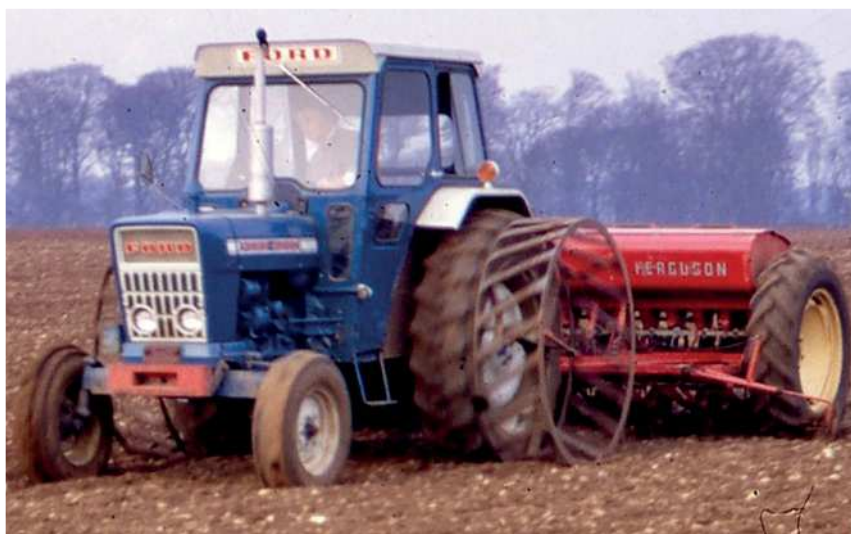
A Ford 4000 with a Massey Ferguson No. 29 combine drill sowing spring barley.
