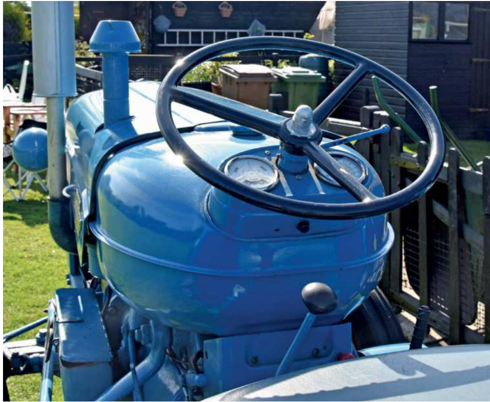
The Power Major's driving position is quite high, which gives the operator good, all-round visibility.
