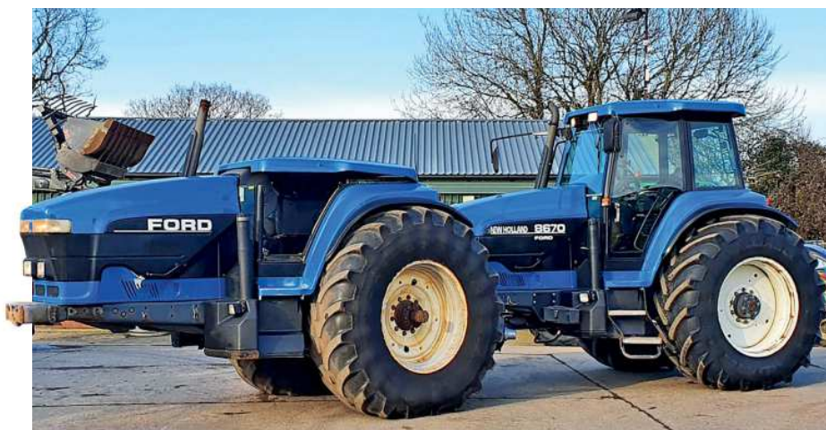
The interesting conversion carried out by Hertfordshire-based Oakfields Ag, marries a New Holland 8870 (front) with an 8670.
