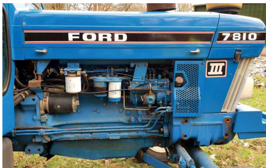
The 7810's six-cylinder, normally-aspirated, 100hp Ford engine is, essentially, bulletproof.
