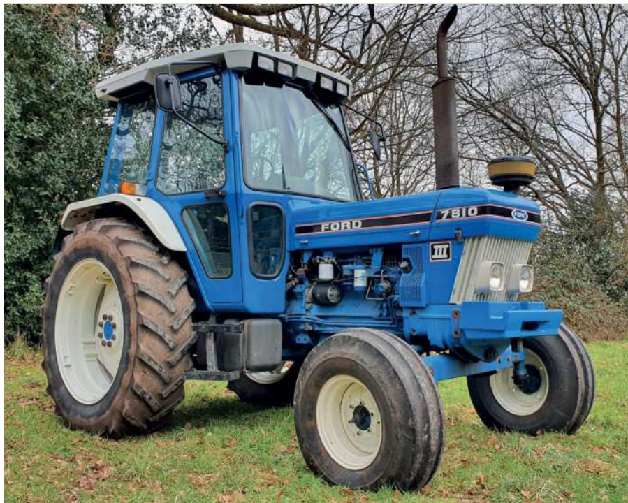
A two-wheel-drive 7810 Gen III; the 4WD variant was a much better seller back in the day which, nowadays, makes a 2WD like this one a rarer find.
