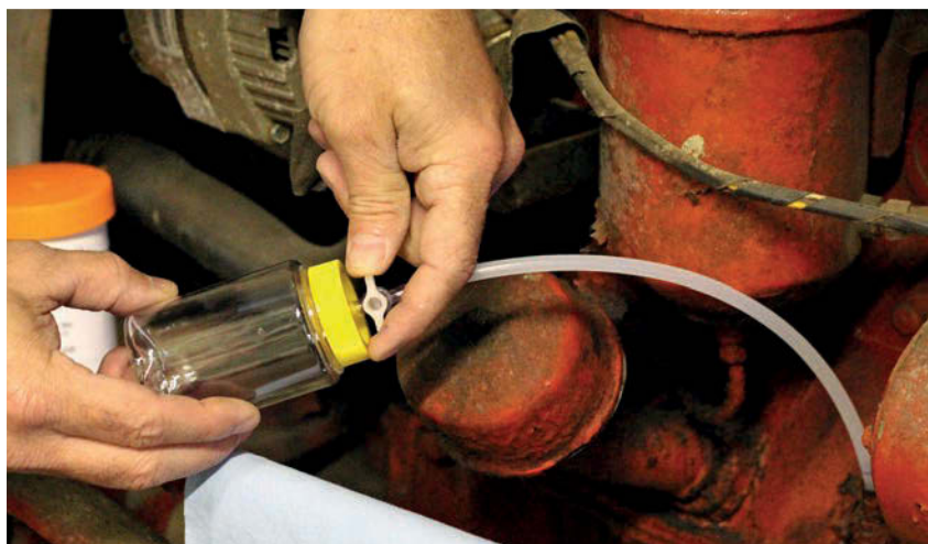
The pipe is fed down to the sump via the dipstick tube, to reach the engine oil. A tap on the vacuumed sampling syringe is then turned to draw out the required amount of engine oil.
