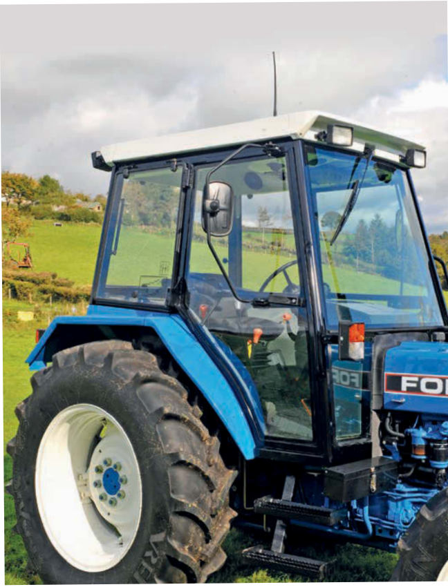
The cab took a lot of restoration; water leaks had caused it to rot from the inside out, and the roof panel was in a bad way, too.
