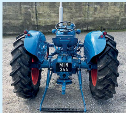
The back end underwent a lot of restoration work and, as you can see, the linkage bar still awaits its paint.
