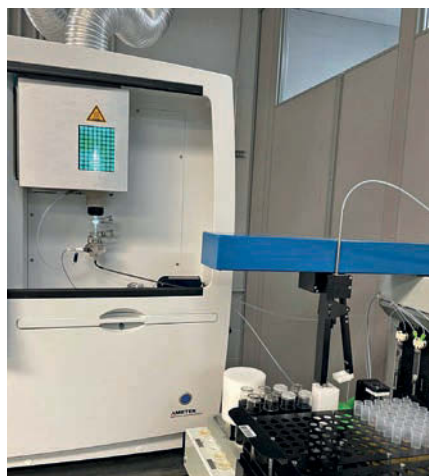
Testing at the laboratory is an efficient and thoroughly scientific process that records the precise concentrations of 20 metals, as well as the presence of water, fuel and coolant additives, plus the oil's viscosity and soot contamination.
