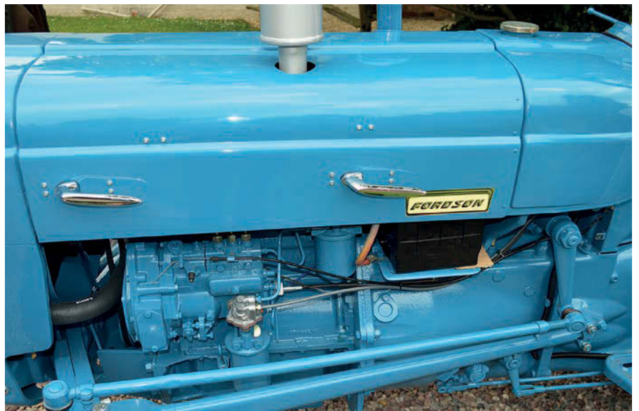
The Perkins engine was extensively rebuilt, and the Simms injector pump seen here was refurbished. I always enjoy the look of shiny, chrome parts. The chunky, bonnet catches really feel great, and look the part, too.
