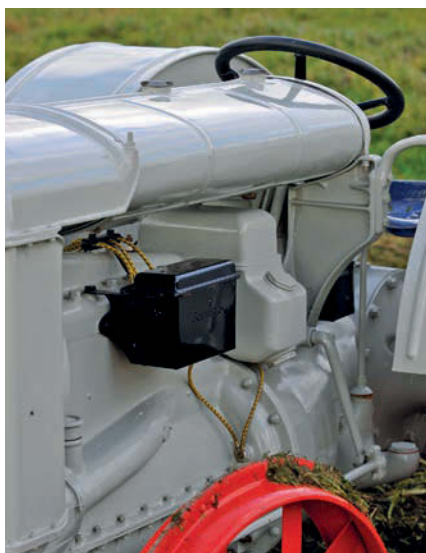
From 1920 onwards, a Ford-made four-cylinder engine replaced the original Hercules unit. Both produced 20hp. The black box on the side of the engine contains the four trembler coils.
