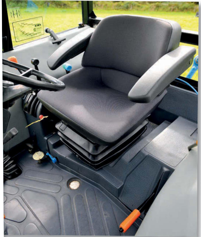
The seat looks standard but, beneath the surface there lurks an air-suspension system that delivers much greater comfort for the driver. Enhanced sound-deadening makes it quieter inside, as well.
