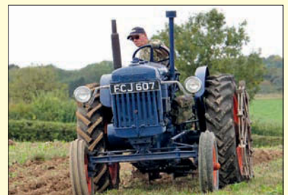
The Divall wheel on the n/s/r of the Fordson E27N wasn't needed here with fine ground conditions underneath.
