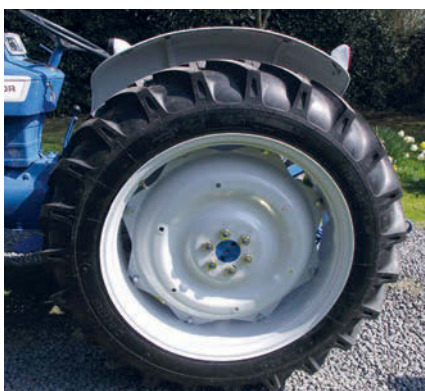
The Ford design feature a single, solid centre dish; the rims were 36in in diameter, which is 4in larger than those on the 165.
