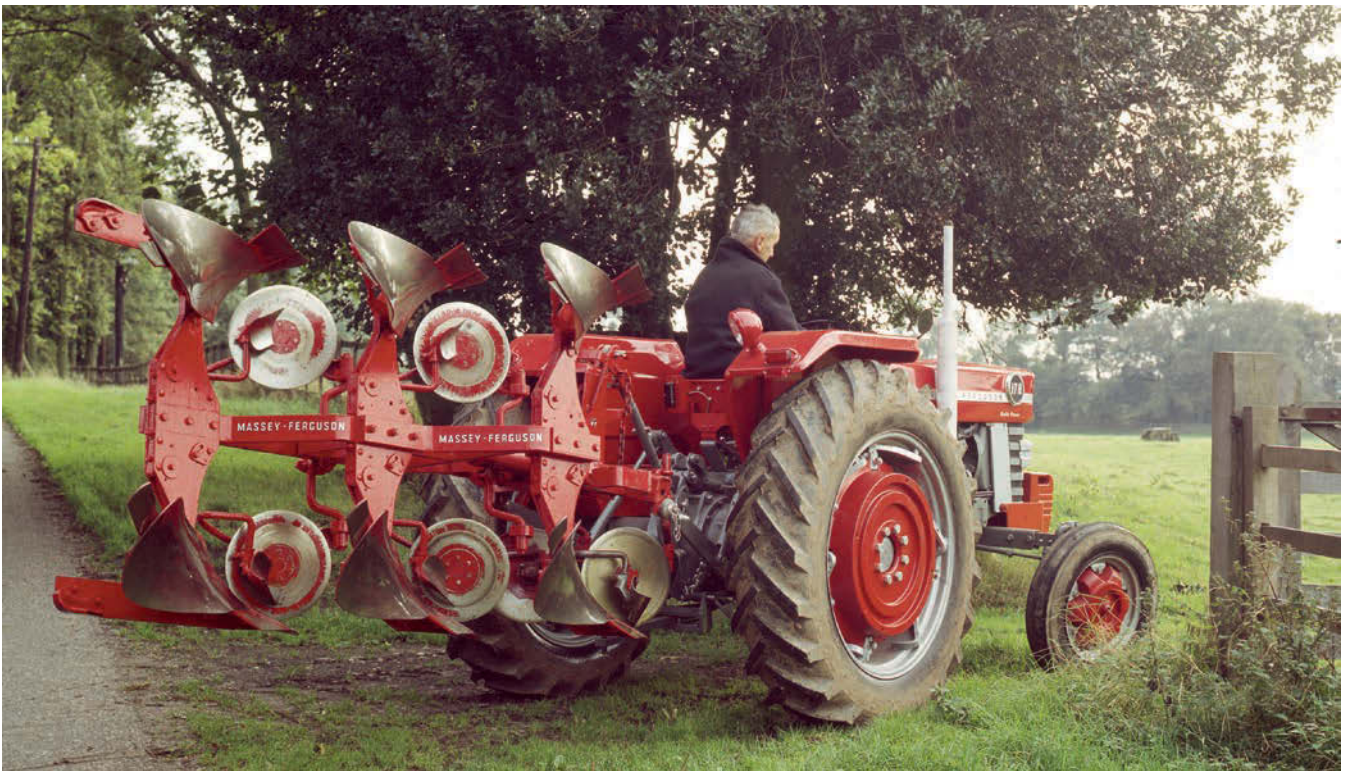
The MF 85 three-furrow reversible was a heavy plough, weighing in at approximately 1,500lb. Fitted with 'N' digger bases, it was designed to plough at a depth of 12in. (Pic: AGCO)
