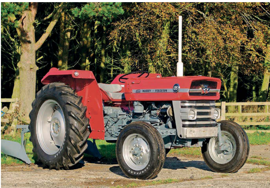
The Massey Ferguson 135 was fitted with the Perkins AD3.152 power unit. (Pic: Alan Barnes)
