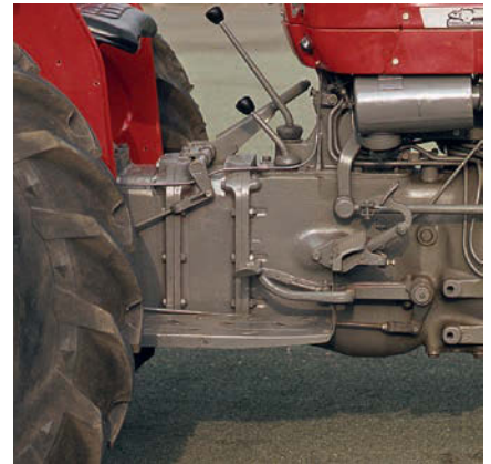
The six-inch transmission spacer was one of the Super-Spec models' most noticeable features, providing more room for the driver, better access and improved weight distribution. (Pic: AGCO)
