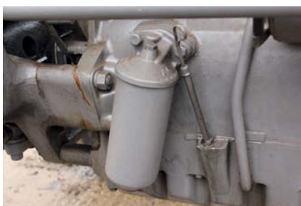
All MF 178 tractors featured a replacement element-type engine oil filter canister from the factory.
