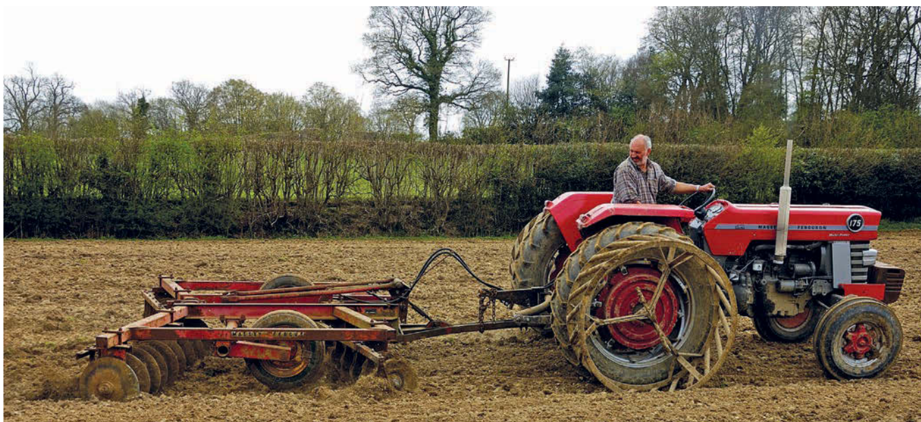
Graham Fellows' tractor is equipped with Pressure Control which, when used in conjunction with the coupler, can aid traction significantly.
