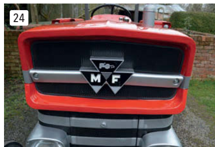
The upper grille and badge bar is typically damaged so often needs replacing; the rubber strip around the edge is essential.
