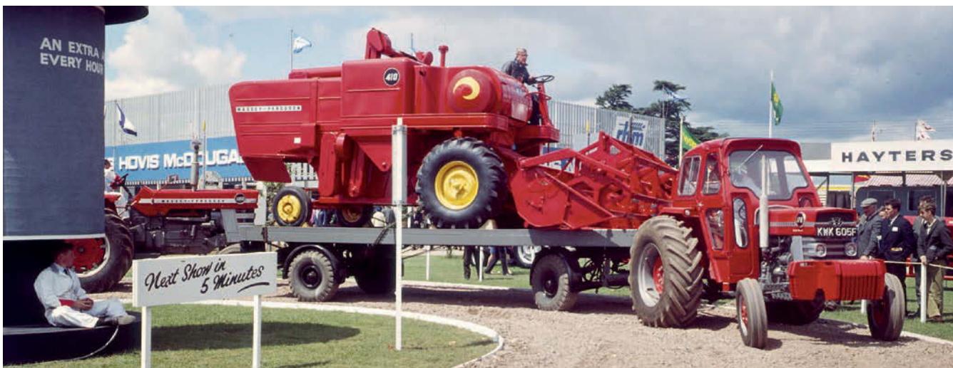
Fitted with the optional cab, costing £74 (1968), and wider rear tyres, this 178 is demonstrating the usefulness of Pressure Control. Note the front weights. (Pic: AGCO)
