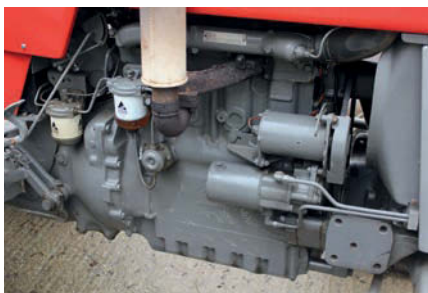
The right-hand side of the Perkins A4.248 engine, which looks identical to the A4.236 lump used in the MF 175.
