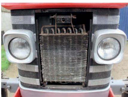
Multi-Power models feature an oil cooler immediately behind the grille door – check for leaks here.
