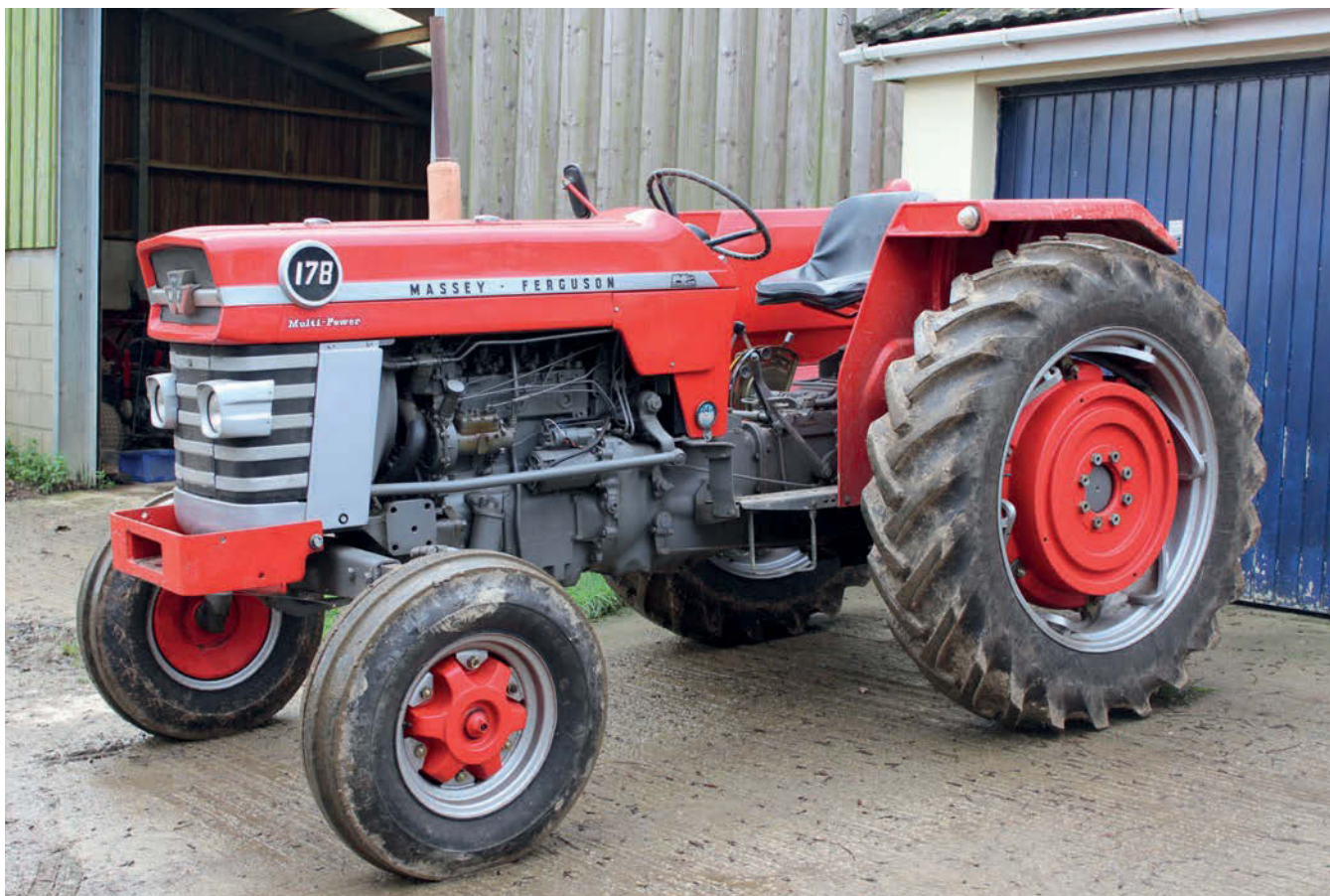
The MF 178 is an imposing, 72.5hp machine when fitted with cast iron wheel centres.
