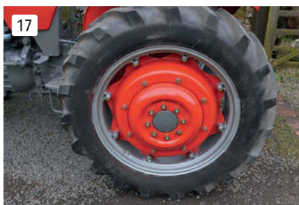
The silver rims contrasting with the red centres make for a perfect colour combination. The rears were re-assembled with all new bolts and nuts.
