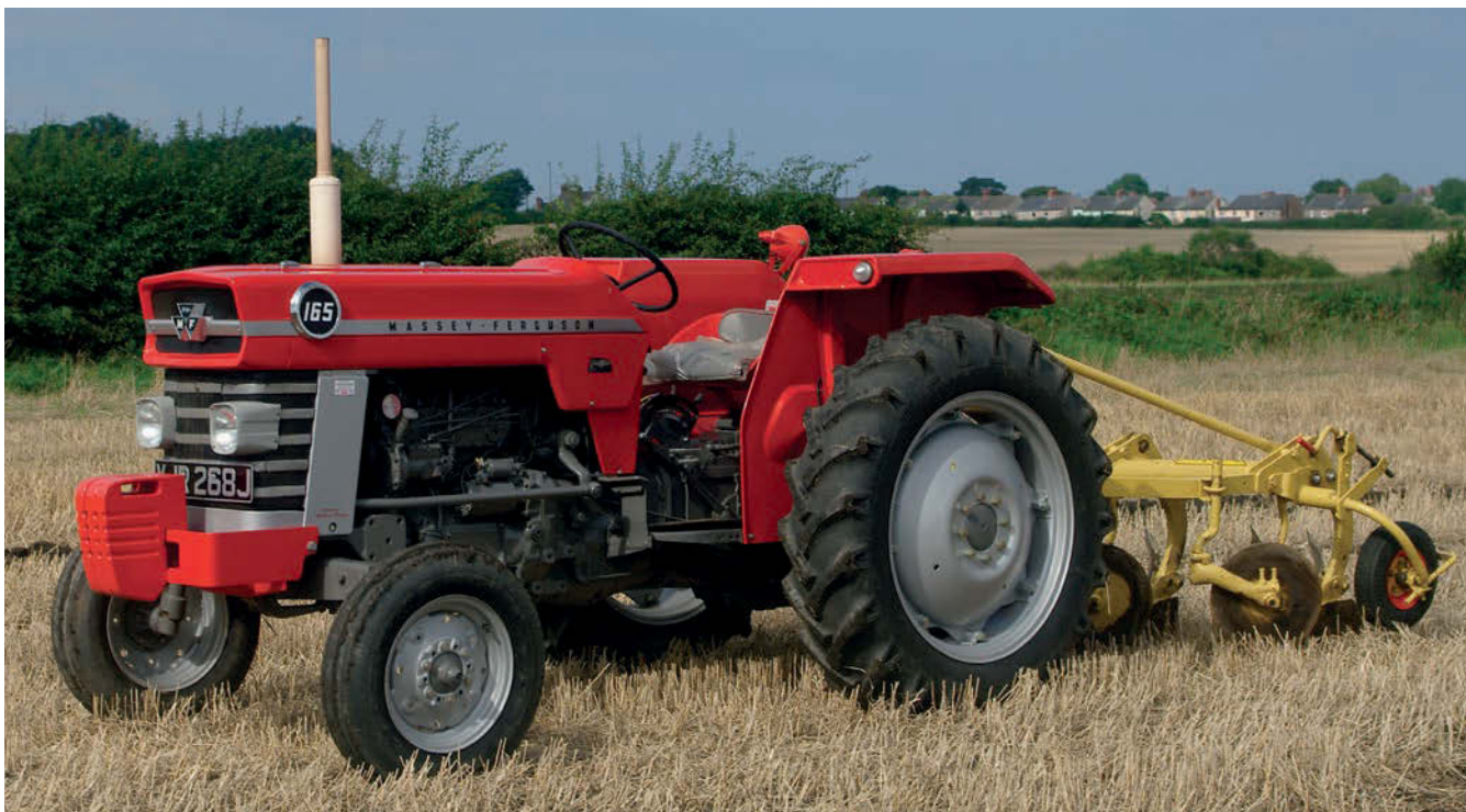
The MF 165 was fitted with the four-cylinder Perkins AD4.203 diesel engine and a choice of the standard six-speed gearbox or a Multi-Power transmission. (Pic: Alan Barnes)
