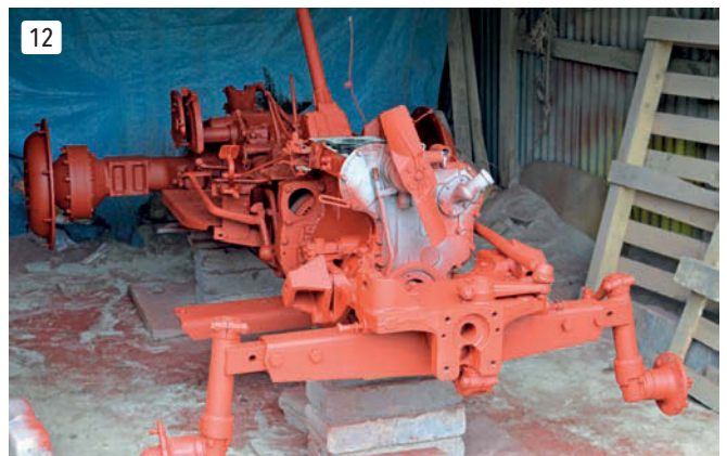
This shows how far a tractor needs to be stripped down before it's ready for sand-blasting. In fact, even more stripping was to follow, as the engine fitted was scrap... but that's another story!
