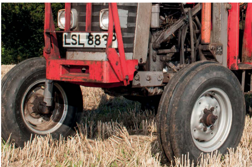
The heavy-duty, 'three-bolt' front axle and 7.5in front rims were upgrades on the 165's spec.
