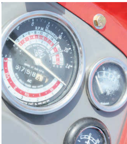
The hours total on the 188 is 6,758; only the amp meter gauge has been replaced.
