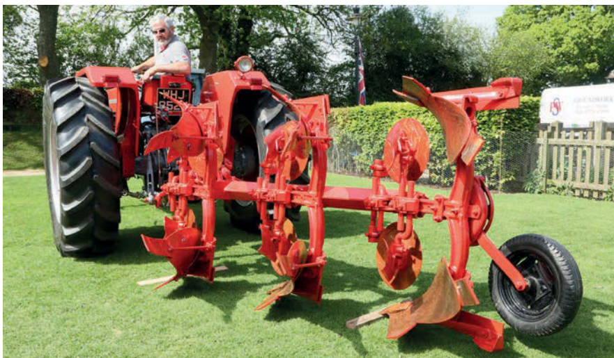
The rigid beam MF 30 three-furrow plough has been given a full restoration by Mick, including a new trailed wheel.
