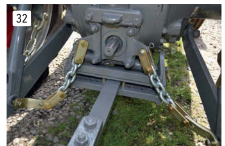
The inner check chains were bought from Sparex, they were exact copies of the originals and were zinc-coated.
