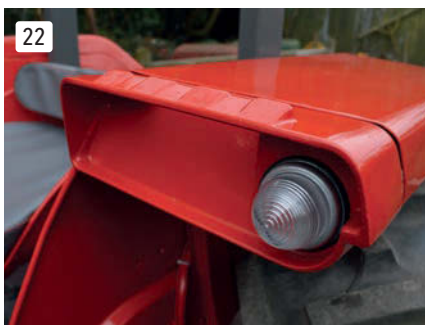
Unfortunately, the original glass Lucas lights couldn't be reused, so these reproduction ones were bought and looked OK.
