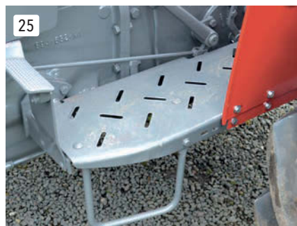
Another feature on the original MF 165 models was this step ring, and it certainly helps getting onto the tractor.
