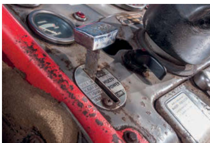
Multi-Power was standard on the 8 Line tractors. The 168 could also be ordered with a 'down-spec' eight-speed 'box.
