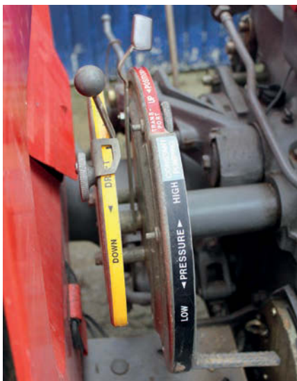
Two levers but with three functions on the hydraulic control quadrant; draft, position and pressure control.
