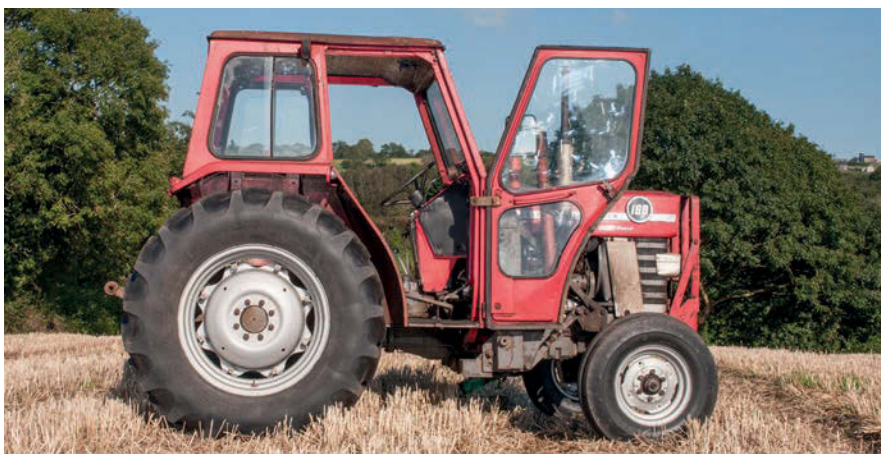
The optional GKN Sankey cab dominates the profile of the 8 Line tractors. Sirocco's Flexi-Cab was the standard fitment. The extra six inches made cab access much easier.
