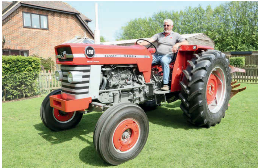
Fitted with the Perkins A4-248 engine that's said to produce 75hp at 2,000rpm, the MF 188 - like all the 8 series range - carries a spacer at the back of the gearbox and rear housing.
