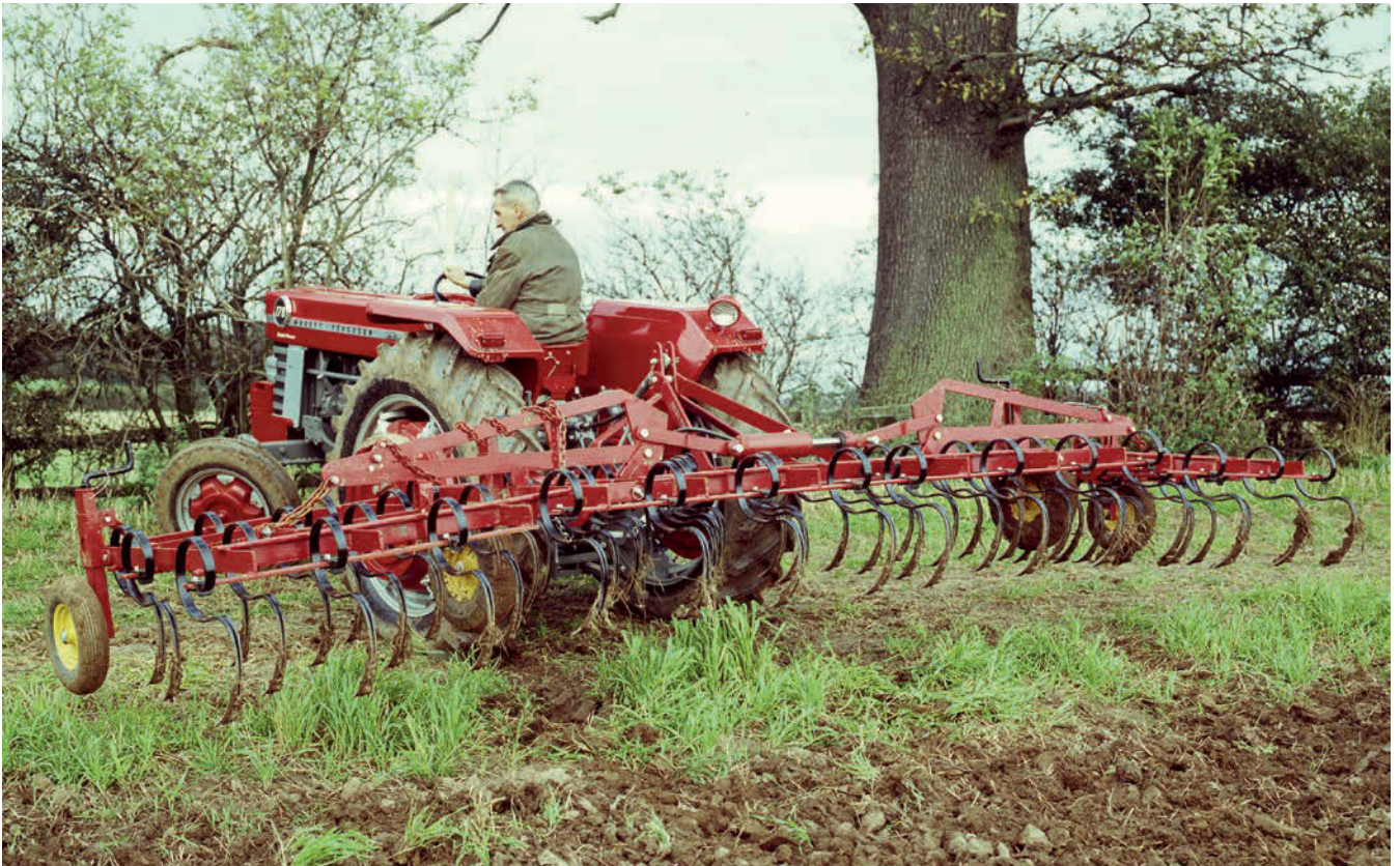
Demonstrating the MF 37 flexible-tine cultivator was another role for the 178 tractor. Available in single- or three-section form, the 53-tine model seen here was said to be suited to both the 178 and 1100 tractors. It had a working width of 18ft 3in (5.56m) and a transport width of 9ft 10 in (3m). (Pic: AGCO)
