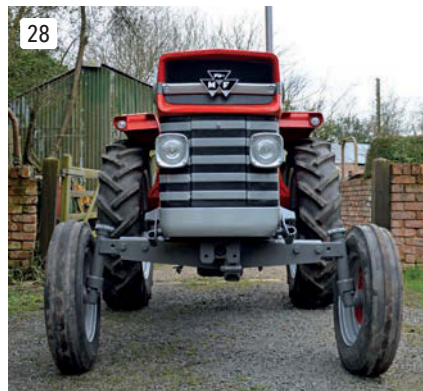
From this angle you can see how good the ground clearance is on the MF 165. The front axle adjustment was, as usual, seized.
