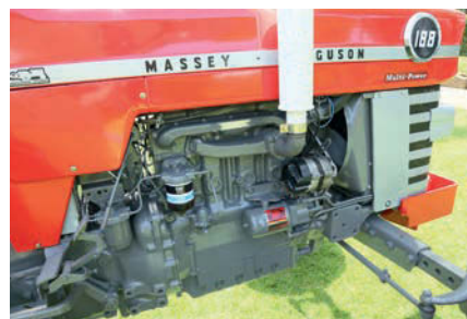
The electrics have been updated with an alternator. Note the correct, period decal on the power steering pump housing.
