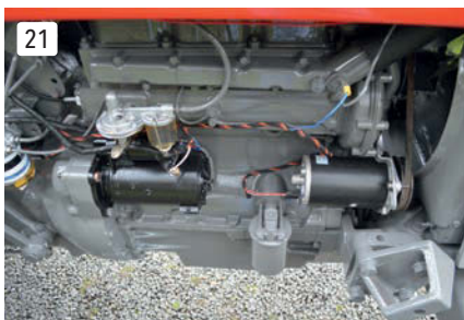
The original starter and dynamo were probably OK. However, if replaced later, they would be black as this was a standard Lucas colour.
