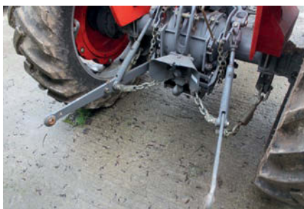
Heavy-duty Category 2 lower links are specified with a 2,900lb (1,769kg) lift capacity.
