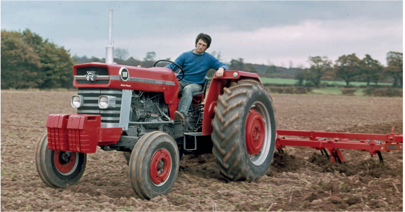
With 71hp (DIN) available to the operator, the A4.248-engined MF 188 was a lively performer. (Pic: AGCO)
