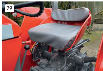
A new seat cushion set is always fitted as the originals are typically either ripped and damaged, or missing altogether.
