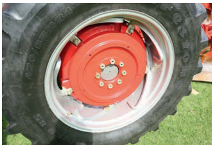
Those PAVT wheels are something else and did their job well when new. But, over the years, the slide mechanism on the cast steel rims with cast steel centres were known to seize through lack of use.
