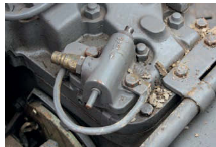
This tractor features a loader diverter valve in place of the combining flow selector valve.
