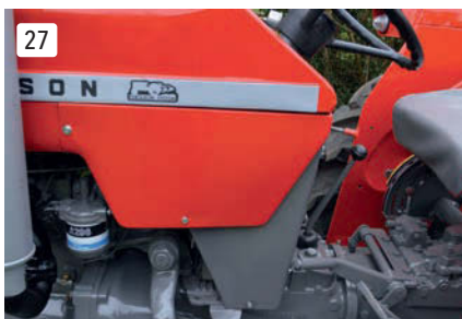
On original MF 165s, the bottom corner of this panel was grey (later ones were red). It took more work to paint like this, but originality was important.
