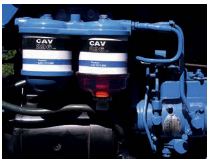
Trying to remove the starter motor on the Ford 4000 is tricky due to the location of these fuel filters and the injector pump.
