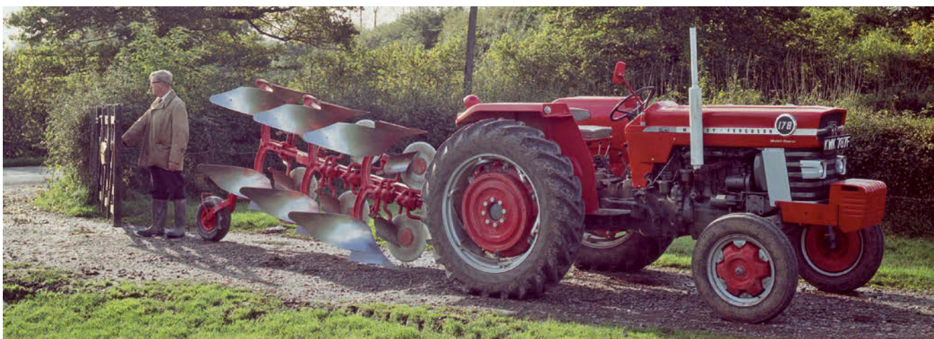
Taken in October 1968, this photograph shows Bill Sargent with the 178 and an MF 32 three-furrow reversible plough. Despite the tractor's adequate lift capacity, a transport wheel was supplied as standard to take the weight off the three-point linkage. (Pic: AGCO)
