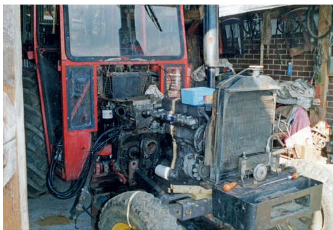
The radiator was in good condition so was simply flushed through.
