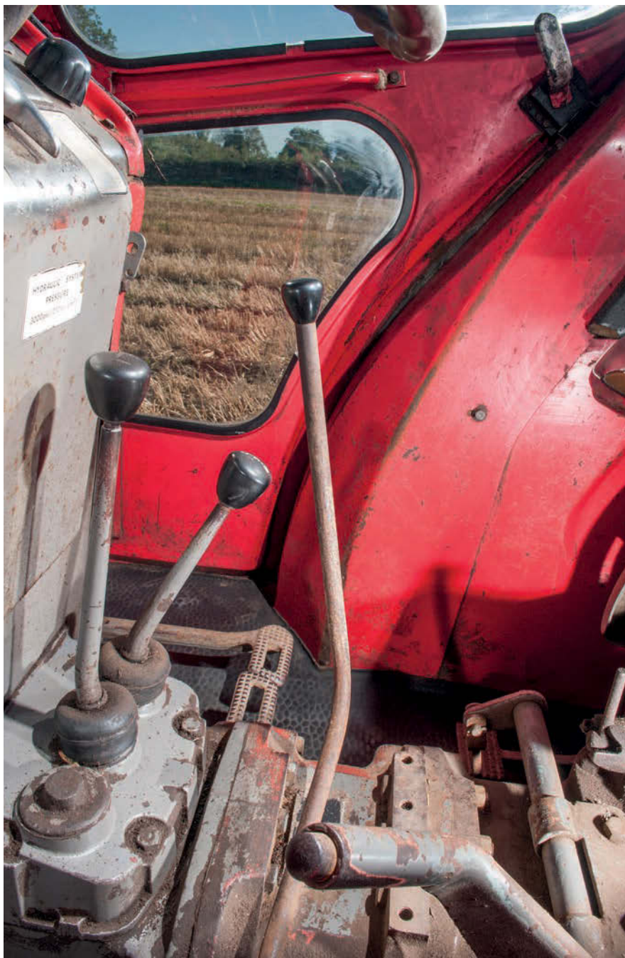
The long lever operates the shuttle gearbox, with equal speeds in forward and reverse gears!
