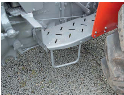
This extra step fitted to the early 165 makes getting on much easier, as the tractor is quite high.
