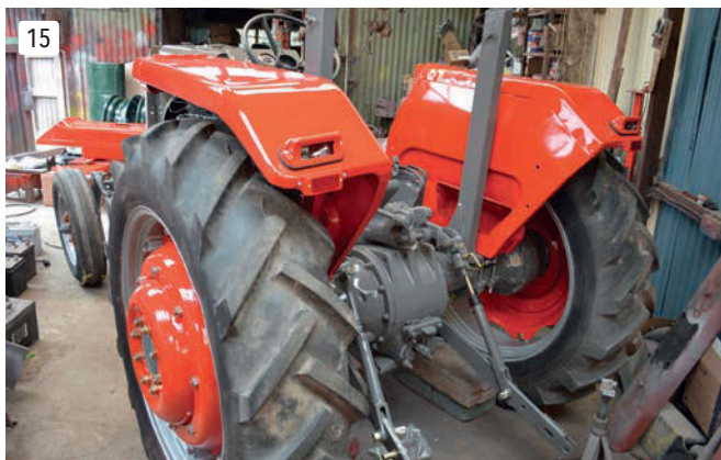
The tractor soon started taking shape once the wheels and wings were fitted. Note the bonnet in the background, waiting to be fitted.
