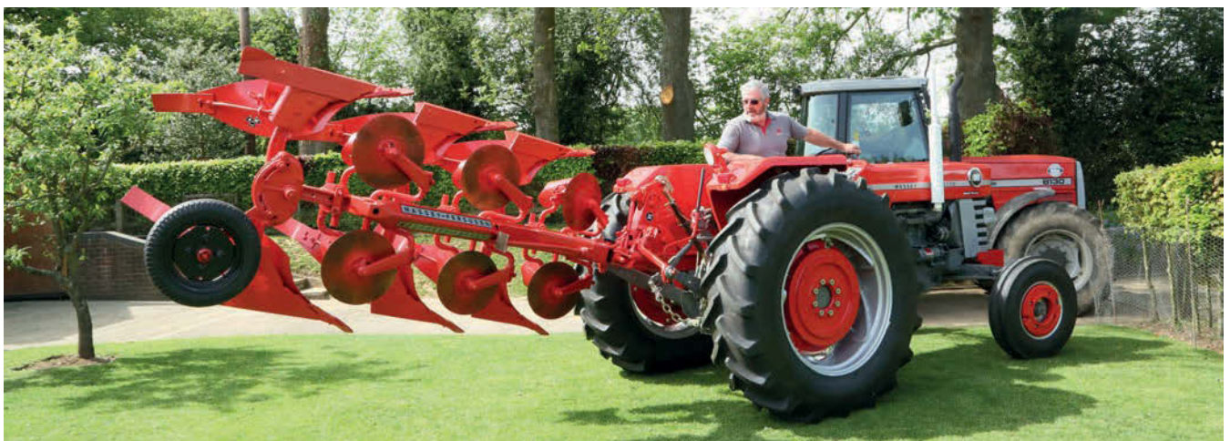
The outfit oozes class; the front tombstone features a 62.5mm spacer to give the tractor more stability, and was standard on this model.
