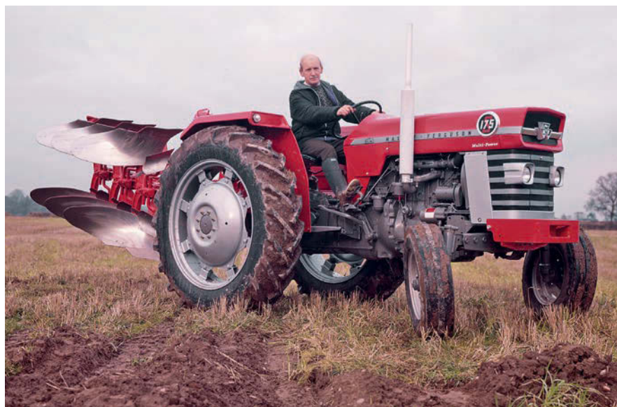
For those that didn't require cast wheel centres, standard pressed-steel versions were available. (Pic: AGCO)
