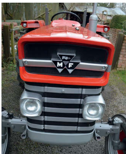
The front of the MF 165 featured the famous three-triangle MF badge. Two round headlamps and a detachable section on the grille made up the distinctive front.
