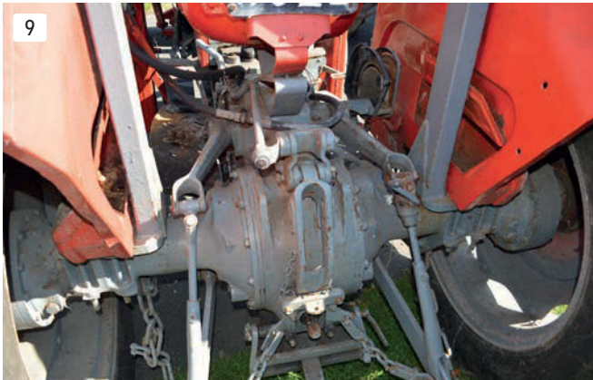
The hydraulic arms were also scrap; they had obviously worn so much in the past that somebody had welded the detachable ball ends into place.
