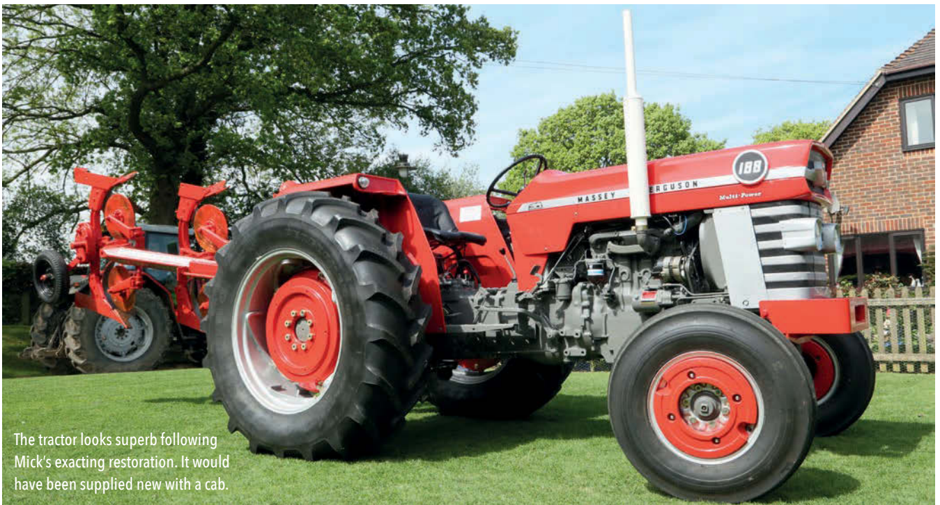
Fitted with the Perkins A4-248 engine that's said to produce 75hp at 2,000rpm, the MF 188 - like all the 8 series range - carries a spacer at the back of the gearbox and rear housing.
