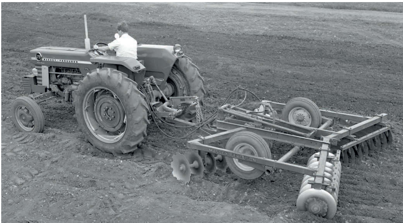
The MF 175 was 137in in length, 72in wide and had a wheelbase of 84in.
