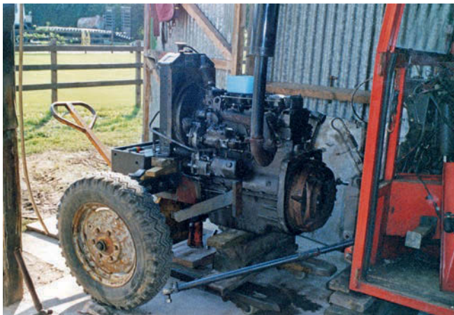
The tractor was split to rebuild the clutch.
