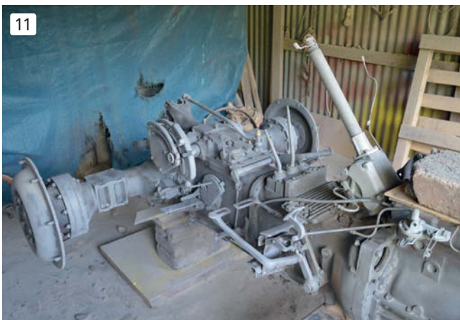
No, this isn't a photograph of the skid unit coated in grey primer, it's bare, sand-blasted metal, and doesn't it look better?
