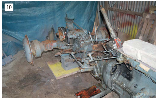
I soon had the tractor stripped and ready to be sand-blasted. By this stage it looked even more of a mess as more rust was now visible.
