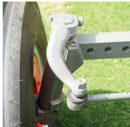
The king pin assembly was rebuilt during the restoration, and included new bearings as well as track rod ends.
