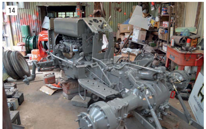
The skid unit went through the same painting process as the panels, and was built up as much as possible before the final coats.
