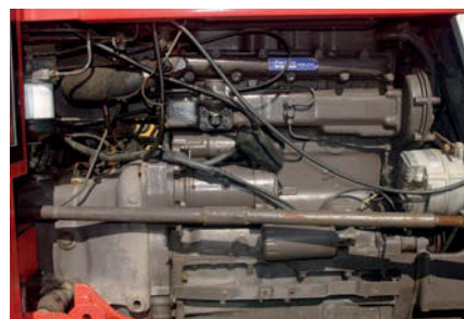
Apart from replacing filters, a service and a repaint, the Perkins A4.203 needed nothing more.
