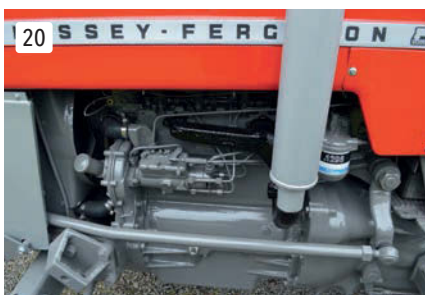
I always paint the manifolds in heat-resistant black. A clamp on the silencer was fitted before it went home.
