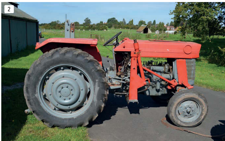
The side view of the 165 shows there's a lot to be done, but all the tinwork was salvageable.
