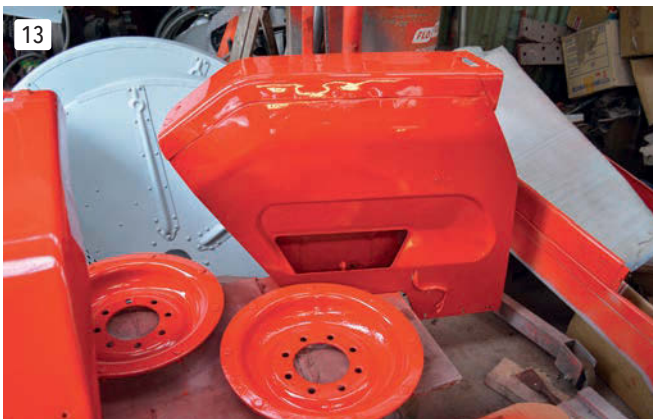
All panels were treated to a coat of primer, two coats of undercoat then three coats of MF Red. They were then left for a week to harden.
