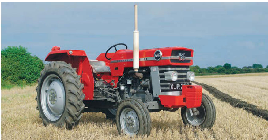
The MF 165 came with Category 1 and 2 rated linkages. (Pic: Alan Barnes)
