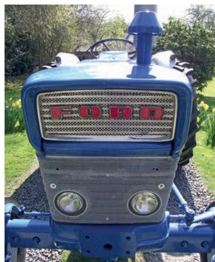
The word 'Ford' picked out in bright red paint, was prominently positioned on the 4000's upper grille section. The whole grille could be removed by undoing a couple of bolts.
