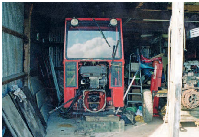
The cab frame proved to be in excellent condition, with just a little surface rusting.
