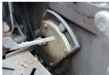
Response control (the implement rate of drop) is preset using this lever on the transmission casing.
