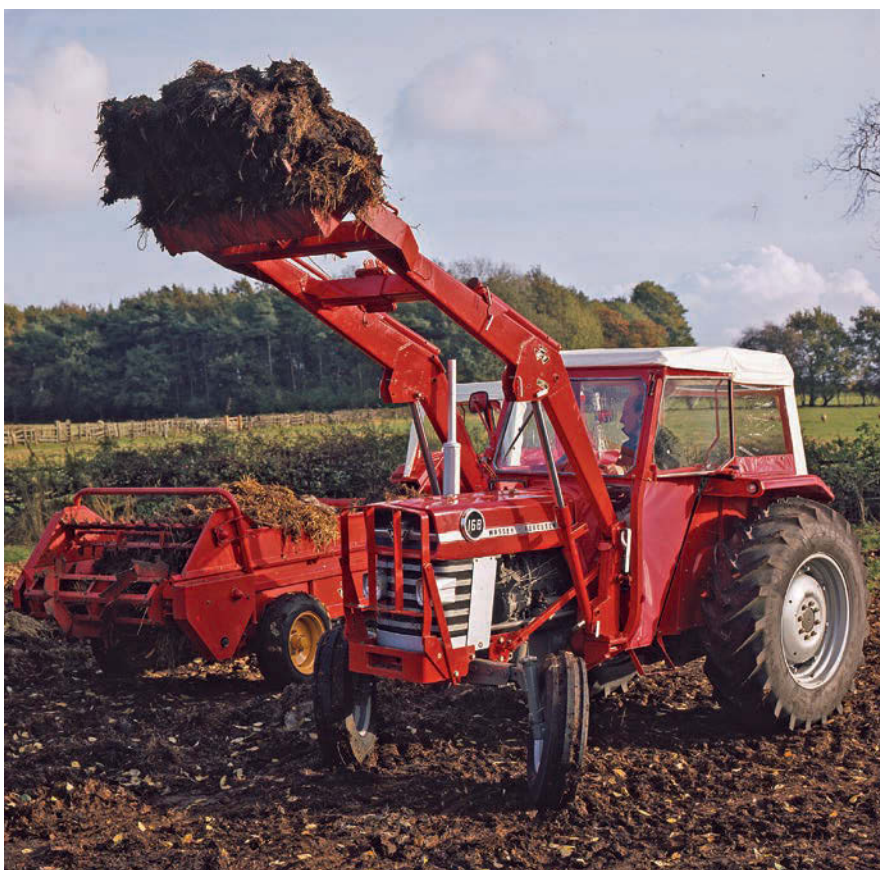
The 168 was well liked, partly due to its excellent Perkins A4.236 engine. (Pic: AGCO)
