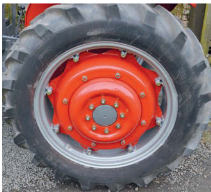
The rear wheels on the MF 165 featured centres that had dishes that could be split, allowing for a greater variety of widths.
