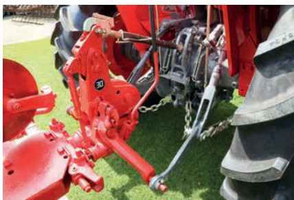
The 188's rear end with hitch in place and the 106.25x18.75mm linkage arms with the 25mm lift rods that were offered with floating slots for wider implements as an option.
