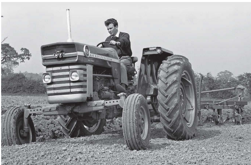
An MF 175 working with a five-furrow MF 86 semi-mounted plough. The plough was available with four to six furrows, and was well matched to this tractor. Note the track-width settings and interesting front tyre pattern. (Pic: AGCO)
