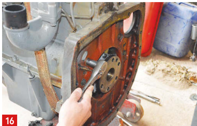
16 Refitting the backplate after the seal is fitted is the first step to putting this job back together. It's all been cleaned prior to fitment.
