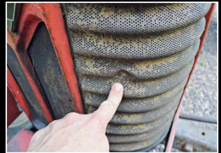
The tinwork was essentially in good condition, although the front grille had a few slight dents, but this sort of damage is always easy to tap out.
