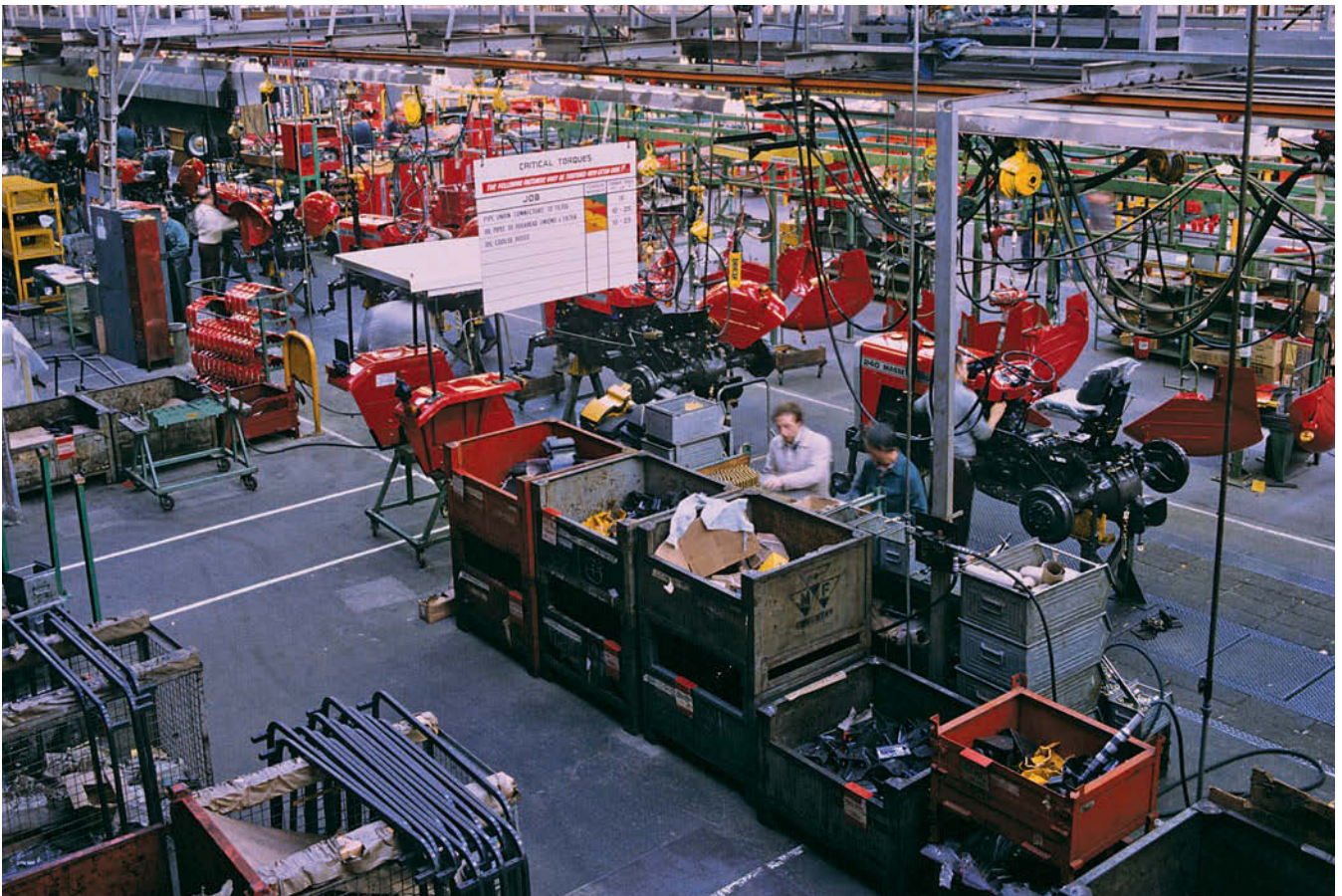
The MF 200 series main production line, in the late 1970s, with a MF 240 in the right foreground. Note the stillages and racks of parts placed strategically at the points on the line where they'll be needed, as listed on the computer-generated build card, produced for each individual tractor.
