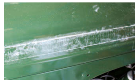
An impression of the lettering is retained when the tracing is removed.
