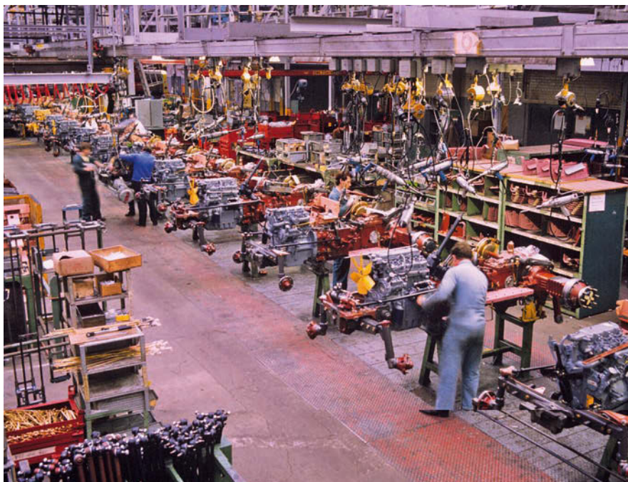
The initial chassis build line, where the main assemblies - front axle, engine, gearbox and rear axle - came together before the complete chassis 'carcass' went for painting.
