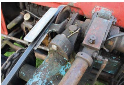
The boom shear bolt (centre of photo) prevents the boom from torque-overload.
