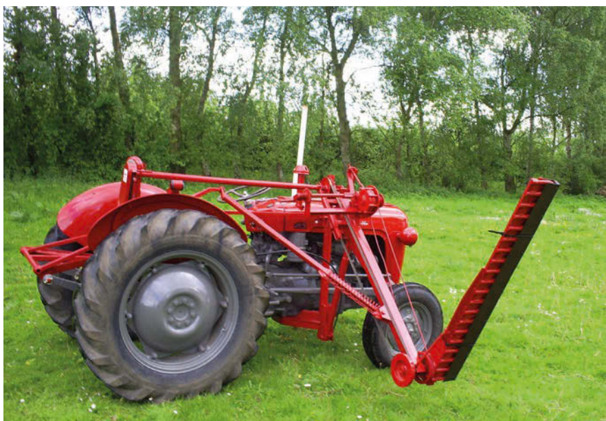
The Teagle mid-mounted Tracut - costing £150 in 1962 - provided competition to the Angle-Draulic. Photograph kindly used by permission of the owner, Reginald Sharpe.
