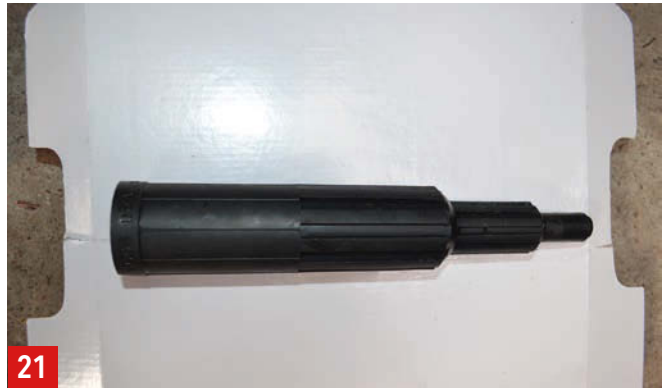
21 This clutch lining tool is a very useful thing that makes lining-up the double clutches easy. It will fit a number of MF Perkins-engined tractors from the 1960s and 1970s.
