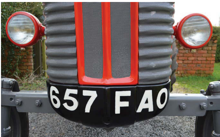
Lights weren't always fitted to the MF 65 but, if they were, they were mounted on the side. The centre grille section could be removed to access the radiator.
