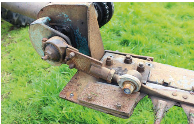
Power drive is transmitted through the swivel head to the knife crank and connecting rod.
