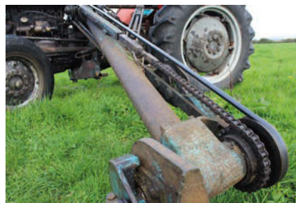
A chain, operated by a double-acting ram, rotates the swivel head and angles the cutter bar.
