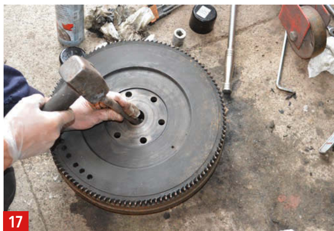
17 The oil-soaked flywheel was degreased and a new spigot bearing was fitted, then it was tapped out from behind.
