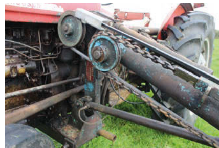
The front mounting bracket attaches to the underside of the clutch housing; the driving pulley receiving power from the PTO is shown.
