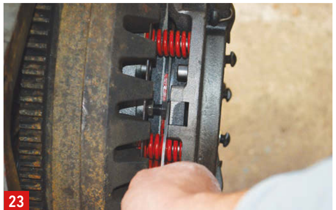
23 Setting the PTO clutch plate gap is done using feeler gauges. A nut locks it into position.
