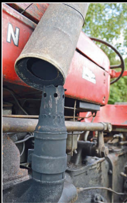
Lifting the silencer revealed the problem; the pipe had broken off just above the clamp.
