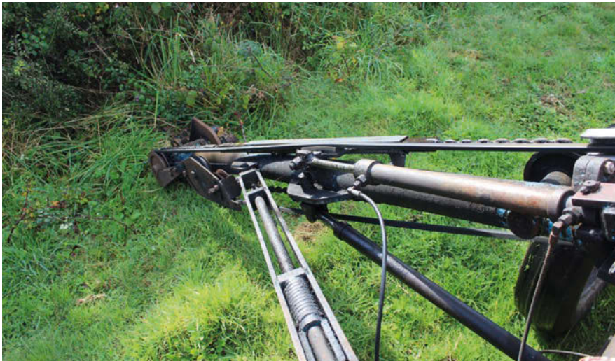
The cutter bar from the operator's seat while taking the base horizontal cut.
