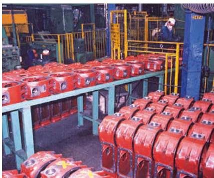
Rear axle centre housing castings, fully machined and in red primer, awaiting fitment of the internal components and the rear axle trumpet housings.
