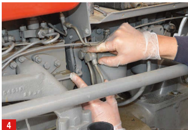
Forgetting to disconnect simple things like fuel lines and throttle levers will prevent the engine from separating - they're easily overlooked!
