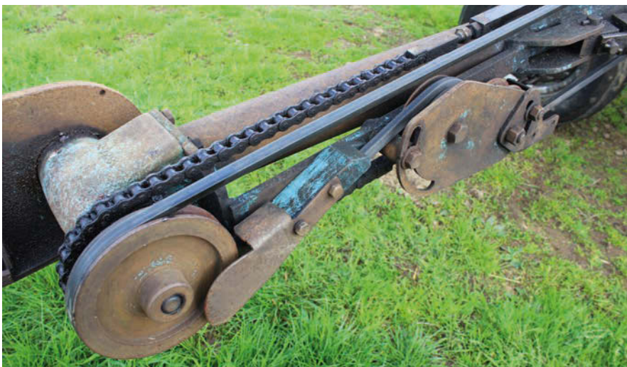
The vee-belt travelling the length of the boom supplies power to the swivel head; the belt-tensioner is clearly visible.
