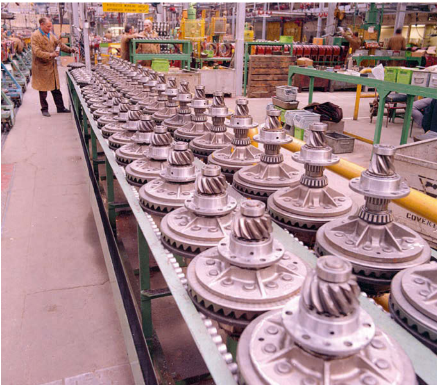
The crownwheel and pinion assembly track showing, at the front, assemblies for the larger, four-cylinder machines (the bigger pinion is the giveaway). The rear line has the smaller, three-cylinder-type assemblies. Note that the pinions and crownwheels are paired when being set up, and have been matched for optimum performance and adjustment.
