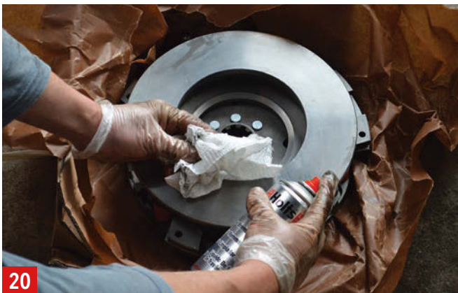
20 The new clutch assembly was wrapped in oiled paper to stop it rusting in transit. Here I'm degreasing the surface.
