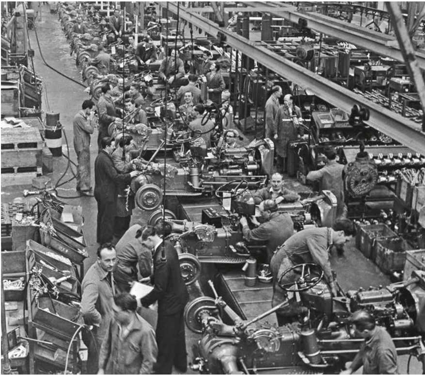
A late 1959 photograph of MF35s. The chassis 'carcass' was largely assembled on the transverse track, before going on to the final 'follow-my-leader' assembly line.
