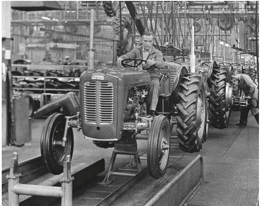
The final checkout and 'snagging' (fault correction) point on the 'grey and gold' FE-35 line, circa 1957/8.
