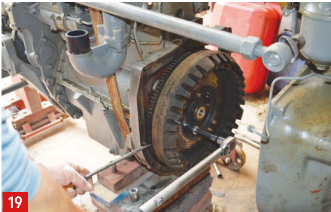
19 Jamming the flywheel with a screwdriver enables the bolts to be torqued up, I always go over them twice to double-check.
