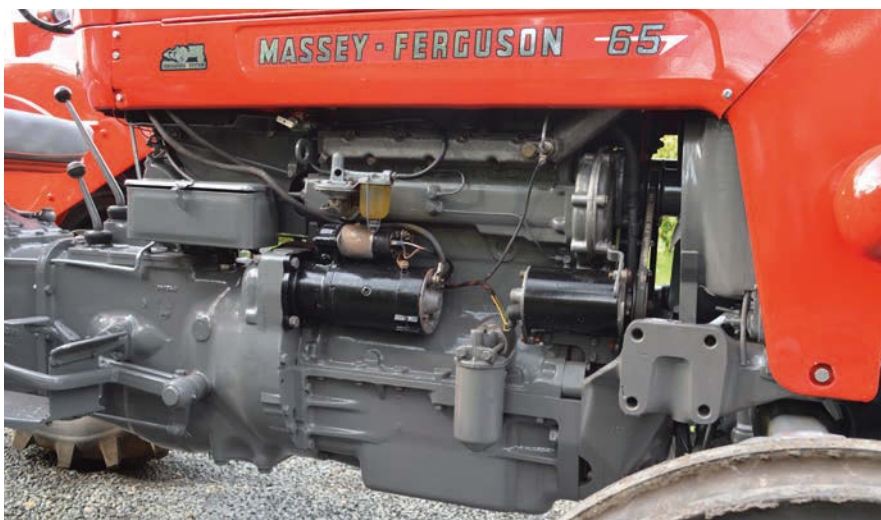
The four-cylinder Perkins engines fitted in the Massey Ferguson 65 were almost unbeatable, due to their impressive reliability.
