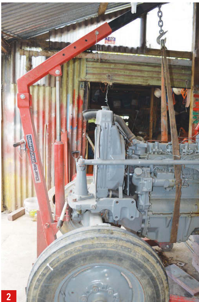
Using an engine crane to support the engine; this helps with sliding it out and, hopefully, with sliding it back in again!
