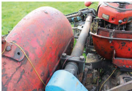
The mounting brackets cradle the boom pivot tube, which carries the driveshaft internally.
