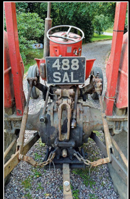
The registration plate explained why the owners referred to this tractor as Sal . Looking closely, I could see signs of oil leakage around the axle and PTO.
