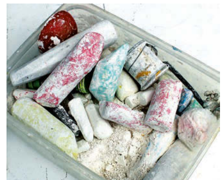
The chalk is powdered and rubbed across the back of the tracing which, when over-written, leaves an impression of the design to be sign-written.
