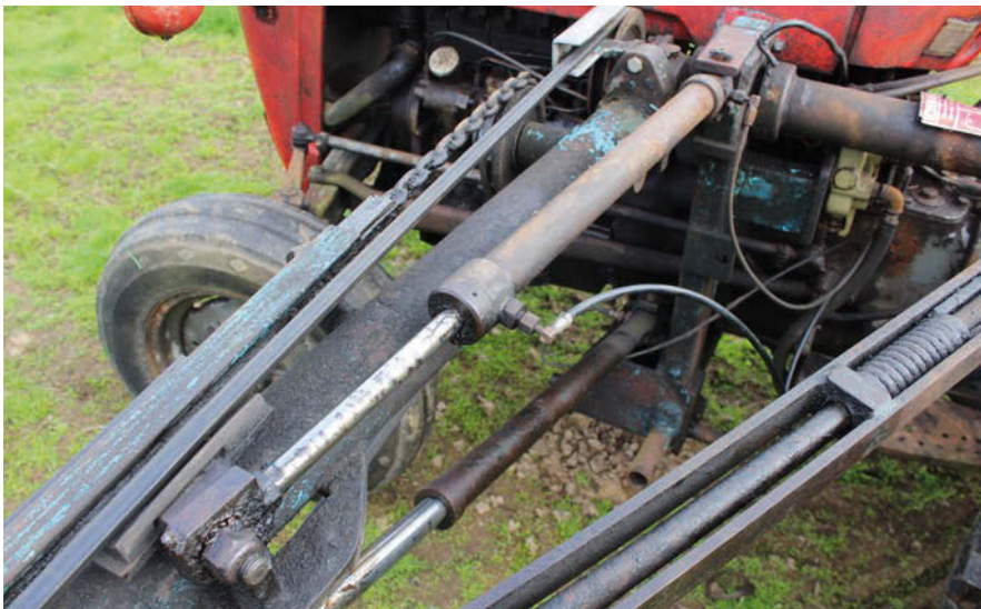
Hydraulic rams control both boom and cutter bar orientation.
