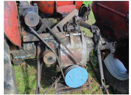
Drive to the cutter bar is taken from the PTO shaft through a double vee-belt arrangement.
