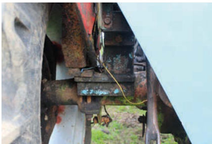
The rear mounting bracket is attached to the rear axle mudguard attachment point.
