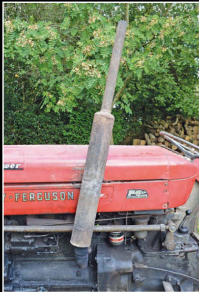
The angle of this exhaust obviously isn't right. It was being held in place by wire and rattled a lot when the engine was running.
