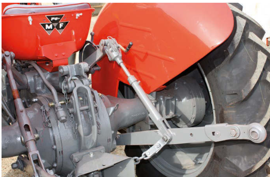
The Ferguson System hydraulic control makes the 65 a pleasure to operate – it's both simple and effective. (Pic: Andrew Hall)
