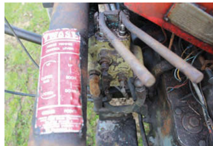
Trimmer hydraulic controls are well placed to the lower left of the dash panel.
