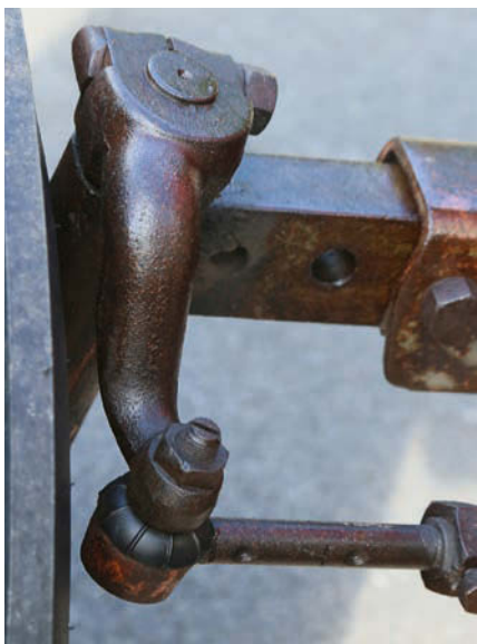
The ball joint rubbers are the original ones and have cleaned up well.
