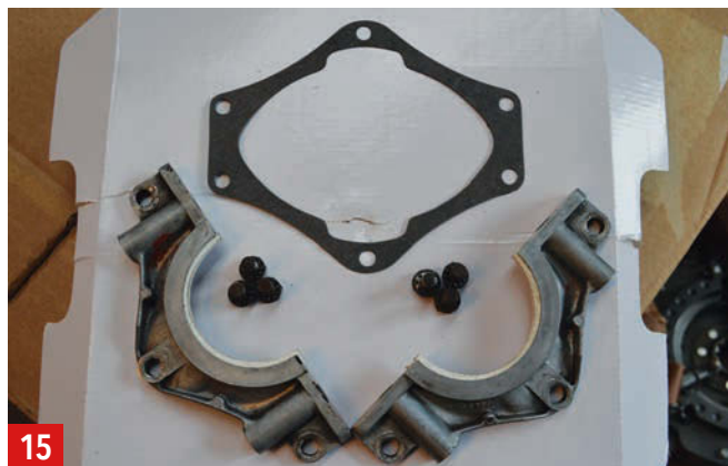
15 Here is what the rear crank oil seal involves – the new rope seal has been rolled into the grooves.
