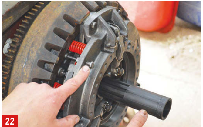
22 In the middle, the clutch lining tool is in position. My left hand is showing the installation bolts that need removing.
