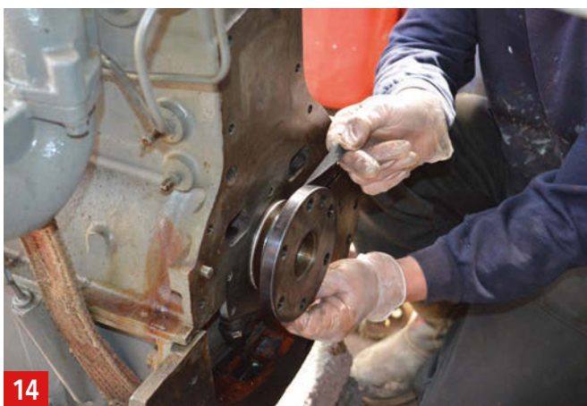
14 Dressing the crank up with some Emery tape gives the new seal a nice smooth surface to sit against.
