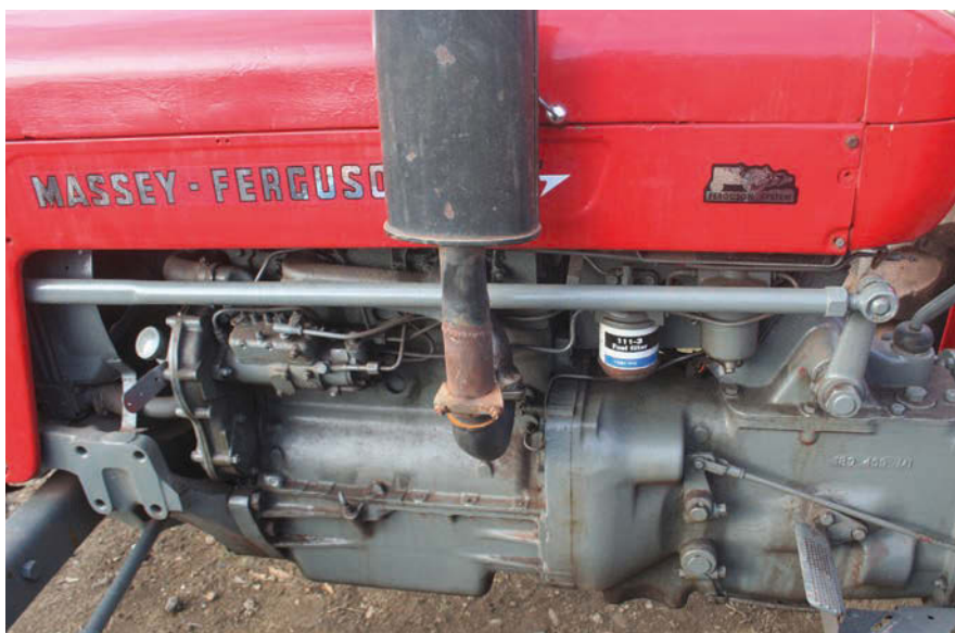
This photograph clearly shows the single-arm steering system used on the MF 65. (Pic: Andrew Hall)
