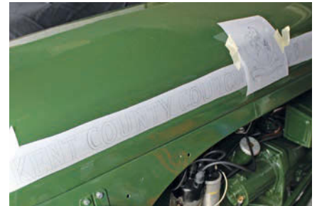
The draft is temporarily attached to the bonnet and adjustments made to the script.
