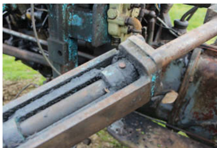
The boom shear pin or nail (centre of photo) provides a breakaway device for the cutter bar.
