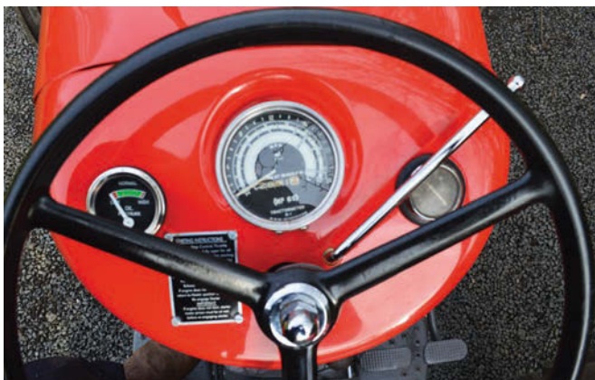
The MF 65's dash was a simple affair that stayed largely the same throughout the model's production run. The three gauges provide all the essential information that the driver would need.
