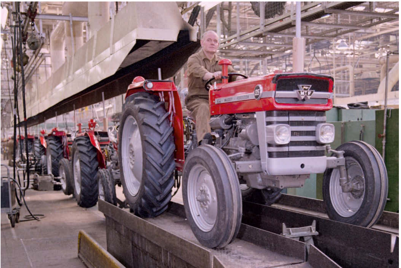
A post-1970 photograph of the MF 135 final assembly line. Here the tractor is almost complete and ready for despatch. It's the later type with pressed-steel rear fenders and 'straight' front axle.
