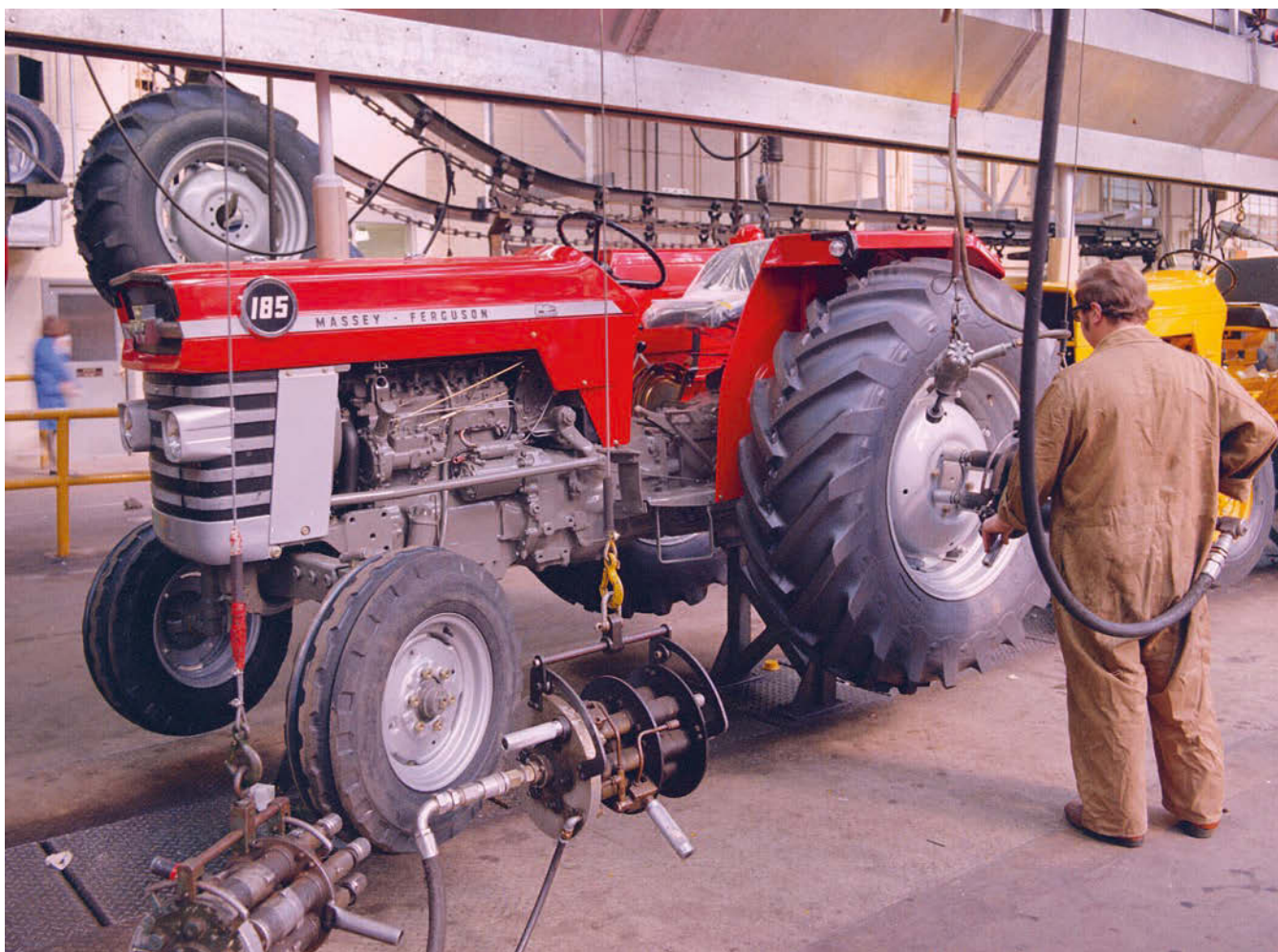
Back in time, to the early 1970s (can it really be nearly 50 years ago?). One of the superb MF 185 models, of which many thousands were made. In this case, an export build, as denoted by the big rear tyres, has its wheels fitted, on final assembly. Note the air-powered, multi-spindle wrenches, that fitted a full set of six wheel nuts in one shot, to speed production.
