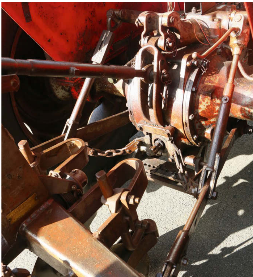
Repairs have been made to the drop arms during the tractor's working life, but Richard has left these alone.
