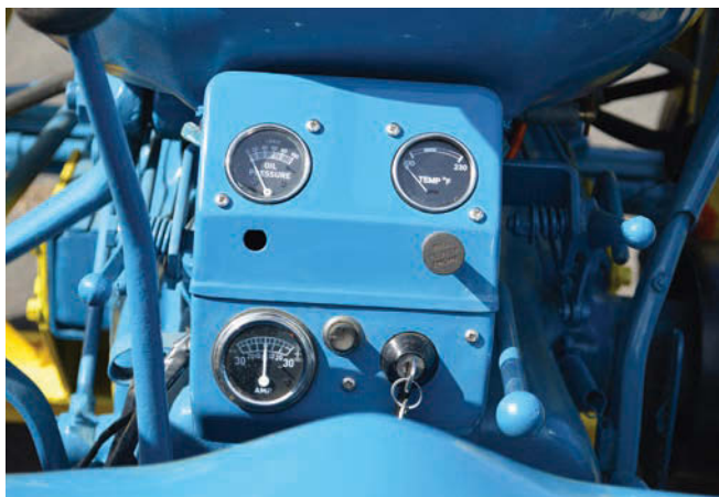
The Fordson dash was updated later in production; this is the early type that doesn't include a tractorometer.
