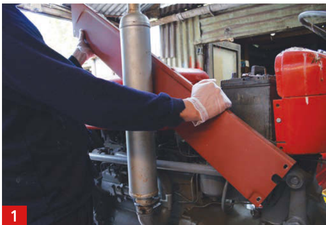
The first job was to remove the tinwork and exhaust on this Massey Ferguson 65; these were all due to be painted later.
