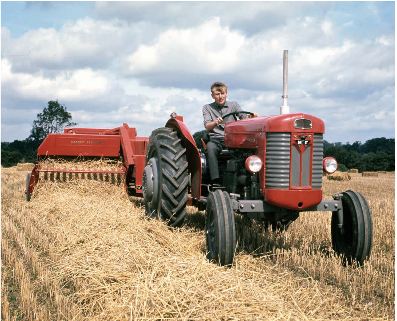
John Senior baling straw with a Massey Ferguson 65 Mk.II. The obvious differences between this model and its predecessor were the introduction of the AD4.203 engine and a Stoneleigh Grey skid unit. (Photo courtesy of Ted Everett)
