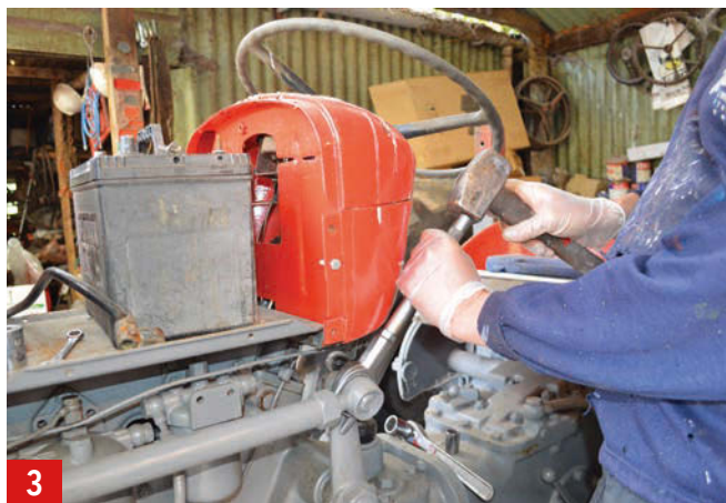
There is only one steering arm on the MF 65; it's up level with the bonnet and you'll need a ball joint separator, as shown.
