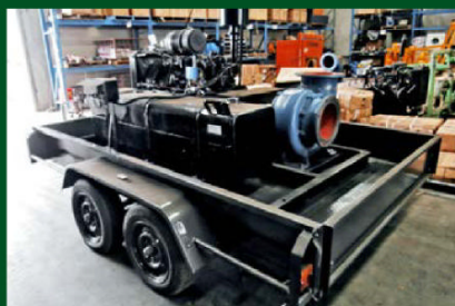
12" 300 IS TRAILER MOUNTED PUMP SET new pump direct drive coupled to second hand 6cyl Nissan diesel with new tandem trailer with Vin. S33. TA750753. $18,810 + GST
