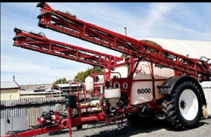
CROPLANDS PEGASUS 6036 30hw / 1002 BA7000 controller non section control, 7 section 30m bargam boom, hyd fold, lift & tilt, 60lt chemmix, hand wash tank, air mix 110-02 nozzles, AR185 pump PTO driven, series 500 compressor, air bag suspension, 20.8-42 tyres 70%. TA1168472. $62,000 + GST
