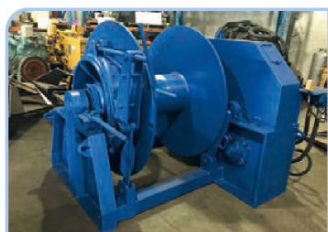
MARINE WINCHES 20 TON 300M / 32MM WIRE CAPACITY
