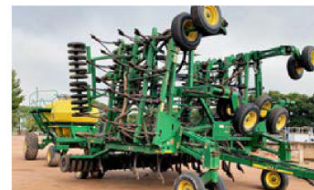
JOHN DEERE 1820 & 1900 45ft bar, 7.5" spacings, c/w Agpoint points, single shoot, gang presswheels, coupled to TBH air cart, 2 bin, 9500Lt, c/w auger. 51207. TA1164890.
