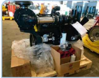
NEW CUMMINS 6CTA8.3-260 260HP RADIATOR INCLUDED
