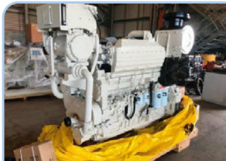
NEW CUMMINS KTA19-M500 500HP HEAT EXCHANGER COOLED
