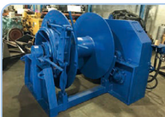
MARINE WINCHES 20 TON 300M / 32MM WIRE CAPACITY
