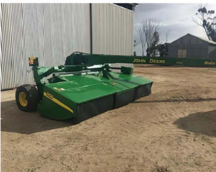
2006 John Deere 956 Mower conditioner, impeller conditioner, 14' cut drawbar, pull manual tilt ram, presents like new.
