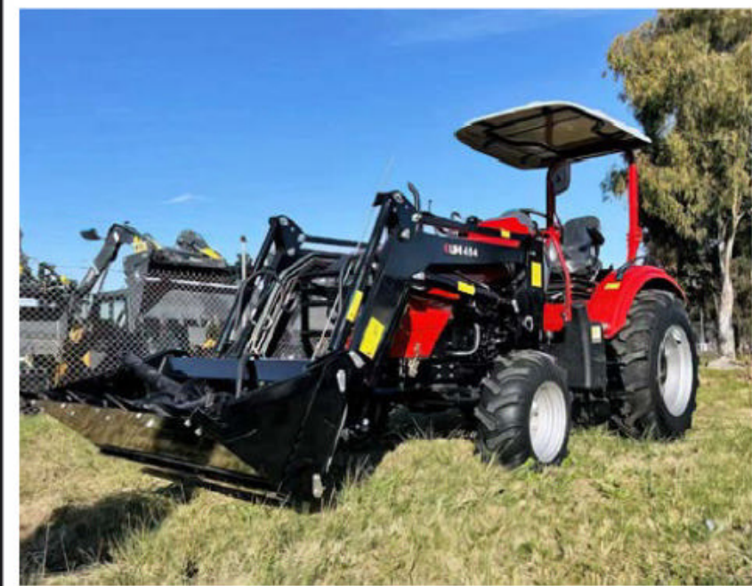
UHI 454 Power Steering, 400kg Front End Loader, 45HP Diesel Engine, Euro quick hitch, FEL 4 in 1 bucket, 200mm bucket, slasher and backhoe.
