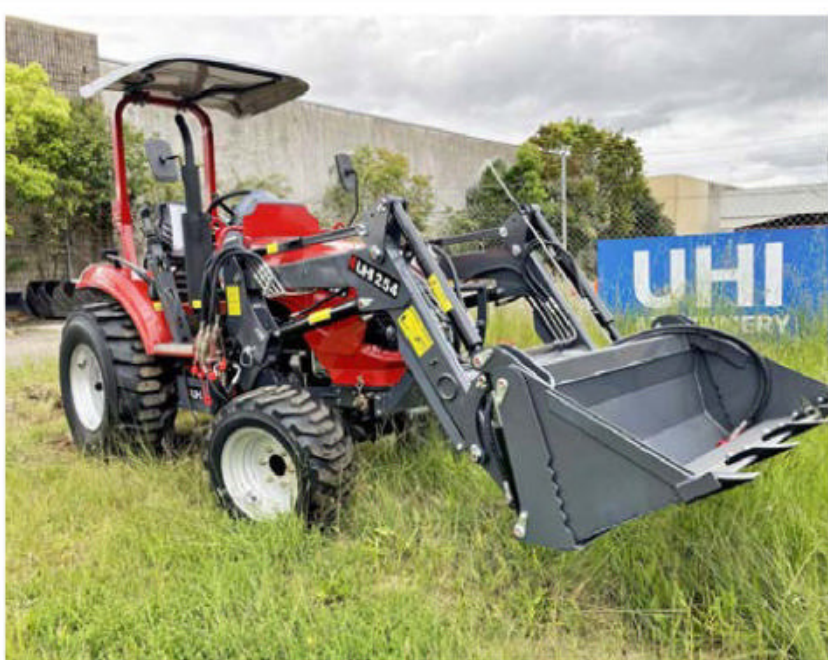
UHI 1254 25hp 4wd with front end loader, Euro quick hitch FEL 4-1 bucket, 200kg front end loader SWL, 8 inch dual functional clutch with metal ceramic friction plate, dedicated hydraulic pump.
