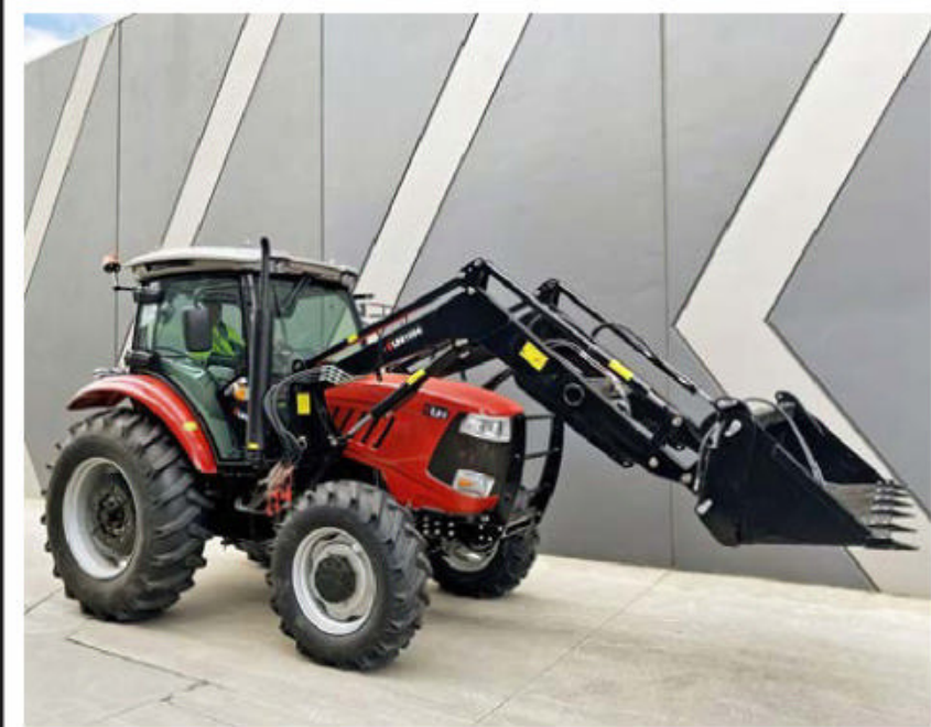
UHI 1004 100hp 4wd with front end loader, Euro quick hitch FEL 4-1 bucket, 1000kg front end loader SWL, 12 inch dual functional clutch with metal ceramic friction plate.
