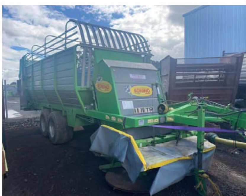
Bonino AB 70 TR Self loading cutter wagon. Equipped with a rotating cutter bar with two drums adjustable in height, which allows a clean and precise cut even on undulating ground.
