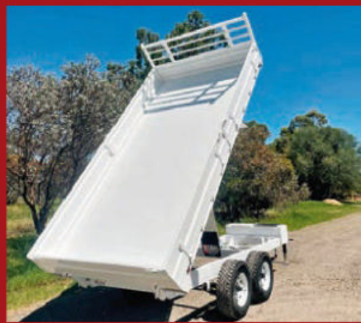
REBEL EQUIPMENT 4M X 2M Rebel Equipment tipper trailer in 3500kg GVM, Made in Forbes nsw.. S24. TA1125368. POA
