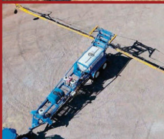
SONIC 201 45 metre boom, 5 sections on single nozzle bodies Farmscan fluid controller 10.4-28 dual tyre 12V Sotera Chemical Pump Coming in September 2023. 102844. TA1171712. $70,000
