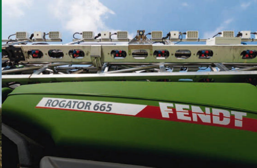
The smart spraying solution with cameras on a Fendt Rogator 665 sprayer
