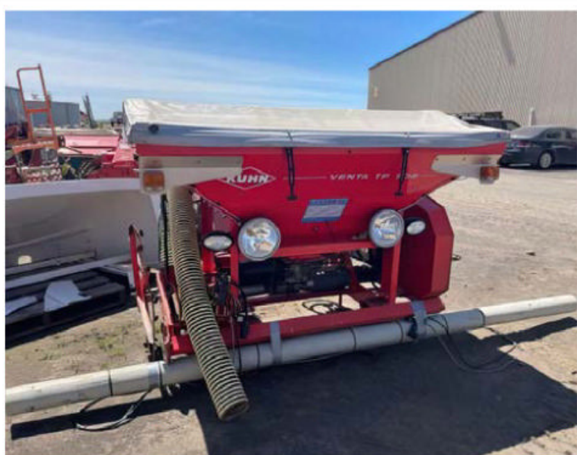
Kuhn Venta TF 702 Front linkage air seed box, 700ltr capacity. Skeleton wheel metering system, can be adjusted for different working widths.
