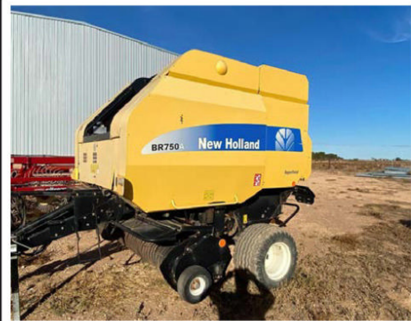
2007 New Holland BR750A Round Baler Super feed round baler, has net and string options, comes with bale command plus monitor. 480/45-17 tires. 23,878 bales.
