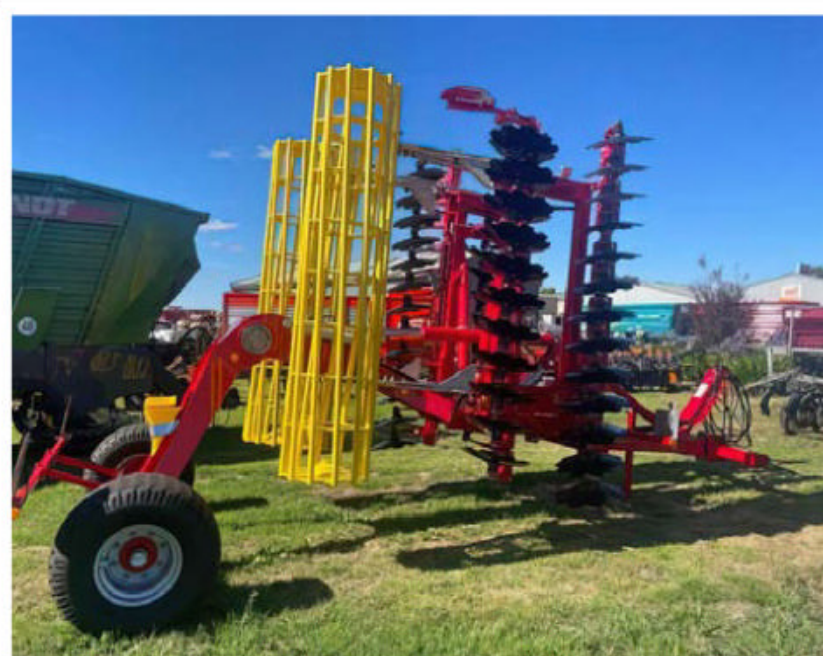
2023 Poettinger Terradisc 6001T New. Trailing 6m folding speed disc with crumbling rollers.
