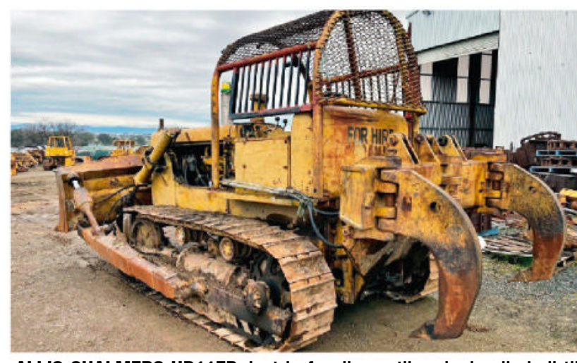
ALLIS CHALMERS HD11EP Just in for dismantling, hydraulic bull tilt blade, swivel tyne rear rippers, turbo 11,000 series running engine, Powershift transmission and converter, good undercarriage all round, all parts available, phone Brendan on 02 6762 4466. S172. TA1144219. POA
