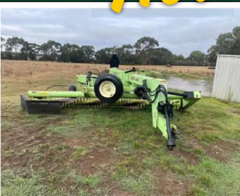
Schulte Trailing SRW1400 Rock Windrower Max 4.27M working width 2.36M transport width. Good for rock, wood and debris for land clearing operations.
