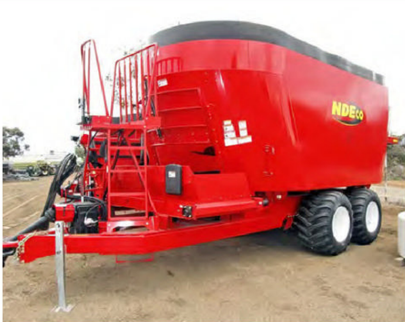
NDE FS1000D All purpose feed-mixer with Weightronix scales, 18 large 24" carbide-insert knives, 12" rubber top, ladder platform. Front door feed-out. PTO drive.
