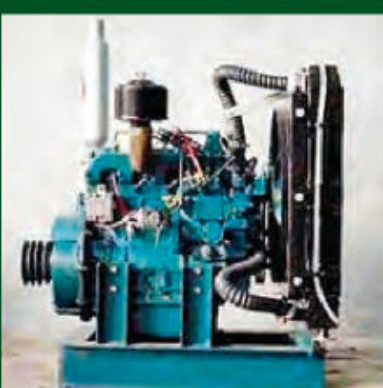
KUBOTA V1200 With 28 hp, 4 cylinder diesel power pack New radiator, muffler, hoses, filters, 35mm keyed shaft. PM045-072-03. DPLIn27547. $3,985
