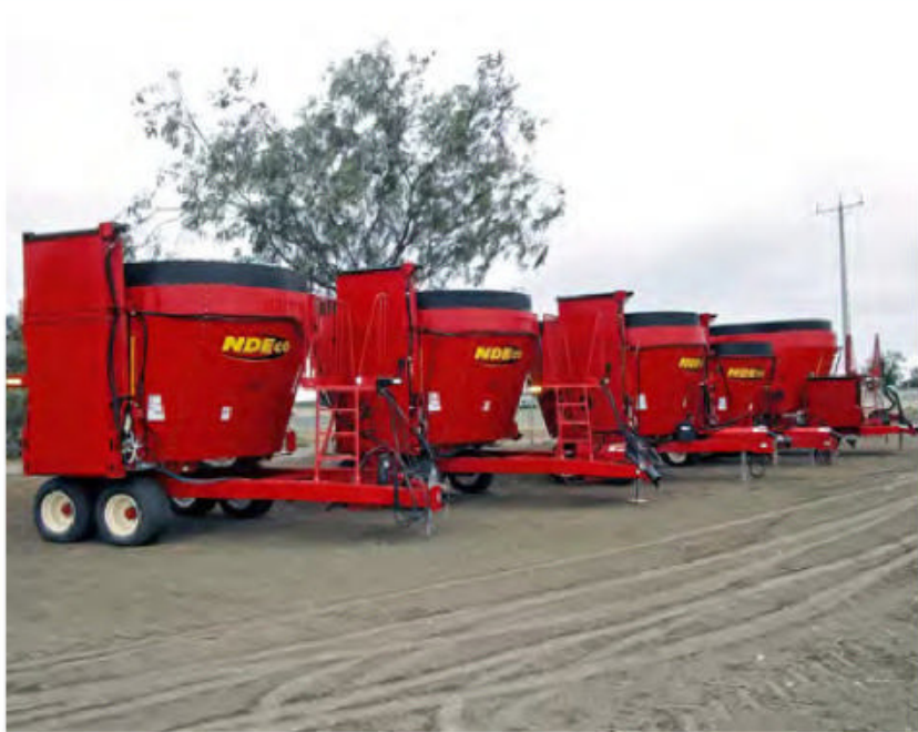
NDE FS700 All purpose feed-mixer with Weightronix scales, 9 large carbide-insert knives, 12" rubber top, ladder platform. Available with front or side doors.
