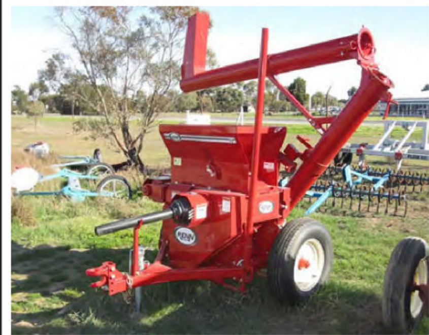
Renn RMC12 Chill cast rolls, removable roll shafts, leaf spring roll protection, tip up feed hopper, grate magnet, feed gate control. 12", 24", 30", 36" & 48" wide models - New.
