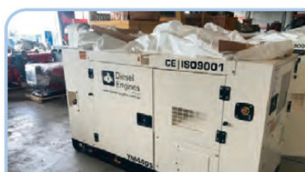
NEW 40 KVA YANMAR GENERATOR, 4TNV98T-GGE (JAPAN BUILT ENGINE), STAMFORD PI144J/COMAP AMF20
