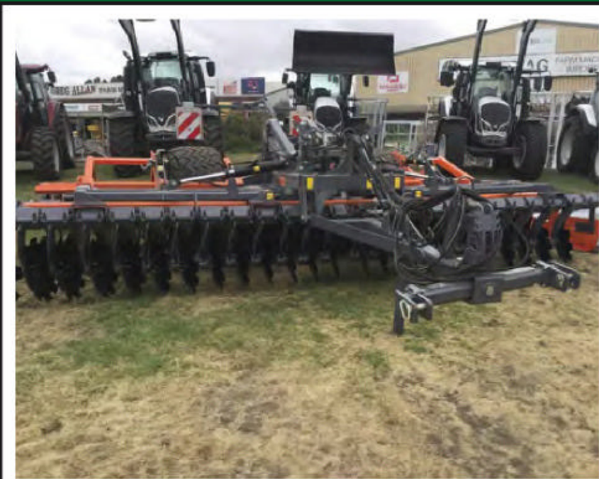
2012 Mandam Gal-K6.0M New. Folding 6.0m Gal-K discs with vring roller Mandam cultivation equipment.
