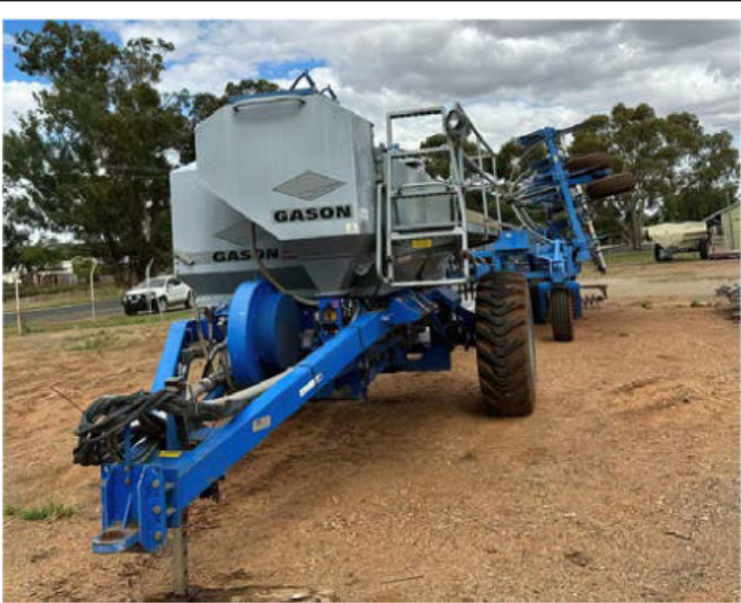
Gason 1850 Bar & Bin Air seeder, 1850 series 2 bin tow between air cart (2,000 lts each bin), ground driven with Gason small seed box, 18.4-26 tyres @ 90%, single fan, LED worklights, cameras in each bin.
