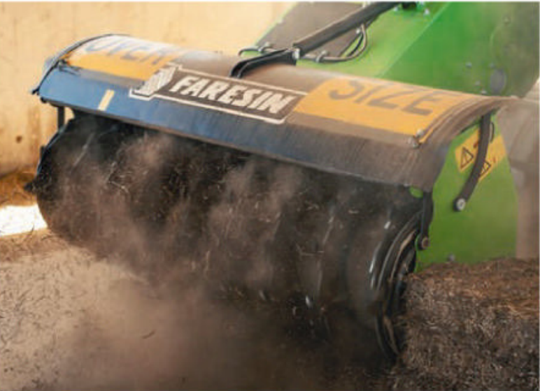
A separate milling head helps take a load off the augers
