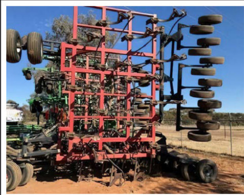
CASE IH Concord 4012 Air Drill. 40ft single fold frame with 4 rows of 500Lb trips spaced at 12 Inch rows, single shoot air package. knife point opener with 6 Inch seeding sweep. New matching packer tyres
