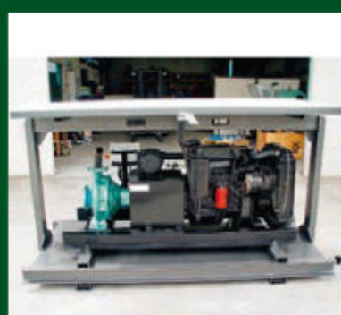
SOUTHERN CROSS 100X65-315 PUMP SET with Nissan QD32 (65hp), skid fuel tank, oil-temp, hi/lo timer watchdog and fork lift roof. Vel67912. TA11060. $13,750
