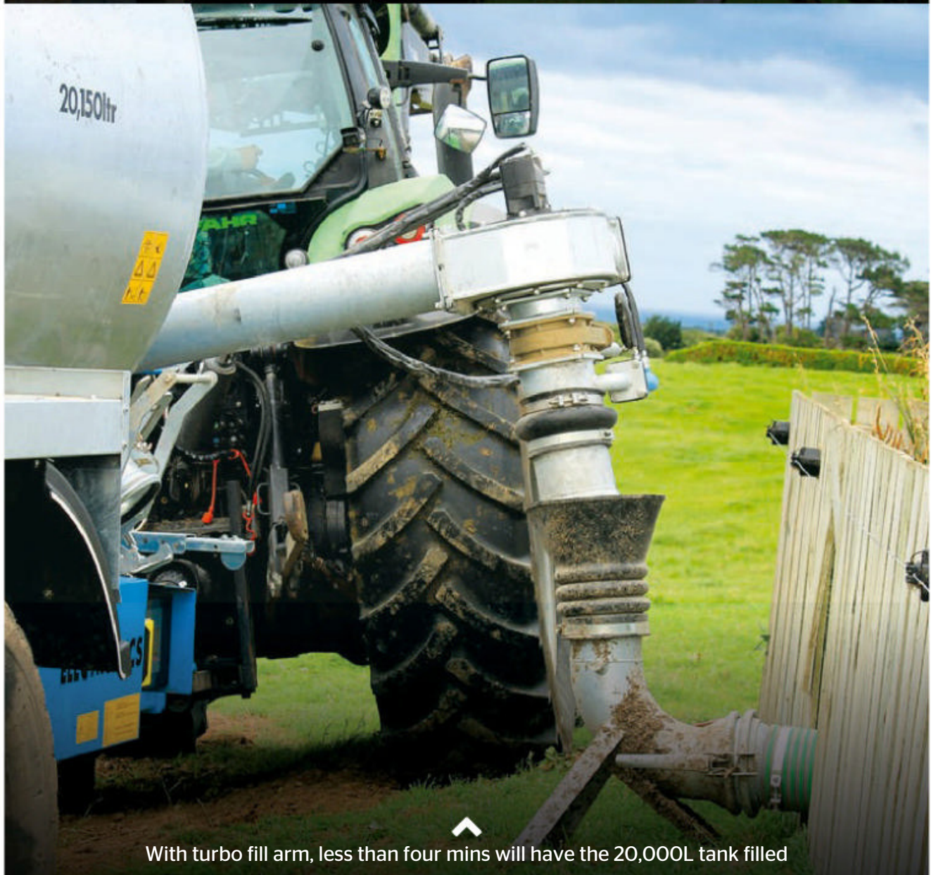
Autofill arm saves time getting on and off the tractor
