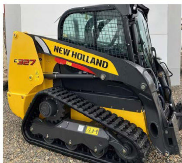
2022 New Holland C327 BRAND NEW 300 SERIES compact track loader. 74HP FPT engine, electro-hydraulic controls, enclosed air conditioned cab, 2 speed travel, ride control, self leveling system.
