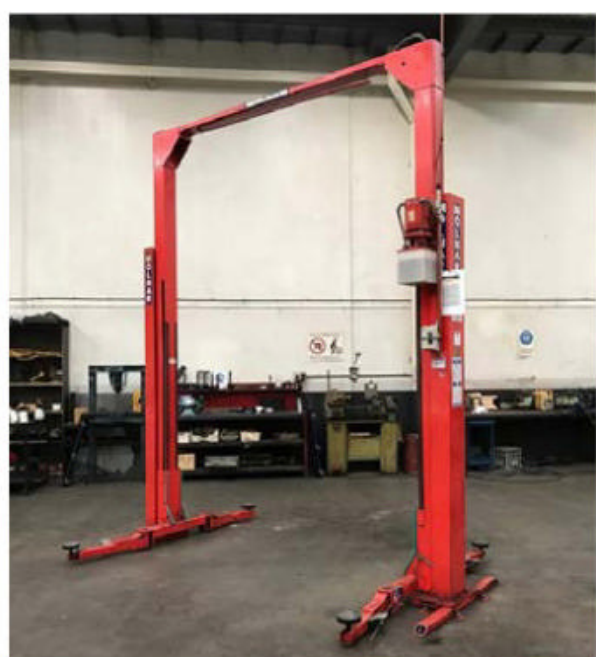
Molnar MF1705-93-OH-3T Clear floor car hoist, type MF1705-93-OH-3T, 3 ton capacity, 2 post.
