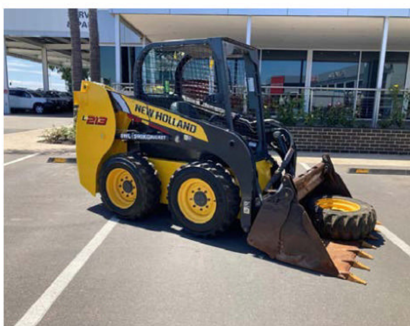
2012 New Holland L213 Skid steer, 676 hours, Digga 4 in 1 bucket with teeth, safe work load (SWL) 590 kgs, mechanical control, fire extinguisher, spare wheel.
