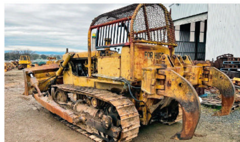
ALLIS CHALMERS HD11EP Just in for dismantling, hydraulic bull tilt blade, swivel tyne rear rippers, turbo 11,000 series running engine, Powershift transmission and converter, good undercarriage all round, all parts available, phone Brendan on 02 6762 4466. S172. TA1144219. POA
