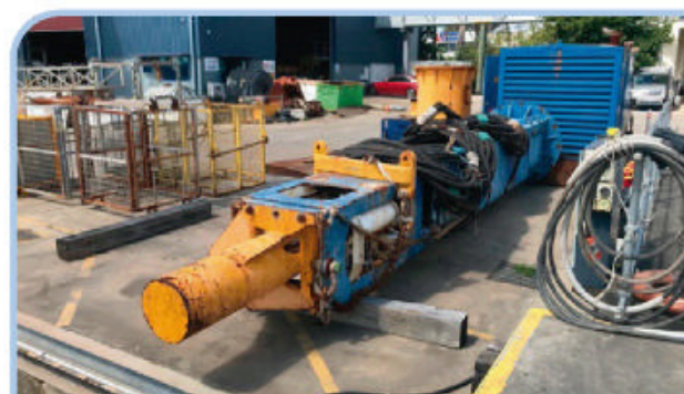
JUNTAN 16 TON PILE DRIVER MODEL HHK16A, 16 TON PILE DRIVER HAMMER, PILE LEADER, PILE CAP & CUSHION, HAMMER ASSEMBLY WEIGHT 24 TON, HOISING INCLUDED
