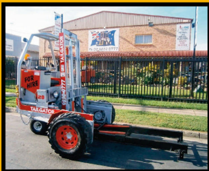
2 tonne diesel self loading forklift with 3 metre
