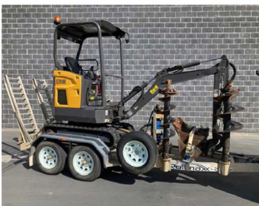
2019 Volvo ECR18E Excavator, 940 hours, engine power - 16.3 HP, maximum flow - 34 ltr/min, operating Weight - 1800 kg, 300mm, 450mm and 1000mm trim bucket, ripper.
