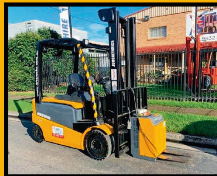
3 tonne electric forklift with 4 meter lift. M049.
