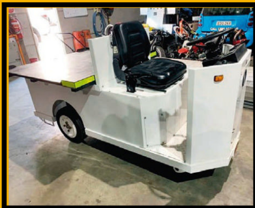
3,000KG Weight Capacity, Electric, Tow Tug.
