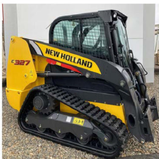
2022 New Holland C327 BRAND NEW 300 SERIES compact track loader. 74HP FPT engine, electro-hydraulic controls, enclosed air conditioned cab, 2 speed travel, ride control, self leveling system.
