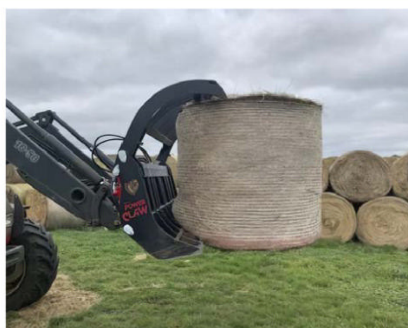
Rata Powerclaw 180 Grab 1.8M Versatile interlocking grab that can be used for fencing & wire cleanup, storm cleanup etc.
