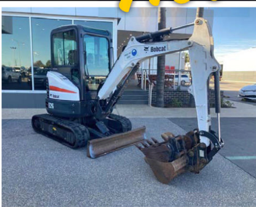
2014 Bobcat E26 Mini excavator. Engine power - 24.8 HP. Maximum flow - 47.4 ltr/min. Operating weight - 2600 kg. 300mm, 450mm and 1000mm trim bucket. Hydraulic hitch.
