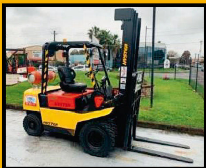
2.5 tonne LPG forklift with 7.4 metre lift. L062.
