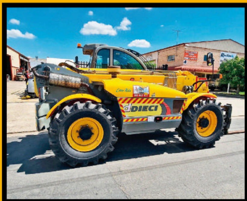
3.5 Tonne Diesel Telehandler 10 Metre Lift
