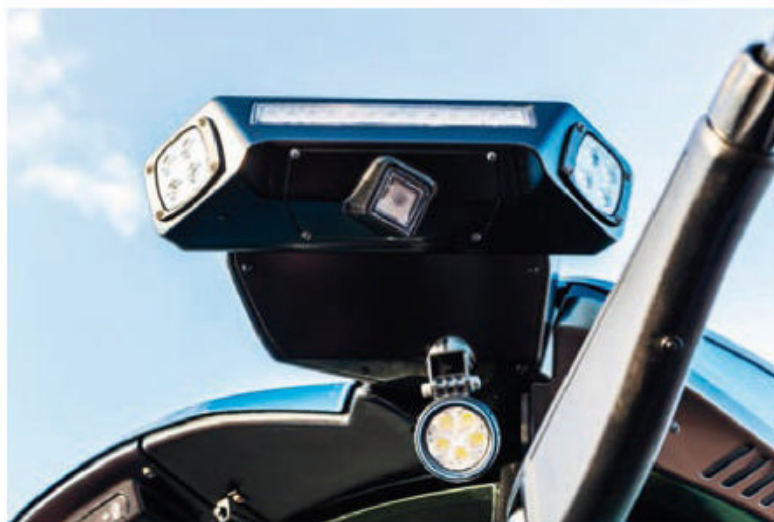
The autonomous features are aided by sensors and cameras on the T4 Electric Power's roof
