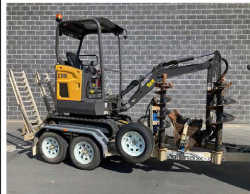
2019 Volvo ECR18E Excavator, 940 hours. Engine power - 16.3 HP. Maximum flow - 34 ltr/min. Operating Weight - 1800 kg. 300mm, 450mm and 1000mm trim bucket. Ripper. Hydraulic hitch.
