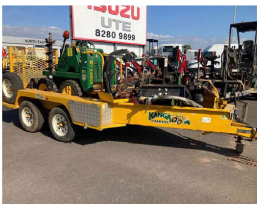
2004 Kanga Loaders DW625 2344 hours, 4 in 1 bucket, chain trencher, auger drive with auger, road sweeper.
