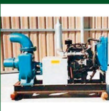
ISUZU DIESEL 6 X SELF PRIMING PUMP with secondhand 25 hp. AW54939-FM077-051-09. DPLIn27515. $6,310 + GST
