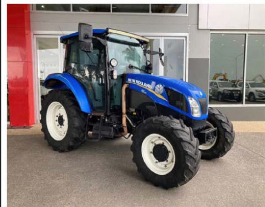
2018 New Holland T5.95 3268 Hours, 95 horsepower, 24 x 24 hi lo power shift transmission, wet clutch, 3 rear remotes, super steer front diff, UHF radio, LED light bar.
